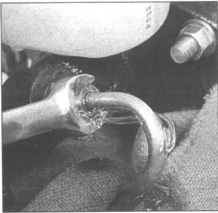
7.27 Have an assistant depress the brake pedal and hold it down, then loosen the fitting nut, allowing the air and fluid to escape - repeat this procedure on both fittings until the fluid is free of bubbles
