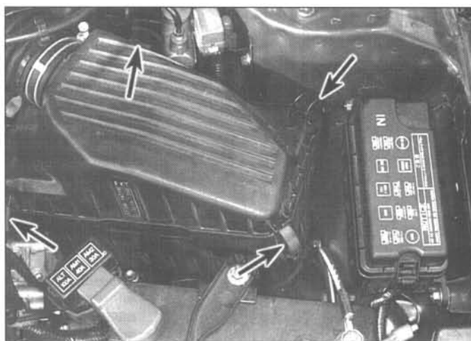
17.3 On fuel-injected models, the air cleaner cover may be secured by screws or clips (arrows)
