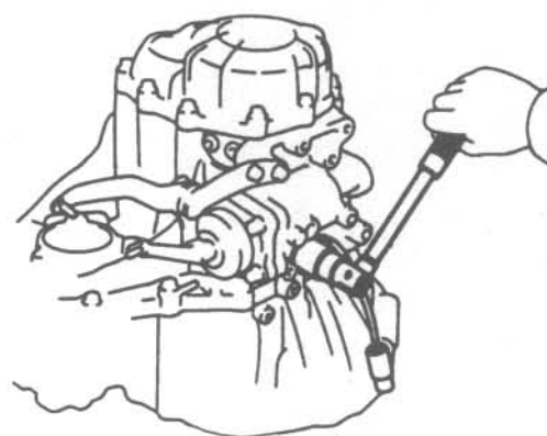
6.3 To remove the back-up light switch, simply unplug the electrical connector and unscrew the switch
