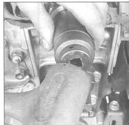
9.4 Drive the new seal into place with a hammer and a deep socket
