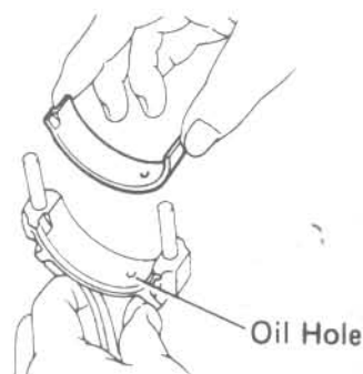
24.3 Align the oil hole in the bearing with the oil hole in the rod
