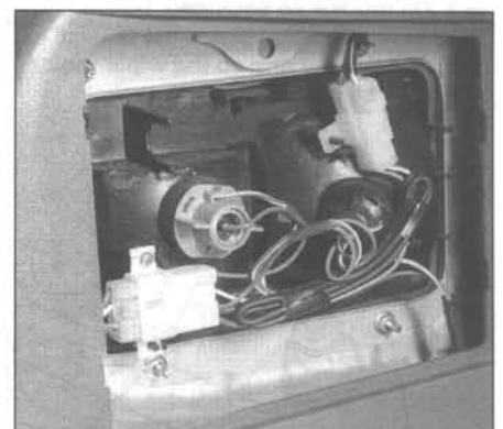
14.7a To replace a rear light on early models, open the small access door, turn the locking bulb holder counterclockwise, pull it out and pull the bulb straight out of the holder
