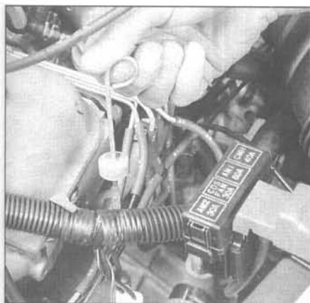
7.4 The automatic transaxle dipstick is located adjacent to the battery
