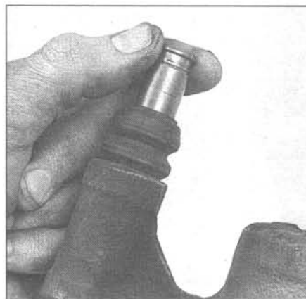
3.8a Push the sliding bushing on each side of the caliper up through the boot and pull it free, then remove the dust boots
