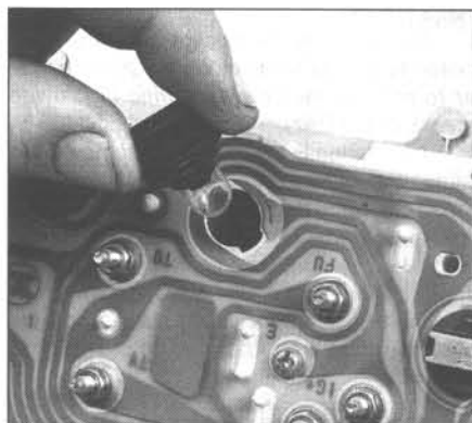
14.6 Instrument cluster bulbs have locking type bulb holders - to replace a bulb, simply turn the holder counterclockwise, pull it out, pull the bulb straight out of the holder, push in a new bulb, insert the holder into the back of the cluster and turn it clockwise to lock it into place
