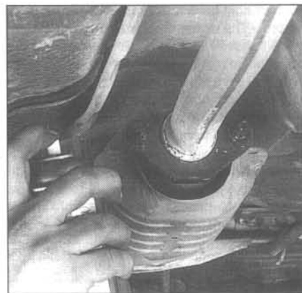
14.1c Exhaust system bolts and nuts, particularly those on the exhaust manifold and catalytic converters, can be very difficult to loosen - spraying them with a penetrant will free up the threads
