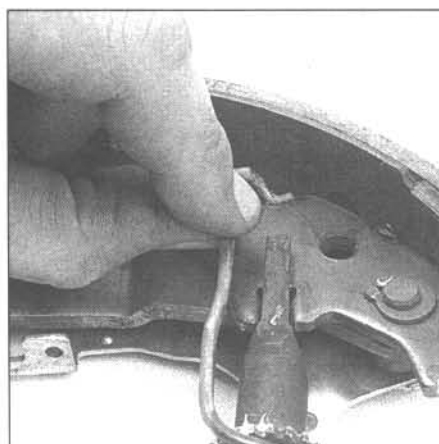
5.4p Install the adjuster assembly on the rear shoe (make sure the end fits properly into the slot in the shoe and hook the spring into the opening in the show)
