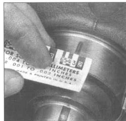
22.14 Compare the width of the crushed Plastigage to the scale on the envelope to determine the main bearing oil clearance (always take the measurement at the widest point of the Plastigage) - be sure to use the correct scale; standard and metric scales are included
