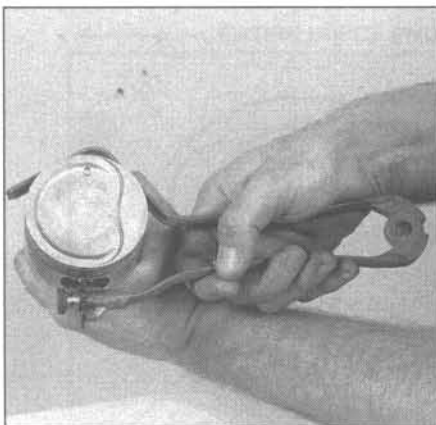
17.4a The piston ring grooves can be cleaned with a special tool, as shown here . . .
