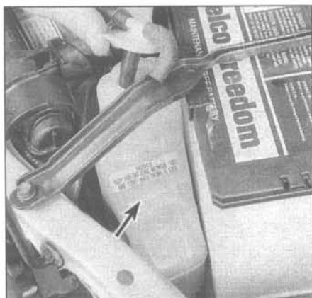
4.8 Make sure the coolant level in the reservoir is above the Low mark (arrow) - if it's below the mark, add more antifreeze/water mixture
