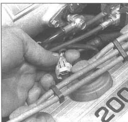
11.24 The injector connectors can be tricky to unplug - firmly depress the tang (arrow) to unlock each connector
