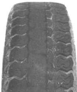
INCORRECT TOE-IN OR EXTREME CAMBER
