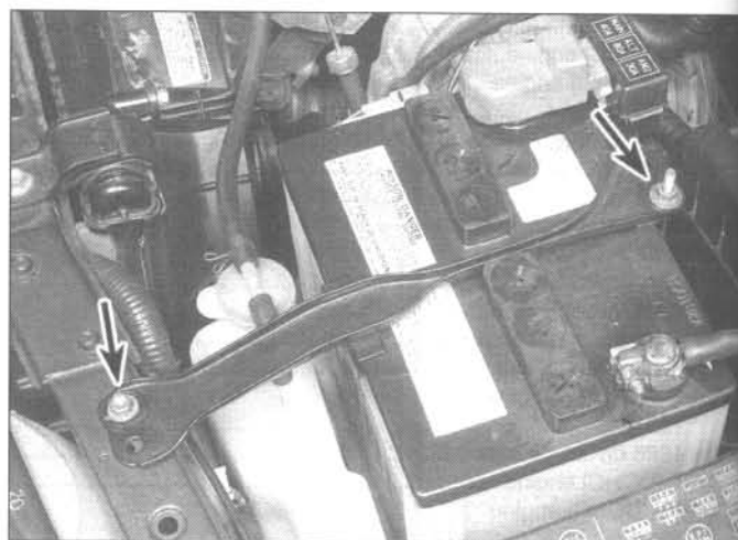
2.2 To remove the battery, detach the negative and positive cables, then remove the hold-down strap bolt and nut (arrows) and the strap, then carefully lift the battery out of the engine compartment
