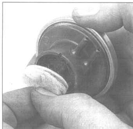
6.8b ... then pull out the two filters and blow them out with compressed air - be sure the coarse side of the outer filter faces the atmosphere (out) when reinstalling the filters
