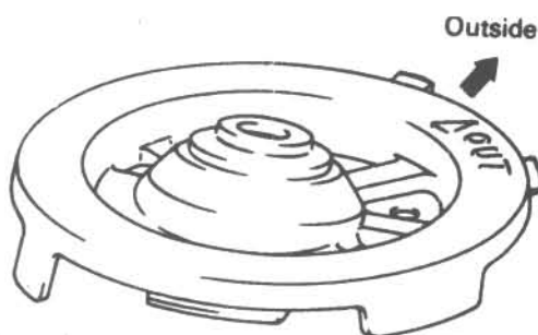
4.8 Remove the compressed spring assembly - keep the ends of the spring pointed away from your body!
