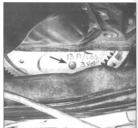
9.19 Mark the torque converter and driveplate so they can be reinstalled in the same relative positions, then remove each of the torque converter-to-driveplate bolts (arrow)
