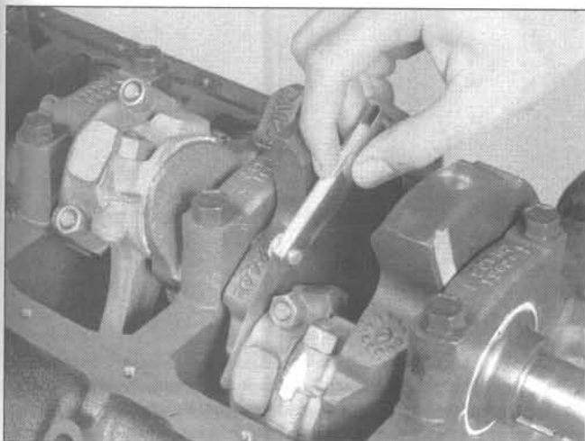
12.3 Check the connecting rod side clearance with a feeler gauge as shown here
