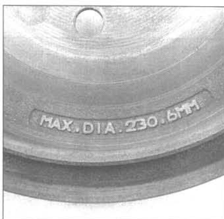
5.5 The maximum drum diameter is cast into the inside of the rear drums
