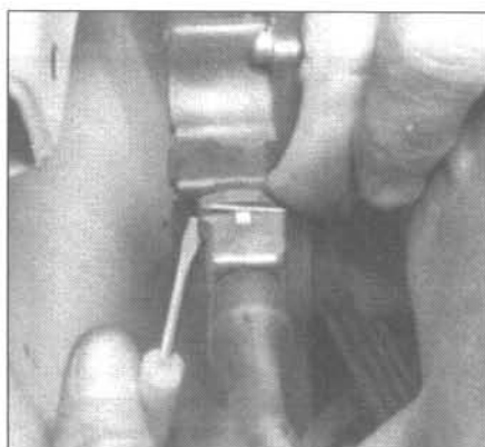
11.7 Pry the spring clip up far enough to release the electrical connector plug from the throttle position sensor (TPS) and unplug the connector
