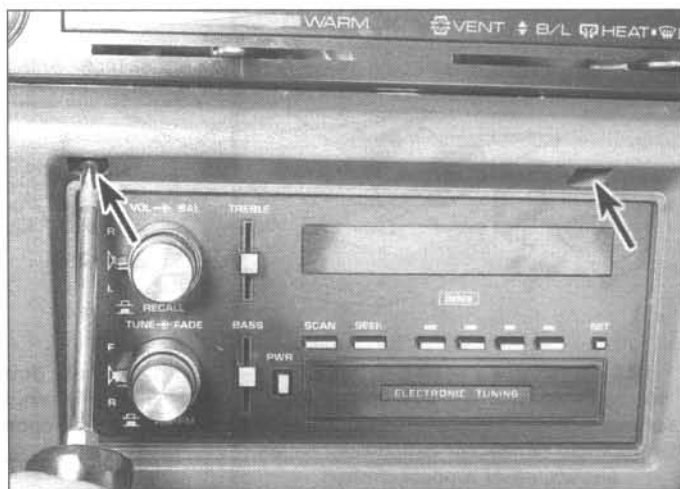
11.3b . . . then remove these two radio trim panel screws (arrows) and the trim panel
