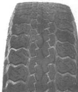
FEATHERING DUE TO MISALIGNMENT
