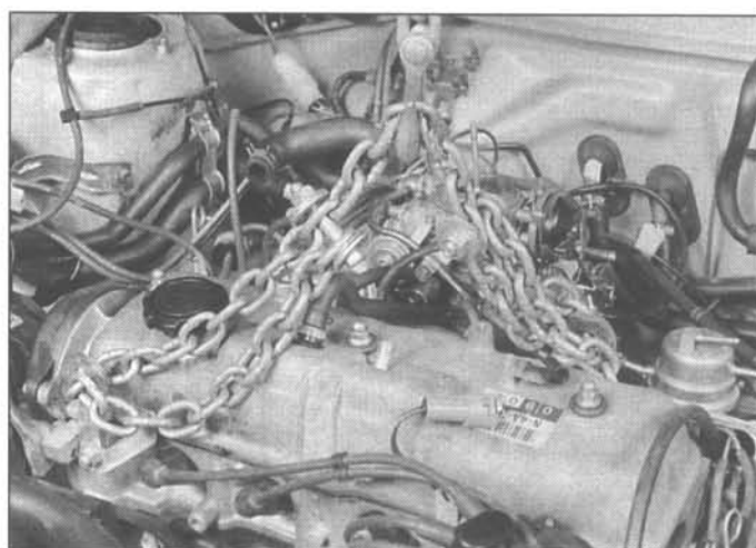
5.16 Attach a sling to the lifting brackets on the engine
