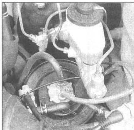
34.2 The evaporative emissions (charcoal) canister is located below the brake master cylinder - check the hoses for cracks and other damage
