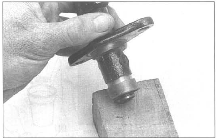
5.10 Invert the cylinder and tap it against a block of wood to eject the piston
