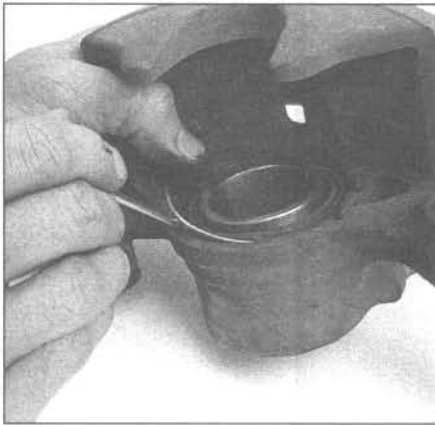
3.4c Using a screwdriver, remove the piston dust bolt retaining ring
