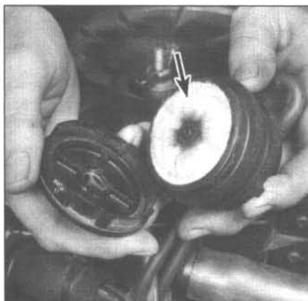
8.24 Remove the HAC cover, peel the filter out, clean it with compressed air, inspect it and, if necessary, replace it
