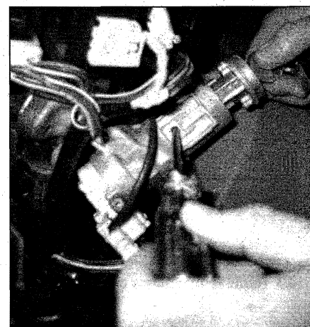
8.8 With the lock cylinder in the ACC position, depress the retaining pin with a small screwdriver, then pull the cylinder straight out
