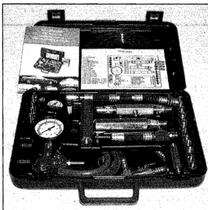
3.3a A fuel pressure testing kit like this should contain all the necessary fittings and adapters, along with the fuel pressure gauge, to test most automotive systems
