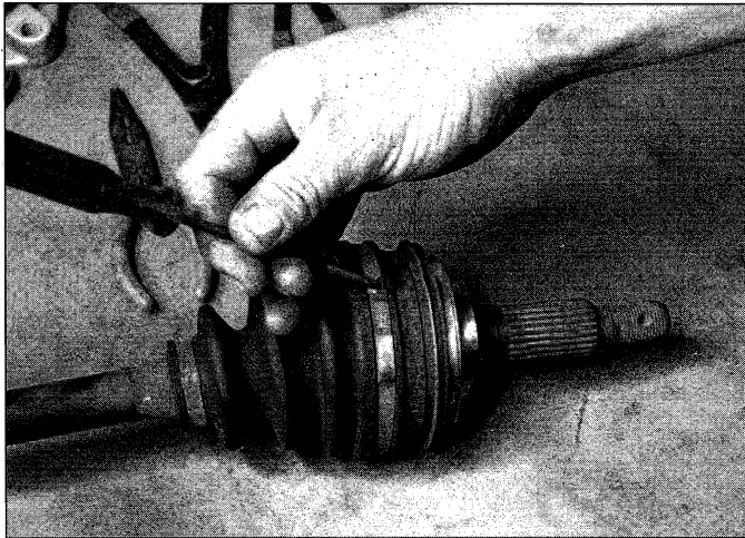
11.3 Lift the tabs on all the boot clamps with a screwdriver, then open the clamps
