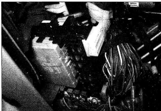
3.1a The interior fuse box is tucked up under the instrument panel, to the left of the steering column - it's fairly difficult to reach
