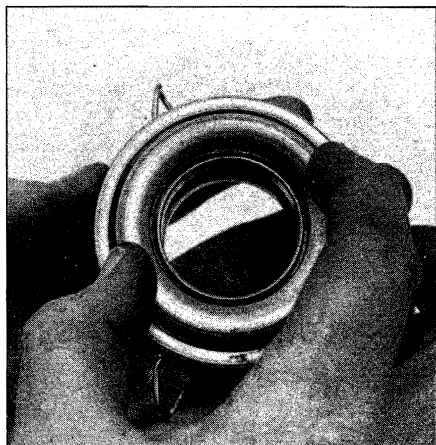
4.4 To check the operation of the bearing, hold it by the outer race and rotate the inner race while applying pressure - the bearing should turn smoothly - if it doesn't, replace it
