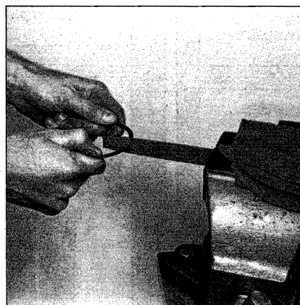
9.15 If the ring end gap is too small, clamp a file in a vise as shown and file the piston ring ends - be sure to file the ends squarely and finish by removing all raised material or burrs with a fine stone
