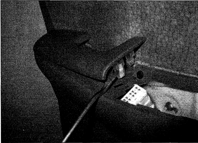
11.5a Pry the armrest up with a screwdriver or trim tool . . .
