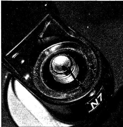
11.7 Lift the end cap to access the wiper arm nut, remove the nut, then make a reference mark before removing the arm
