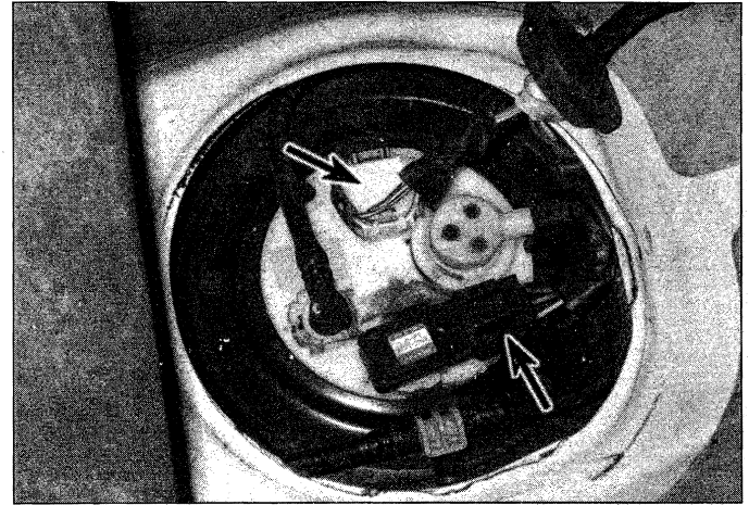
5.5a Disconnect both of the electrical connectors
