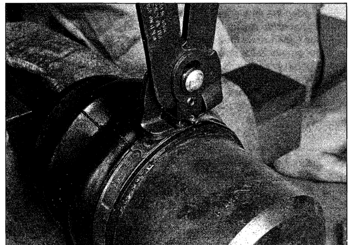
11.12b You'll need a special boot clamp installation tool like this one to tighten the new clamps; follow the instructions provided by the tool manufacturer
