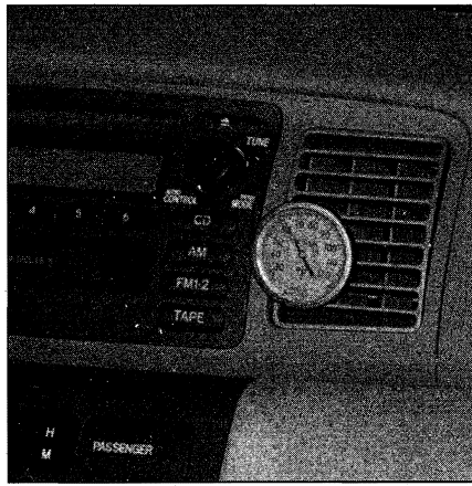
12.10 Check the temperature of the output air in the center register with a thermometer - it should be 35-40 degrees below the ambient air temperature
