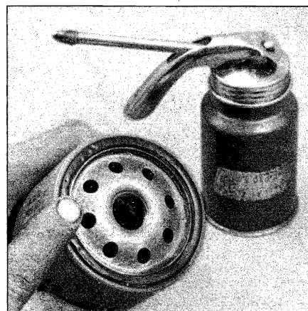
6.14 Lubricate the oil filter gasket with clean engine oil before installing the filter on the engine
