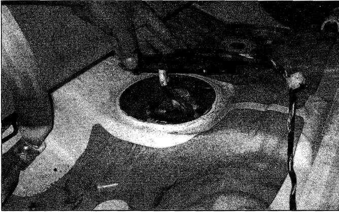
5.4 On 2003 and 2004 models, pry the fuel pump access cover off (it's secured by butyl tape). On 2005 models it's secured by four screws
