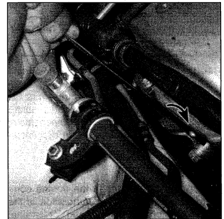
10.4 To release the tension on the drivebelt, place a long wrench or socket and ratchet on the hex-shaped boss, then turn the tensioner clockwise
