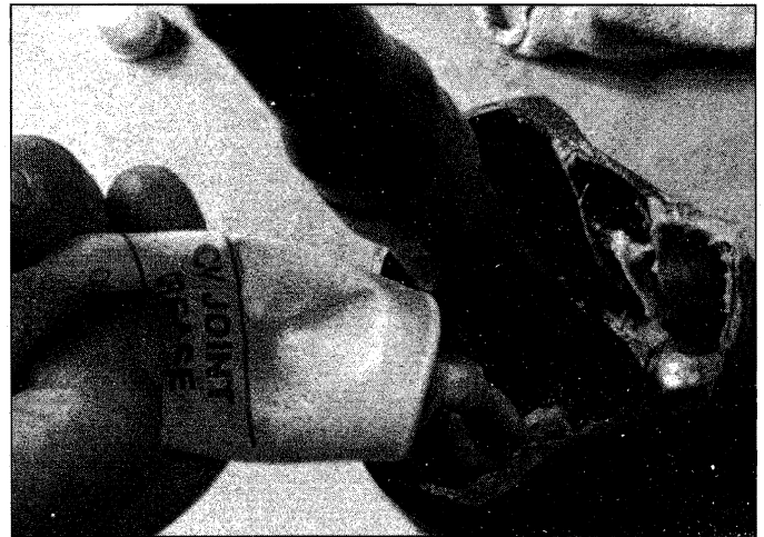
11.10c Install the boot and clamps onto the axleshaft, then insert the tripod into the housing, followed by the rest of the grease
