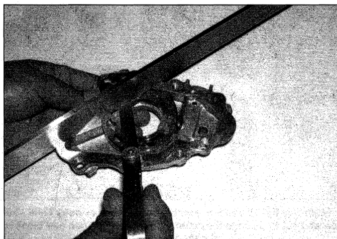
15.8b Using a straightedge and feeler gauge, measure the rotor-to-cover clearance
