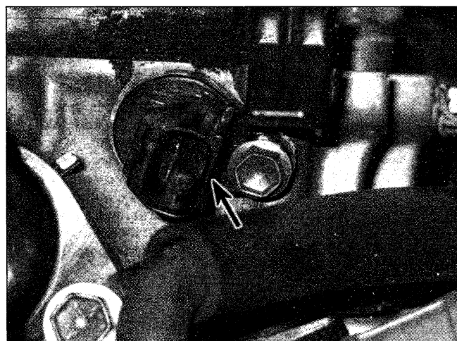
8.1 The camshaft position sensor mounts with one bolt to the cylinder head (connector removed for clarity)
