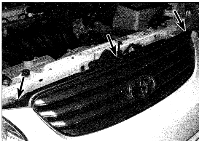
24.1 Along the top of the grille, remove the screws at each side and the pushpin at the center, then disengage the clips at the bottom and pull the grille forward and out
