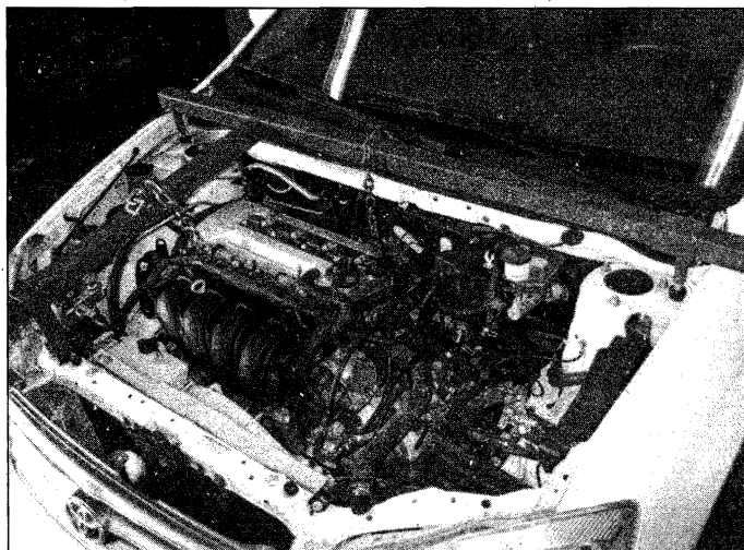
7.12 Support the engine with an engine support fixture (these are available at most tool rental yards and some auto parts stores)
