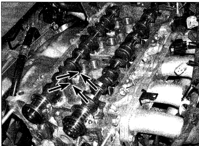
8.20 Place the camshafts in the cylinder head with the No.1 cylinder lobes pointing inward at approximately a 30 degree angle
