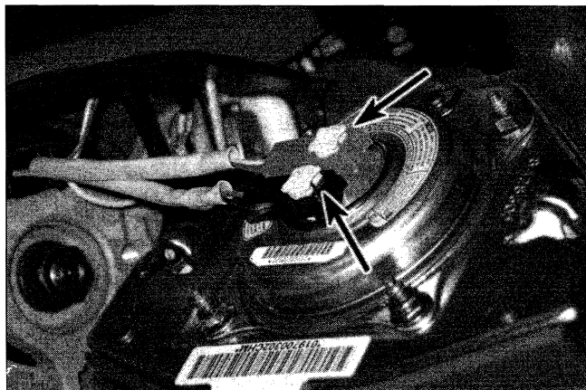
14.3 Lift the airbag module straight out from the steering wheel, then disconnect the electrical connectors at the back of the module
