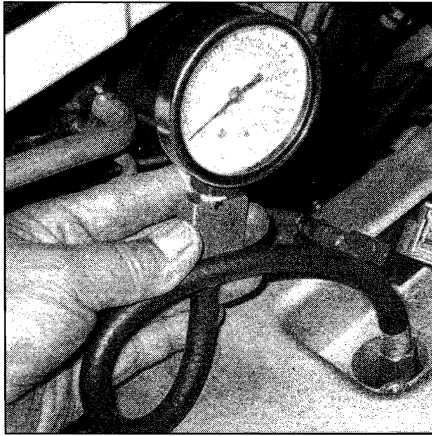
3.6 Use a compression gauge with a threaded fitting for the spark plug hole, not the type that requires hand pressure to maintain the seal - be sure to open the throttle valve as far as possible during the test
