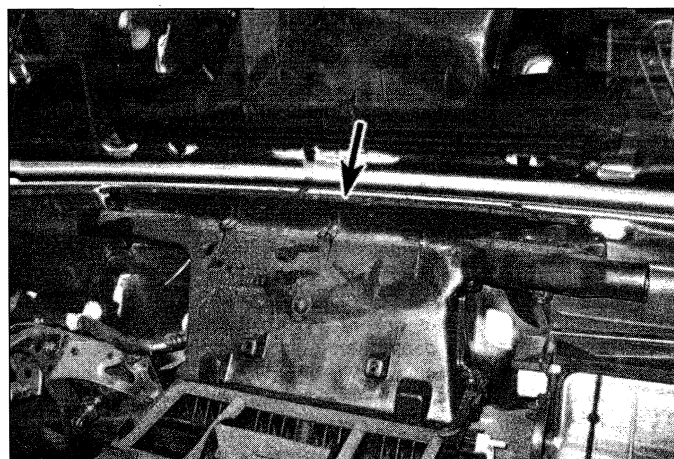
10.10 Remove the defroster duct from the top of the heat/AC housing
