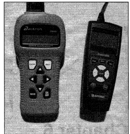
2.2 Scanners like these from Actron Scantool and AutoXray are powerful diagnostic aids - they can tell you just about anything you want to know about your engine management system
