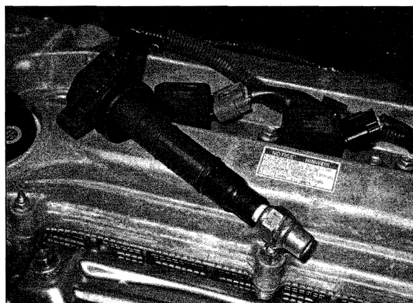
6.2 To use a calibrated ignition tester (available at most auto parts stores), remove one coil and plug the tester into the boot, clip the tester to a good ground, then crank the engine over - if there is enough voltage to fire the test plug, bright blue spark will be clearly visible between the electrode tip and the tester body
