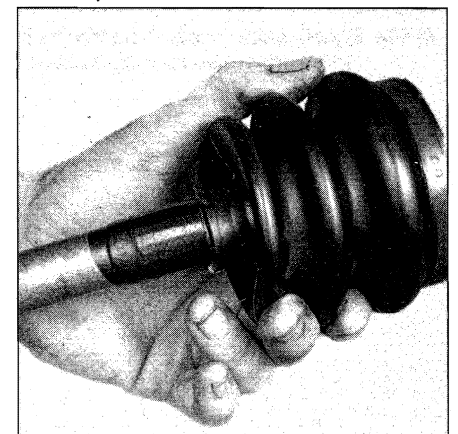
11.10a Wrap the splined area of the axleshaft with tape to prevent damage to the boots when removing or installing them
