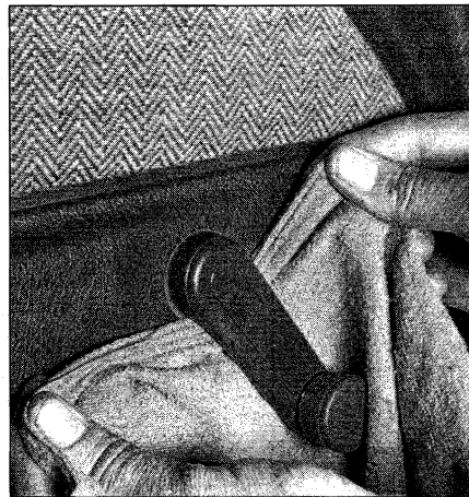
11.2a Work a cloth up behind the regulator handle and move it back-and-forth . . .
