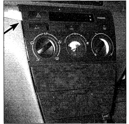
20.4a Use a trim tool to release the clips holding the lower trim panel and pull it out
