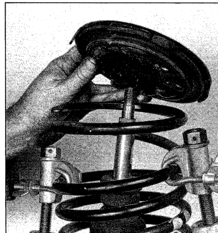
3.6 Remove the spring seat from the damper shaft
