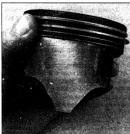
1.7 Uneven piston wear like this indicates a bent connecting rod
