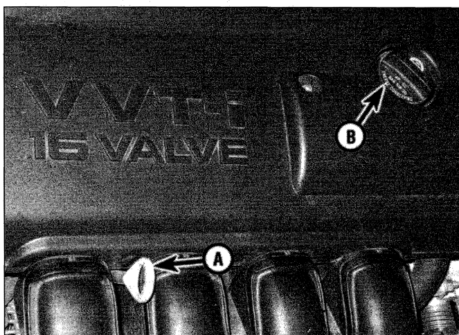
4.2 The engine oil dipstick (A) is located at the front of the engine - the oil filler cap (B) is in the valve cover
