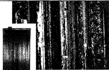
Microscopic detail of gouges Overplated copper alloy bearing gouged by cast iron debris
