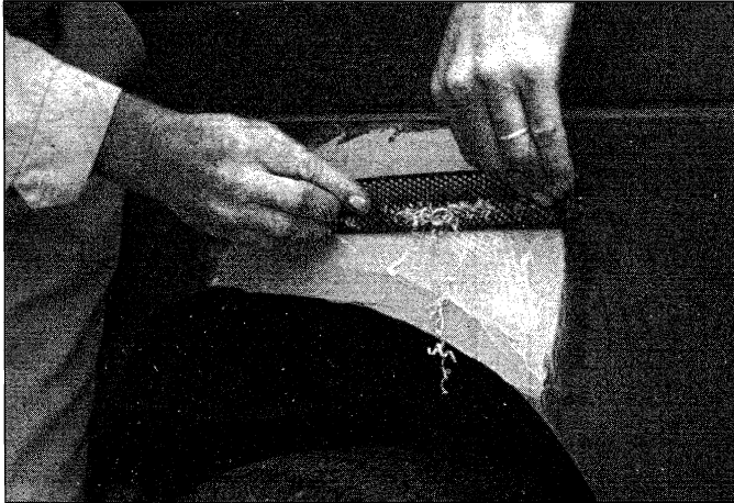
7 Let the filler harden until you can just dent it with your fingernail. Use a body file or Surform tool (shown here) to rough-shape the filler
