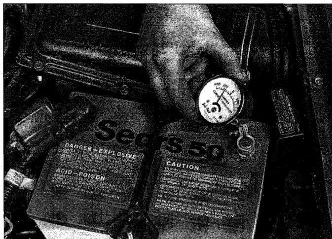
12.3 To use an inductive ammeter, simply hold the ammeter over the positive or negative cable (whichever is more accessible)
