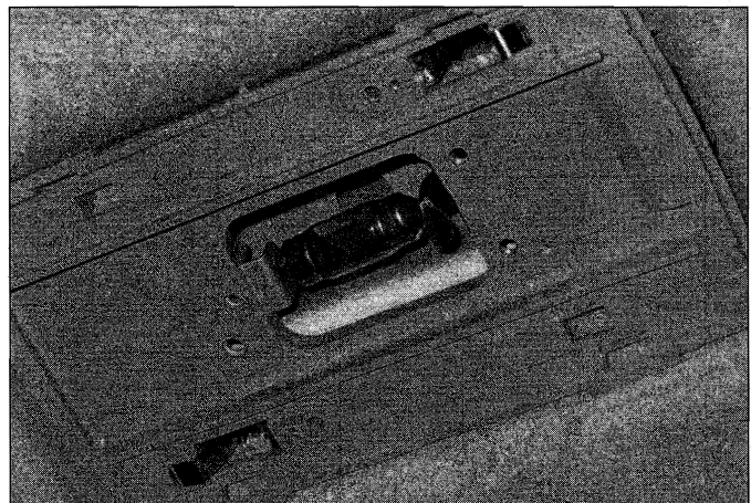
19.15 Carefully pry off the dome light lens using a flat-bladed screwdriver, then remove the bulb
