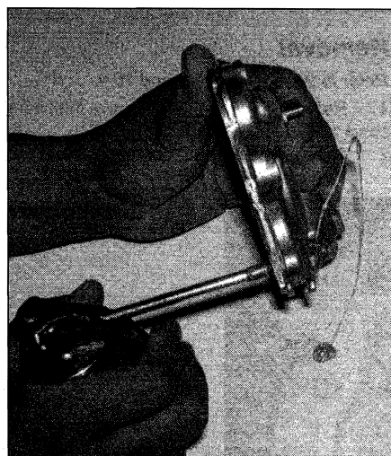
15.9 Check that the oil jet is free of debris (here, oil is being squirted into the port) - a blockage here will lead to an excessively worn timing chain and guides
