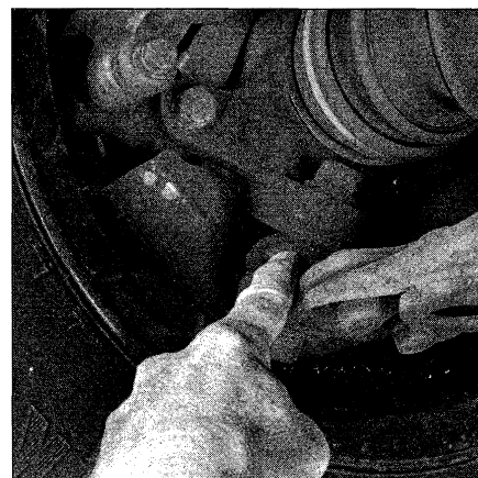
19.8 Push on the balljoint boot to check for damage
