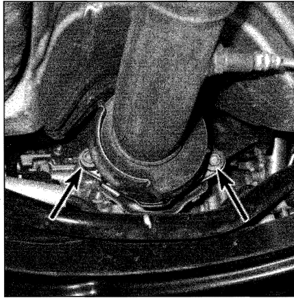
14.6 Remove the two spring-loaded bolts at the front of the catalytic converter
