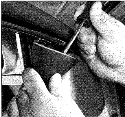
16.1b Detach the cover and lift it out (power mirror shown)
