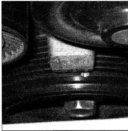
3.8 Align the groove in the damper with the "0" mark on the timing chain cover
