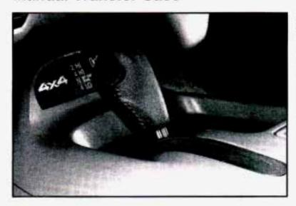
If your four-wheel drive vehicle has the manual transfer case, the transfer case shift lever is on the floor next to the driver. Use this lever to shift into and out of four-wheel drive.
