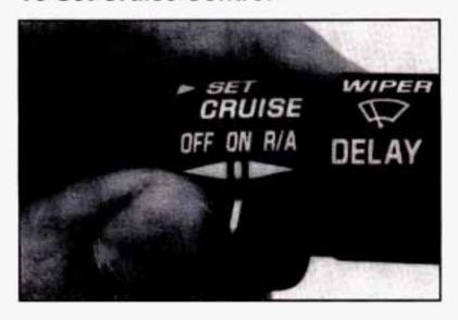
Move the Cruise Control switch to ON.
