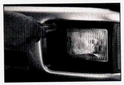
Remove the screws from the headlamp retainer.
