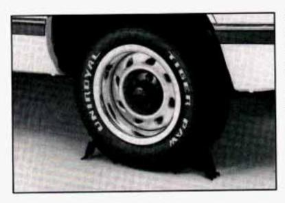
Before you start, block the front and rear of the tire farthest away from the one being changed. Put your spare tire near the flat tire.
