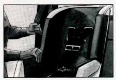
To tighten the belt, feed the shoulder belt into the retractor while you push down on the child restraint.
