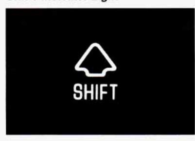
This amber SHIFT indicator light is at the top of the instrument cluster of vehicles with manual transmissions. Shifting when the indicator light is on will help you get the best fuel economy. See "SHIFT Light" in this section.
