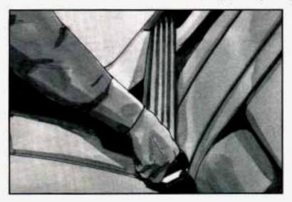
Pull the rest of the shoulder belt all the way out of the retractor to set the lock.
