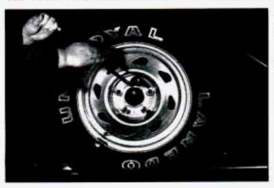
Use the socket end of your wheel wrench to remove the wheel nuts that secure the tire to the carrier. Then, lift the tire off its mounting bracket.
