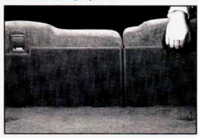
The rear seat release handles are in the upper center of the rear of the seatbacks. Push back on the seatbacks as you pull up on the handles.
