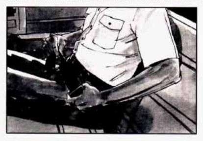
When you sit in the center front seating position, you have a lap safety belt, which has no retractor. To make the belt longer, tilt the latch plate and pull it along the belt.
