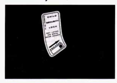
With this feature, you can lock the rear doors so they can't be opened from the inside by passengers.
