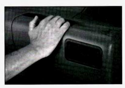
To open your glove box, squeeze the lever at the top of the glovebox and pull the handle towards you to lower the door. Two cup depressions are provided for your convenience, but the glovebox should not be open while driving.
