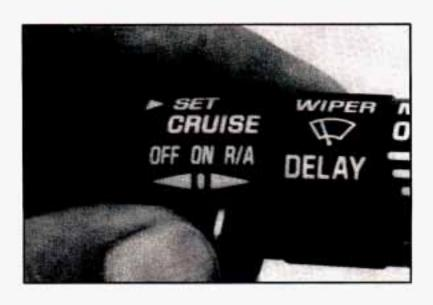
Move the Cruise switch from ON to R/A (Resume/Acceler ate). Hold it there until you get up to the speed you want, and then release the switch.
