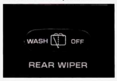
You control your rear window wiper/washer from a switch on your instrument panel located below the rear defogger switch.
