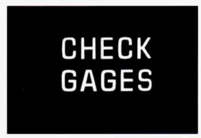
This amber CHECK GAGES light is above the fuel gage on the instrument cluster and will come on briefly when you are starting the engine.
