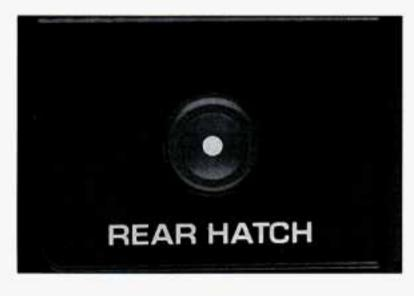
The electric hatch release lets you open your endgate glass by just pressing a button. The button is on the driver's side of the steering column.
