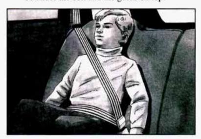
Buckle the belt around the child, and make sure that both the lap belt and the shoulder belt are secured properly. Make sure that the shoulder belt crosses the shoulder. See "Safety Belts, Rear Seat Passengers" in the Index.
