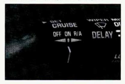
Use the accelerator pedal to get to the higher speed. Push the button at the end of the lever, then release the button and the accelerator pedal. You'll now cruise at the higher speed.
