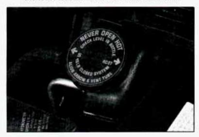
Then replace the pressure cap. At any time during this procedure if coolant begins to flow out of the filler neck, reinstall the pressure cap. Be sure the arrows on the pressure cap line up like this.
