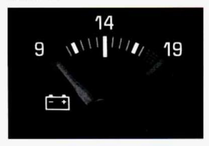
When your engine is not running, but the ignition is on (in the RUN position), this gage shows your battery's state of charge in DC volts.
