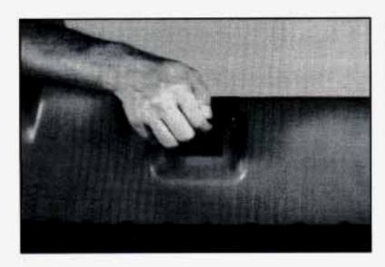
Open the glass and reach inside the endgate to lift the handle and open the endgate.
