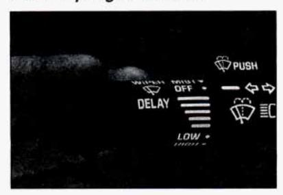
To change the headlamps from low beam to high or high to low, pull the Multifunction lever all the way toward you. Then release it.
