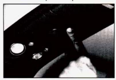
To install the garage door opener, first open the compartment door by pressing the latch forward.
