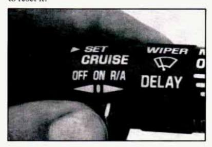
Once you're going about 25 mph (40 km/h) or more, you can move the Cruise Control switch from QN to R/A (Resume/Accelerate) for about half a second.
