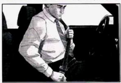
To make the lap part tight, pull down on the buckle end of the belt as you pull up on the shoulder belt.
