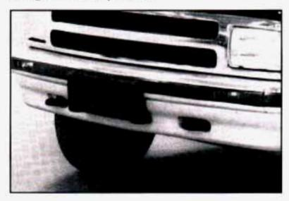
Your vehicle may be equipped with recovery hooks. The recovery hooks are provided at the front of your vehicle. You may need to use them if you're stuck off-road and need to be pulled to some place where you can continue driving.
