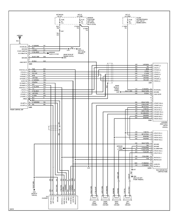
SYSTEM WIRING DIAGRAMS Premium Sound Radio Circuit, W/O CD Player (p. 56) 1996 Ford Explorer
