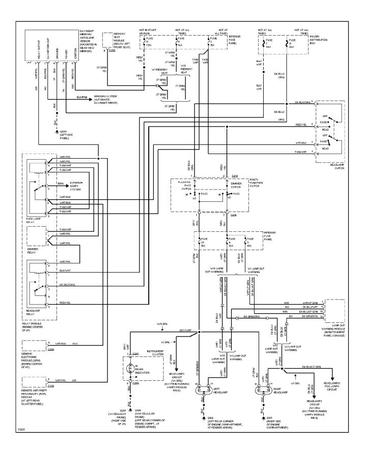
SYSTEM WIRING DIAGRAMS Headlamps Circuit, W/ DRL (p. 29)
