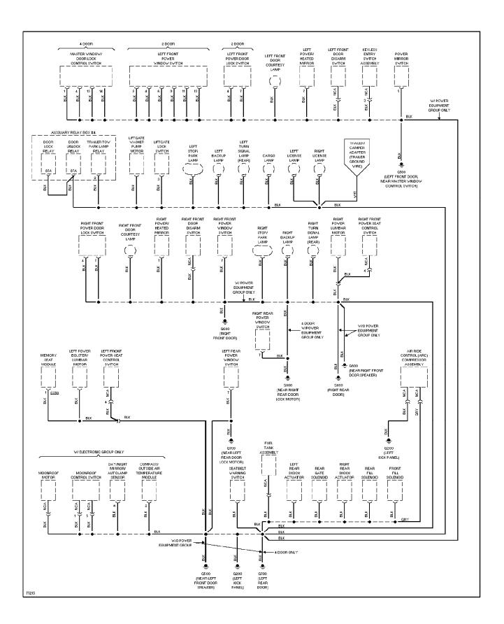
SYSTEM WIRING DIAGRAMS Ground Distribution Circuit (4 of 4) (p. 27) 1996 Ford Explorer
