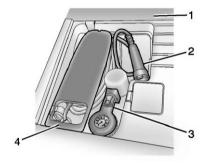
Open the rear hatch, lift the load support floor covering (1), and remove the charge cord (4). It is located near the tire sealant and compressor kit (3). Pull up on the charge cord handle (4) to release it from the handle clip.
