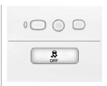
TCS can be turned off by pressing and releasing the TCS/ESC button on the overhead console. When TCS is turned off, comes on, and the appropriate DIC message also displays. See *Ride Control System Messages on page 5-49*. With TCS turned off, the system does not limit wheel spin. Driving should be adjusted accordingly. See *Traction Off Light on page 5-23*.
