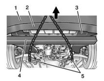
4. Place a 1.2 m (4 ft) X 102 mm (4 in) X 102 mm (4 in) wood beam (4) under the front cradle crossmember (3), and on top of both tow chains (5) to ensure the tow chains do not come into contact with the front fascia (1).
