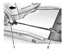
8. Secure the vehicle to the flatbed (2) using nonabrasive straps (1) through all four wheel openings and secure the straps to the flatbed (2).
