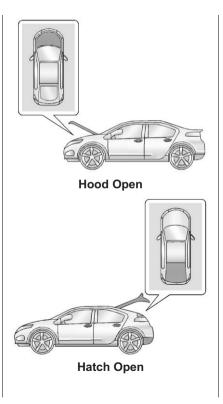
The DIC indicates when a door, the hood, or the hatch is open. The light displays the open area as shaded.
