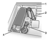
Open the rear hatch, lift the load support floor covering (1), and remove the charge cord (4). It is located near the tire sealant and compressor kit (3). Pull up on the charge cord handle (4) to release it from the handle clip.
