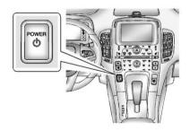
The vehicle has an electronic pushbutton start. The POWER  $\circlearrowleft$  button light flashes when the driver door is open and the vehicle is not on. The flashing light will eventually time out. The POWER  $\circlearrowleft$  button light is on steady when in ON/RUN power mode. When the vehicle is turned off, the POWER  $\circlearrowleft$  button light will turn off.
