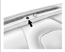
The vehicle has a Charging Status Indicator (CSI) at the center of the instrument panel near the windshield.
