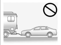
Notice: If the vehicle is towed with all four wheels on the ground, the drive unit could be damaged. Repairs would not be covered by the vehicle warranty. Do not tow the vehicle with all four wheels on the ground.
