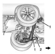
Notice: When using tow straps to move the vehicle, damage may occur if the tow straps contact the rear fascia. Do not let the tow straps contact the rear fascia.
