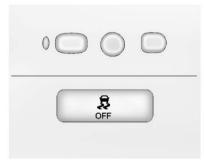
To turn off both StabiliTrak and TCS, press and hold the TCS/ ESC button on the overhead console, until and illuminate and the appropriate DIC message is displayed. See Ride Control System Messages on page 5-49.
