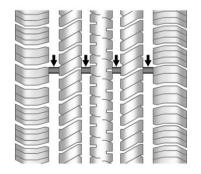
Treadwear indicators are one way to tell when it is time for new tires. Treadwear indicators appear when the tires have only 1.6 mm (1/16 in) or less of tread remaining. See *Tire Inspection on page 10-52* and *Tire Rotation on page 10-53*.
