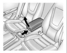
To remove the armrest storage bin, push the button and lift the armrest storage bin up.
