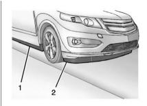
If the vehicle is parked off the shoulder of the road, at an angle that it cannot be pulled onto a flatbed, a hook/chain can be placed into either of the front torque box openings to pull the vehicle onto a flat surface. Make sure that the chains do not come in contact with the rocker panel (1) or the front fascia (2).
