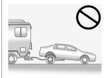
Notice: Towing the vehicle from the rear, with the front wheels on the ground, could damage the drive unit, and front fascia. Do not tow the vehicle from the rear with the front wheels on the ground.
