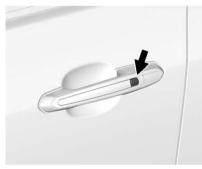
When the Remote Keyless Entry (RKE) transmitter is within 1 m (3 ft) of the driver door, the door can be locked and unlocked by pressing the door handle button. When unlocking from the driver door, the first press will unlock only that door; press again within five seconds to unlock all passenger doors. See Remote Keyless Entry (RKE) System Operation on page 2-2.
