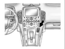
The vehicle has an Electric Parking Brake (EPB). The (P) switch is on the center stack. The EPB can always be activated, even if the vehicle is off. To prevent draining the 12-volt battery, avoid repeated cycles of the EPB system when the vehicle is off.
