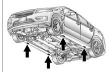
The front lifting points can be accessed from either side of the vehicle, behind the front tires.
