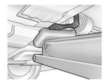
When lifting the vehicle from the front, place the service jack directly under the cradle mount. Ramps may be needed under the front tires to provide the necessary clearance for certain service jacks in this location.
