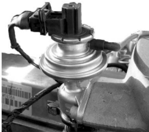
Hoover EGR System for IDI Engine (Including the EGR Valve Potentiometer)
