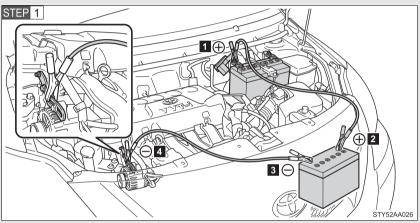
Connecting the jumper cables
