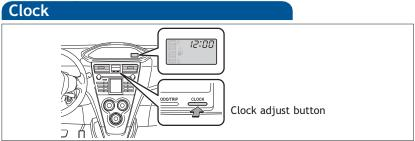
(1) Push and hold the CLOCK button to enter adjustment mode. (2) Press CLOCK button to adjust hours. (3) Wait five seconds to adjust the minutes.(4) Wait another five seconds for process to complete.
