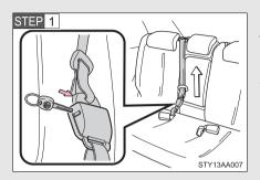
Insert the key into the hole on the center seat belt buckle to release tab (with hooked end), and allow the belt to retract.
