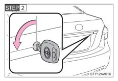
Turn the master key counterclockwise to lock the trunk opener feature.
