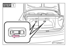
Vehicles with split rear seats: Move the security lock levers to lock the rear seatbacks.
