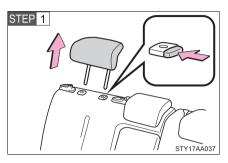
Remove the head restraint.
