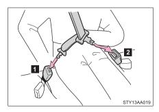
Make sure that the buckle **I** is securely latched for ready use of the center seat belt.
