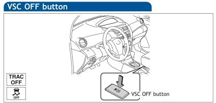
The VSC OFF button is used to switch between modes related to the TRAC and VSC.
