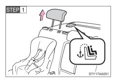
Remove the head restraint.
