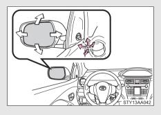
Adjust the mirror up, down, in or out using the lever.
