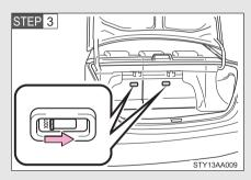
Check that the security lock levers in the trunk are in unlock position.
