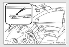
Close the doors, trunk and hood, and lock all doors using the key (vehicles without wireless remote control) or wireless remote control door lock function (vehicles with wireless remote control). The system will be set automatically after 30 seconds.
