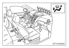
When the dial is set to **\***, air flows to the feet and the wind-shield defogger operates.
