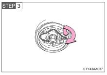
Release the bulb retaining spring.
