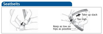
If belt is fully extended, then retracted even slightly, it cannot be re-extended beyond that point, unless fully retracted again. This feature is used to help hold child restraint systems securely.
