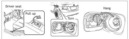
**NOTE:** Tighten until one click is heard. If the cap is not tightened enough, Check Engine "  $\bigcirc$  " indicator may illuminate.
