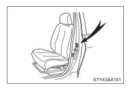
For the GAWR, see the Certification Label. For the maximum load of the tire, see the load limit at maximum cold tire inflation pressure mentioned on the sidewall of the tire. ( $\rightarrow$ P. 346)
