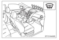
When the dial is set to  $\langle \mu\mu\rangle$ , air flows to the windshield and side windows to defog them.
