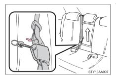
To release the hooked end tab, insert the vehicle's key into the hole on the buckle.
