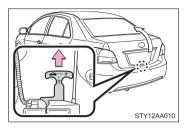
The trunk lid can be opened by pulling up on the glow-in-the-dark lever located on the inside of trunk lid.
