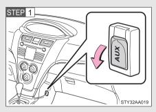
Connect the portable audio device.
