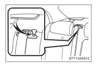
1 Make sure that the seatback is securely locked in position by lightly rocking it back and forth.
