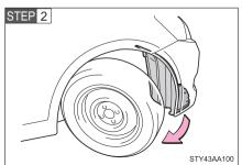
Partly remove the fender liner.
