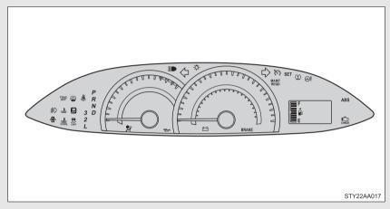
Instrument cluster (vehicles without Optitron type meters)
