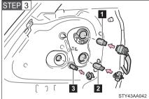
Partly remove the cover and turn the bulb bases counterclockwise.
