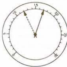
9. BURNED OR WARPED VALVE Regular, evenly spaced down-scale flick about 4 in.
