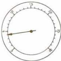
4. INTAKE LEAK Low steady reading.
