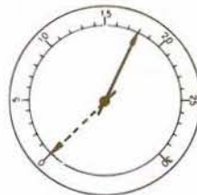
6. WORN RINGS, DILUTED OIL Drops to 0, then rises to 18 when accelerator is rapidly depressed and released.
