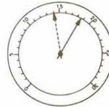
7. STICKING VALVE(S) Normally steady. Intermittently flicks downward about 4 in.
