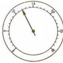
2. LATE IGNITION TIMING About 2 inches too low at idle.
