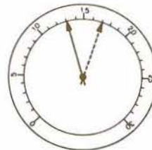
12. IMPROPER IDLE MIXTURE Floats slowly between 13-17 in.
