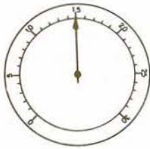
1. NORMAL READING Reads 15 in. at idle.
