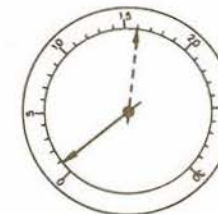
15. RESTRICTED EXHAUST SYSTEM Normal when first started. Drops to 0 as rpm increases. May eventually rise to about 16.
