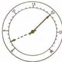
5. NORMAL READING Drops to 2, then rises to 25 when accelerator is rapidly depressed and released.
