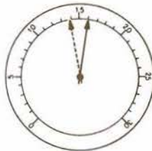
13. SMALL SPARK GAP or DEFECTIVE POINTS Slight float between 14-16 in.
