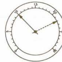
11. WEAK VALVE SPRINGS Violent oscillation (about 10 in.) as rpm increases. Often steady at idle.
