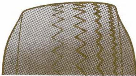
Wheel Alignment – Worn more on one side than the other. Edges of tread feathered.
