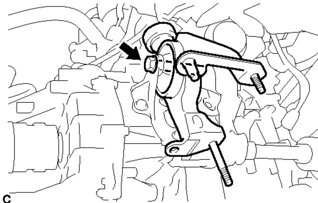
Fig. 168: Identifying Engine Mounting Bracket With Bolt Courtesy of TOYOTA MOTOR SALES, U.S.A., INC.
