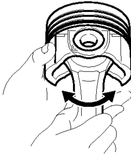
Fig. 461: Checking Fitting Condition Between Piston And Piston Pin Courtesy of TOYOTA MOTOR SALES, U.S.A., INC.
