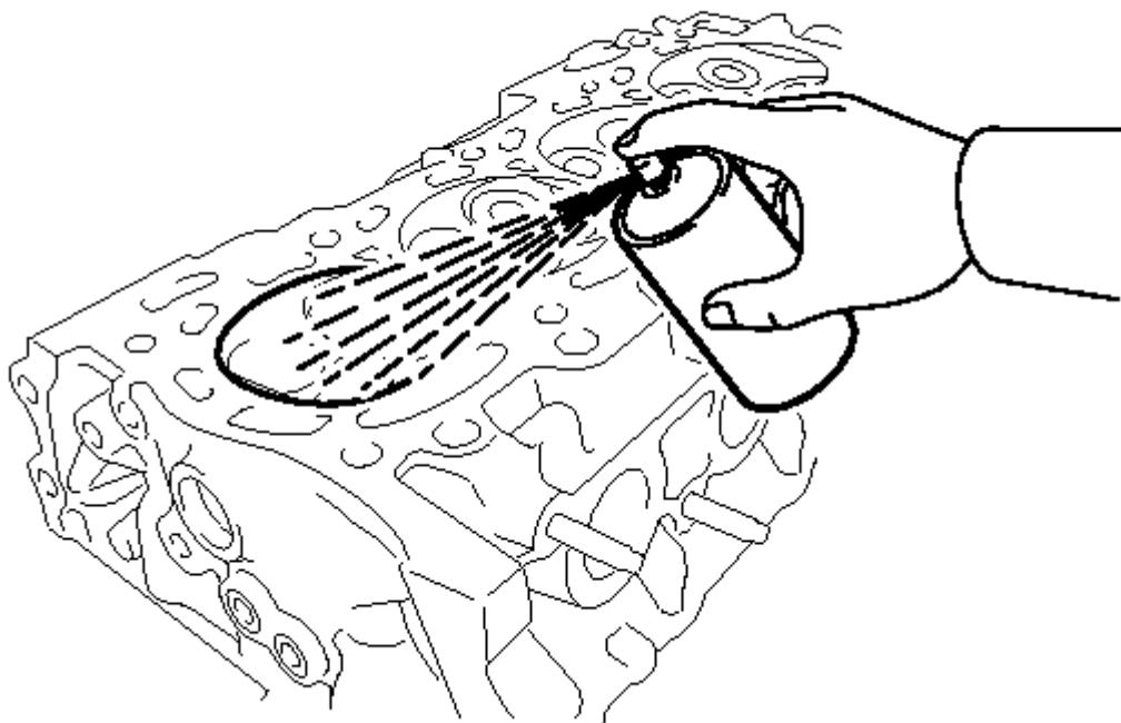
Fig. 373: Inspecting Cylinder Head For Cracks Courtesy of TOYOTA MOTOR SALES, U.S.A., INC.
