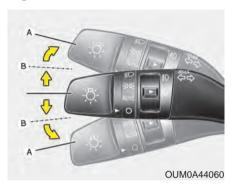
The ignition switch must be on for the turn signals to function. To turn on the turn signals, move the lever up or down (A). The green arrow indicators on the instrument panel indicate which turn signal is operating. They will self-cancel after a turn is completed. If the indicator continues to flash after a turn, manually return the lever to the OFF position.
