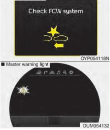
When the FCWS is not working properly, the warning message will come on for a few second. After the message disappears, the master warning light will illuminate.
