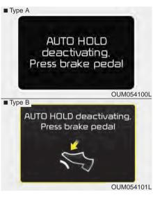
When the conversion from Auto Hold to EPB is not working properly a warning will sound and a message will appear.
