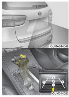
The rearview camera will activate with the ignition switch ON and the shift lever in the R (Reverse) position.
