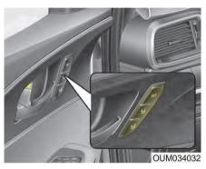
A driver position memory system is provided to store and recall the driver seat and outside rearview mirror position with a simple button operation. By saving the desired position into the system memory, different drivers can reposition the driver seat based upon their driving preference. If the battery is disconnected, the desired seat position memory will need to be re-saved.
