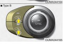
This is used to select the outside (fresh) air position or recirculated air position.
