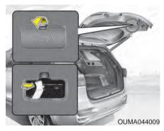
Your vehicle is equipped with an emergency liftgate (tailgate) safety release lever located on the bottom of the liftgate (tailgate). When someone is inadvertently locked in the cargo area, the liftgate (tailgate) can be opened by pushing the release lever and pushing open the liftgate (tailgate).
