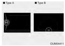
This indicator displays which automatic transaxle shift lever is selected.
