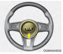
To sound the horn, press the horn symbols on your steering wheel. Check the horn regularly to be sure it operates properly.
