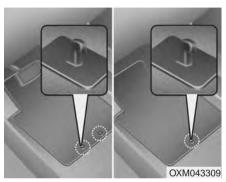
When using a floor mat on the front floor carpet, make sure it attaches to the floor mat anchor(s) in your vehicle. This keeps the floor mat from sliding forward. The following must be observed when installing ANY floor mat to the vehicle.
