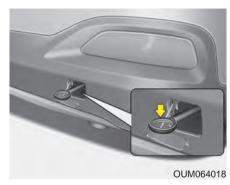
If towing is necessary, we recommend you to have it done by an authorized Kia dealer or a commercial tow truck service. If towing service is not available in an emergency, your vehicle may be temporarily towed using a cable or chain secured to the emergency towing hook under the front (or rear) of the vehicle. Use extreme caution when towing the vehicle. A driver must be in the vehicle to steer it and operate the brakes.
