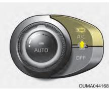
Press the A/C button to turn the air conditioning system on (indicator light will illuminate).
