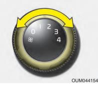
The ignition switch must be in the ON position for fan operation.
