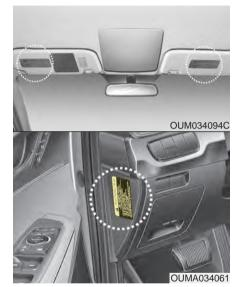
Air bag warning labels, some required by the Canada Motor Vehicle Safety Standards (CMVSS), are attached to the sunvisor to alert the driver and passengers of potential risks of the air bag system.
