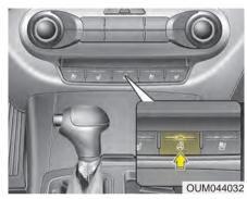
With the ignition switch in the ON position, pressing the heated steering wheel button warms the steering wheel. The indicator on the button will illuminate.
