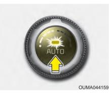
1. Press the AUTO button. The modes, fan speeds, air intake and air-conditioning will be controlled automatically by setting the temperature.
