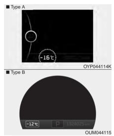
This gauge indicates the current outside air temperatures by 1°C (1°F).
