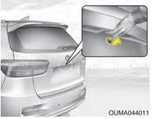
• Press the liftgate (tailgate) handle switch carrying the smart key with you.
