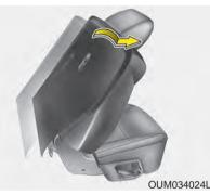
3. Fold the 2nd row seatback and push the seat to the farthest forward position.
