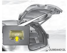
The driver may set the height of a fully opened liftgate (tailgate) by following the below instruction.
