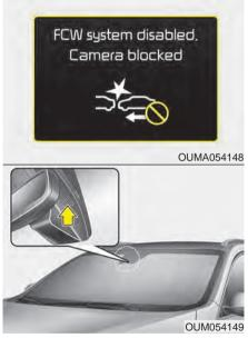
The message will appear when camera's field of view is covered by some objects. The system stops until the field of view is normal. Check the windshield around the camera view area. If the system does not work normally even though camera's field of view is cleared, take your vehicle to an authorized Kia dealer and have the system checked.
