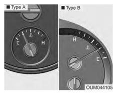
This gauge indicates the temperature of the engine coolant when the ignition switch or Engine Start/Stop button is ON. If the gauge pointer moves beyond the normal range area toward the "H" position, it indicates overheating that may damage the engine.
