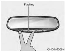
To erase the three programmed buttons (individual buttons cannot be erased):
