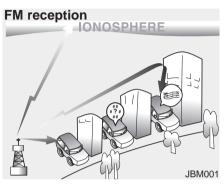
This can be due to factors, such as the distance from the radio station, closeness of other strong radio stations or the presence of buildings, bridges or other large obstructions in the area.
