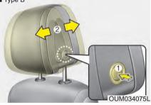
The headrest may be adjusted forward to 4 different positions by pulling the headrest forward to the desired detent. To adjust the headrest to it's full rearward position.
