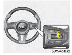
• Press the CRUISE button (the CRUISE indicator light in the instrument cluster will go off).
