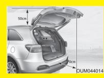
Make sure that there are no people or objects in the path of the power liftgate (tailgate) (or smart liftgate (tailgate)) prior to use. Serious injury, damage to the vehicle or damage to surrounding objects may result if contact with the power liftgate (tailgate) (or smart liftgate (tailgate)) occurs.
