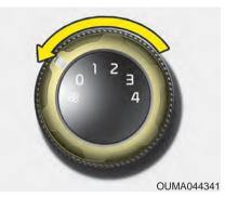
To turn off the blowers, turn the fan speed control knob to the "0" position.
