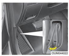
1. Pull the release lever to unlatch the hood. The hood should pop open slightly. Open the hood after turning off the engine on a flat surface, shifting the shift lever to the P (Park) position and setting the parking brake.
