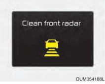
If the radar or cover is dirty or obscured with foreign matter such as snow, this message will appear. In this case, the system may not function temporarily, but it does not indicate a malfunction of the Advanced Smart Cruise Control System. Clean the radar or cover by using a soft cloth.
