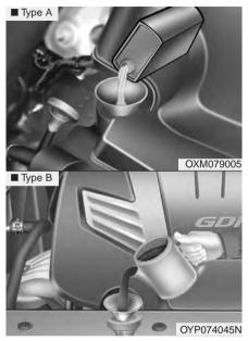
Use only the specified engine oil. (Refer to "Recommended lubricants and capacities" in section 8.)
