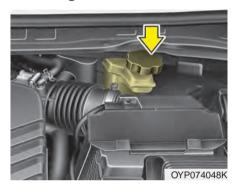
Check the fluid level in the reservoir periodically. The fluid level should be between MAX (Maximum) and MIN (Minimum) marks on the side of the reservoir.
