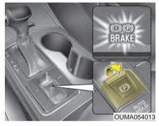
To apply the EPB (electric parking brake):
