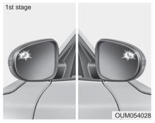
If a vehicle is detected within the boundary of the system, a warning light will illuminate on the outside rearview mirror.
