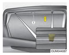
To avoid injury or damage to the side curtain and door moldings, lower side curtain by the handle all the way back to the stowed position. Do not release handle after disengaging from the hooks on the door.
