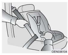
5. Remove as much slack from the belt as possible by pushing down on the child restraint system while feeding the shoulder belt back into the retractor.
