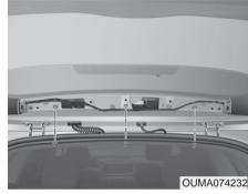
4. Loosen the retaining nuts and remove the spoiler.
