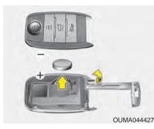
A smart key battery should last for several years, but if the smart key is not working properly, try replacing the battery with a new one. If you are unsure how to use your smart key or replace the battery, contact an authorized Kia dealer.
