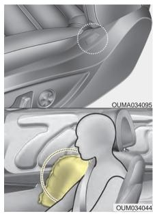
Your vehicle is equipped with a side air bag in each front seat. The purpose of the air bag is to provide the vehicle's driver and/or the front passenger with additional protection than that offered by the seat belt alone.
