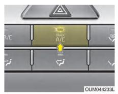
To select the MAX A/C, turn the fan speed control knob to the right then press the MAX A/C button.
