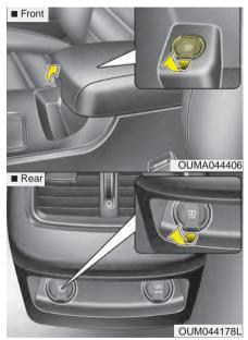
The USB charger is designed to recharge batteries of small size electrical devices using a USB cable. The electrical devices can be recharged when the Engine Start/Stop button is in ACC/ON/START position.
