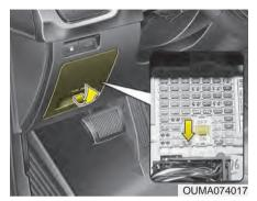
Always, put the fuse switch at the ON position.
