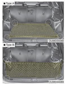
To keep items from shifting in the cargo area, you can use the holders located in the cargo area to attach the luggage net.
