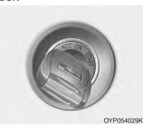
The steering wheel locks to protect against theft (if equipped). The ignition key can be removed only in the LOCK position.
