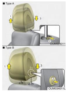
To raise the headrest, pull it up to the desired position (1). To lower the headrest, push and hold the release button (2) on the headrest support and lower the headrest to the desired position (3).
