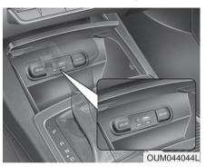
If your vehicle has an aux and/or USB(universal serial bus) port, you can use an aux port to connect audio devices, USB, or iPod<sup>®</sup>.
