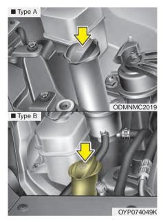
The reservoir is translucent so that you can check the level with a quick visual inspection.
