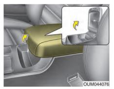
To open the center console storage, pull up the lever.
