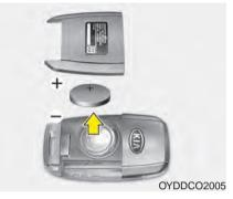
The transmitter uses a 3 volt lithium battery which will normally last for several years. When replacement is necessary, use the following procedure.
