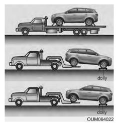
If emergency towing is necessary, we recommend having it done by an authorized Kia dealer or a commercial tow-truck service. Proper lifting and towing procedures are necessary to prevent damage to the vehicle. The use of wheel dollies or flatbed is recommended. For trailer towing guidelines information, refer to "Trailer towing" in section 5.
