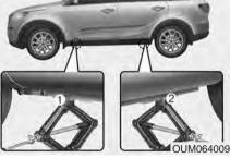
7. Place the jack at the front (1) or rear (2) jacking position closest to the tire you are changing. Place the jack at the designated locations under the frame. The jacking positions are plates welded to the frame with two tabs and a raised dot to index with the jack.
