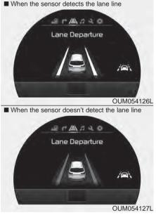
If the system detects that your vehicle is leaving the lane when the LDWS is operating and vehicle speed exceeds 60 km/h (37 mph), the warning operates as follows:
