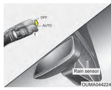
The rain sensor located on the upper end of the windshield glass senses the amount of rainfall and controls the wiping cycle for the proper interval. The more it rains, the faster the wiper operates. When the rain stops, the wipers stop. To vary the speed setting, turn the speed control knob (1).
