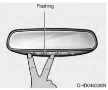
When programming the buttons for the first time, press and hold the left and center buttons (⊉, 1) simultaneously until the indicator light begins to flash after approximately 20 seconds. (This procedure erases the factory-set default codes. Do not perform this step when programming the additional HomeLink buttons.)
