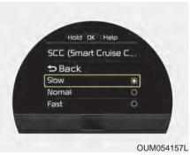
The sensitivity of vehicle speed when following the front vehicle to maintain the set distance can be adjusted. Go to the User Settings Mode (Driving Assist) and select SCC (Smart Cruise Control). You may select one of the three stages you prefer.
