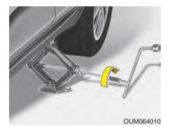
8. Insert the wheel lug nut wrench into the jack and turn it clockwise, raising the vehicle until the tire just clears the ground. This measurement is approximately 30 mm (1 in.).
