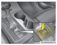
To release the EPB (electric parking brake), press the EPB switch in the following condition:
