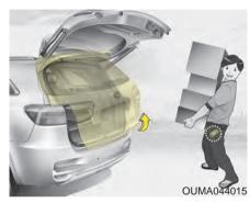
On a vehicle equipped with a smart key, the liftgate (tailgate) can be opened using the Smart Liftgate (Tailgate) system.
