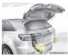
During power opening and closing if the power liftgate (tailgate) is blocked by an object or part of the body, the power liftgate (tailgate) will detect the resistance.
