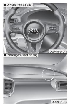
Your vehicle is equipped with an Advanced Supplemental Restraint (Air Bag) System and lap/shoulder belts at both the driver and passenger seating position.
