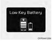
• This warning message illuminates if the battery of the smart key is discharged when the Engine Start/Stop Button changes to the OFF position. Press start button while turn steering (for smart key system)
