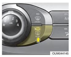
The defroster heats the window to remove frost, fog and thin ice from the rear window, while the engine is running. To activate the rear window defroster, press the rear window defroster button located in the center facia switch panel. The indicator on the rear window defroster button illuminates when the defroster is ON.
