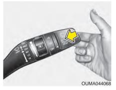
In the OFF position, pull the lever gently toward you to spray washer fluid on the windshield and to run the wipers 1-3 cycles.
