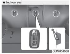
Child restraint hook holders are located on the back of the rear cushions.
