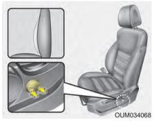
The lumbar support can be adjusted by pressing the lumbar support switch on the side of the seat.
