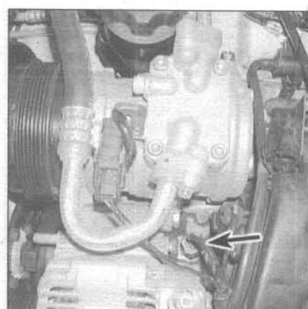
7.2c Engine coolant temperature sensor location - 4.7L V8 models
