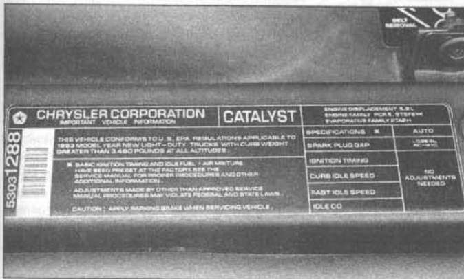
1.6a The Vehicle Emission Control Information (VECI) label, located in the engine compartment, contains information on the emission devices installed on your vehicle
