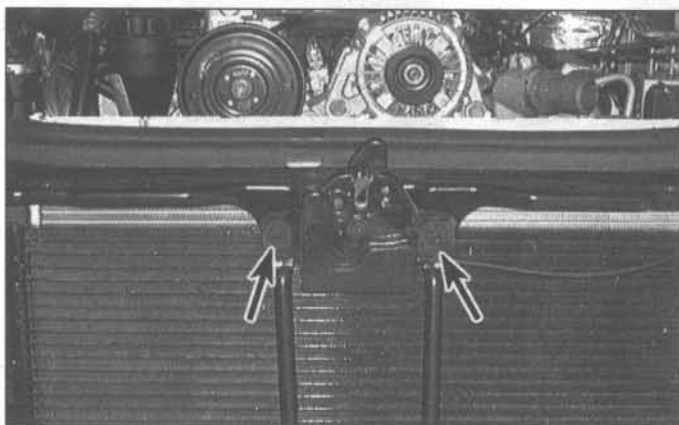
6.10 Radiator support panel mounting bolts - 1999 and later models
