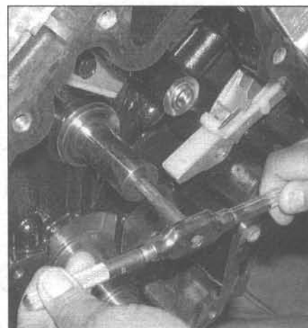
15.5a Tap the end of the idler shaft to accept a slide hammer tool - the factory has predrilled the end of the idler shaft to accept a 12mm x 1.75 tap
