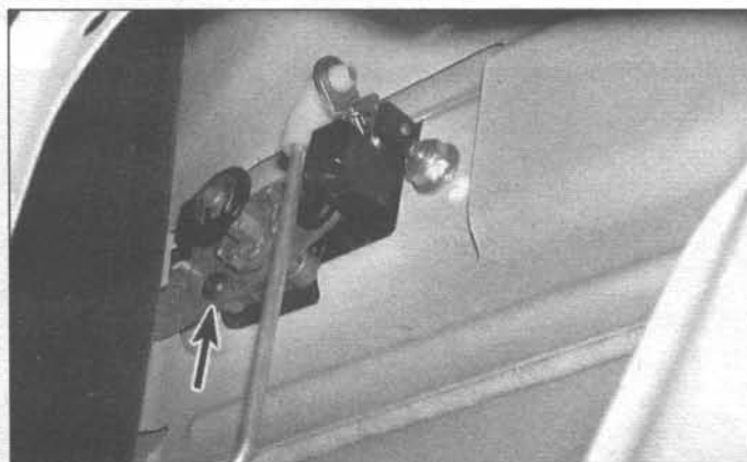
16.9 Remove the Torx screw (arrow) and the retainer plate to separate the lock cylinder from the outside door handle on 1999 and later models
