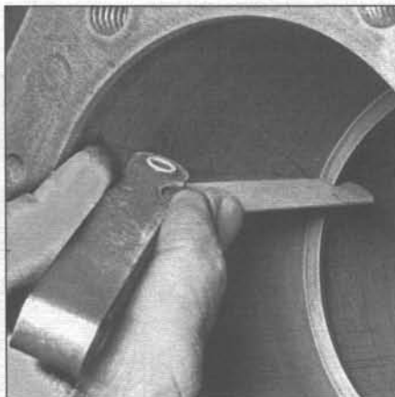
23.4 With the ring square in the cylinder, measure the end gap with feeler gauges
