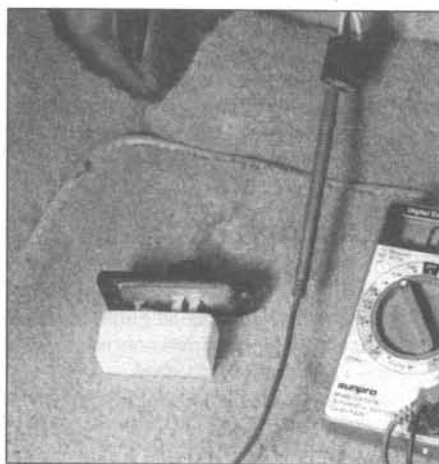
9.7c Check for voltage in the harness to the resistor, at each blower switch speed
