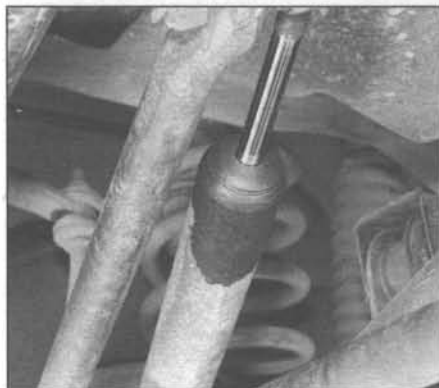
13.4 Inspect the suspension for damage - this steering damper is leaking fluid
