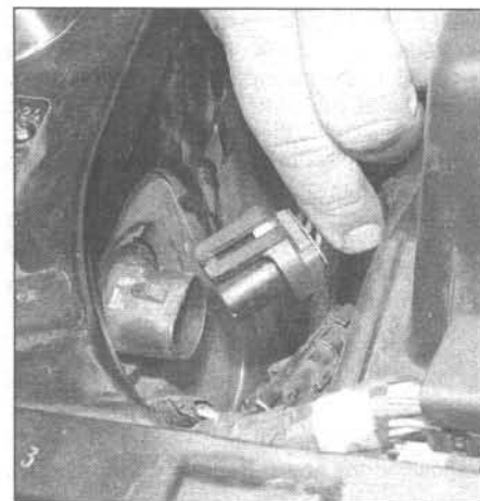
12.3a Disconnect the headlight bulb electrical connector - 1998 and earlier models
