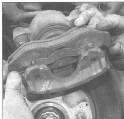
3.6e To remove the outer brake pad from the caliper, push up on the ears at either end of the pad, disengage the pad retaining clips from the caliper and remove the pad
