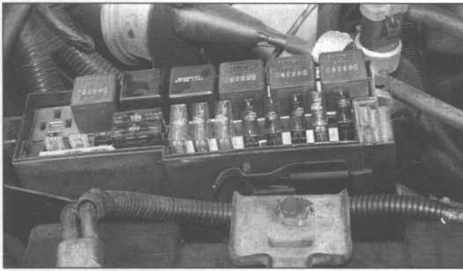
6.2 The power distribution center in the engine compartment contains fuses and relays
