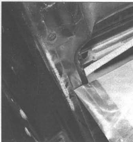
14.6 Peel the water deflector carefully away from the door, taking care not to tear or distort it
