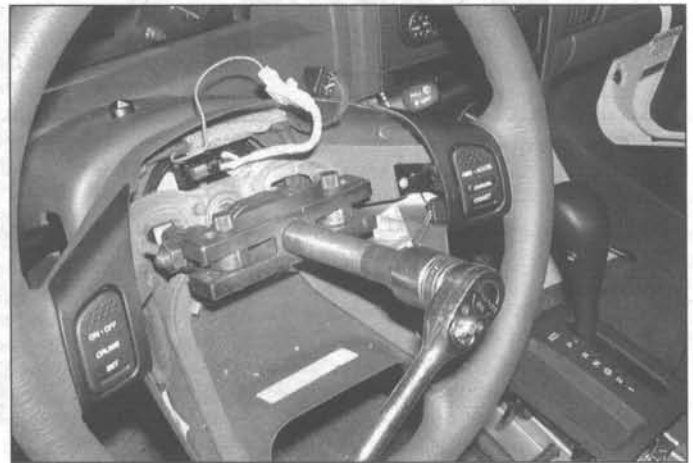
14.4b On 1999 and later models, a jaw type puller will have to be used; make sure the jaws of the puller seat completely in the pockets in the steering wheel hub
