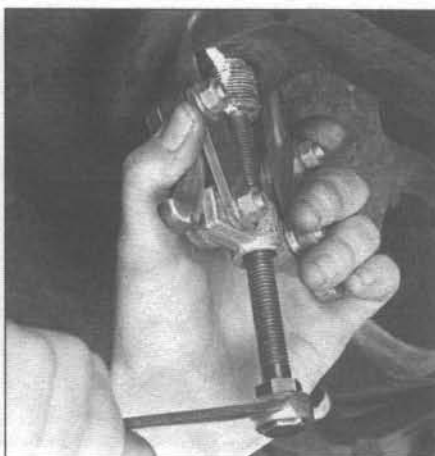
16.5 Use a puller to separate the Pitman arm from the steering gear shaft
