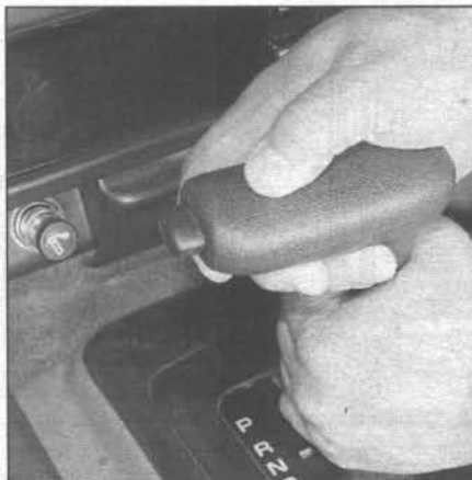
19.2b ... grasp the shift knob securely and pull it straight up sharply to remove it ...
