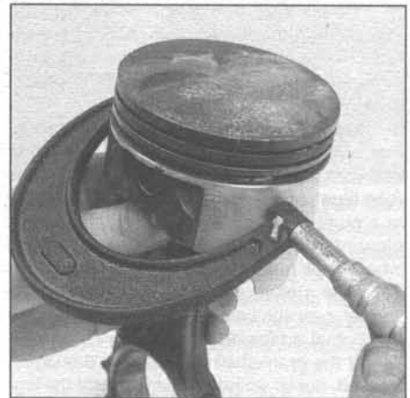
18.11 On engines without moly-coated pistons, measure the piston diameter at a 90-degree angle to the piston pin and in line with it
