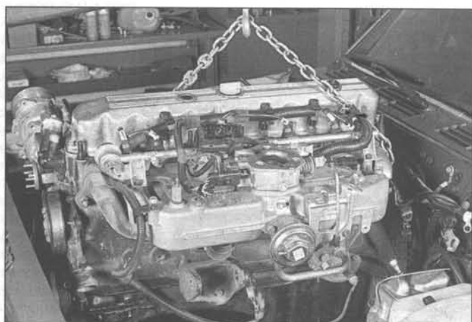
6.24 Pull the engine forward as far as possible to clear the transmission, then lift the engine high enough to clear the body
