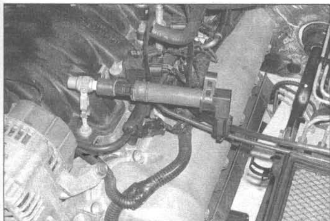
6.20 To use a calibrated ignition tester on a 1999 or 2000 V8 model, remove an ignition coil and connect the tester to the spark plug boot, clip the tester to a convenient ground and crank the engine over - if there's enough power to fire the plug, bright blue sparks will be visible between the electrode tip and the tester body (weak sparks or intermittent sparks are the same as no sparks)
