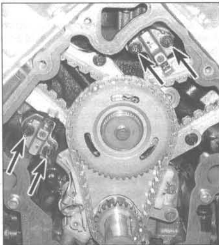
7.15 Secondary timing chain tensioner mounting bolts (arrows)
