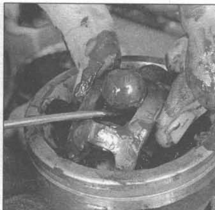
13.6b If necessary, pry the ball bearings out with a screwdriver
