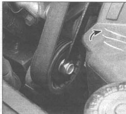
21.8a Release the belt tension by rotating the tensioner clockwise using a wrench on the tensioner bolt
