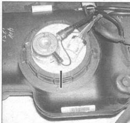
7.4 Before loosening the fuel pump module locknut, apply an alignment mark on the fuel pump module flange and fuel tank
