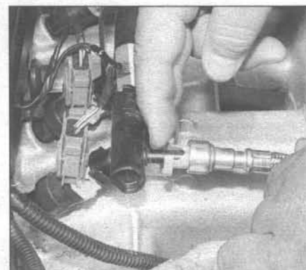
15.8b . . . insert the fuel line disconnect tool into the fitting and disconnect the fuel line from the fuel rail
