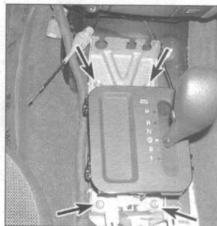
3.17 The shifter assembly is secured by four nuts (arrows) - 1999 and later models
