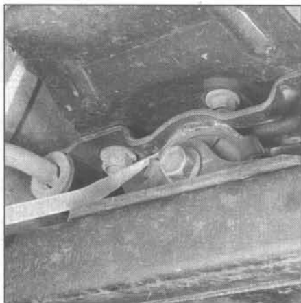
8.2 To check the transmission mount, insert a large screwdriver or prybar between the extension housing and crossmember (2WD models) or between the transfer case and crossmember (4WD models) and pry the transmission up, looking for cracks in the rubber
