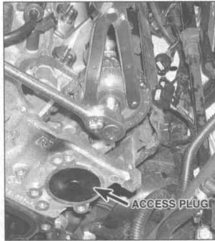
7.16a Removing the left camshaft sprocket bolt while holding the sprocket with a pin spanner wrench - note the chain guide access plug
