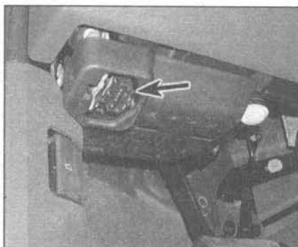
2.36 The diagnostic connector is typically located under the instrument panel
