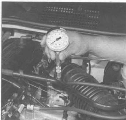
3.6a Connect a fuel pressure gauge to the test port (4.0L six-cylinder engine shown)
