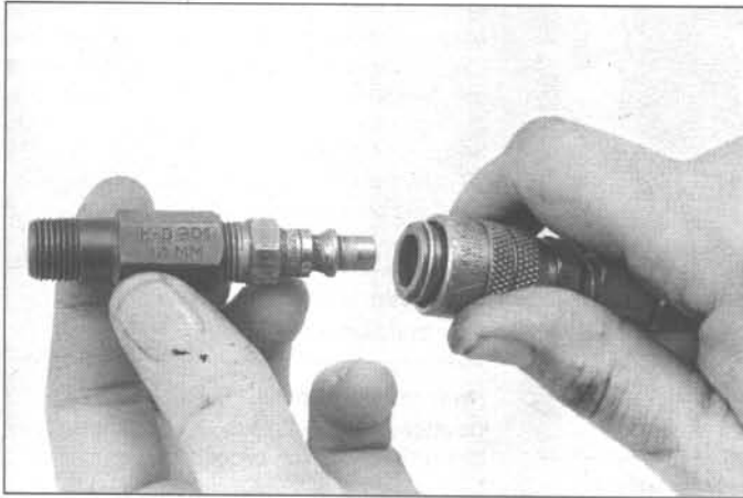
6.4 This is what the air-hose adapter that threads into the spark plug hole looks like - they're commonly available in auto parts stores
