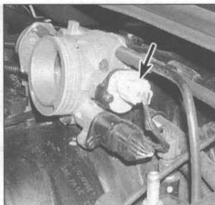
4.2b Throttle position sensor location - 4.7L V8 models
