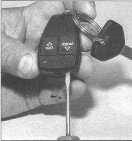
24.15 Use a small screwdriver to separate the transmitter halves
