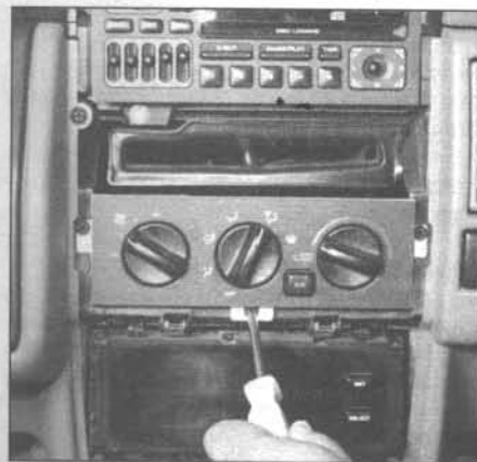
11.3 Remove the screws retaining the air conditioning and heater control panel
