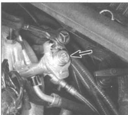
14.3b Fuel pressure regulator location - 1993 and 1994 5.2L/5.9L V8 engines
