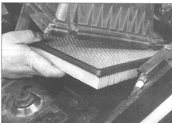
25.4 Lift the cover and slide the element out of the air cleaner housing
