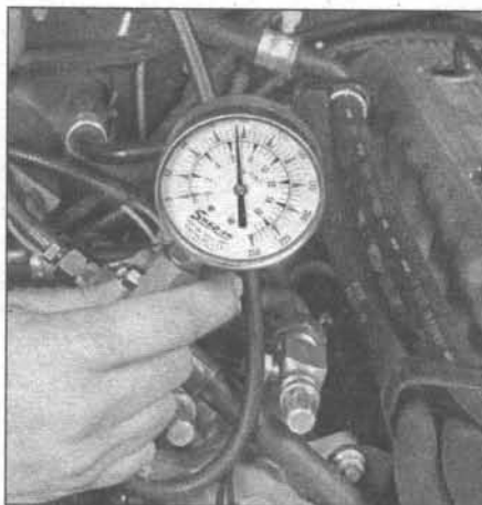
3.6 A compression gauge with a threaded fitting for the spark plug hole is preferred over the type that requires hand pressure to maintain the seal
