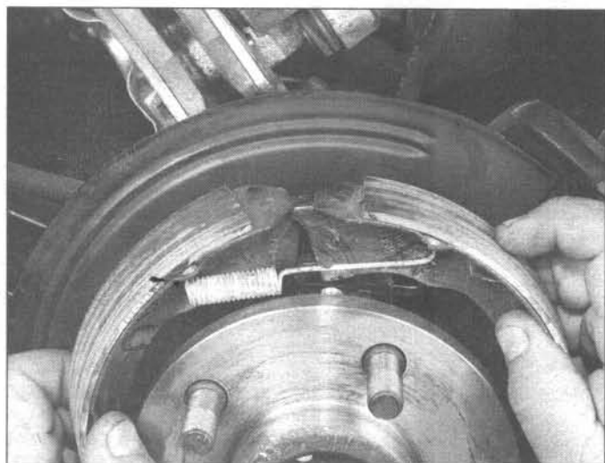
16.4h Holding them together with the upper spring, install the new shoes
