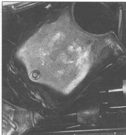
12.13 Remove the oil pan from the rear by sliding it out between the axle and bellhousing
