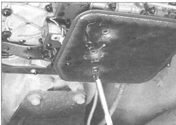
26.9 Remove the filter screws - a special Torx-head wrench is necessary
