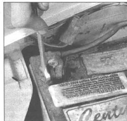
9.6b Removing the cable from a battery post with a wrench - sometimes special battery pliers are required for this procedure if corrosion has caused deterioration of the nut hex (always remove the ground cable first and hook it up last!)
