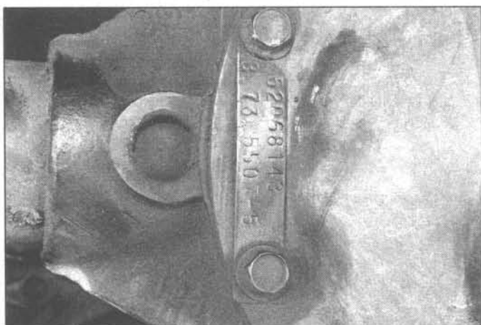
8.11 This tag on the differential housing cover contains information such as the part number and gear ratio
