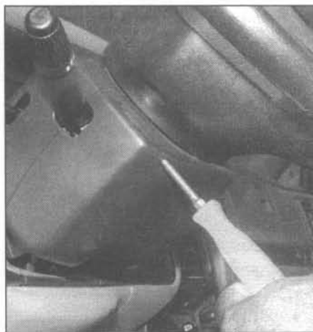
26.3 Remove the Phillips head screws and detach the lower steering column cover
