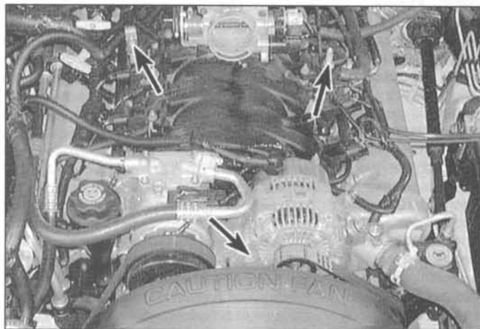
6.20 4.7L V8 engines are equipped with engine lifting studs (arrows) that protrude from the cylinder heads and the front of the water pump
