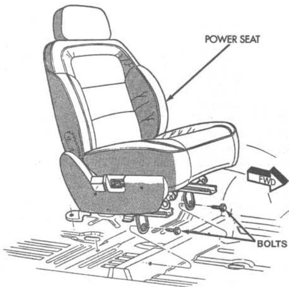
29.2 Front seat installation details
