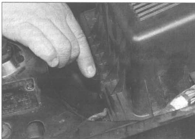
25.3 Release the four air cleaner housing retaining clips
