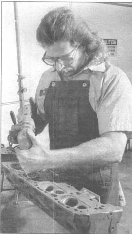
11.3a The valve seats are ground at the machine shop using a machine like this one - the precisely-shaped grinding stone is centered on a mandrel in the new valve guide, making the new seat concentric to the guide
