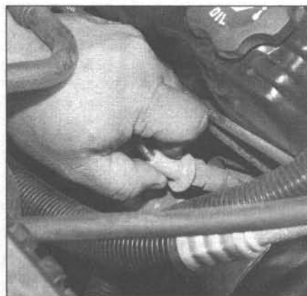
37.6a When removing the spark plug wires, pull only on the boot and twist it back-and-forth
