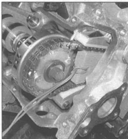
8.7b The wedge is pushed down between the chain strands to secure the secondary chain and the tensioner in place while the camshaft is removed - this wedge is fabricated from a block of wood and a piece of wire
