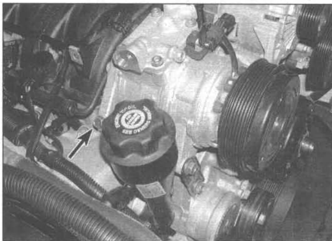
16.6d Right side compressor mounting bolts (arrows) - 4.7L V8 engine
