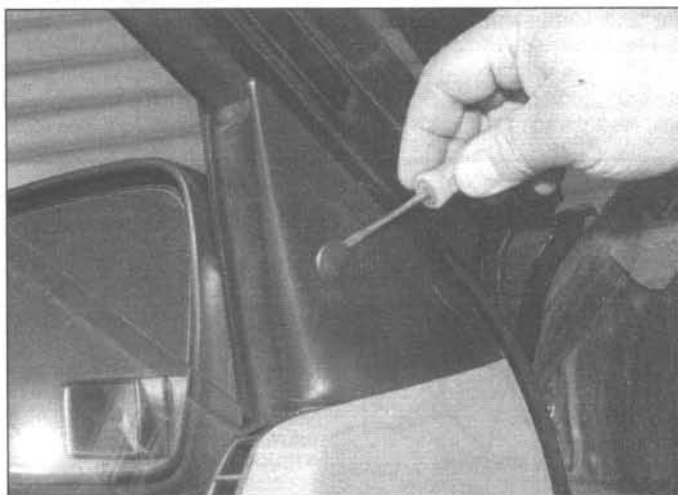
27.7a Use a small screwdriver to pry out the screw cover . . .
