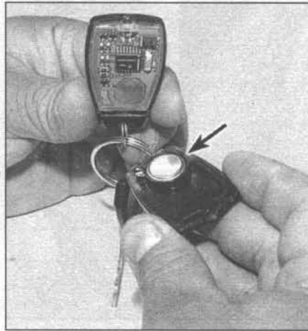
24.16 Replace the lithium batteries (arrow)
