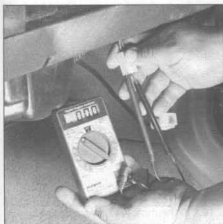
9.4 Disconnect the electrical connector to the blower motor and attach a voltmeter to the harness side of the connector
