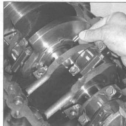
22.8b Insert the thrust bearing into the machined surface between the crankshaft and the upper bearing saddle, then rotate it down into the block until its flush with the parting line of the main bearing saddle - make sure the oil grooves on the thrust bearings face the crankshaft
