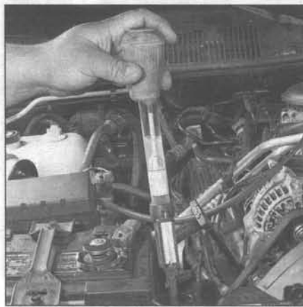
2.6 An inexpensive hydrometer can be used to test the condition of your coolant
