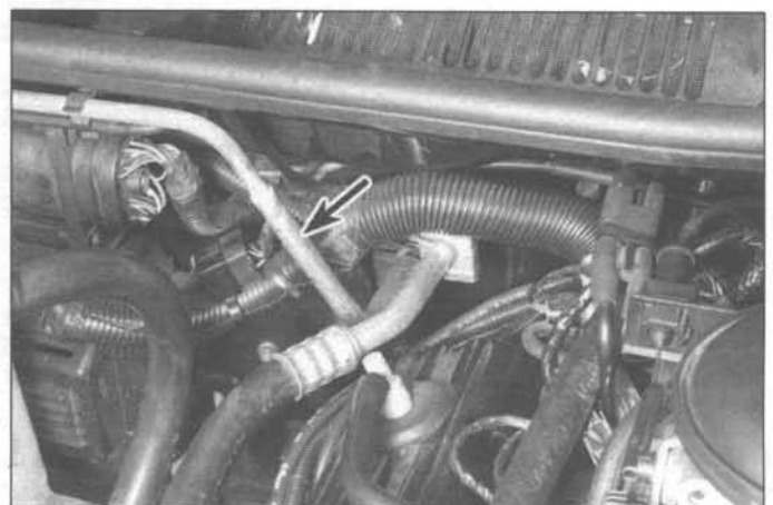
18.3 The fixed orifice tube (arrow) is an integral part of the line to the evaporator (1998 and earlier shown, 1999 and later similar but mounted lower)
