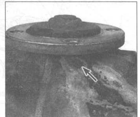
7.3 The water pump weep hole (arrow) will drip coolant when the seal on the pump shaft fails
