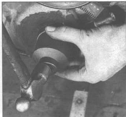
9.10 Gently drive the new seal into place with a hammer and large socket
