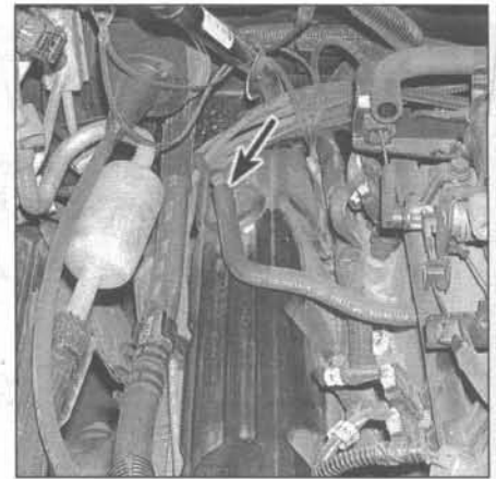
14.3a On 5.2L/5.9L V8 models, the PCV valve is located in the right valve cover
