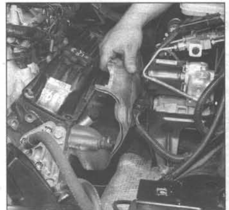
8.3 Remove the exhaust manifold heat shield
