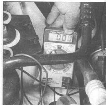
9.4 Disconnect the electrical connector from the camshaft position sensor and check the power and ground circuits on the harness side
