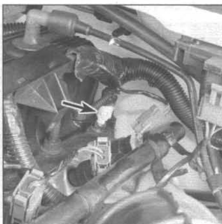
5.1a Coolant temperature sender location (arrow) - six-cylinder engine
