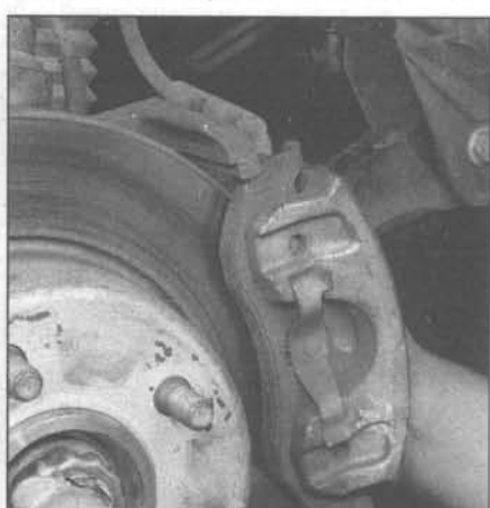
3.6p Install the caliper and pads over the disc, install the caliper bolts and tighten them to the torque listed in this Chapter's Specifications
