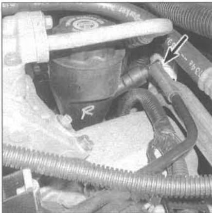
14.3b On 4.7L V8 models, the PCV valve is located in the oil filler tube
