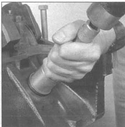
15.11 A large socket on an extension can be used to drive the new core plugs into the block - go slowly and stop when the plug is evenly flush with the block
