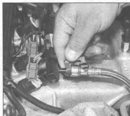
15.8a To disconnect the fuel line from the fuel rail, remove the safety clip from the quick-connect fitting . . .
