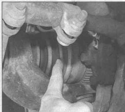
13.6 Push in on the CV joint boots and check for damage and leaking grease
