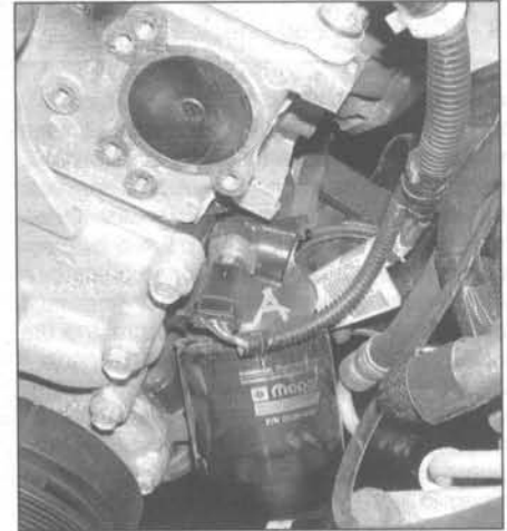
2.4c On 4.7L V8 engines, the oil pressure sending unit is located at the front of the block, just above the oil filter
