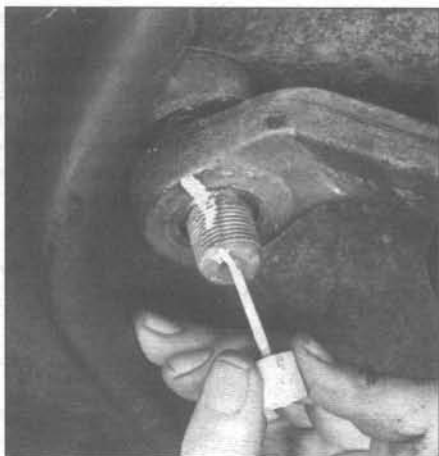
16.4 Before removing the Pitman arm, mark its relationship to the steering gear shaft
