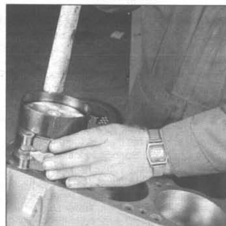
24.11 Drive the piston in gently with the end of a wooden hammer handle - go evenly and stop if you feel an obstruction
