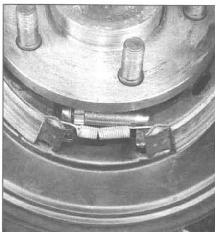
16.4m Make sure the coils of the lower spring are facing down, away from the adjuster, as shown
