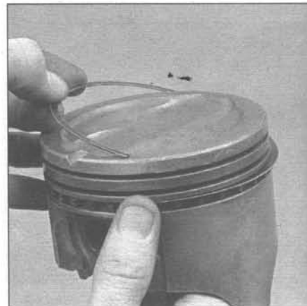
23.9b Slip the oil ring side rails in by hand - do not use a ring expander
