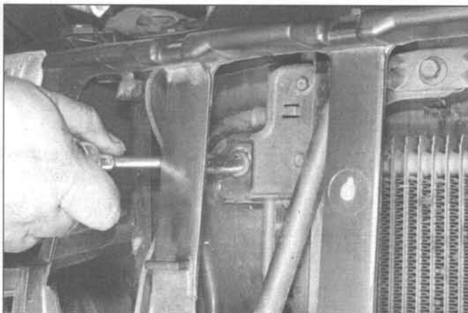
17.6 Mounting bolts for the condenser are reached through the grille opening
