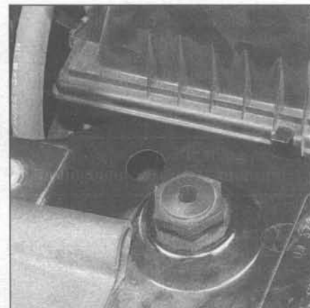
9.11 Thread the rubber bumper in-or-out to make fine adjustments to the hood closed height
