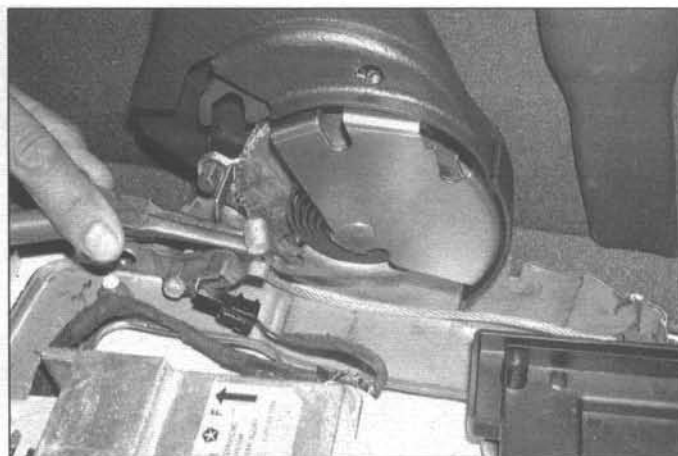
15.24 Unhook the front end of the cable from the tensioner on the parking brake lever
