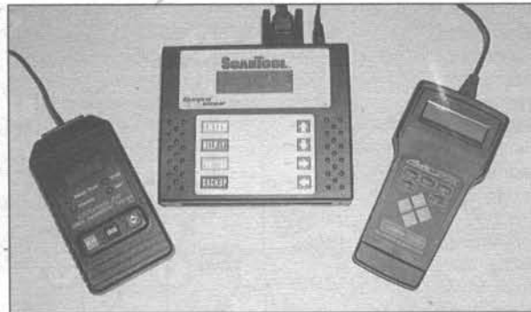
2.2 Scanners like the Actron OBD-II diagnostic tester, the Actron Scantool and the AutoXray XP240 are powerful diagnostic aids - programmed with comprehensive diagnostic information, they can tell you just about anything you want to know about your engine management system
