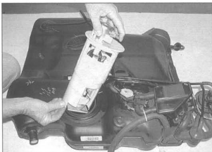
7.6 Carefully remove the fuel pump module from the tank
