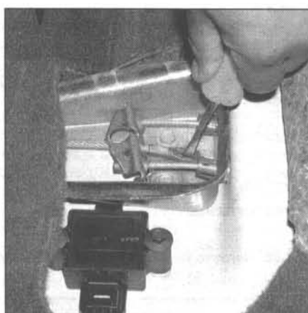
15.22a Using a screwdriver inserted through the cable eyelet, pry the front cable back . . .
