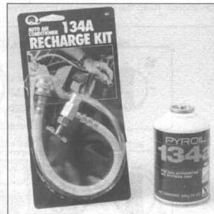
13.12 A basic charging kit for 134a systems is available at most auto parts stores - it must say 134a (not R-12) and so should the 12-ounce can of refrigerant
