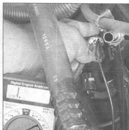
8.2 Disconnect the electrical connector from the crankshaft position sensor and check the power and ground circuits on the harness side
