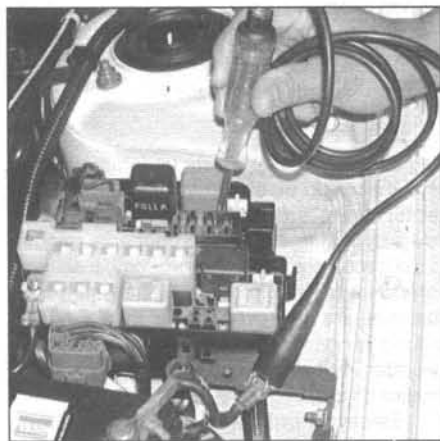
2.6 In use, a basic test light's lead is clipped to a known good ground, then the pointed probe can test connectors, wires or electrical sockets - if the bulb lights, battery voltage is present at the test point
