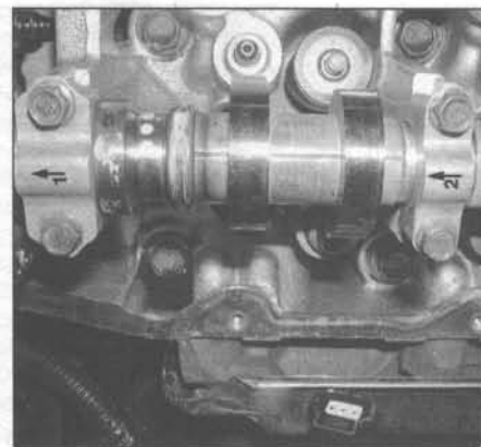
8.9 Verify that the camshaft bearing caps are marked to ensure correct reinstallation - do not mix-up the caps from the left cylinder head with the caps from the right cylinder head
