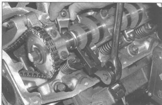
5.5 Using a special type valve spring compressor, depress the valve spring just enough to remove the rocker arm
