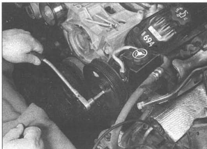
7.7 Access the power steering pump mounting bolts through the holes in the pulley
