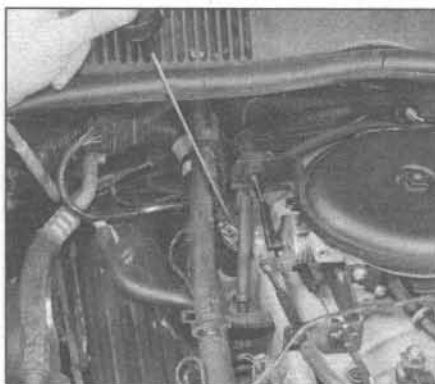
12.7 Use a stethoscope to determine if the injectors are working properly - they should make a steady clicking sound that rises and falls with engine speed changes
