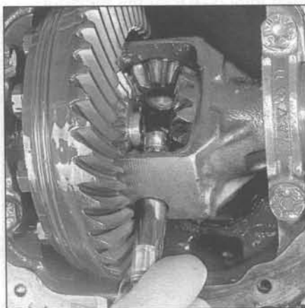
15.4 Carefully remove the pinion mate shaft from the differential case (don't turn the differential case after the shaft has been removed, or the pinion gears may fall out)
