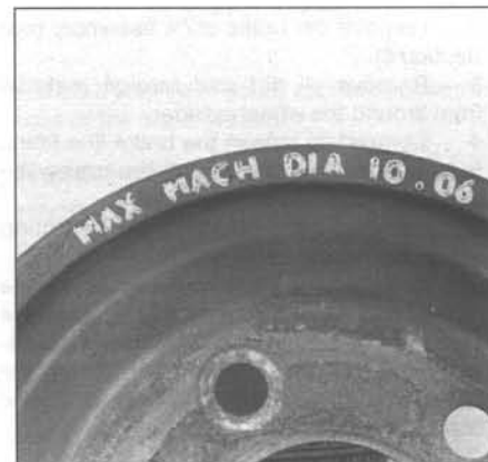
6.5 The maximum allowable drum diameter is cast into the drum (typical)
