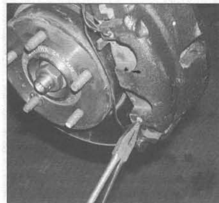
3.7h Install the caliper support spring, making sure it seats properly
