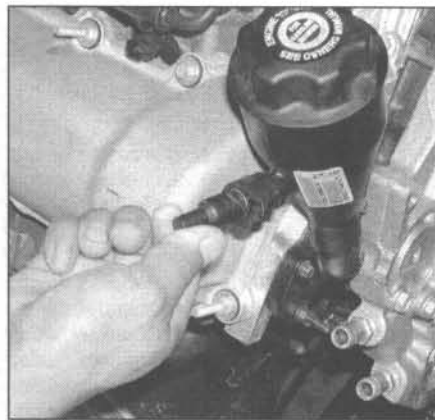
32.2 On 4.7L engines, rotate the PCV valve 90 degrees counterclockwise and pull straight out to remove it
