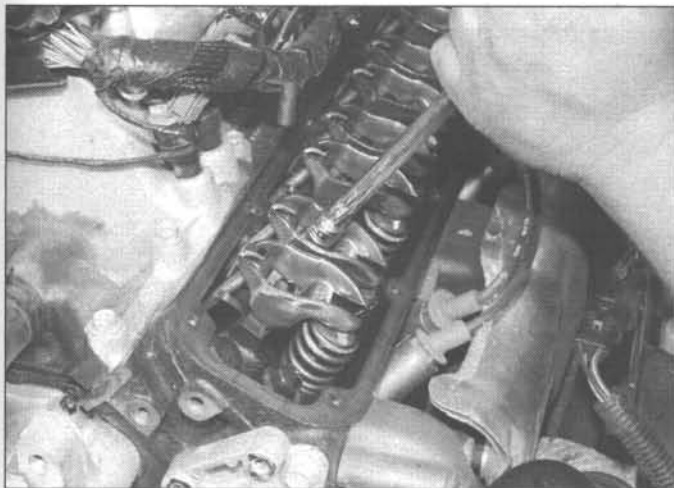
5.2 Remove the rocker-arm bolts, pivots and rocker arms
