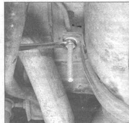
5.11a On 1998 and earlier models, remove the fuel tank strap nuts
