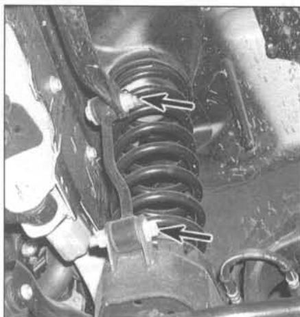
2.2b On 1999 and later models the stabilizer bar link is retained by a nut and bolt at each end
