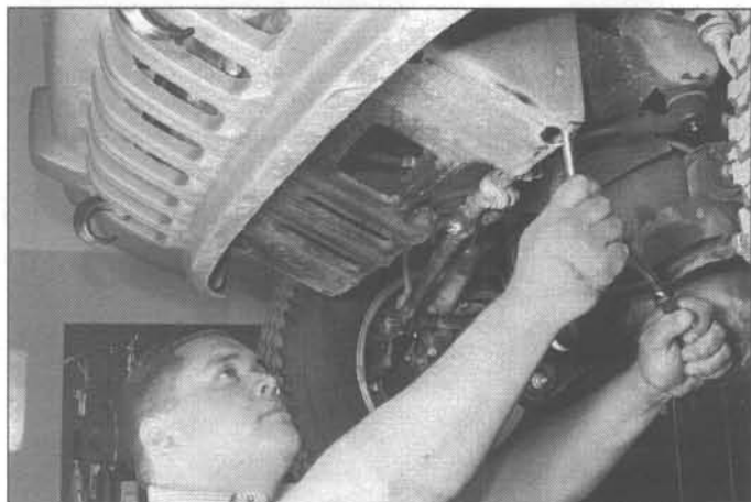
13.2 Remove the front skid-plate - use a long extension through these holes to reach the rear bolts
