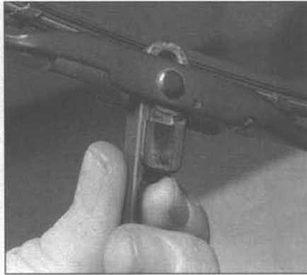
12.7 On later models press the retaining tab in and slide the wiper assembly down and out of the hook in the end of the wiper arm
