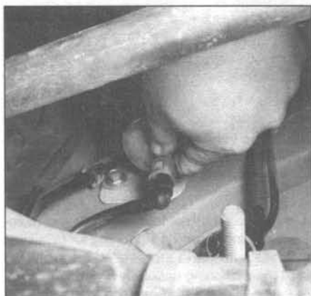
5.9c Depress the tabs on the fuel filter line and separate the line
