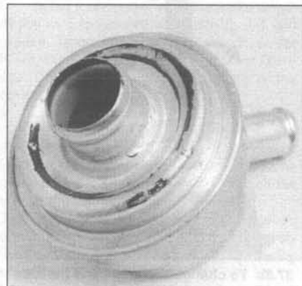
35.3 Lubricate the filter by pouring clean engine oil into the large opening until it drains out the smaller opening
