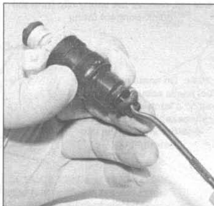
15.10b Carefully remove the O-rings from the injector
