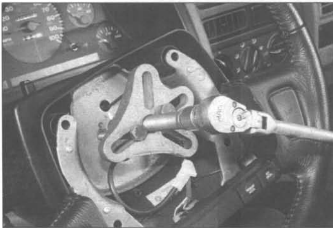
14.4a On 1998 and earlier models, remove the wheel from the shaft with a puller that uses bolts threaded into the hub of the wheel - DO NOT HAMMER ON THE SHAFT!
