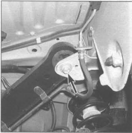
12.9 Upper suspension arm bushing bolt (1999 and later models)
