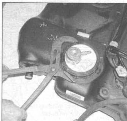
7.5 Loosen the fuel pump module locknut by turning it counterclockwise
