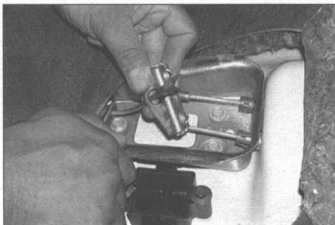
15.23 Detach the front cable from the equalizer by passing it through the slot
