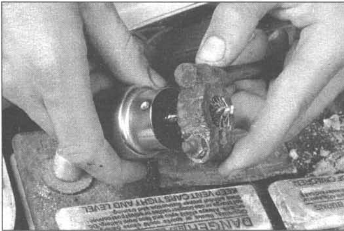
9.7a When cleaning the cable clamps, all corrosion must be removed (the inside of the clamp is tapered to match the taper on the post, so don't remove too much material)
