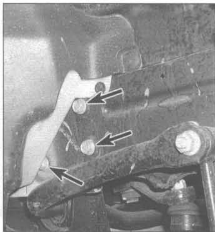
16.6b On 1999 and later models, the steering gear is mounted with four bolts (the fourth bolt, not visible in this photo, is behind the windshield washer fluid reservoir)
