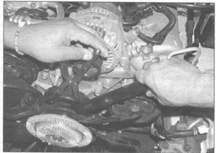
4.14b Use a special spanner wrench to hold the water pump pulley while the mechanical fan drive nut is loosened
