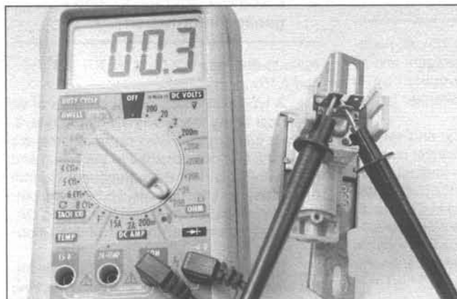
2.9 With a multimeter set to the ohms scale, resistance can be checked across two terminals - when checking for continuity, a low reading indicates continuity, a very high or infinite reading indicates lack of continuity
