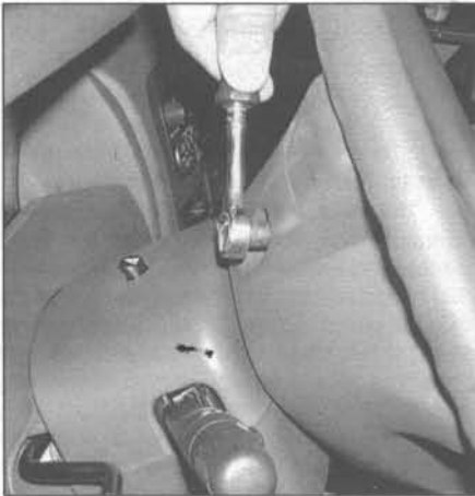
14.2c To remove the airbag module on a 1999 or later model, remove the screw from each side of the steering wheel
