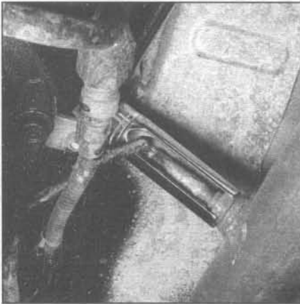
10.14 A special slotted socket, allowing clearance for the wiring harness, may be required for oxygen sensor removal (the tool is available at most auto parts stores)
