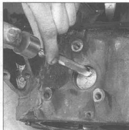
15.1 The core plugs should be removed carefully by tapping in one side, then pulling out the opposite side with locking pliers
