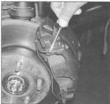
3.7a Wash the brake with brake system cleaner (see illustration 3.6a), then pry off the caliper support spring
