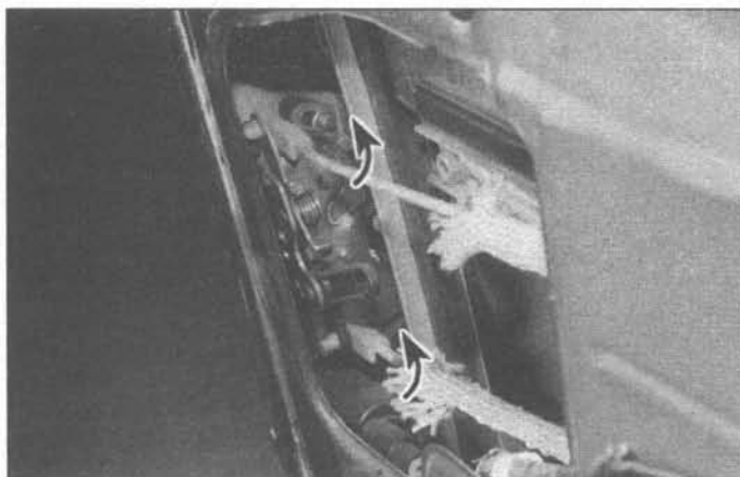
16.2 Rotate the plastic clip up and disconnect the latch rod links
