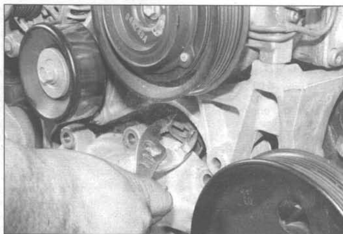
8.7c Reach behind the water pump with pliers to detach the bypass hose - V8 engine
