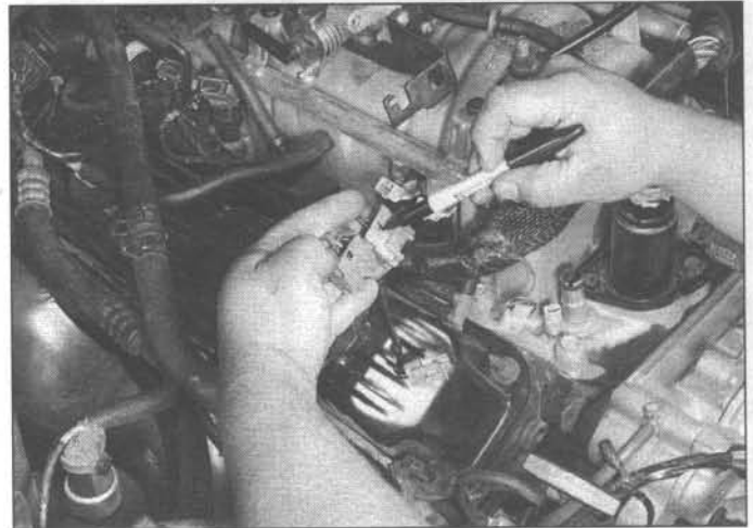
7.9 Disconnect each fuel injector electrical connector and label it clearly so it can be installed on the proper injector during reassembly
