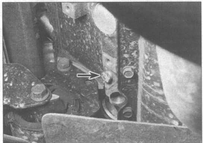
31.4b V8 engine cylinder block drain location - there is one on each side of the block
