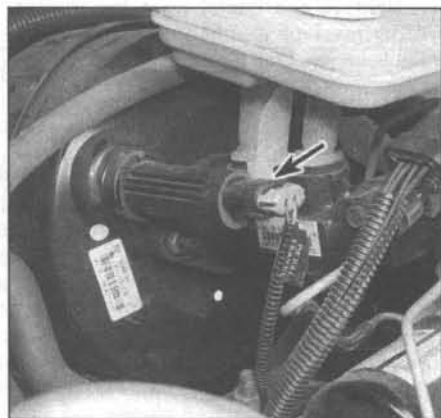
12.5 On 1993 and 1994 models, unplug the electrical connector for the pedal travel sensor
