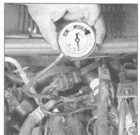
15.9 Check for manifold vacuum at the EGR control solenoid vacuum supply hose with the engine running
