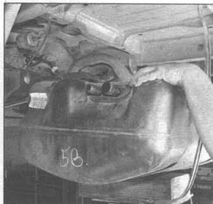
5.13 Slowly lower the fuel tank from the vehicle
