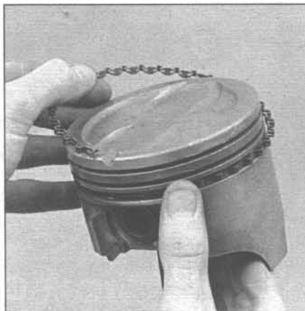
23.9a Installing the spacer/expander in the oil control ring groove
