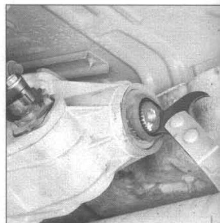
9.5 Using a screwdriver or seal removal tool, carefully pry the oil seal out of the rear of the transmission or transfer case (but don't damage the splines on the transmission output shaft)
