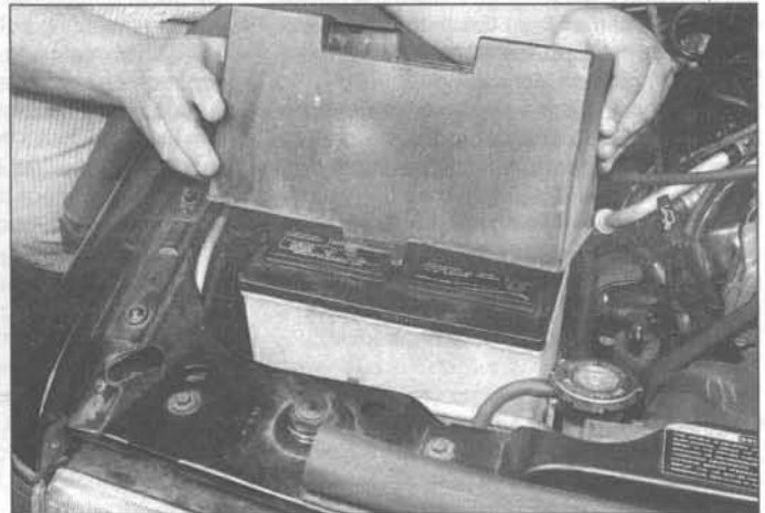
3.5b On 1998 and earlier models, remove the thermo-guard from the battery
