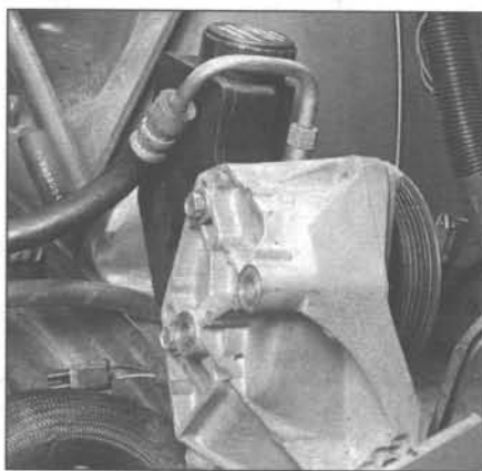
6.11 Set the power steering pump aside with the lines still connected - be sure it's upright so fluid won't spill
