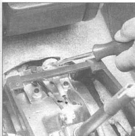
7.5a Pull the cable lock button up to release the cable (1998 or earlier model shown; on 1999 and later models, the shift cable and Park/Lock cable are reversed)
