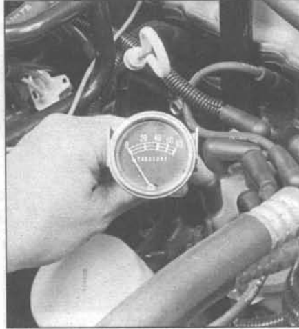
2.4b . . . and connect a gauge to check oil pressure - inline six-cylinder engine shown; the sending unit on 5.2L/5.9L V8 engines is on the top of the block, behind the intake manifold
