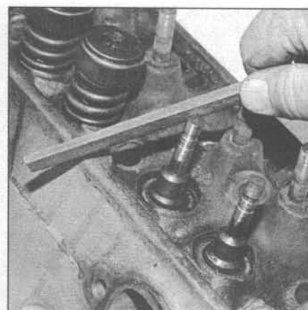
9.4 If the valve won't pull through the guide, deburr the edge of the stem and the area around the top of the keeper groove with a file
