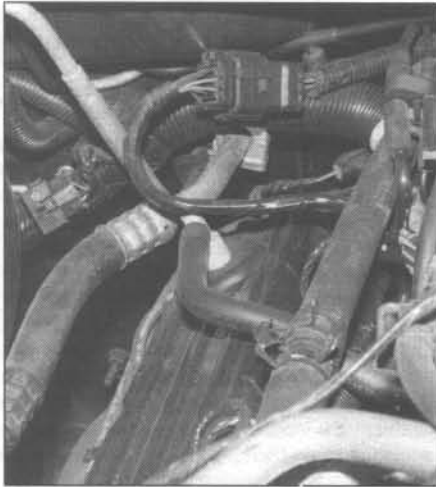
32.1 The PCV valve (arrow) on 5.2L/5.9L engines is pressed into the right side valve cover
