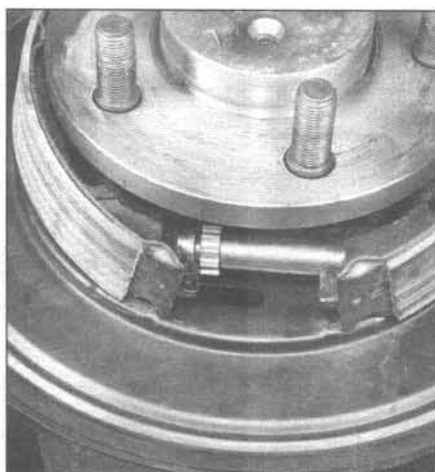
16.4k Make sure the adjuster is engaged with the shoes as shown
