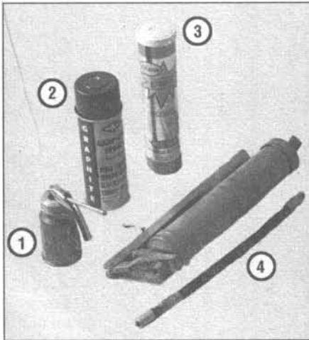
24.1 Materials required for chassis and body lubrication
