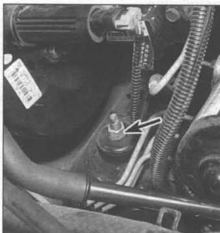
3.2 When removing the shock absorber stem nut (arrow), it may be necessary to hold the stem with an open end wrench or locking pliers to prevent it from turning
