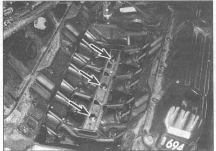
12.14 Remove the three bolts (arrows) and lift out the lifter guide retainer
