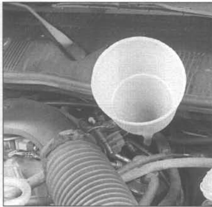
6.6 Use a funnel like this one (available at auto parts stores) inserted into the transmission filler tube to add fluid
