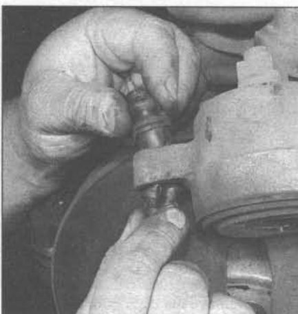
3.6i If either rubber dust boot for the pins and bushings is cracked, torn or dried out, replace it
