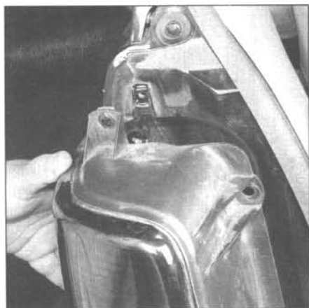
15.6 Open the liftgate, remove the screws and detach the tail light housing by pulling it straight back - 1998 and earlier shown, 1999 and later similar
