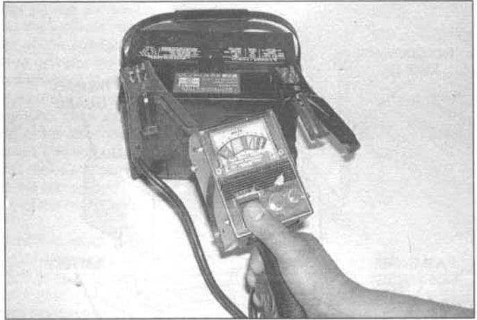
3.3 Connect a battery load tester to the battery and check the battery condition under load following to the tool manufacturers instructions
