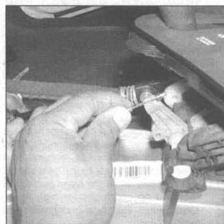
7.13 Pull the end of the cable back and pass it through the slot in the lever
