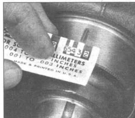
22.15 Compare the width of the crushed Plastigage to the scale on the envelope, taking the measurement at the widest point of the Plastigage
