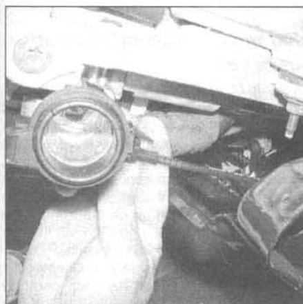
7.11 To detach the Park/Lock cable from the lock cylinder housing on a 1999 or later model, depress the plastic locking tang and pull the cable end out of the housing
