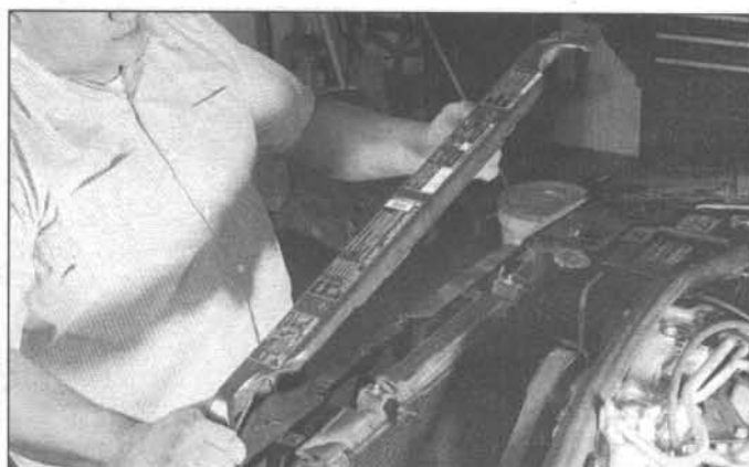
6.9 On early models, remove the radiator support with the hood latch attached and lay it aside
