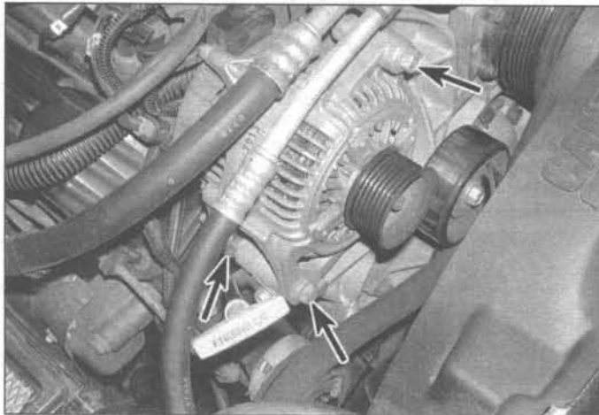
11.4a Remove the alternator mounting nut/bolts (arrows) and remove the alternator from the bracket (5.2L/5.9L V8 model shown)
