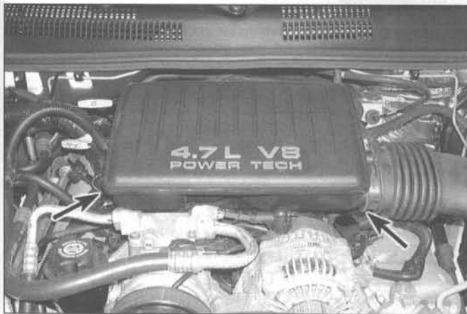
9.4 On 4.7L V8 models, the air intake duct resonator is fastened to the intake manifold with two screws beneath the resonator (arrows)
