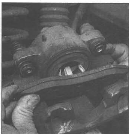
3.6n Install the new inner brake pad by pushing the retaining clips into the piston; make sure the clips are fully engaged (the pad should be seated flat against the piston)
