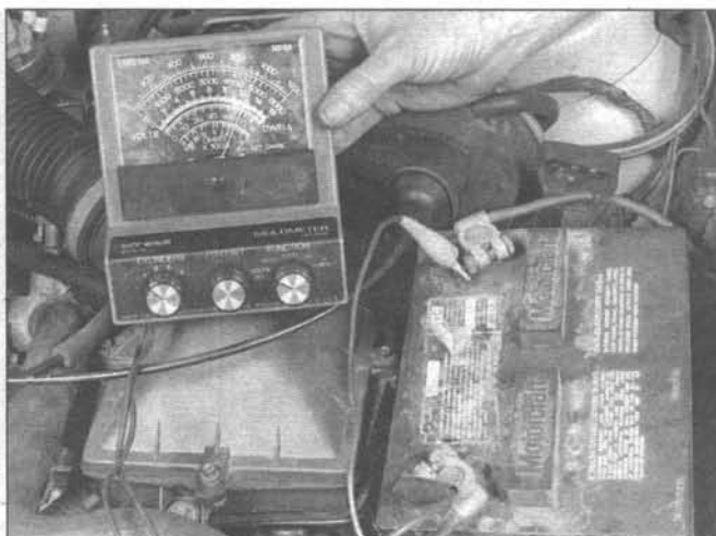
10.3 To measure battery voltage, attach the voltmeter leads to the battery terminals (engine OFF) - to measure charging voltage, start the engine
