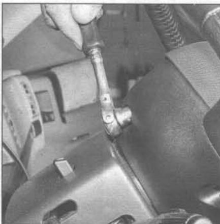
14.2a To remove the air bag module on a 1998 or earlier model, remove the upper nuts...
