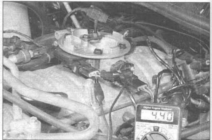
5.4 To check the manifold absolute pressure sensor, backprobe the center wire terminal of the manifold absolute pressure sensor and connect a voltmeter
