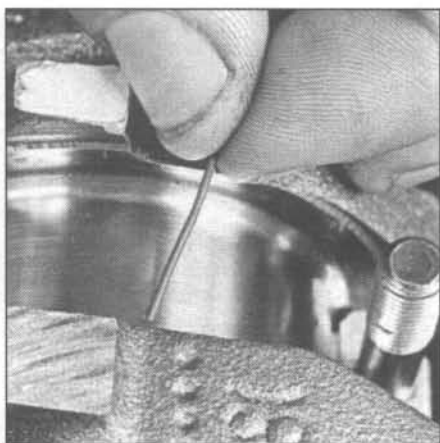
24.13 Lay the Plastigage strips on each rod bearing journal, parallel to the crankshaft centerline
