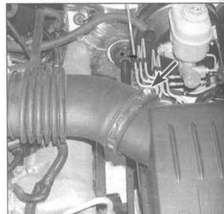
9.1 Loosen the hose clamp (arrow) and detach the intake duct from the air cleaner cover
