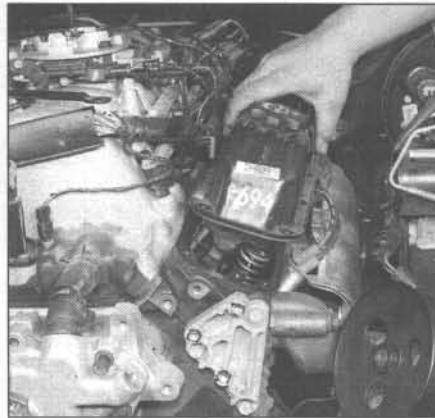
4.8 After striking the valve cover with a rubber mallet to break it loose, pull it straight up
