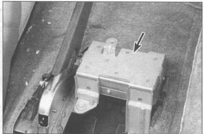
27.6 The airbag control module (arrow) is located under the floor console - be careful not to disconnect the yellow connectors attached to it
