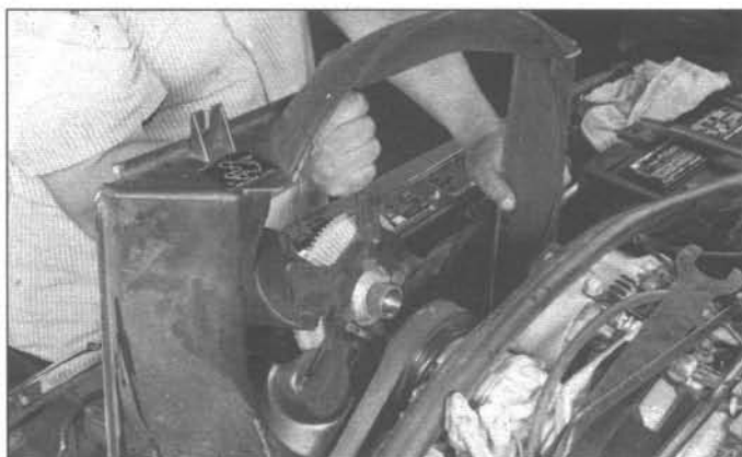
4.17 Lift the fan assembly and fan shroud out together
