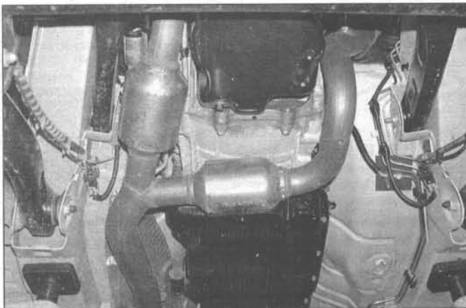
17.3b On 1999 and later California emissions models, two mini-catalytic converters are located in the header pipe near the exhaust manifolds ...
