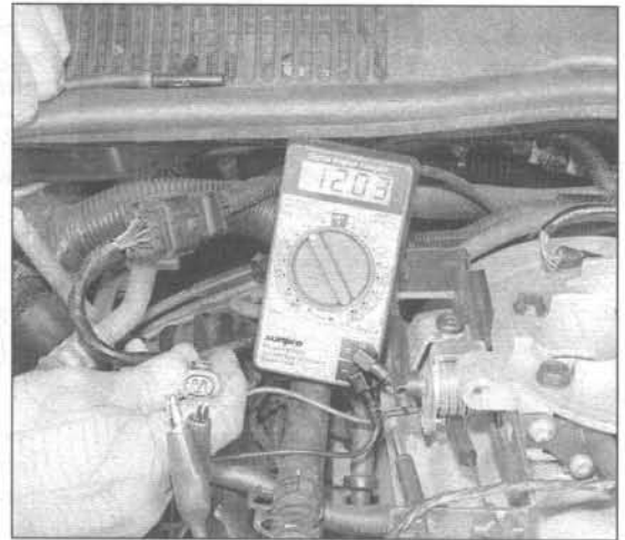
15.4 Check for battery power to the EGR control solenoid with the ignition key ON
