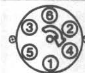
Cylinder location and distributor rotation - distributor used on 1998 and earlier models only
