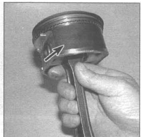
18.8 Later model engines have pistons with a moly coating (arrow) applied to the piston skirt - check the coating for excessive scoring and flaking - never use abrasive materials to clean the coating or damage to the piston will occur
