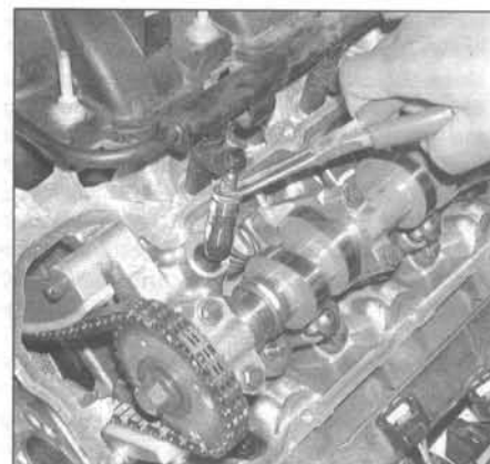
5.7 Pull the lash adjuster up and out of its bore to remove it from the cylinder head
