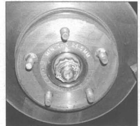
5.5b On later models the minimum thickness is cast into the outside of the disc (typical)
