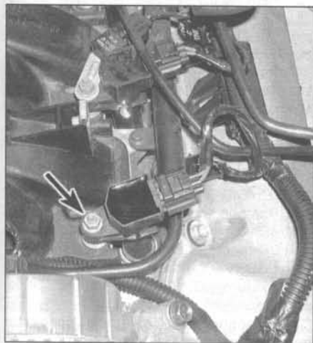
7.23 Ignition coil mounting stud/nut (arrow) - 1999 and 2000 V8 models
