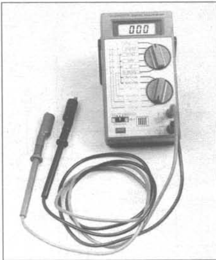
2.1 Digital multimeters can be used for testing all types of circuits; because of their high impedance, they are much more accurate than analog meters for measuring low-voltage computer circuits
