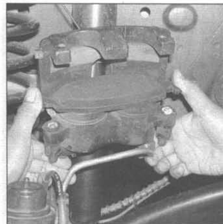
3.7e Apply anti-squeal compound to the backs of the new pads (see illustration 3.6m), then install the new inner pad by pushing the retaining clip(s) straight into the piston(s); make sure the clips are fully engaged - the pad should be seated flat against the piston(s)
