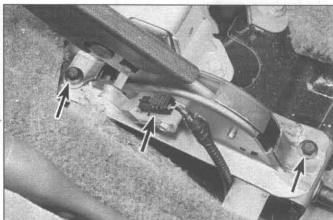
15.5 To remove the parking brake lever, unplug the parking brake switch electrical connector (center arrow) and remove the parking brake lever retaining bolts (left and right arrows) (1998 and earlier models)
