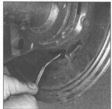
16.3a Remove the plug from the hole in the brake backing plate, insert a brake adjuster tool through the hole...
