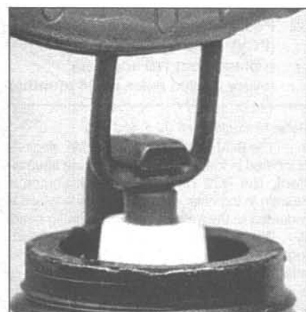
37.5a Spark plug manufacturers recommend using a wire-type gauge when checking the gap - if the wire does not slide between the electrodes with a slight drag, adjustment is required
