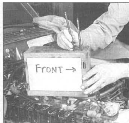
5.4 Store the pushrods in a box like this to ensure reinstallation in the same location
