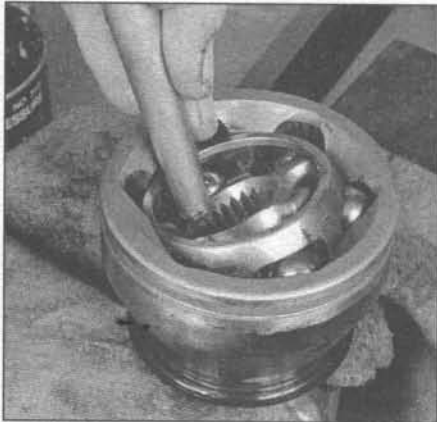
13.6a Tilt the inner race far enough to allow ball removal - a brass punch can be used if the inner race is difficult to move
