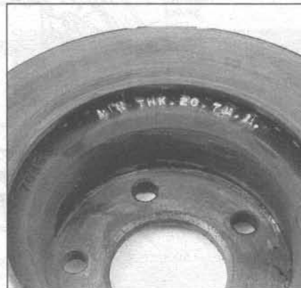
5.5a The minimum thickness is cast into the inside of the disc on early models (typical)
