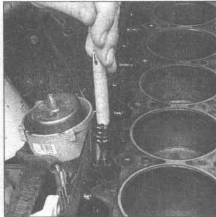
11.16 Remove the lifters with a magnetic pick-up tool (shown here) or a special lifter removal tool
