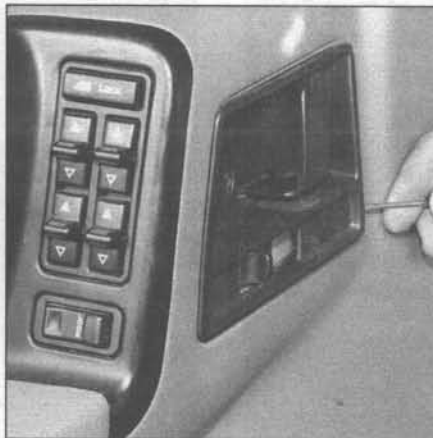
14.2c Remove the screw, then pry off the door handle cover
