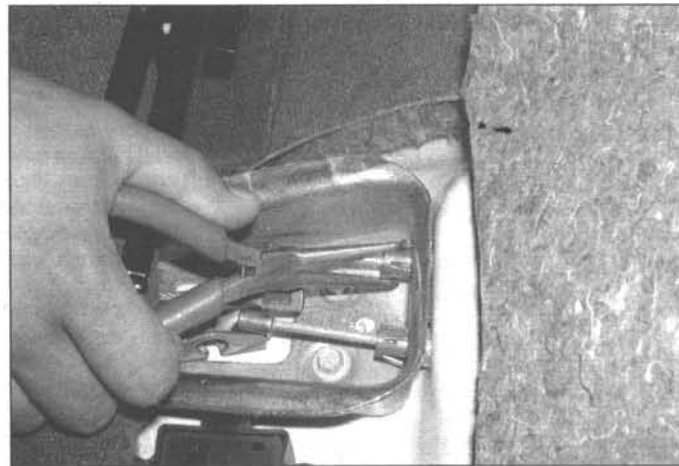
15.31 Depress the tangs on the retainer and pass the cable through the equalizer bracket
