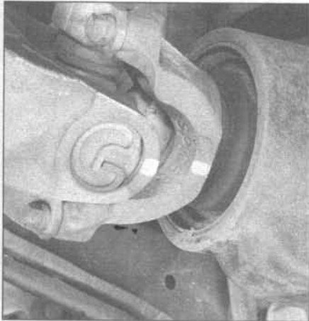
9.12a Before disconnecting the U-joint from the front axle differential pinion yoke on 1993 and 1994 models, mark the relationship of the U-joint joint to the yoke (shown); before disconnecting the CV joint from the front axle differential pinion yoke on 1995 and later models, mark the relationship of the CV joint to the yoke (not shown)
