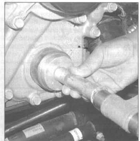
13.4 Use a seal driver or large-diameter socket to drive the new seal into the cover
