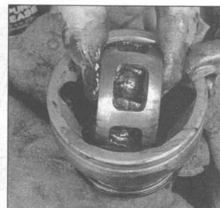
13.7 Tilt the inner race and cage 90-degrees, then align the windows in the cage with the lands and rotate the inner race up and out of the outer race
