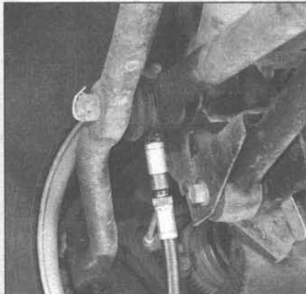
24.6b Pump the grease into the fitting until the rubber seal is firm to the touch
