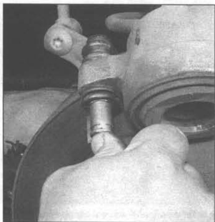
3.6k Install the bushings
