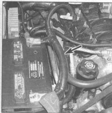
4.4 The battery cables are wrapped in a protective sheathing (arrow) - if necessary, cut the electrical tape and remove the sheathing
