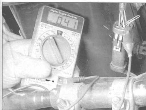
10.7a Backprobe the oxygen sensor electrical connector signal wire and monitor the sensor output voltage
