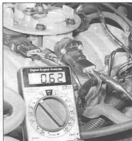
4.4 To check the throttle position sensor, backprobe the center wire terminal of the throttle position sensor and connect a voltmeter
