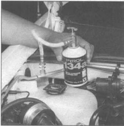
13.15a Add refrigerant to the system at the low-pressure port (1998 and earlier shown)
