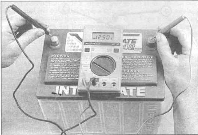
3.2 To test the open circuit voltage of the battery, connect a voltmeter to the battery - a fully charged battery should measure at least 12.4 volts (depending on outside air temperature)
