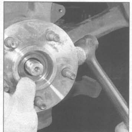
12.4c Carefully tap the hub assembly out of the steering knuckle
