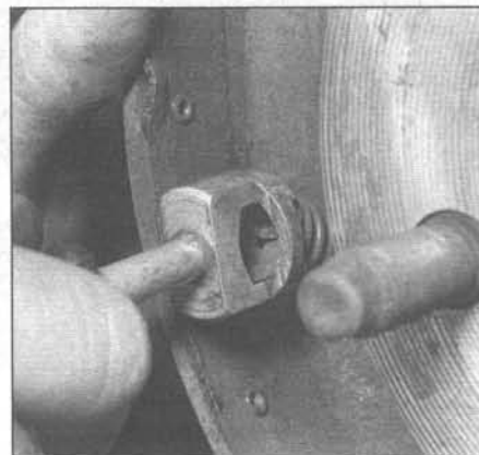
6.4h Remove the primary shoe hold-down spring and pin ...
