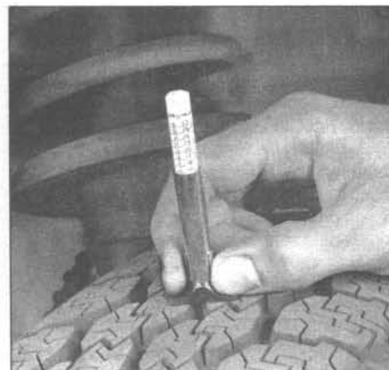
5.2 Use a tire tread depth indicator to monitor tire wear - they are available at auto parts stores and service stations and cost very little
