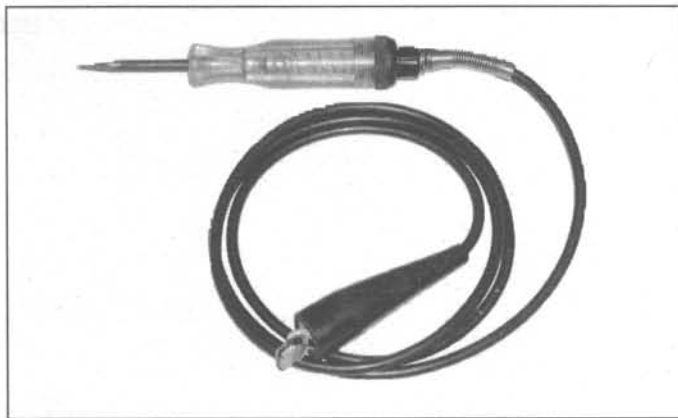
2.5b A simple test light is very handy, especially when testing for voltage
