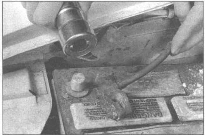
9.7b Regardless of the type of tool used on the battery posts, a clean, shiny surface should be the result
