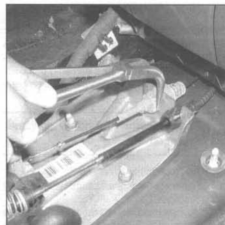
7.14 Squeeze the tangs on the sides of the cable adjuster, then detach the cable from the shifter base
