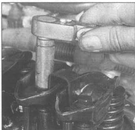
5.2 Alternating between the intake and exhaust rocker arms, loosening each bolt 1/4-turn at a time
