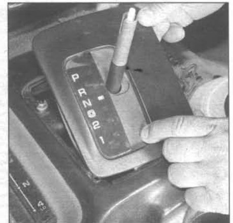
19.2c ... then detach the shift plate
