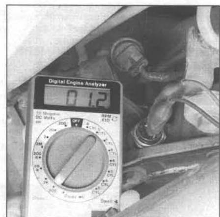
6.6 Shift the transmission into Reverse and check continuity at the switch outer terminals; there should be continuity only when the transmission is in Reverse, but there should be no continuity between the outer terminals and the transmission case
