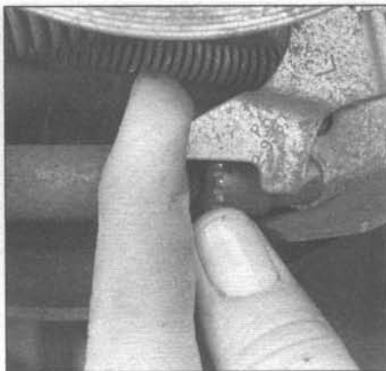
6.4c Pull out on the adjuster lever and turn the star wheel to retract the brake shoes
