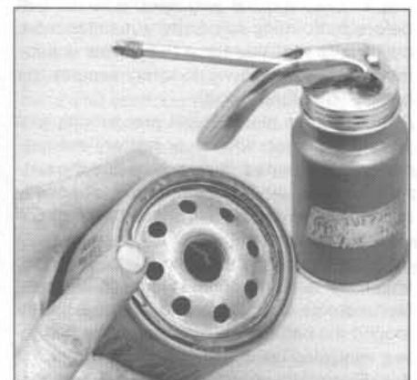
8.18 Lubricate the oil filter gasket with clean engine oil before installing the filter on the engine
