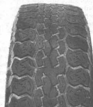
FEATHERING DUE TO MISALIGNMENT
