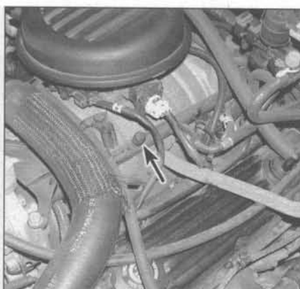
3.6b Fuel pressure test port location - 5.2L/5.9L V8 engines
