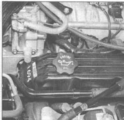
4.6 Oil is added to the engine after removing the oil filler cap from the valve cover (or the oil filler tube on 4.7L engines) - always make sure the area around the opening is clean before removing the cap to prevent dirt from contaminating the engine (5.2L/5.9L engine shown)
