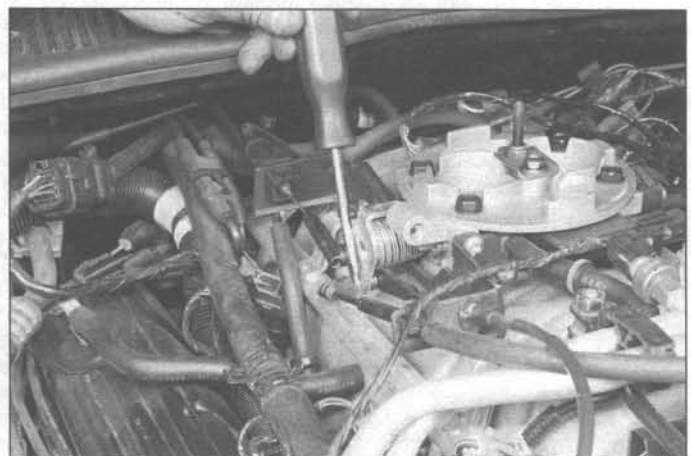
10.2 Rotate the throttle lever and detach the cable from the stud
