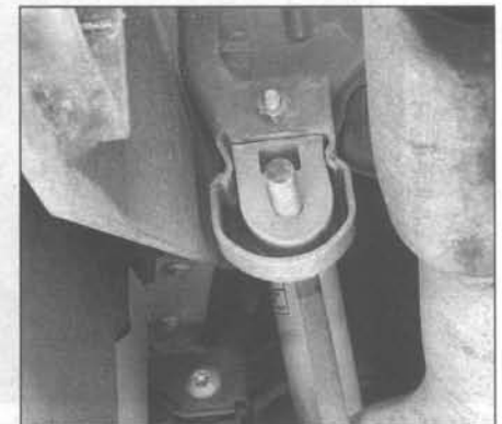
14.4 Inspect the rubber exhaust system mounts for damage
