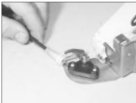
14.33 Slide the outer cable from the lock bracket
