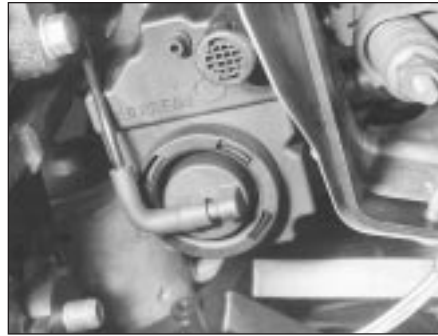
7.13 Disconnect vacuum hose from base of pulse-air filter housing . . .
