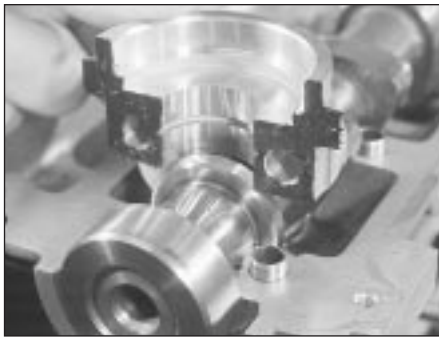
13.19 Apply sealant to mating surface of camshaft right-hand bearing caps
