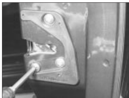
14.4A Unscrew the lock mounting bolts . . .
