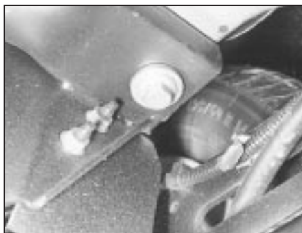
26.7B Rear suspension crossmember front mounting bolt
