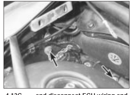
4.13C . . . and disconnect ECU wiring and earth lead (arrowed) to release engine wiring loom from vehicle body
