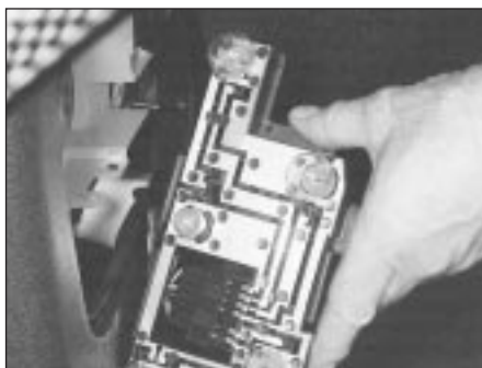
5.27C Removing the rear light cluster (Saloon)
