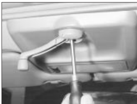
31.3 Removing the sunroof handle securing screw
