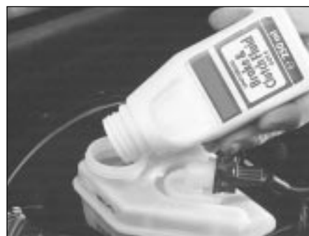
3.22 Topping-up the brake fluid reservoir
