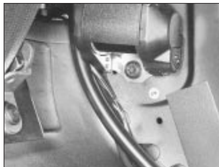
28.7B Rear seat belt reel mounting bolt
