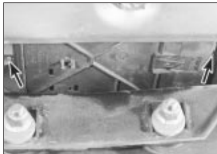
5.15 . . . lower crossmember by 3 inches, and unscrew charcoal canister assembly rear retaining bolts (arrowed) . . .
