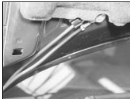
8.5 Earth lead and washer hoses on the underside of the bonnet
