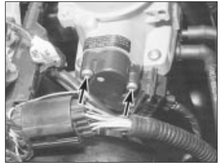
4.53 Throttle potentiometer is secured by two screws (arrowed)
