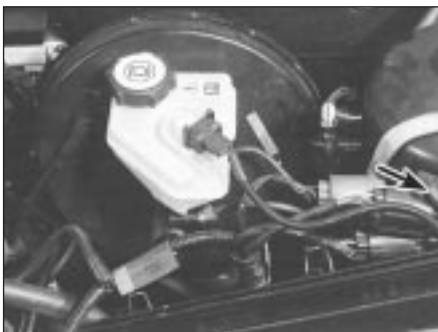
4.13A Unplug three large electrical connectors (arrowed) . . .
