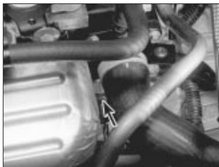
6.9 Location (arrowed) of coolant temperature gauge sender
