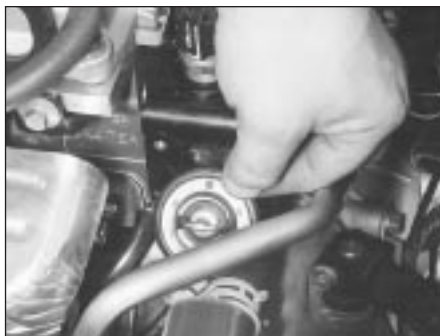
4.14 Ensure thermostat is refitted as shown
