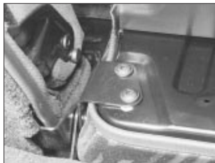
27.10 Rear seat backrest mounting bolts
