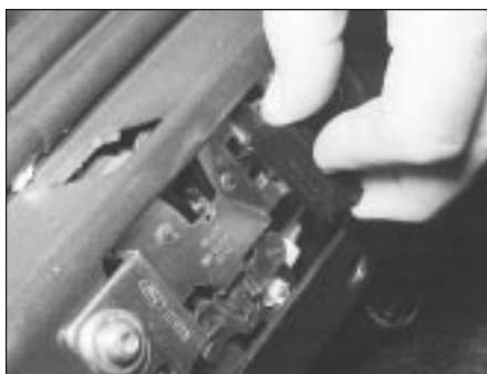
22.14 Removing the door-ajar sensor from the lock
