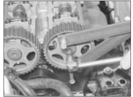
13.3 Using forked holding tool while camshaft toothed pulley bolt is slackened
