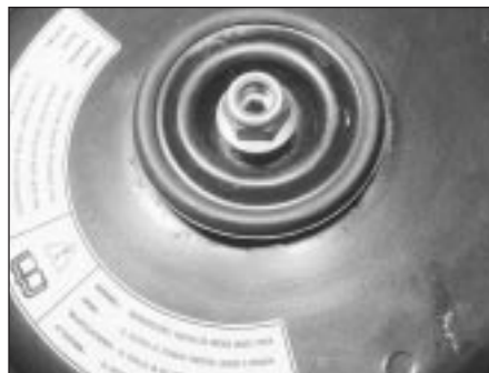
4.10 Front suspension strut upper mounting nut
