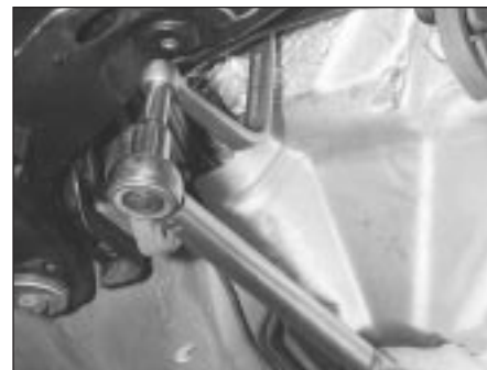
30.9 Tightening the steering gear mounting bolts using the U-shaped spanner (arrowed)
