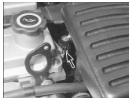
6.15 Location (arrowed) of coolant temperature sensor
