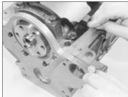
20.16 Check the oil seal carrier is correctly positioned
