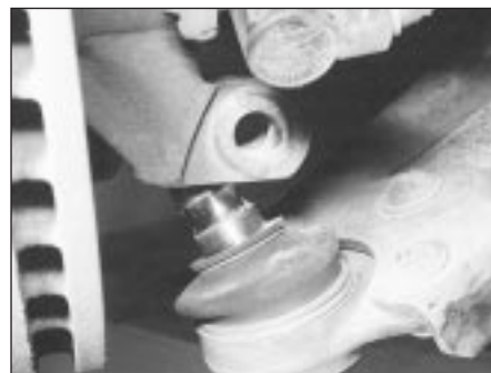
7.7B . . . and disconnect the balljoint from the knuckle
