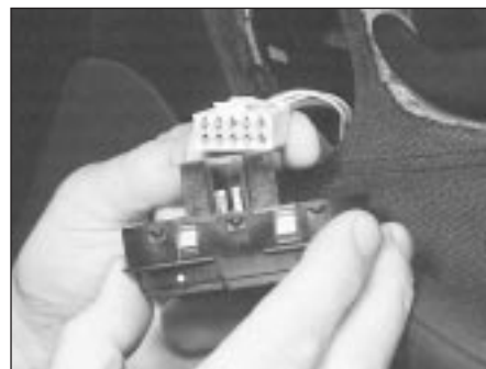
11.3B . . . and disconnect the multi-plug
