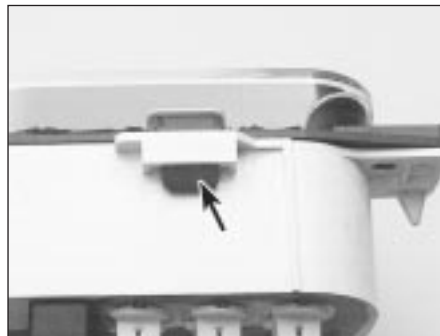
11.2 Bezel retaining lug on the instrument panel
