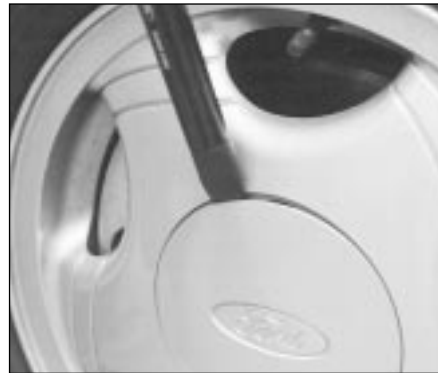
Use flat end of wheelbrace to remove trim covering roadwheel nuts
