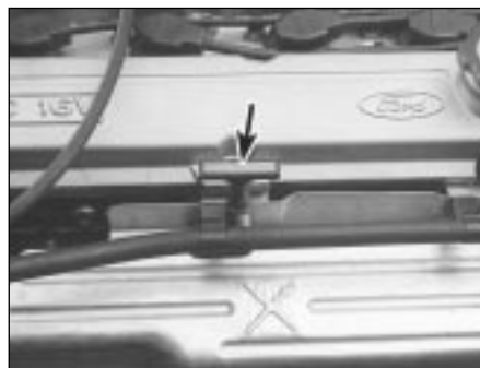
3.2 The engine oil dipstick (arrowed) is located at the front of the engine - note yellow/black plastic grip
