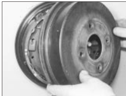
5.2B Removing a rear brake drum
