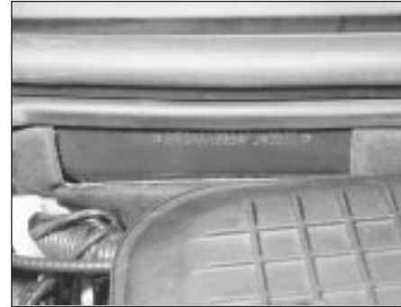
Vehicle identification number on engine compartment bulkhead
