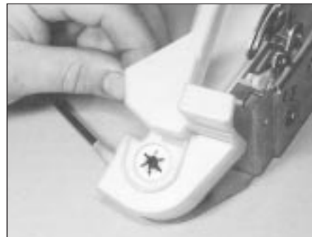
14.32 Removing the plastic shield from the locating post
