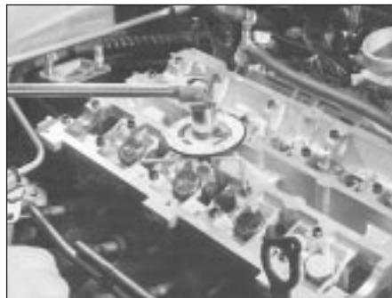
14.32B . . . and to third stage using angle gauge
