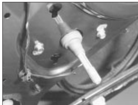
13.2D Manual winder mounting bolts (rear door)
