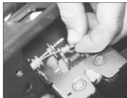
22.16 Disconnecting the cables from the lock
