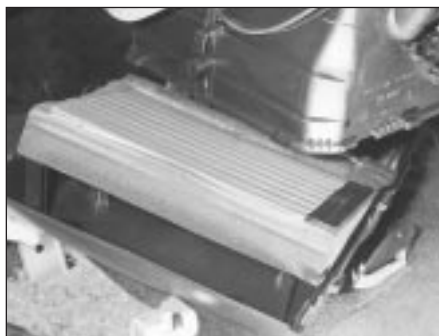
9.13 . . . heater unit's bottom cover, complete with matrix
