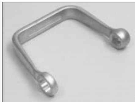
30.6 U-shaped Ford spanner for unscrewing the steering gear mounting bolts
