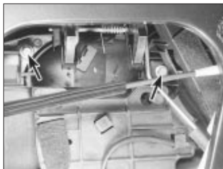
14.3A Remove the two bolts (arrowed) . . .
