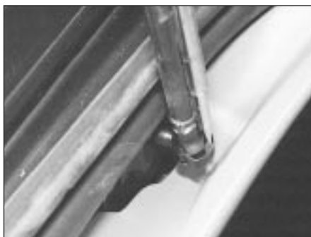
21.3 Prising the spring clip from the lower end of the strut
