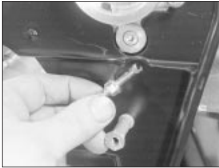
10.19A Fitting tensioner spring retaining pin
