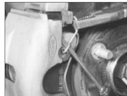
2.3A Prise the retaining clip from the caliper. Hold it with a pair of pliers, to avoid personal injury. On models fitted with pad wear sensors, it will be necessary to disconnect the wiring
