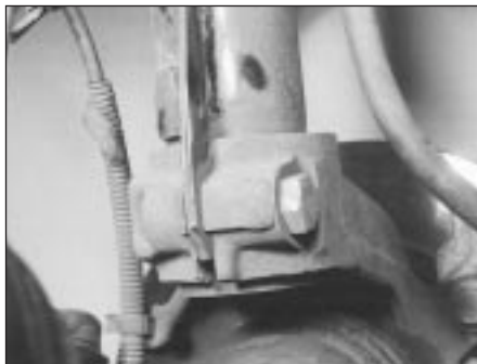
4.12A Steering knuckle-to-strut pinch-bolt
