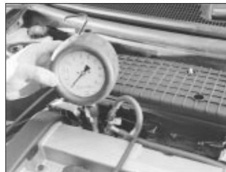
8.4 A fuel pressure gauge, equipped with an adaptor to suit the Schrader-type valve on the fuel rail pressure test/release fitting, is needed to check fuel pressure
