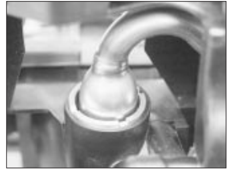
6.10 Check end fitting of EGR pipe into inlet manifold whenever manifold is removed, but do not disturb
