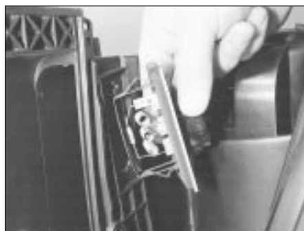
9.5 Heater blower motor control resistor can be prised out of heater unit
