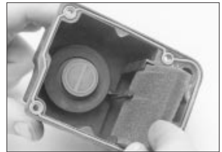
7.17B . . . and withdraw foam filter for cleaning, if required - note valve in base of housing
