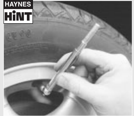
4.2B A tyre tread depth indicator should be used to monitor tyre wear - they are available at accessory shops and service stations, and cost very little
