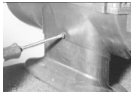
9.11 Remove screw to allow air duct to be retracted into air distributor at base of heater unit . . .
