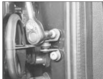
15.2A Front door check strap mounting screw removal
