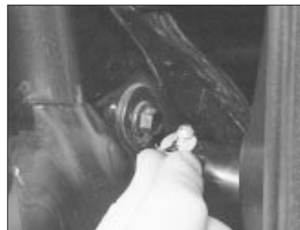
15.4 Extract the small circlips . . .
