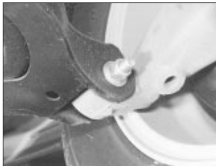
21.5 Rear lower arm-to-knuckle mounting bolt
