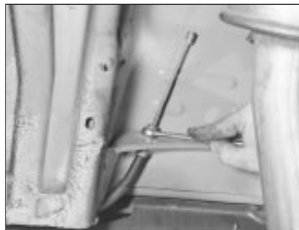
27.10A Release the lugs using a ring spanner . . .
