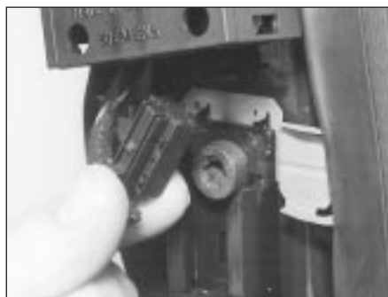
20.3A Disconnecting a movement sensor multi-plug
