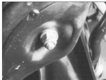
7.3 One of the nuts and bolts securing the lower arm to the subframe
