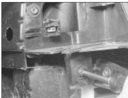
7.8A Unscrew the outer mounting screws . . .
