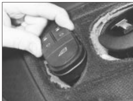
11.3A Remove the window operating switch . . .
