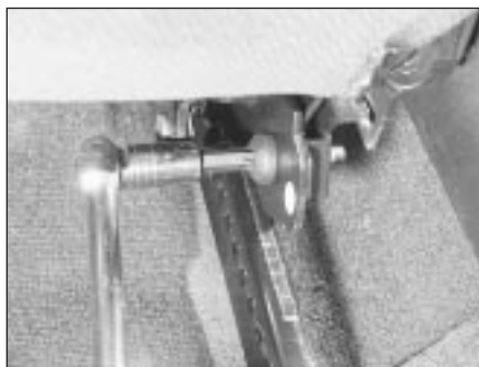
28.5C ... and unscrew the seat belt end retaining bolt
