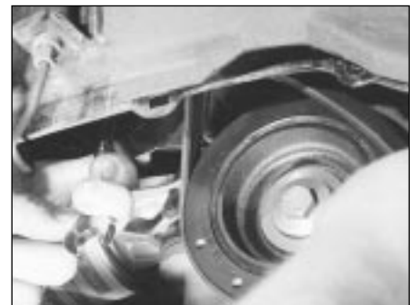
11.9 Rotate the tensioner pulley clockwise to release its pressure on the drivebelt, then slip the drivebelt off the crankshaft pulley
