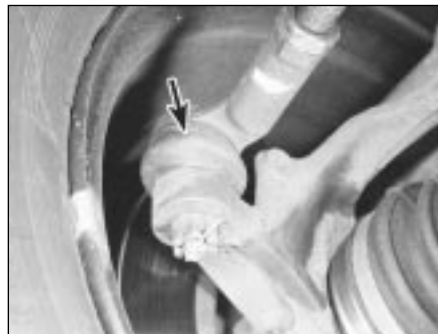
19.2A Check the condition of the track rod balljoint dust cover (arrowed)
