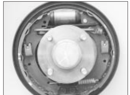
6.2A Note the fitted position of the springs and the adjuster strut, then clean the components with brake cleaner, and allow to dry. Position a tray beneath the backplate, to catch the fluid and residue
