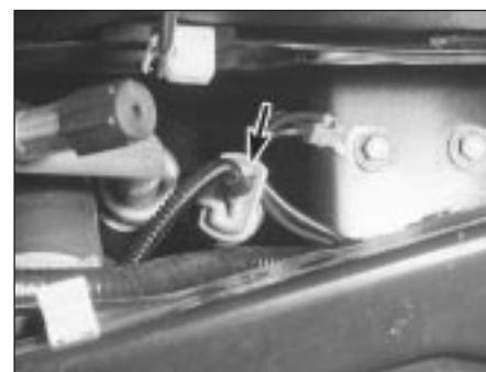
12.23 Unplug pressure-cycling switch electrical connector (arrowed)
