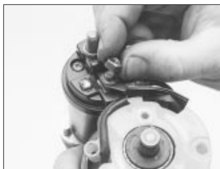
17.2E . . . unscrew the nut securing the solenoid link . . .
