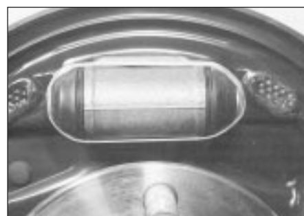
6.2J To prevent the wheel cylinder pistons from being accidentally ejected, fit a suitable elastic band or wire lengthwise over the cylinder/pistons. Don't press the brake pedal while the shoes are removed
