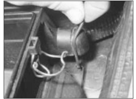
4.4 Remove rubber retaining band to withdraw air cleaner assembly
