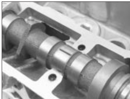
13.13A Lay a strip of Plastigage on each camshaft journal
