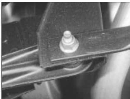
23.2 Front lower arm-to-crossmember securing bolt
