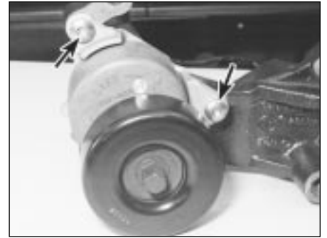
11.6 The auxiliary drivebelt is tensioned by an automatic tensioner; Torx screws (arrowed) secure it to alternator mounting bracket
