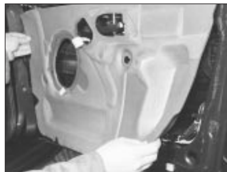
11.12 Removing the foam insulation
