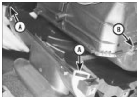
9.12 . . . release clips (A) to free air distributor from base of heater unit - note clips (B) securing . . .
