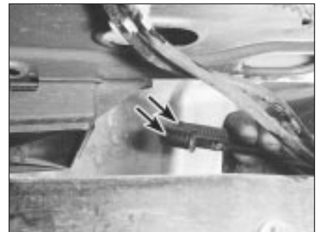
5.16 . . . unplug hoses (arrowed) from canister assembly . . .
