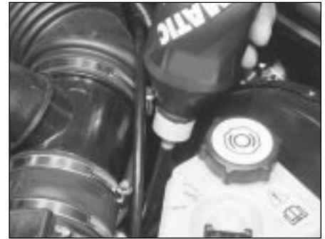
7.6B Adding automatic transmission fluid through the dipstick tube
