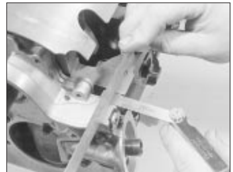
16.13 Check the oil pump is positioned correctly
