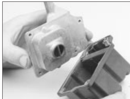
7.17A Remove four screws to release filter housing top from base . . .
