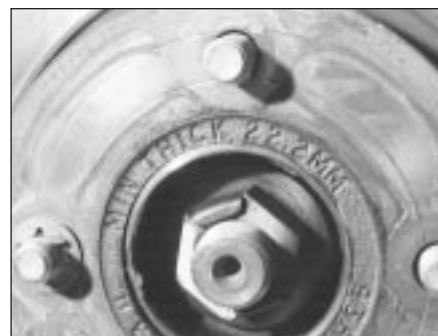
4.4B Disc minimum thickness marking
