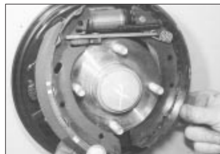
6.2G Move the bottom ends of the brake shoes together, and disconnect the top ends of the shoes from the wheel cylinder, taking care not to damage the rubber boots
