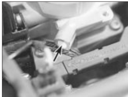
3.45 Throttle housing air bypass screw is sealed on production with a white tamperproof plug (arrowed)
