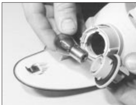
5.15 Removing the front direction indicator bulb
