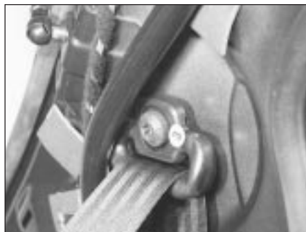
28.7A Rear seat belt shackle mounting bolt
