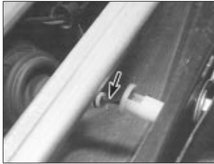
12.7B . . . and disconnect the speedometer main cable from the intermediate cable
