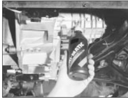
16.2 Topping-up the manual transmission oil
