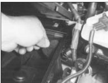
30.5 The Positive Crankcase Ventilation (PCV) system filter in the air cleaner assembly must be cleaned whenever the air filter element is renewed
