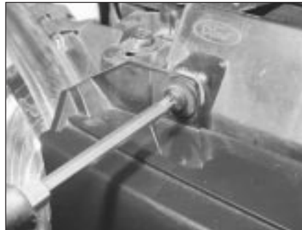
7.2 Removing a radiator grille mounting screw
