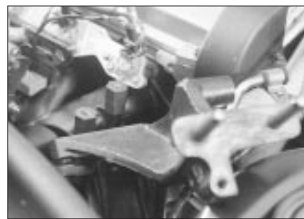
6.15 Alternator mounting bracket must be unbolted from rear of cylinder block to permit access to inlet manifold nut
