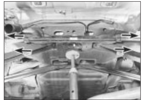
5.14 Support rear suspension crossmember on jack, and remove mounting bolts (arrowed) . . .
