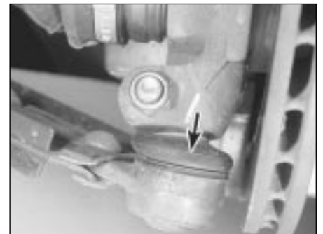
19.2B Check the condition of the lower arm balljoint dust cover (arrowed)
