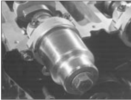
12.5 Using socket and toothed pulley bolt to install camshaft oil seal
