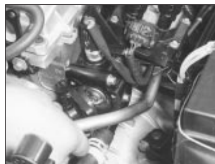
4.5 Unbolt water outlet to withdraw thermostat
