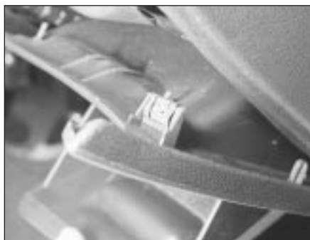
29.23C . . . and withdraw the lower facia panel
