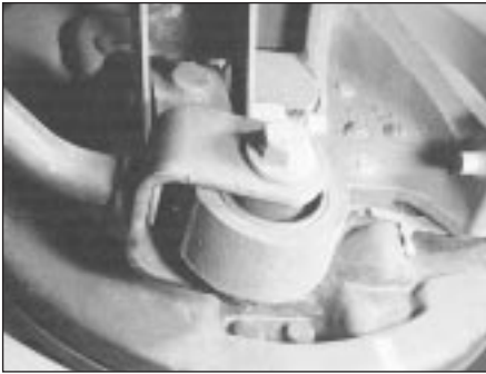
11.8A Tie-bar mounting bolt on knuckle
