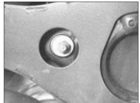
20.2B View of the anti-roll bar link nut through the rear lower arm
