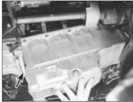
15.18 Engine/transmission lower adaptor plate (arrowed) must be refitted with sump
