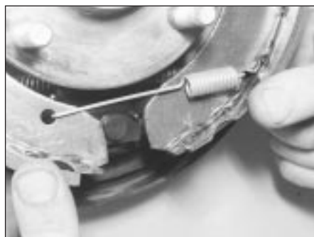
6.2E Release the trailing (rear) brake shoe from the anchor, then move the bottom ends of both shoes towards each other
