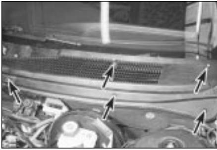
27.3 Remove screws (arrowed) to release cowl grille panel . . .
