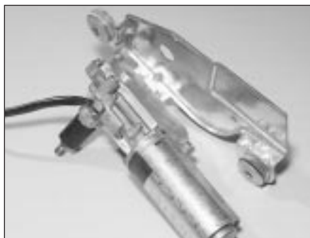
17.7A Tailgate wiper motor assembly and mounting plate
