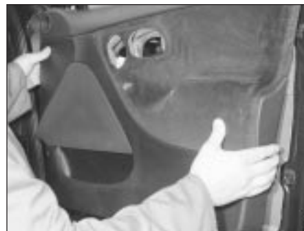
11.8D ... then lift off the trim panel
