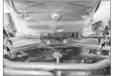
5.21 Refitting rear suspension crossmember with Ford service tools (arrowed) in place to align it with underbody ...
