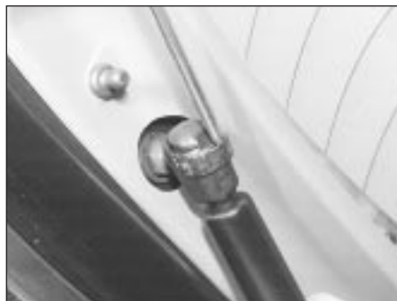
21.2 Prising the spring clip from the upper end of the strut
