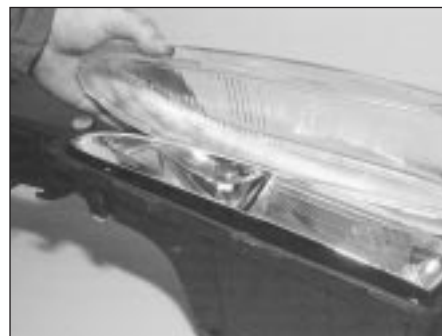
7.9B . . . and remove the headlight lens
