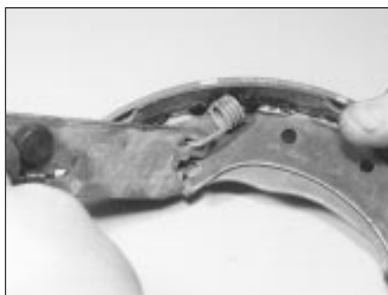
6.2L Unhook the automatic adjustment strut from the trailing brake shoe . . .
