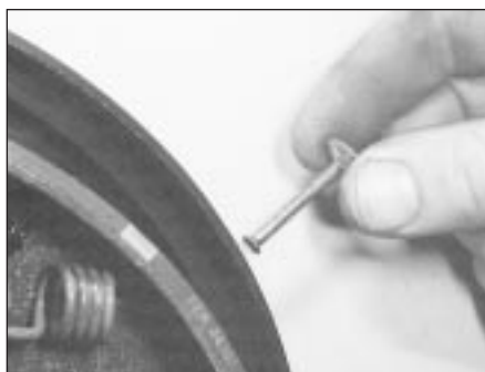
6.2C Remove the hold-down pins from the backplate
