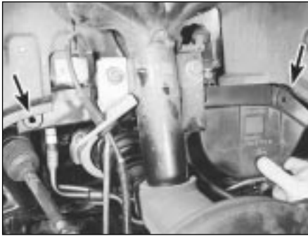
11.3 Removing the auxiliary drivebelt cover - it is secured by a fastener at each end (arrowed) - from inside the right-hand front wheel arch
