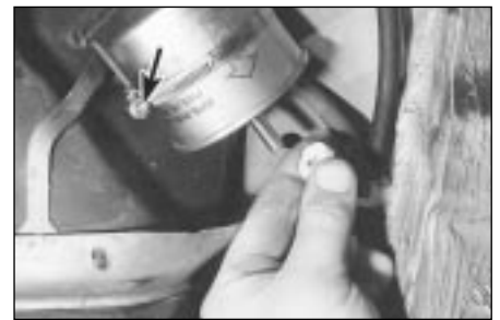
33.7B . . . secure pipe unions as described - do not overtighten clamp screw (arrowed)
