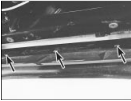
28.11 Ensure radiator undershield is located securely in three clips at front edge (arrowed) when refitting
