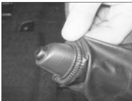
30.7B Passing the gaiter over the handbrake lever
