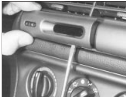
13.2 Prising the clock out of the facia
