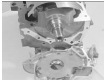
16.12 Use new gasket when refitting oil pump
