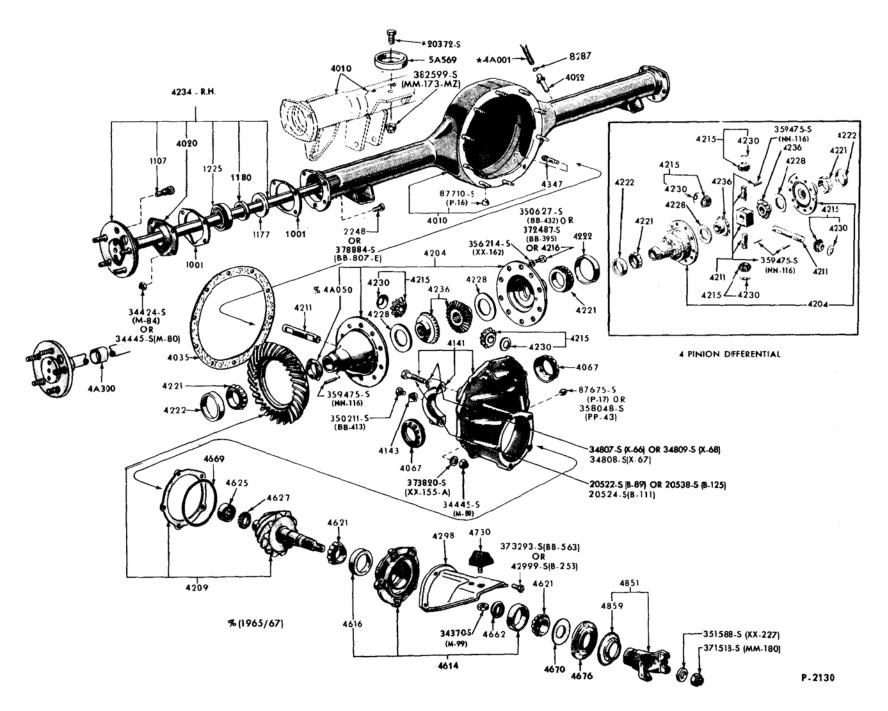
REAR AXLE - NON LOCKING WITH SEPARATE CARRIER - TYPICAL 7 3/4", 8", 8 3/4", 9" RING GEAR 1966 /72 BRONCO, 1965 / 72 FALCON, FAIRLANE/TORINO, FORD, MUSTANG 1971 / 72 MAVERICK, 1965 / 67, 1970/72 THUNDERBIRD
