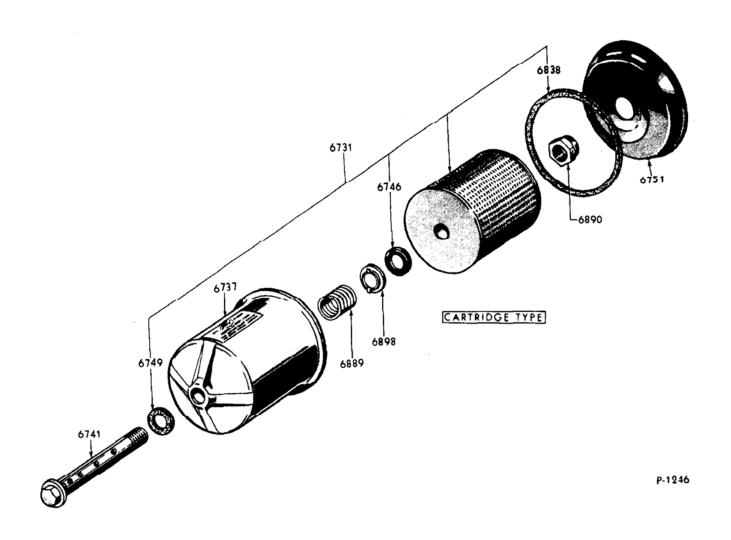
ENGINE FILER AND RELATED PARTS - CARTRIDGE TYPE - TYPICAL 1965 / 72 6 CYLINDER 170, 200, 240, 250 AND 8 CYLINDER 260, 289, 302 AND 351
