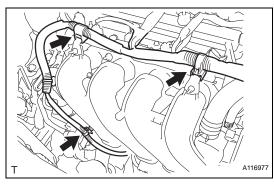
(b) Install the intake manifold with the 3 bolts and 2 nuts.
