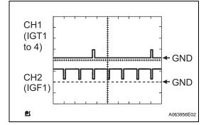
Reference: Inspection using an oscilloscope. While cranking or idling the engine, check the waveform between terminals IGT (1 to 4) and E1, and IGF1 and E1 of the ECM connector.
