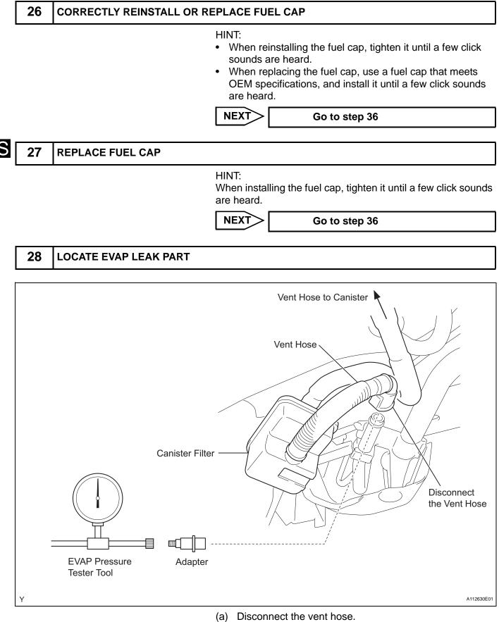
(b) Connect the EVAP pressure tester tool to the vent hose with the adapter.
