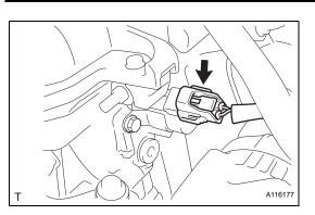
(c) Connect the camshaft timing oil control valve assembly connector.
