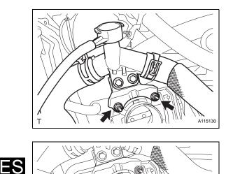
(c) Install the water filler sub-assembly with hose using the 2 nuts.
