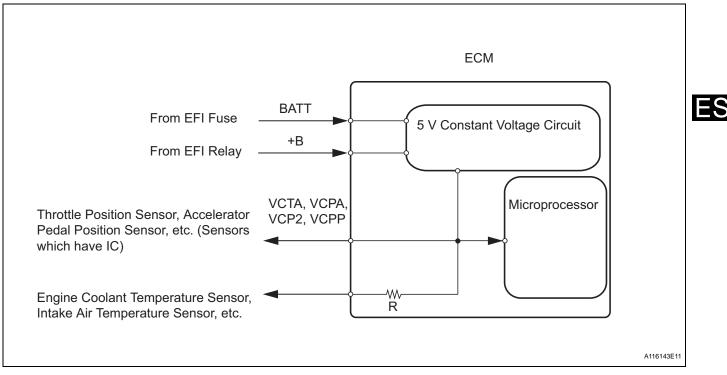
When the VC circuit is short-circuited, the microprocessor in the ECM and sensors that are supplied with power through the VC circuit are inactivated because the power is not supplied from the VC circuit. Under this condition, the system does not start up and the MIL does not illuminate even if the system malfunctions.
