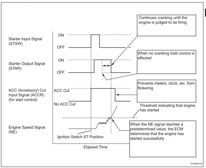
While the engine is being cranked, the positive battery voltage is applied to terminal STA of the ECM. If the ECM detects the Starter Control (STA) signal while the vehicle is being driven, it determines that there is a malfunction in the STA circuit. The ECM then illuminates the MIL and sets the DTC. This monitor runs when the vehicle is driven at 12.43 mph (20 km/h) for over 20 seconds.
