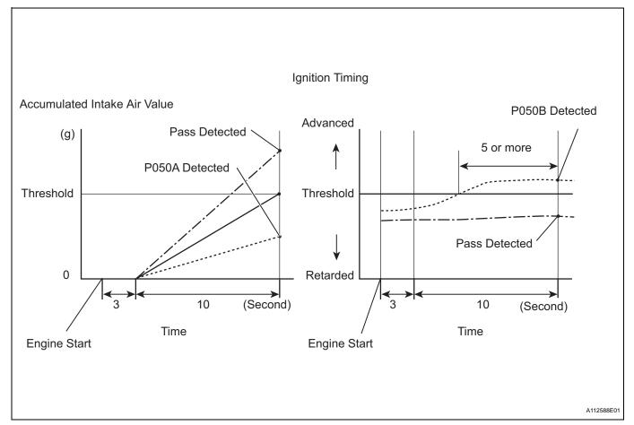
The ECM monitors the intake air amount during idling and the ignition timing.
