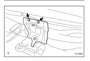
(b) Install the cowl top panel outer center bracket and install the 2 bolts.
