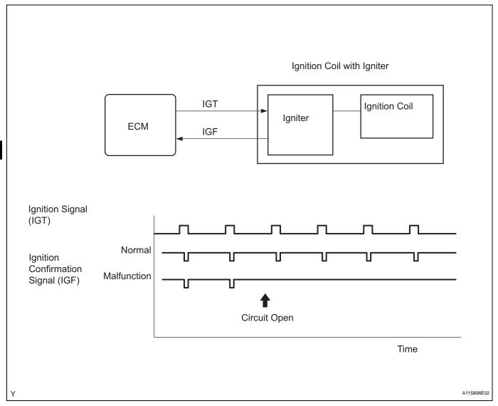
If the ECM does not receive any IGF signals despite transmitting the IGT signal, it interprets this as a fault in the igniter and sets a DTC.
