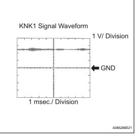
The correct waveform is as shown.
