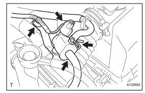
(c) Connect the wire harness clamp and mass air flow meter connector.
