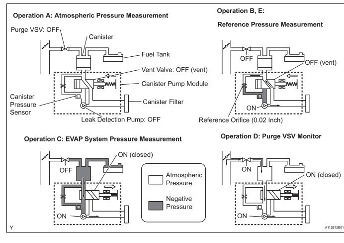
1. P2401: Leak detection pump stuck OFF
