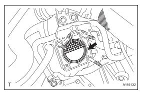
(e) Remove the gasket from the intake manifold.
