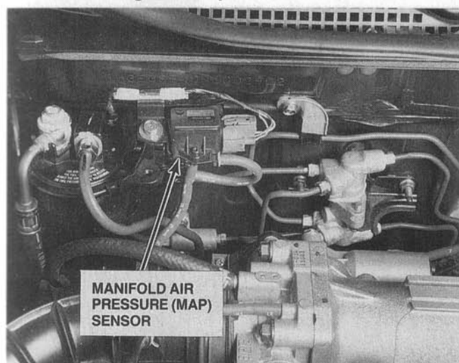
26. Rear of Engine Compartment
