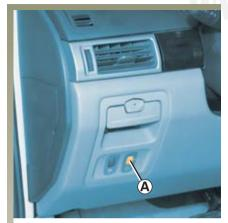
On vehicles fitted with this function, control  $\boldsymbol{A}$  allows you to adjust the height of the beams according to the load.
