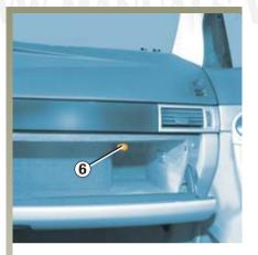
This storage compartment is ventilated and air conditioned the same as the passenger compartment.
