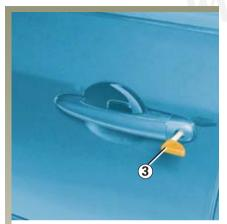
Using the separate emergency key 3 (depending on vehicle)
