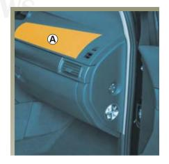
The airbag system uses the principles of pyrotechnics. This explains why, when the airbag inflates, it will generate heat, produce smoke (this does not mean that a fire is about to start) and make a noise upon detonation. In a situation where an airbag is required it will inflate immediately and this may cause some minor, superficial grazing to the skin.
