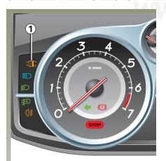
The particle filter warning light 1 lights up to show that the filter is liable to become saturated.
