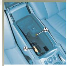
**Emergency release** (battery fault of system not available).
