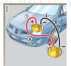
Fix the positive cable (+) A on the terminal (+) 1 of the flat battery, then onto the terminal (+) 2 of the battery supplying the current.
