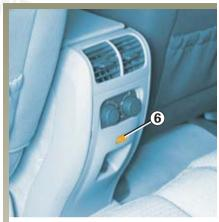
Doors and boot status indicator With the switched ignition on, the indicator lights integrated into switches 5 and 6 inform you whether or not the doors and tailgate are open:
