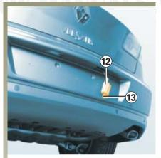
Registration plate lights 12 Unclip light 12 by pressing tab 13. Remove the light cover to gain access to bulb.
