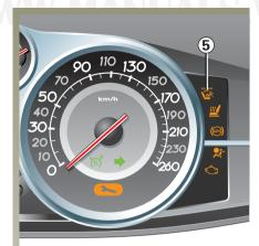
With the ignition switched on, check that warning light 5, AIRBAG OFF on the dashboard is lit up.
