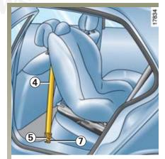
For the mounting ring on a rear-facing seat, use belt 4 supplied with the seat:
