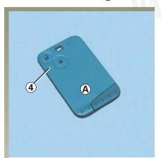
The RENAULT cards  $\boldsymbol{A}$  and  $\boldsymbol{B}$  are powered by a battery that should be replaced when the battery indicator light  $\boldsymbol{4}$  no longer lights up (refer to the information on "RENAULT card: battery", in Section 5).
