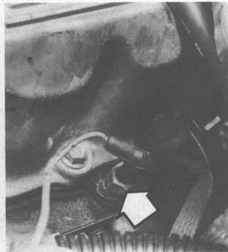
6.1c The coolant temperature sending unit on inline six-cylinder engines is located near the left rear corner of the cylinder head (arrow)
