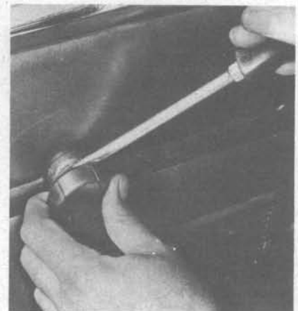
12.3 Pry off the crank handle
