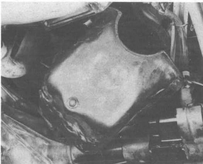
15.13 . . . then remove the oil pan from the rear by sliding it out between the axle and bellhousing
