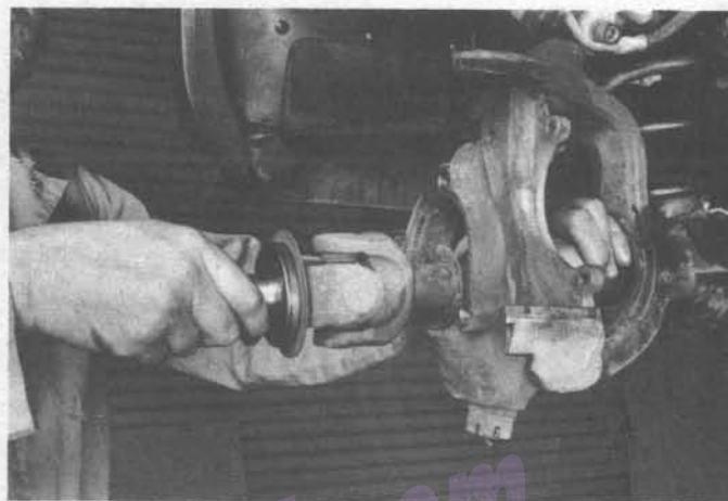
16.4 Once the hub and bearing assembly has been removed, the axleshaft can be pulled straight out of the housing
