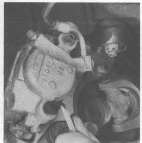
3.6b Using an Allen wrench, unscrew the two caliper mounting pins
