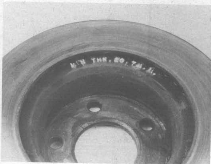
5.5a The minimum thickness is cast into the inside of the disc
