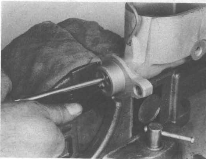
8.7 Use a Phillips head screwdriver to push the primary piston into the cylinder, then remove the snap-ring with a pair of snap-ring pliers
