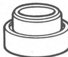
12.3 A special tool is recommended for crankshaft front seal installation
