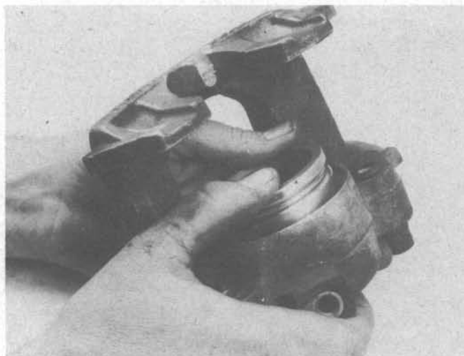
4.15 When installing the piston, make sure it doesn't become cocked in the caliper bore while pushing it down
