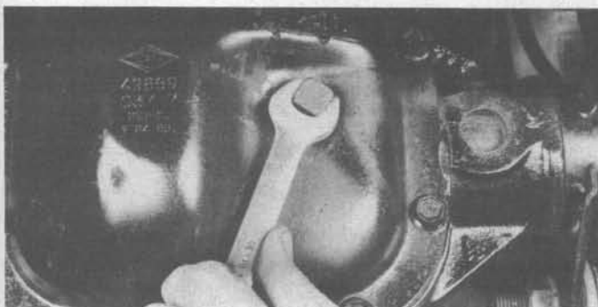
17.2 Use the correct size open-end wrench to remove the differential check/fill plug
