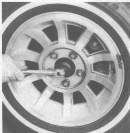
15.1 Before raising the vehicle, remove the cotter pin and nut lock, then loosen the axle hub nut
