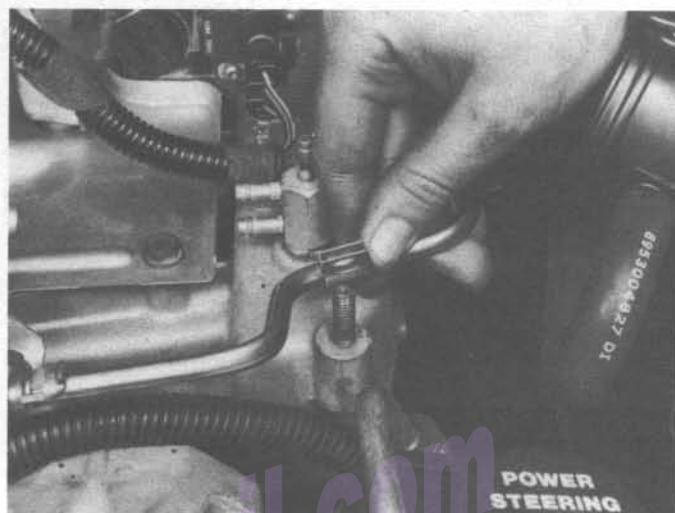
15.23b Remove the nut from the fuel return line bracket and slide the bracket off its mounting stud, ...
