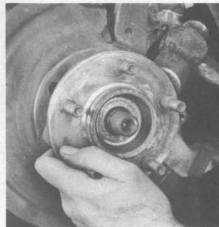
15.4b Carefully tap the hub assembly out of the steering knuckle
