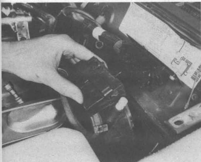
5.5b Remove the attaching screw and unplug the firewall electrical connector
