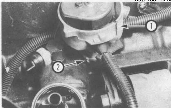
13.6 Before loosening the distributor hold-down bolt, make a mark on the edge of the distributor base directly below, and in line with, the rotor tip (1), then mark the distributor base and the engine block (2) to ensure that the distributor is installed correctly
