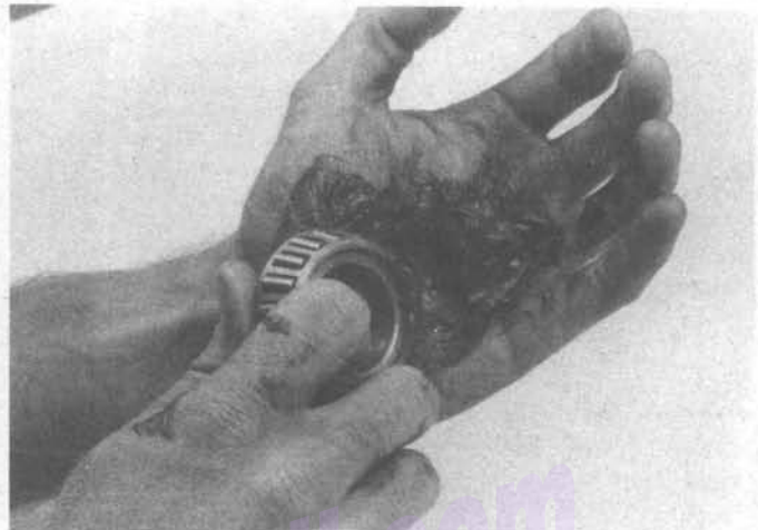
38.15 Work the grease into each bearing from the large-diameter side until grease oozes out the small-diameter side
