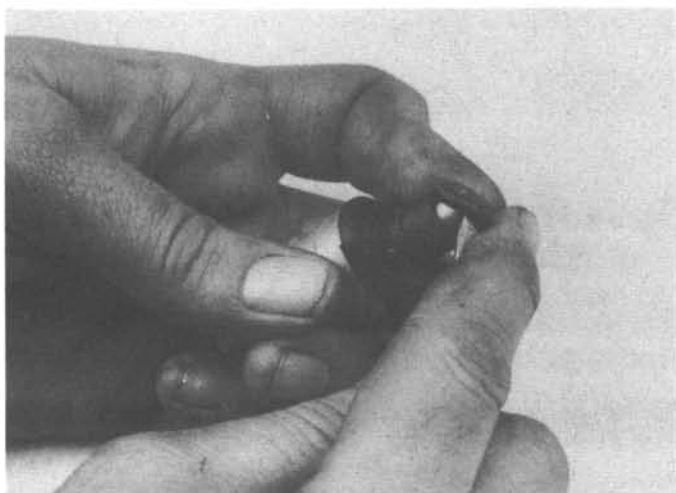
15.33 Be sure to remove the old O-ring and seal from the injector (a replacement kit, available at a dealer, includes six O-rings and seven seals — enough O-rings and seals for all six injectors and an extra seal for the fuel pressure regulator)
