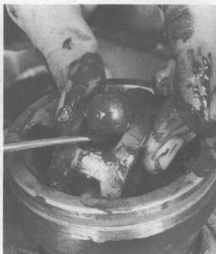
16.12b If necessary, pry the ball bearings out with a screwdriver
