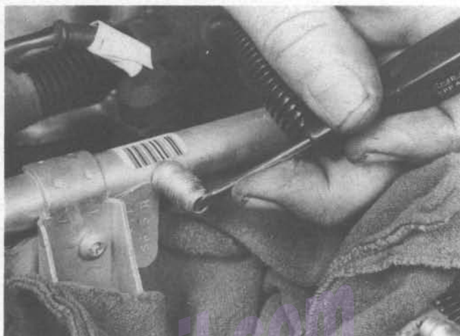
2.7 . . . then depress the valve in the test port with a small screwdriver or pin punch — wear safety goggles during pressure relief to protect your eyes from spraying fuel
