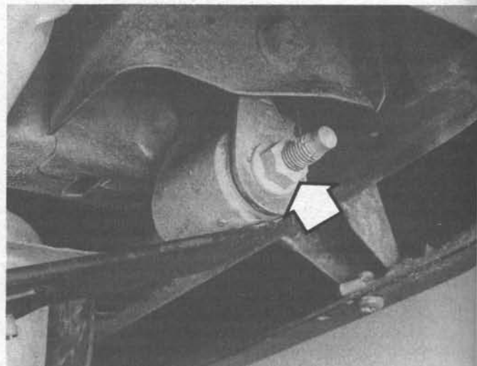
11.6 Unscrew the nut (arrow), then remove the rear spring-to-shackle bolt
