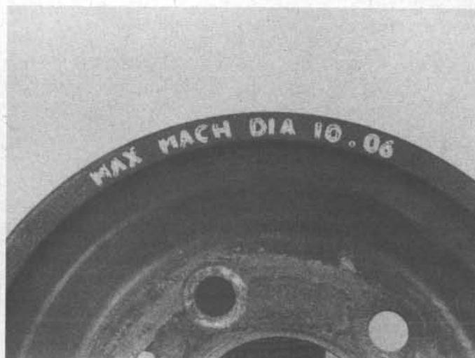
6.5 The maximum allowable drum diameter is cast into the drum
