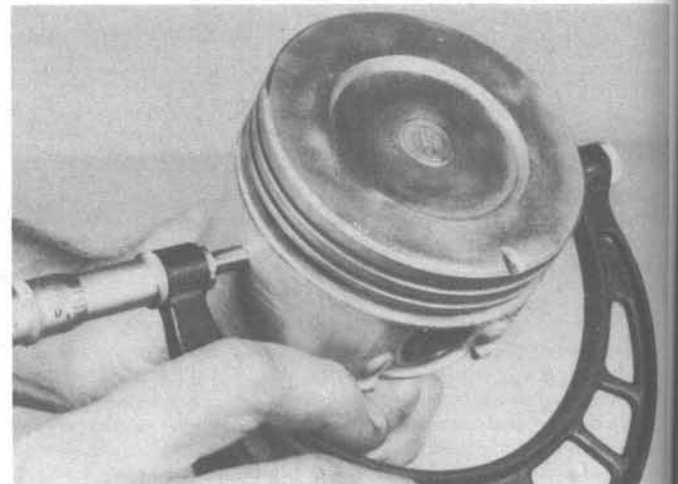
17.11a Measure the piston diameter at a 90° angle to the piston pin and in line with it
