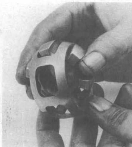
16.14 Align the inner race lands with the cage windows and rotate the inner race out of the cage
