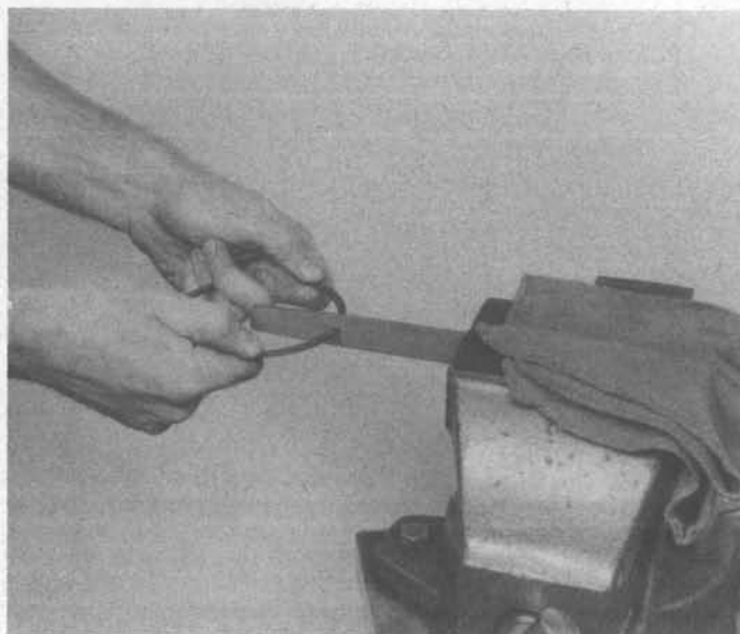
21.5 If the end gap is too small, clamp a file in a vise and file the ring ends (from the outside in only) to enlarge the gap slightly
