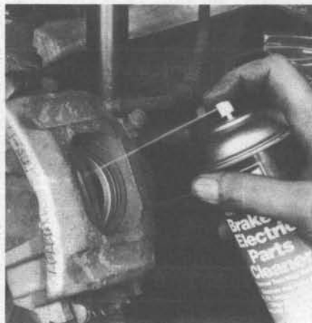
3.6a Before removing the caliper, wash off all traces of brake dust with brake system cleaner
