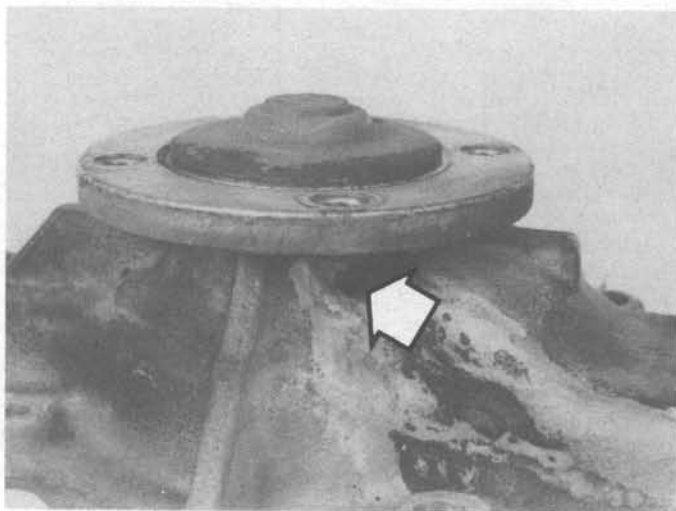
8.4 The water pump weep hole (arrow) will drip coolant when the seal on the pump shaft fails (pump removed from engine for clarity)
