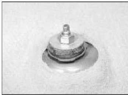
12.2 Rear shock absorber upper mounting - Hatchback
