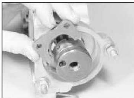
9.5b Removing the camshaft thrust plate
