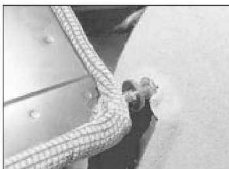
33.3b Seat pivot lifts out of hinge
