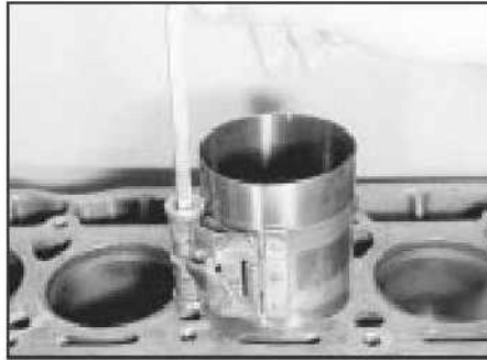
15.12 Piston ring compressor fitted
