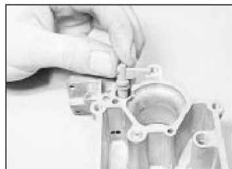
19.11 Removing the fuel discharge nozzle
