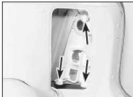
11.17a Rear lamp unit retaining screws (arrowed) Hatchback
