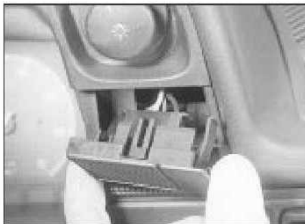
4.5 Removing a foglamp switch
