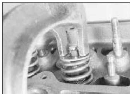
9.20 Compress the spring and fit the collets
