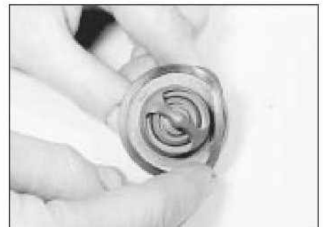
4.14 Fitting a new seal to the thermostat
