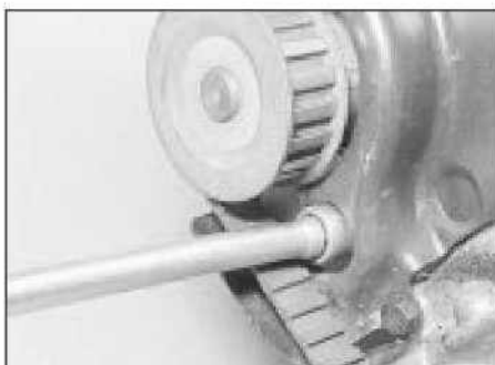
7.8 Slackening a water pump bolt
