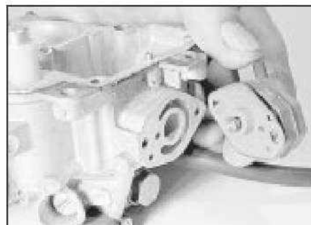
21.6 Removing the part-load enrichment device
