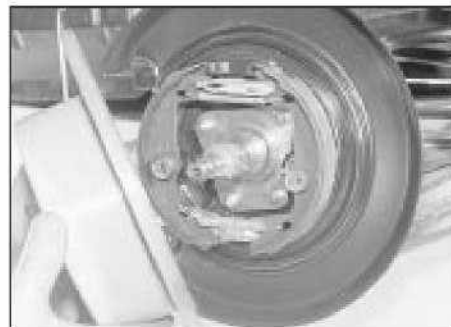
8.5 Removing the rear disc
