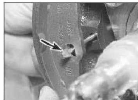
20.3b . . . and the rear steady pin
