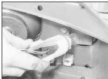
11.9 Removing a direction indicator bulb and holder
