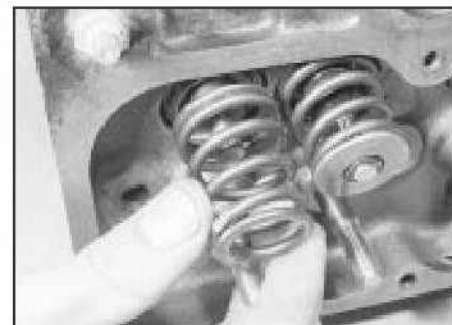
9.18a Fit the valve spring . . .
