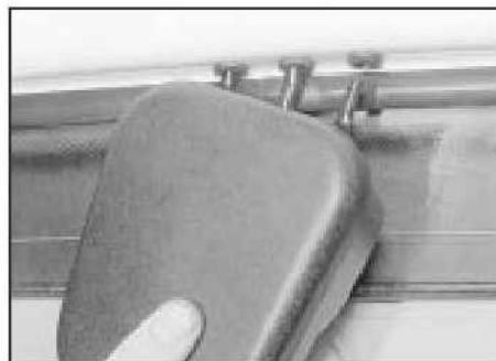
21.9 Removing the window-mounted motor
