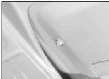
26.9 Boot lid handle retaining nut
