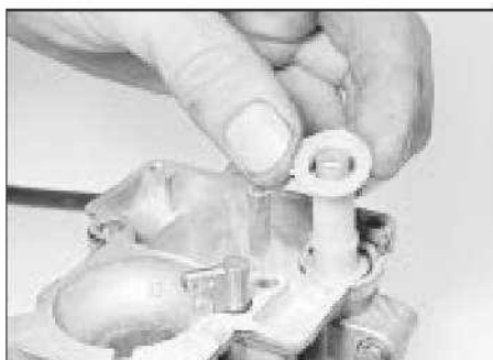
21.7a Removing the accelerator pump collar ...
