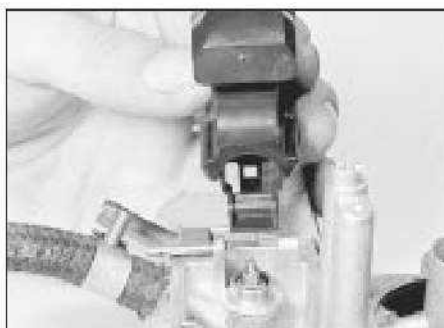
21.9a Removing the float ...
