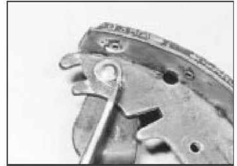
6.16 Handbrake lever secured by pin
