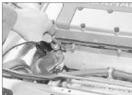
14.3 Removing an exhaust manifold heat shield bolt
