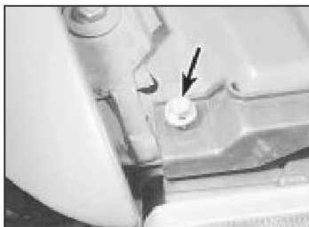
12.3a Headlamp lens outboard securing screw (arrowed)
