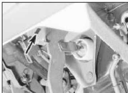
17.1 Stop-lamp switch 'keyhole' mounting (arrowed)
