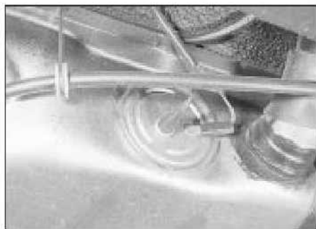
6.2 Fuel gauge sender unit (screw-fit sender unit)
