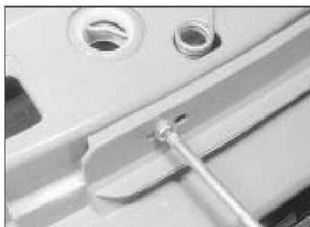
8.2 Undoing a front trim panel screw
