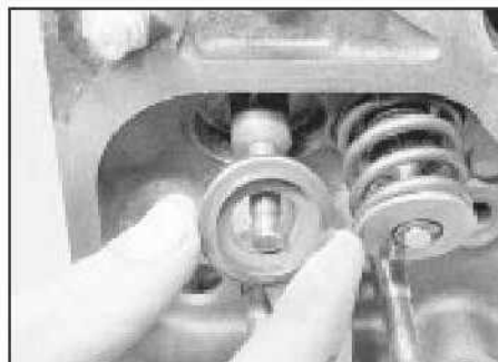
9.17 Fitting an exhaust valve rotator
