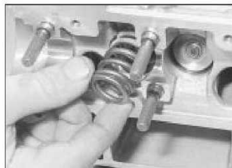
12.6c ... the valve spring ...
