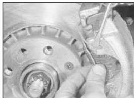
4.17 . . . then lever out the spring clip
