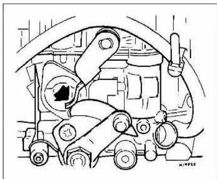
14.11 Accelerator pump adjustment point. Loosen clamp screw (under arrow) and rotate the cam plate
