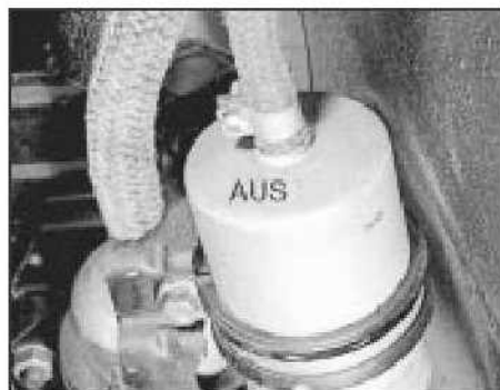
25.4 Fuel filter directional marking
