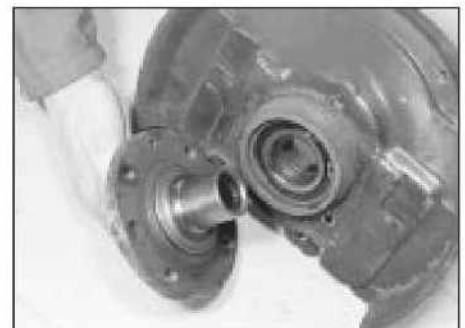
3.3b Hub removed from the carrier
