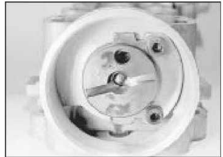
3.19c ... to engage the offset slot in the camshaft
