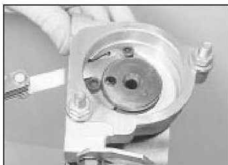
9.10 Checking the camshaft endfloat
