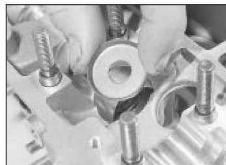
12.6e ... and the valve spring seat
