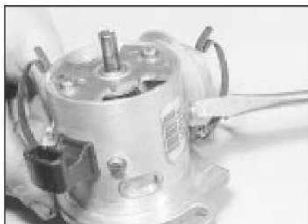
4.16a Removing a vacuum unit retaining screw
