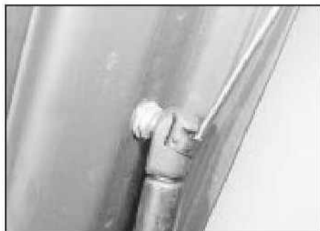
22.2 Releasing a tailgate strut spring clip
