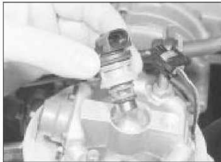
11.6c ... and remove the injector
