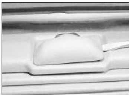
11.22 Prising out the number plate lamp
