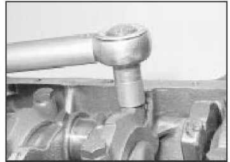
20.16b Tightening a main bearing cap bolt
