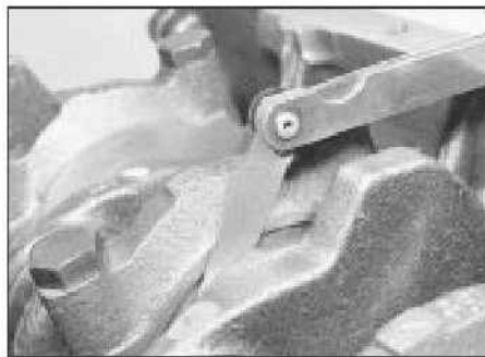
20.19 Checking crankshaft endfloat
