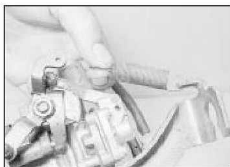
19.3 Removing the throttle return spring
