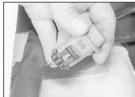
2.10 Octane plug in the "95" position - later 1.6 litre models
