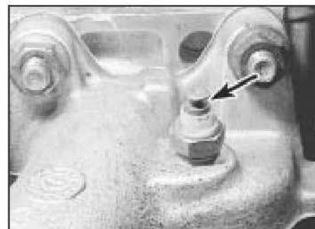
32.19b On 1.3 litre models, unscrew temperature gauge sender unit from the manifold to bleed the cooling system
