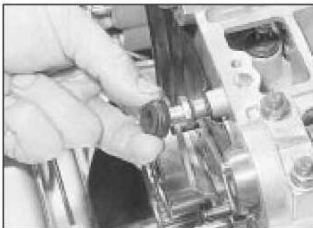
11.18a Remove the rubber bush ...
