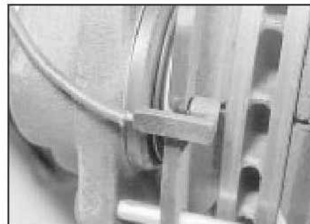
4.4b Wear warning sensor clipped to pad
