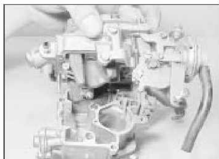
19.5b Separating the cover from the float chamber housing
