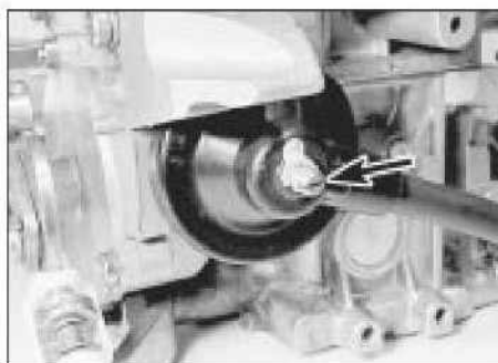
14.8a Choke valve gap adjustment screw (arrowed)
