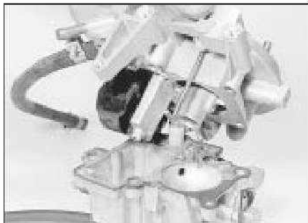
21.3 Lifting off the carburettor top cover
