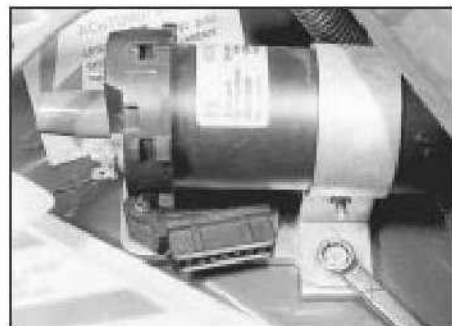
6.4a Removing a coil securing bolt
