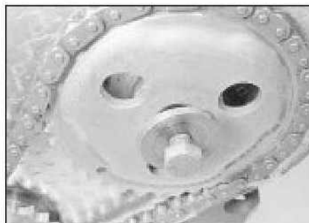
14.10 Camshaft sprocket retaining bolt and washer
