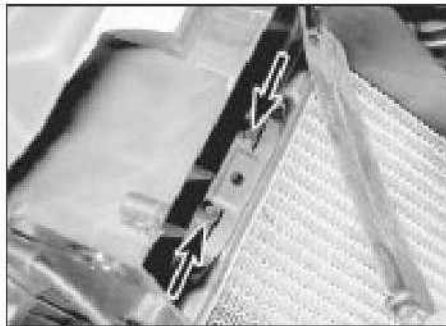
9.17b Heater matrix upper securing screws (arrowed)
