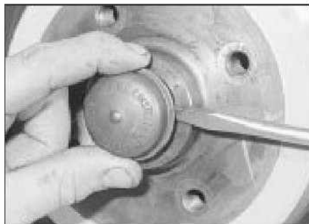
8.3 Levering off the grease cap
