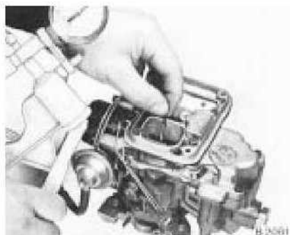
16.10 Choke pull-down measurement
