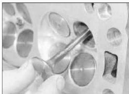
12.6a Remove the valve ...
