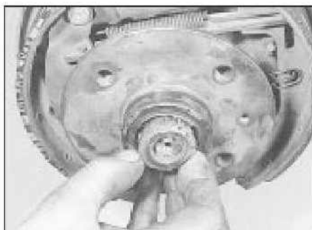
10.6a Fit the outer bearing race . . .
