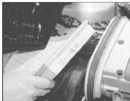
24.13 Fitting a new air cleaner element - 2.0 litre 16-valve models
