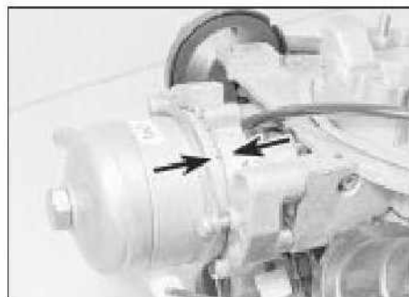
15.12 Choke cover alignment marks (arrowed)
