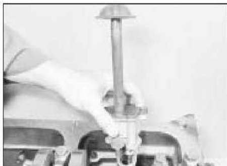
12.2b ... and remove the oil pump
