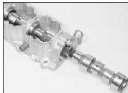
9.6 Removing the camshaft from the housing
