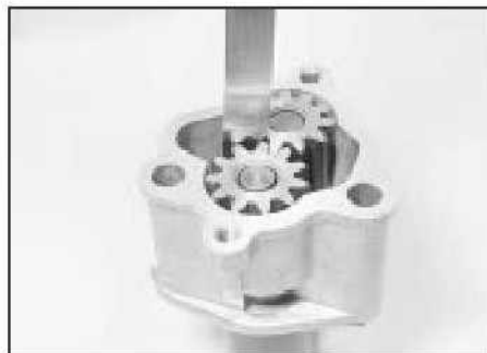
13.8 Check the pump gear teeth backlash
