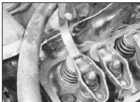
7.10 Checking a valve clearance
