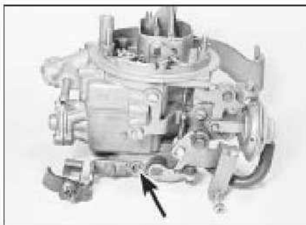
11.7a Mixture (CO) adjustment screw - 32TL carburettor
