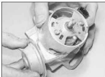
4.16b Removing the vacuum unit
