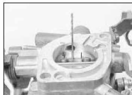
12.3 Using a drill bit to check the fast idle gap
