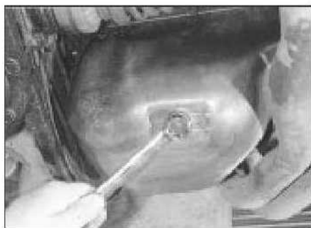
6.4 Removing the sump drain plug
