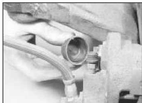
10.6a On the GMF caliper, remove the caliper bolt caps . . .
