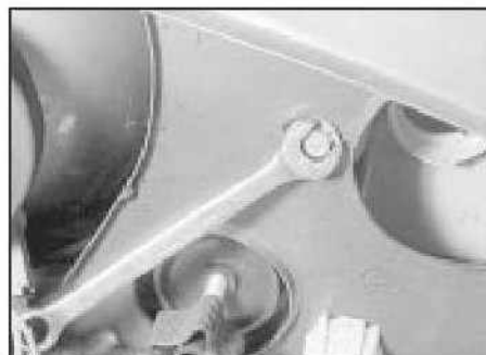
12.2a Undoing a direction indicator lens screw
