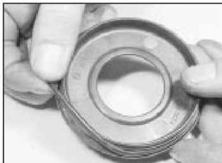
3.27 Renewing the insulator sealing ring
