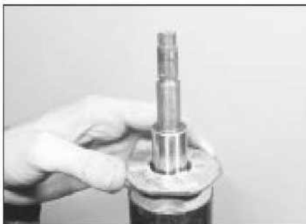
4.6b Removing the strut ring nut
