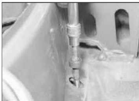
16.8 Removing a servo bracket screw
