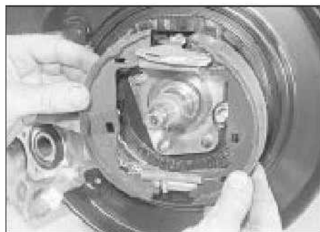
20.4 Removing the handbrake shoe assembly
