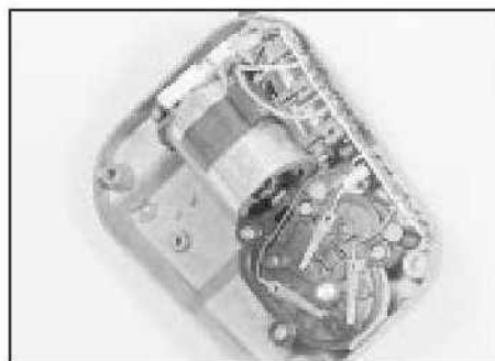
21.13c ... and remove the motor cover to gain access to the motor wiring
