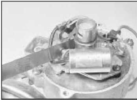
3.6 Checking the contact breaker points gap using a feeler blade
