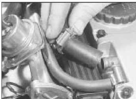
11.7 Disconnecting the small breather hoses from the camshaft cover
