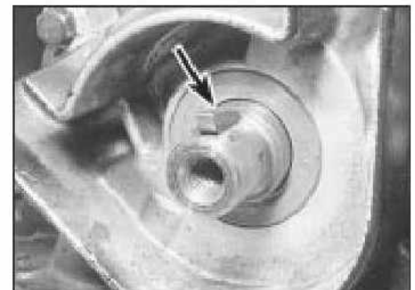
13.2b Woodruff key (arrowed) in crankshaft nose
