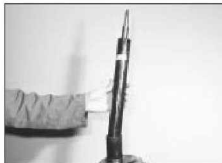
4.7 Removing the shock absorber cartridge
