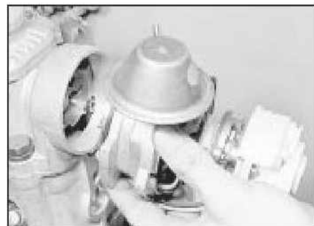
3.5 Removing the distributor from the camshaft housing
