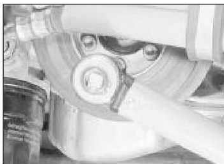
7.14 Tightening one of the crankshaft pulley screws
