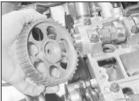
10.3b Removing a camshaft sprocket
