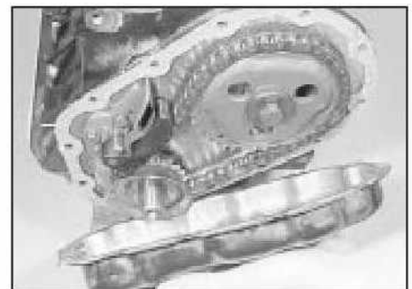
14.21 Refitting the timing cover
