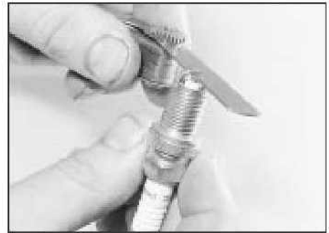
7.10a Measuring a spark plug electrode gap using a feeler blade
