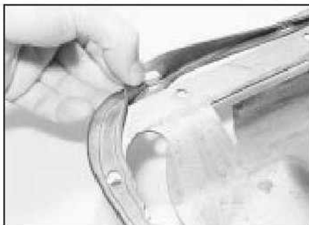
12.7b . . . while this one has one double-sided rubber gasket
