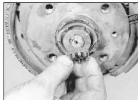
10.6b . . . the washer and the castellated nut
