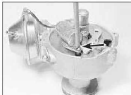
7.5 Undoing the condenser retaining screw
