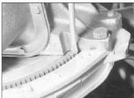
7.4 Jamming the flywheel ring gear
