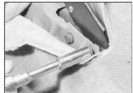
19.5 Unbolting the handbrake lever
