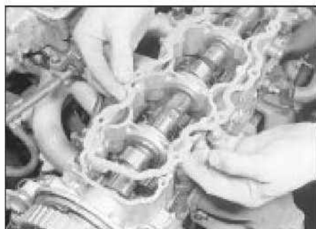
8.29a Fitting a new camshaft cover gasket
