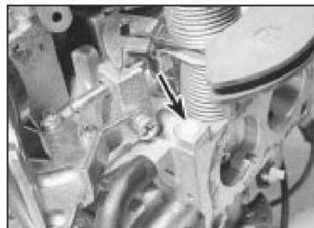
11.7b Mixture (CO) adjustment screw cap (arrowed) 2E3 carburettor
