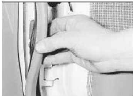
12.46b . . . and peel back the door surround strip
