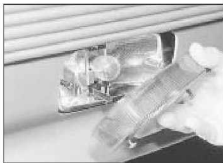
11.19 Removing a rear foglamp lens
