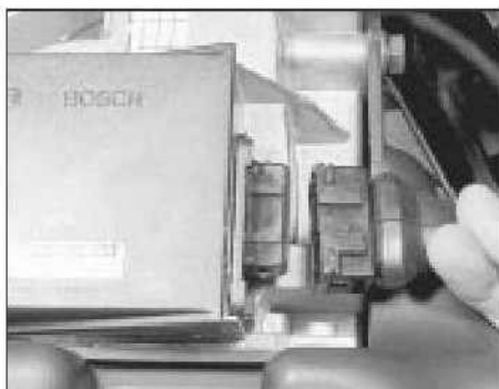
24.7 On 1.8 and 2.0 litre 8-valve models, disconnect the airflow sensor wiring connector ...
