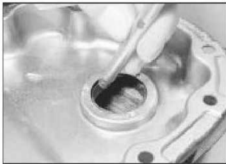
14.13 Using a drift to remove the timing cover oil seal
