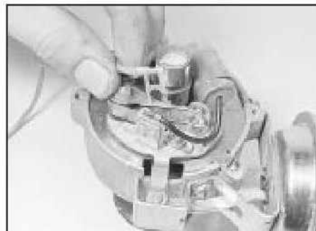
4.3 Slip the low tension and condenser leads out of the insulator
