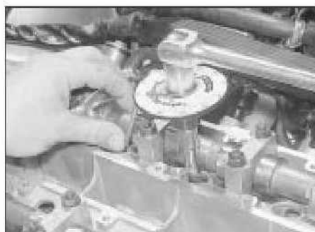
11.24b Angle tightening a cylinder head bolt
