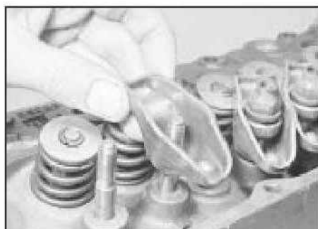
9.24a Fitting a rocker arm . . .
