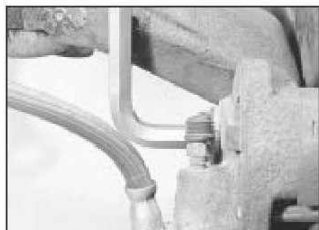
10.6b . . . then unscrew the caliper bolts . . .
