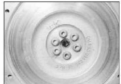
16.4 Flywheel retaining bolts are socket-headed
