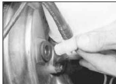
15.3 Brake servo vacuum connection at servo
