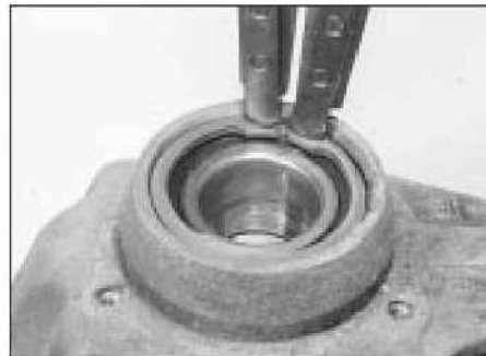
3.5b Removing a hub bearing circlip
