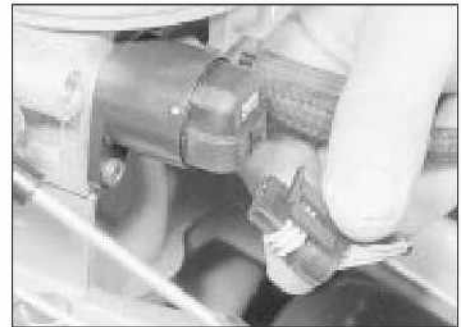
11.11a Detach the wiring connector ...
