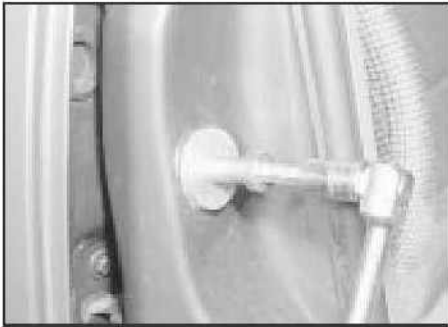
13.4 Adjusting a door lock striker
