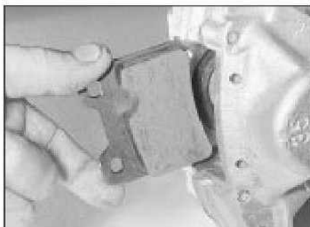
5.9a Fitting a rear pad
