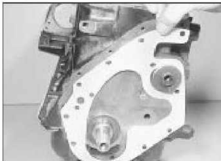
18.10 Fitting a new front plate gasket
