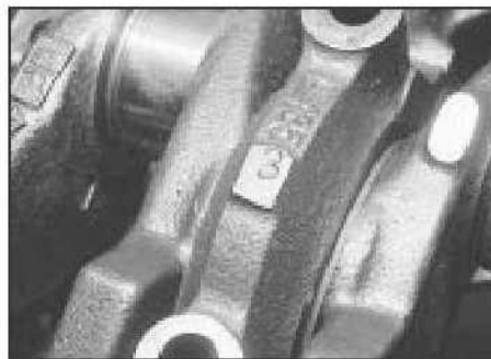
20.3 Identification number on No 3 main bearing cap
