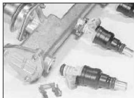
12.69b . . . and pull out the injector
