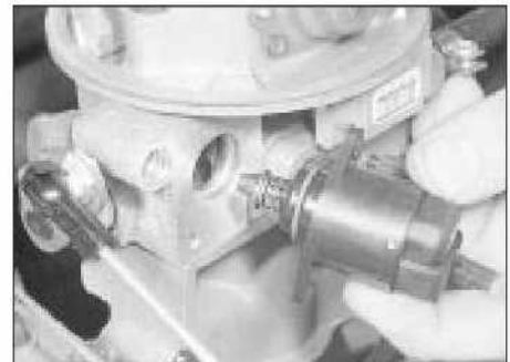
11.11c ... and remove the idle air stepper motor
