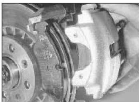
4.20 Lift the caliper off the disc . . .
