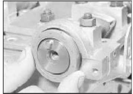
9.4a Fitting a new camshaft oil seal
