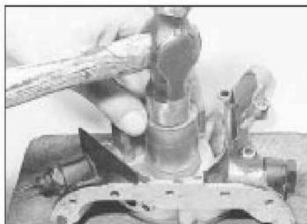
14.6 Fitting a new front oil seal
