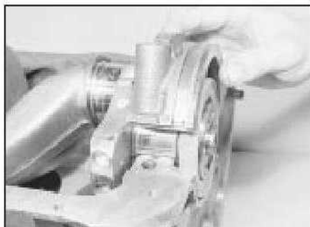
20.16 Fitting the rear main bearing cap
