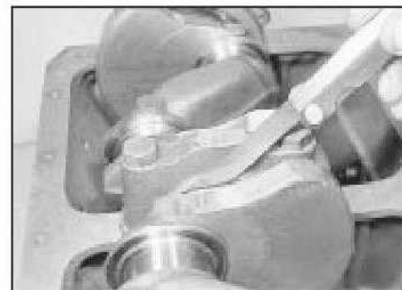
20.18 Checking the crankshaft endfloat
