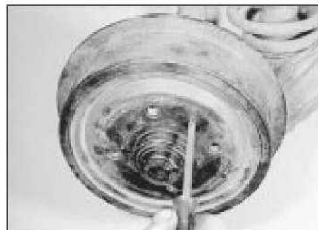
9.3a Removing a brake drum securing screw
