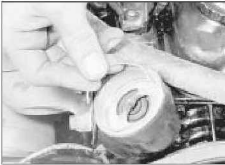
4.3a Remove the thermostat retaining snap-ring . . .
