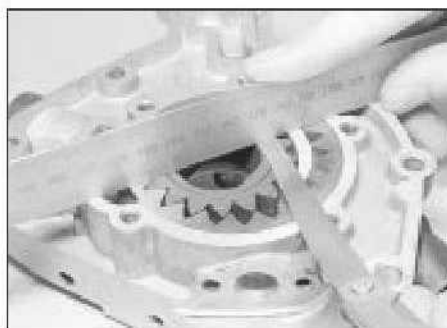
14.3 Checking oil pump gear endfloat
