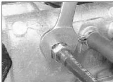
15.2 Brake servo vacuum connection at inlet manifold (fuel injection model)
