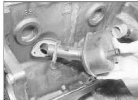
22.8 Crankcase ventilation system oil separator - 1.3 litre engine
