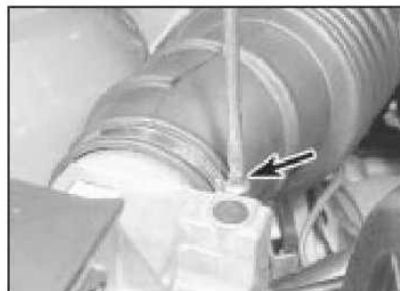
12.12 Disconnecting the airflow meter trunking
