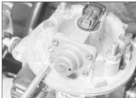
11.17a Undo the retaining screws ...
