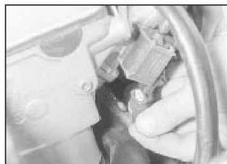
12.100 Disconnecting the vent valve multi-plug
