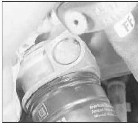
16.2 Circlip securing oil cooler thermostatic valve
