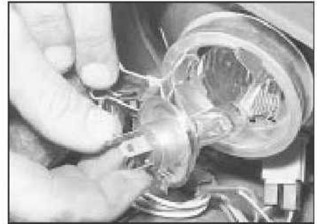
11.3 Removing a headlamp bulb
