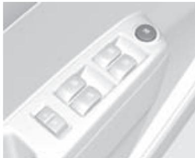
Pulse el interruptor
