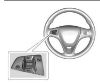
CRUIST: Press to turn the cruise control system on and off. A white indicator comes on in the instrument cluster when cruise is turned on.
