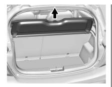
To remove, pull the cargo cover upwards.
