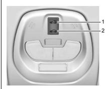
**Vent/Open:** Press and hold the switch (1) to vent. Press (1) again to express-open the sunroof. To stop the express-open press the switch
