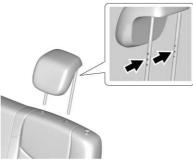
Insert the head restraint posts into the holes in the top of the seatback. The notches on the posts must face the driver side of the vehicle.
