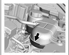
If coolant is visible but the coolant level is not at or above the mark pointed to, add a 50/50 mixture of clean drinkable water and DEX-COOL coolant.
