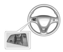
ENGINE : Press to turn the cruise control system on and off. A white indicator comes on in the instrument cluster when cruise is turned on.
