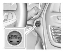
The vehicle may be equipped with an electronic keyless ignition with pushbutton start.
