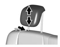
The height of the head restraint can be adjusted. Pull the head restraint up to raise it. Try to move the head restraint to make sure that it is locked in place. To lower the head restraint, press the button, located on the top of the seatback, and push the head restraint down. Try to move the head restraint after the button is released to make sure that it is locked in place.
