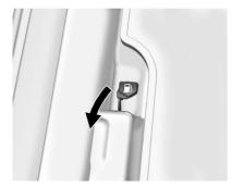
The tethered fuel cap is behind a hinged fuel door on the passenger side of the vehicle. To open the fuel filler door, lift the fuel door release lever. The lever is on the floor, on the left front side of the driver seat. The fuel door is unlocked when the vehicle is unlocked. Locking the vehicle locks the fuel door.
