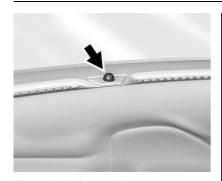
The vehicle has a light sensor on top of the instrument panel. Make sure it is not covered, or the headlamps will be on when they are not needed.
