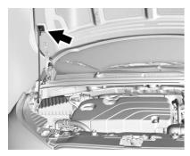
Lift the hood and release the hood prop rod from the prop rod retainer, which is under the hood.  Securely place the hood prop rod into the hood prop rod holder, at the rear passenger side of the engine compartment.
