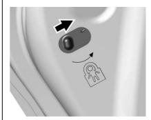
The vehicle has rear door safety locks on each rear door that prevent passengers from opening the rear doors from the inside.
