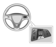
© I № : Press to interact with Bluetooth or OnStar, if equipped. See Bluetooth (Infotainment Controls) \$\dip 142\$ or Bluetooth (Overview) \$\dip 140\$ or OnStar Overview \$\dip 307\$.
