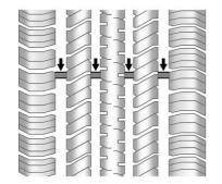
Treadwear indicators are one way to tell when it is time for new tires. Treadwear indicators appear when the tires have only 1.6 mm (1/16 in) or less of tread remaining. See *Tire Inspection* ⇒ 249 and *Tire Rotation* ⇒ 249.
