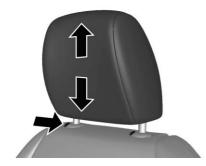
The height of the head restraint can be adjusted. Pull the head restraint up to raise it. Try to move the head restraint to make sure that it is locked in place. To lower the head restraint, press the button, located on the top of the seatback, and push the head restraint down. Try to move the head restraint after the button is released to make sure that it is locked in place.
