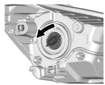
3. Remove the headlamp bulb socket.
