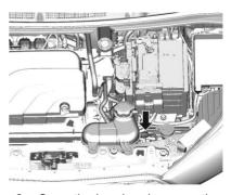
Open the hood and unwrap the electrical cord. The cord is located in the driver side of the engine compartment, near the engine coolant surge tank. It is shipped from the factory with a tie holding it in place. Use care in removing the tie so that the cord is not damaged.
