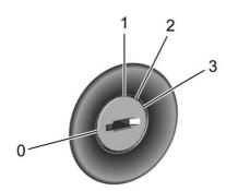
The ignition switch has four different positions.
