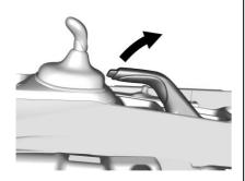
To set the parking brake, hold the brake pedal down and pull up on the parking brake lever. If the ignition is on, the brake system warning light will come on. See *Brake System Warning Light* \$\phi\$ 101.
