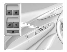
The driver power window switches control all the windows. The passenger switch controls only that window.
