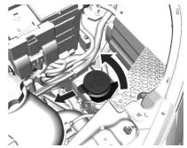
Remove the washer funnel by turning it counterclockwise.
