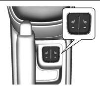
If available, the buttons are below the climate control system. To operate, the engine must be running.
