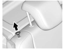
4. Pull up the release knob on the top of the seatback.
