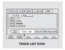
You can also select a file directly from a track list on the audio display. Press the AUDIO button to show the audio display, then touch the Track List icon. The track list menu appears on the display.
