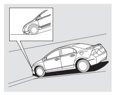
• Curbs and steep inclines could damage the front and rear bumpers. Low curbs that do not affect the average vehicle may be high enough to hit the bumper on your vehicle. The front or rear bumper may scrape when trying to drive onto an incline, such as a steep driveway or trailer ramps.
