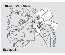
4. The coolant level should be up to the base of the filler neck. Add coolant if it is low.
