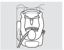
If you ever have a moderate to severe side impact, sensors will detect rapid acceleration and signal the control unit to instantly inflate either the driver's or the passenger's side airbag.
