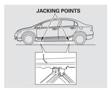
7. Place the jack under the jacking point. Turn the end bracket clockwise until the top of the jack contacts the jacking point. Make sure the jacking point tab is resting in the jack notch.
