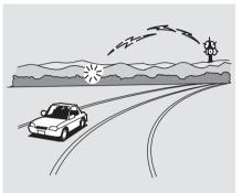
Driving very near the transmitter of a station that is broadcasting on a frequency close to the frequency of the station you are listening to can also affect your radio's reception. You may temporarily hear both stations, or hear only the station you are close to.
