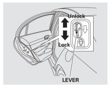
The childproof door locks are designed to prevent children seated in the rear from accidentally opening the rear doors. Each rear door has a lock lever near the edge. With the lever in the LOCK position, the door cannot be opened from the inside regardless of the position of the lock tab. To open the door, push the lock tab in, and use the outside door handle.
