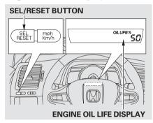
To see the current engine oil life, turn the ignition switch to the ON (II) position, and press the SEL/RESET button repeatedly until the engine oil life display appears (see page 66).
