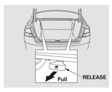
To release the seat-back, pull the release under the trunk panel. Push the seat-back down, then let go of the release.
