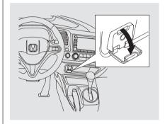
The auxiliary input jack is underneath the accessory power socket on the front panel. The system will accept auxiliary input from standard audio accessories using a 1/8 inch (3.5 mm) stereo miniplug.
