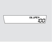
4. Press the SEL/RESET button for more than 5 seconds. The maintenance item code(s) will disappear, and the engine oil life will reset to "100."
