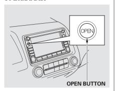
The disc player is behind the navigation screen. To use the disc player, press the OPEN button beside the screen. The screen folds back, and the disc player appears.
