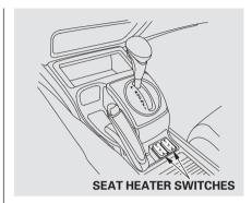
The ignition switch must be in the ON (II) position to use seat heaters. Push the top of the switch, HI, to rapidly heat up the seat. After the seat reaches a comfortable temperature, select LO by pushing the bottom of the switch. This will keep the seat warm.
