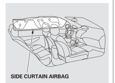
In a moderate to severe side impact, sensors will detect rapid acceleration and signal the control unit to instantly inflate the side curtain airbag and activate the seat belt tensioner on the driver's or the passenger's side of the vehicle.
