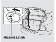
As a safety feature, your vehicle has a release lever on the trunk latch so the trunk can be opened from inside. To open the trunk, push the release lever in the direction pointed by an arrow.
