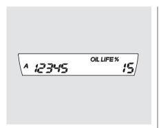
3. Press the SEL/RESET button for about 10 seconds. The engine oil life and the maintenance item code(s) will blink.
