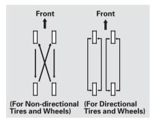
To help increase tire life and distribute wear more evenly, rotate the tires according to the maintenance messages displayed on the information display. Move the tires to the positions shown in the chart each time they are rotated. If you purchase directional tires, rotate only front-to-back.
