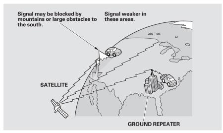
The XM satellites are in orbit over the equator; therefore, objects south of the vehicle may cause satellite reception interruptions. To help compensate for this, ground-based repeaters are placed in major metropolitan areas. Satellite signals are more likely to be blocked by tall buildings and mountains the farther north you travel from the equator. Carrying large items on a roof rack can also block the signal.
