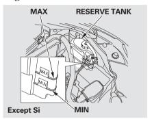
Look at the coolant level in the radiator reserve tank. Make sure it is between the MAX and MIN lines. If it is below the MIN line, see **Adding Engine Coolant** on page 294 for information on adding the proper coolant.
