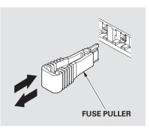
4. Check the smaller fuses in the under-hood fuse box and all the fuses in the interior fuse box by pulling out each one with the fuse puller provided on the back of the under-hood fuse box cover.
