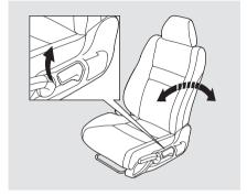
To change the seat-back angle, pull up on the lever on the outside of the seat bottom.
