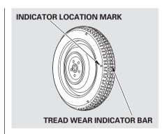
Replace the tire when you can see the tread wear indicator bars. The replacement should be the same size and design tire, mounted on the same wheel. The spare tire is not designed to be mounted on a regular wheel, and the spare wheel is not designed for mounting a regular tire.
