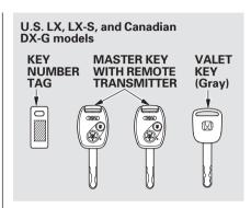
The valet key works only in the ignition and the door locks. You can keep the trunk and trunk release handle locked when you leave your vehicle and the valet key at a parking facility.
