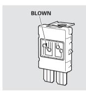
3. Check each of the large fuses in the under-hood fuse box by looking through the top at the wire inside. Removing these fuses requires a Phillips-head screwdriver.
