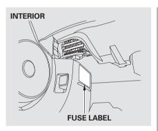
The fuses are in two fuse boxes. The interior fuse box is underneath the steering column.
