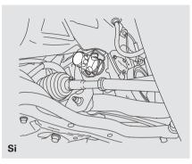
4. Install a new oil filter according to the instructions that come with it.
