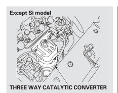
The three way catalytic converter contains precious metals that serve as catalysts, promoting chemical reactions to convert the exhaust gasses without affecting the metals. The catalytic converter is referred to as a three-way catalyst, since it acts on HC, CO, and NOx. A replacement unit must be an original Honda part or its equivalent.
