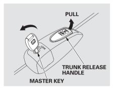
To open the trunk, pull the trunk release handle on the left side of the driver's seat. To protect items in the trunk when you need to give the key to someone else, lock the trunk release handle with the master key, and give the other person the valet key.
