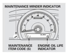
If the remaining engine oil life is 15 to 6 percent, you will see the engine oil life indicator every time you turn the ignition switch to the ON (II) position. The maintenance minder indicator will also come on, and the maintenance item code(s) for other scheduled maintenance items needing service will be displayed next to the engine oil life indicator.
