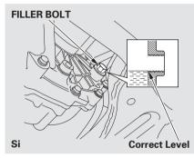
If Honda MTF is not available, you may use an SAE 10W-30 or 10W-40 viscosity motor oil with the API Certification Seal that says "FOR GASOLINE ENGINES" as a temporary replacement. However, motor oil does not contain the proper additives, and continued use can cause stiffer shifting. Replace as soon as it is convenient.
