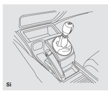
On vehicles with 6-speed manual transmission, the lockout system prevents you from shifting directly from any forward gear to reverse while the vehicle is moving at a certain speed (see page 259).
