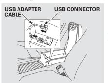
1. Pull out the USB connector from the holder and remove the cable from the clip in the console compartment.
