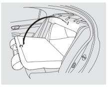
The back of the rear seat folds down, giving you direct access to the trunk. The seat-back is released from inside the trunk.
