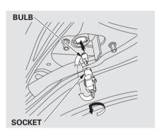
3. Remove the socket by turning it one-quarter turn counterclockwise.
