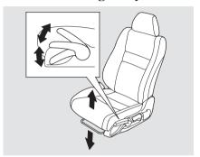
The height of your driver's seat is adjustable. To raise the seat, repeatedly pull up the lever on the outside of the seat cushion. To lower the seat, push the lever down repeatedly.
