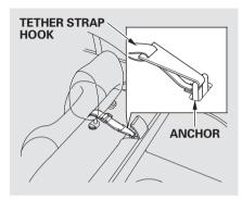
5. Lift the head restraint (see page 95), then route the tether strap through the legs of the head restraint and over the seat-back, making sure the strap is not twisted.
