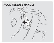
1. Park the vehicle, and set the parking brake. Pull the hood release handle under the lower left corner of the dashboard. The hood will pop up slightly.
