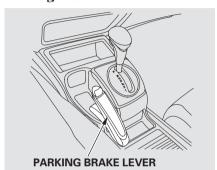
To apply the parking brake, pull the lever up fully. To release it, pull up slightly, push the button, and lower the lever. The parking brake indicator on the instrument panel should go out when the parking brake is fully released (see page 59).
