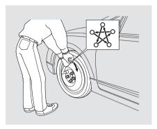
13. Tighten the wheel nuts securely in the same crisscross pattern. Have the wheel nut torque checked at the nearest automotive service facility.
