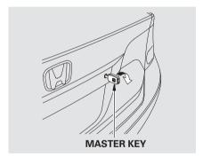
Use the master key to open the trunk lock. The valet key does not work in this lock
