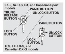
LOCK — Press this button once to lock all doors. Some exterior lights will flash once. When you push LOCK twice within 5 seconds, you will hear a horn to verify that the doors are locked. You cannot lock the doors if any door is not fully closed or the key is in the ignition switch.
