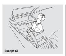
The manual transmission is synchronized in all forward gears for smooth operation. It has a lockout so you cannot shift directly from fifth to reverse.
