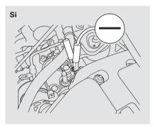
6. Start the vehicle. If the starter motor still operates slowly, check that the jumper cables have good metal-to-metal contact.
