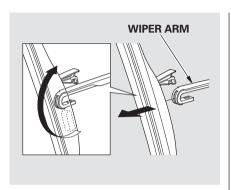
Pivot the blade assembly toward the wiper arm until it releases from the wiper arm.
