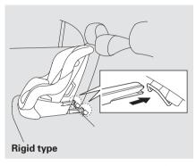
Place the child seat on the vehicle seat, then attach the seat to the lower anchors according to the child seat maker's instructions.
