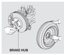
10.Before mounting the spare tire, wipe any dirt off the mounting surface of the wheel and hub with a clean cloth. Wipe the hub carefully; it may be hot from driving.
