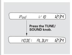
You can also select a file from any list on the iPod menu: playlists, artists, albums and songs, by using the TUNE/SOUND knob. Push the TUNE/SOUND knob to switch the display to an iPod menu, then turn the TUNE/SOUND knob to select a desired list
