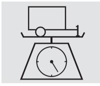
Total Trailer Weight: The maximum allowable weight of the trailer and everything in or on it must not exceed 1,000 lbs (450 kg). Towing a load that is too heavy can seriously affect your vehicle's handling and performance. It can also damage the engine and drivetrain
