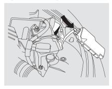
1. To change the headlight bulb on the driver's side, remove the engine coolant reserve tank by pulling it out of its holder.
