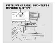
The buttons under the left side vent control the brightness of the instrument panel. Push the + or - button to adjust the brightness.
