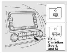
The rear window defogger will clear fog, frost, and thin ice from the window. Push the defogger button to turn it on and off. The indicator in the button comes on to show the defogger is on. If you do not turn it off, the defogger will shut itself off after about 15 minutes. It also shuts off when you turn off the ignition switch. You have to turn the defogger on again when you restart the vehicle.
