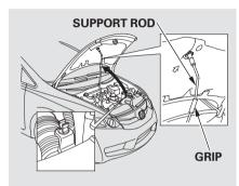
3. Pull the support rod out of its clip by holding the grip, and insert the end into the designated hole in the hood.
