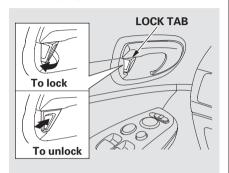
Each door has a lock tab next to the inside door handle. Pull the tab out to lock the door, and push it in to unlock the door
