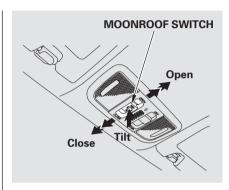
To open or close the moonroof partially, pull or push the moonroof switch lightly to the first detent and hold it. The moonroof will stop when you release the switch.
