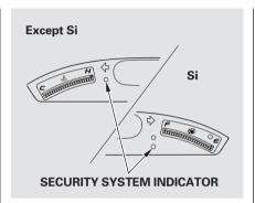
Once the security system is set, opening any door (without using the key or the remote transmitter), the hood, or the trunk will cause the alarm to activate. It will also activate if the audio unit is removed from the dashboard or the wiring is cut.
