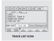
You can also select a file directly from a track list on the audio display. Press the AUDIO button to show the audio display, then touch the Track List icon. The track list menu appears on the display.
