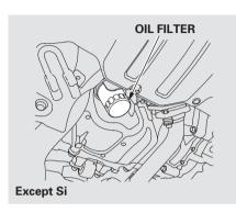
3. Remove the oil filter, and let the remaining oil drain. A special wrench (available from your dealer) is required.
