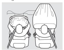
Your vehicle has a supplemental restraint system (SRS) with front airbags to help protect the heads and chests of the driver and a front seat passenger during a moderate to severe frontal collision (see page 24 for more information on how your front airbags work).
