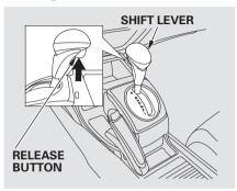
To shift from Park to any position, press the brake pedal, the release button on the front of the shift lever, then pull the lever. You cannot shift out of Park when the ignition switch is in the LOCK (0) or the ACCESSORY (I) position.
