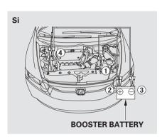
3. Connect one jumper cable to the positive (+) terminal on your battery. Connect the other end to the positive (+) terminal on the booster battery.
