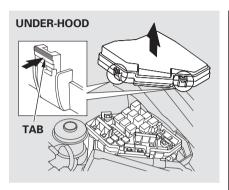
The under-hood fuse box is on the driver's side, next to the brake fluid reservoir. To open it, push the tabs as shown.
