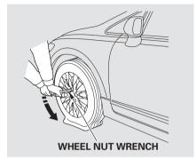
6. Loosen each wheel nut 1/2 turn with the wheel nut wrench.
