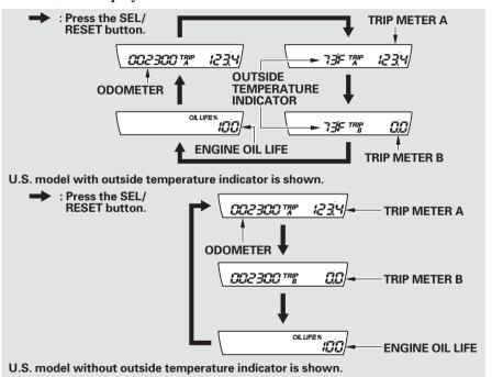
To switch the information display between the odometer, trip meter, outside temperature (if equipped), and engine oil life and maintenance item code(s), press the SEL/RESET button repeatedly.
