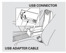
1. Pull out the USB connector from the holder and remove the cable from the clip in the console compartment.
