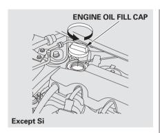
Unscrew and remove the engine oil fill cap on the valve cover. Pour the oil slowly and carefully so you do not spill any. Clean up any spills immediately. Spilled oil could damage components in the engine compartment.
