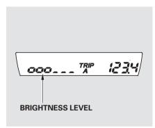
There are six brightness levels. When you push either button, the information display indicates the current level. You will hear a tone when you reach the maximum or minimum brightness. The display returns to the odometer 5 seconds after you stop adjusting the brightness.
