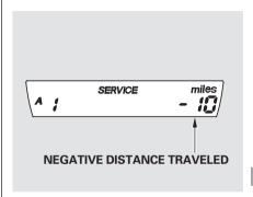
If you do not perform the indicated maintenance, negative distance traveled is displayed and begins to blink after the vehicle has been driven 10 miles (10 km) or more. Negative distance traveled means your vehicle has passed the maintenance required point. Immediately have the indicated maintenance done by your dealer.
