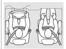
Your vehicle also has side airbags to help protect the upper torso of the driver or a front seat passenger during a moderate to severe side impact (see page 27 for more information on how your side airbags work).
