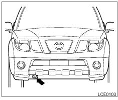
VEHICLE RECOVERY (freeing a stuck vehicle)
