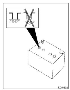
Check the fluid level in each cell If it is necessary to add fluid, add only distilled water to bring the level up to the bottom of the filler opening. Do not overfill. Vehicles operated in high temperatures or under severe conditions require frequent checks of the battery fluid level.
