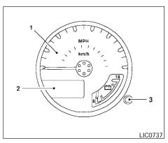
The odometer records the total distance the vehicle has been driven.
