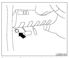
**To engage:** Firmly depress the parking brake.
