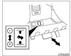
The accelerator and brake pedals can be adjusted for driving comfort.
