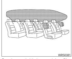
Supplemental side-impact air bag (if so equipped) and curtain side-impact and rollover air bags (if so equipped) system
