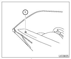
The sunload sensor (1), located on the top center of the instrument panel, helps the system maintain a constant temperature. Do not put anything on or around this sensor.
