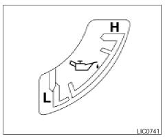
If the gauge needle does not move with the proper amount of engine oil, have the vehicle checked by a NISSAN dealer. Continued vehicle operation in such a condition could cause serious damage to the engine.
