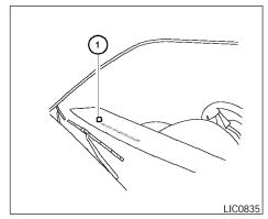
Be sure you do not put anything on top of the autolight sensor (1) located on the top side of the instrument panel. The autolight sensor controls the autolight: if it is covered, the autolight sensor reacts as if it is dark out and the headlights will illuminate. If this occurs while parked with the engine off and the key in the ON position, your vehicle's battery could become discharged.
