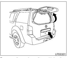
To open, pull up on the smaller outside handle to release the glass hatch, then pull up on the glass hatch. To close, lower and push the glass hatch down securely.
