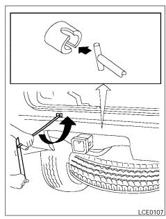
Fit the square end of the jack rod into the square hole of the wheel nut wrench to form a handle.
