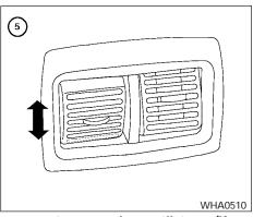
rear center console ventilators (if so equipped)
