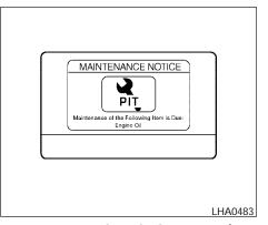
The "MAINTENANCE NOTICE" screen ("EN-GINE OIL" and "TIRE ROTATION") will be automatically displayed as shown when both of the following conditions are met:
