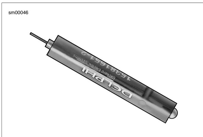
**Figure A-49. Packard Micro 64 Terminal Remover (HD-45928)**
