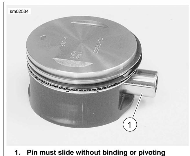
1. Pin must slide without binding or pivoting
