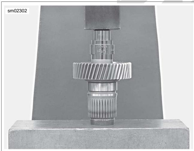
Figure 7-42. Installing Transmission Side Needle Bearing in Main Driver Gear
