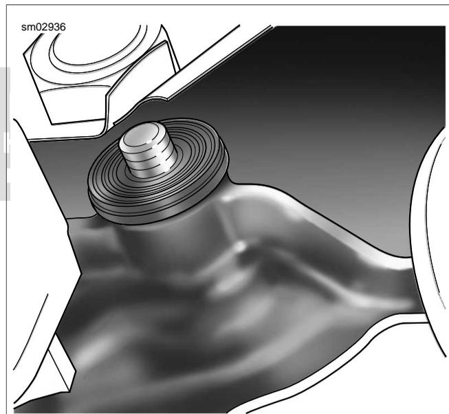
Figure 2-96. Remove Upper Bushing (Right Side)
