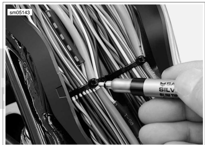
**Figure 8-98. Mark Location of Cable Straps**
