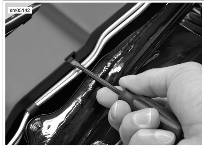
**Figure 8-97. Release Catches From Cover**
