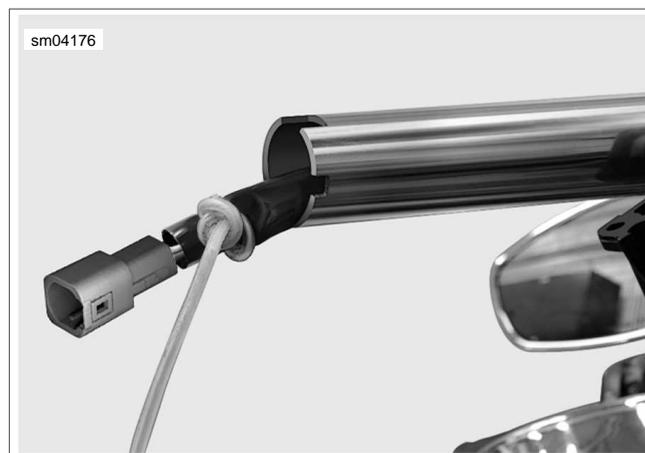
**Figure 4-23. Fix Mechanics Wire to Twist Grip Sensor Jumper Harness**
