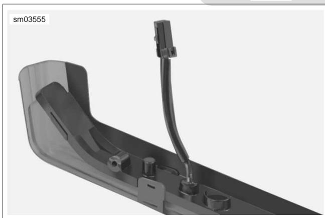
Figure 2-126. Side Marker Lights Assembly (FHLTCU)
