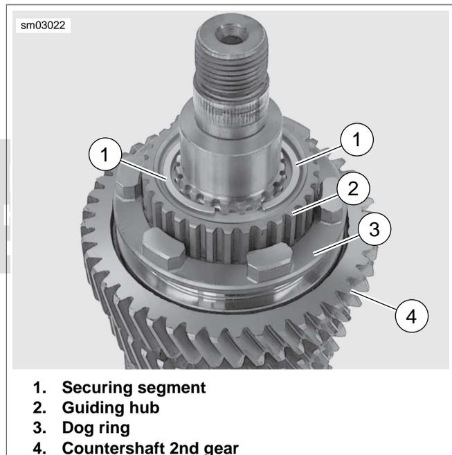
Figure 7-19. Securing Segment
