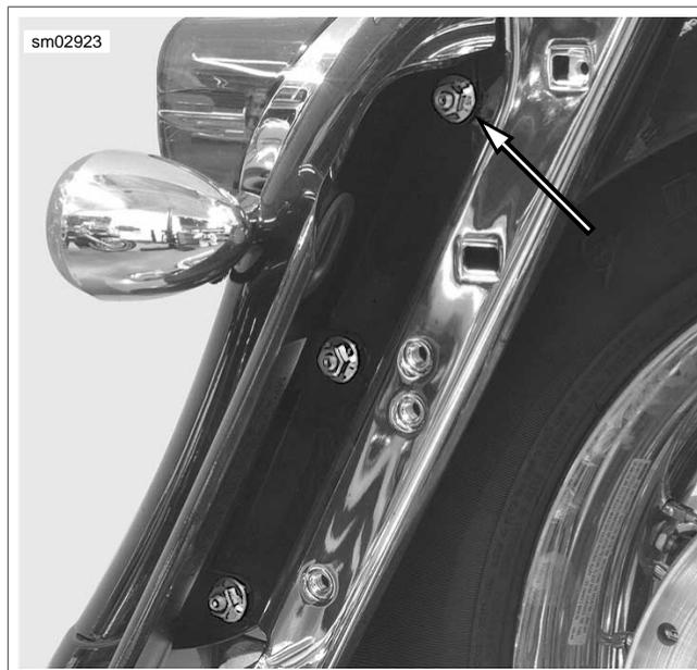
Figure 2-172. Remove Flange Nuts
