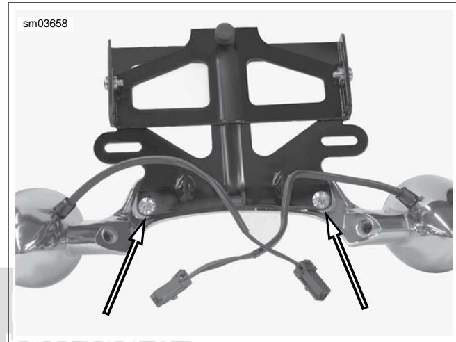
**Figure 8-57. Remove License Plate Bracket**
