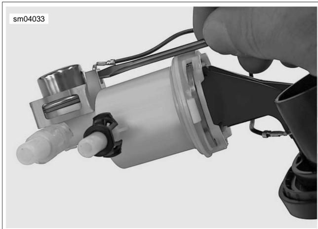
**Figure 4-13. Remove Ground Wire Spade Terminal From Fuel Filter Shell**
