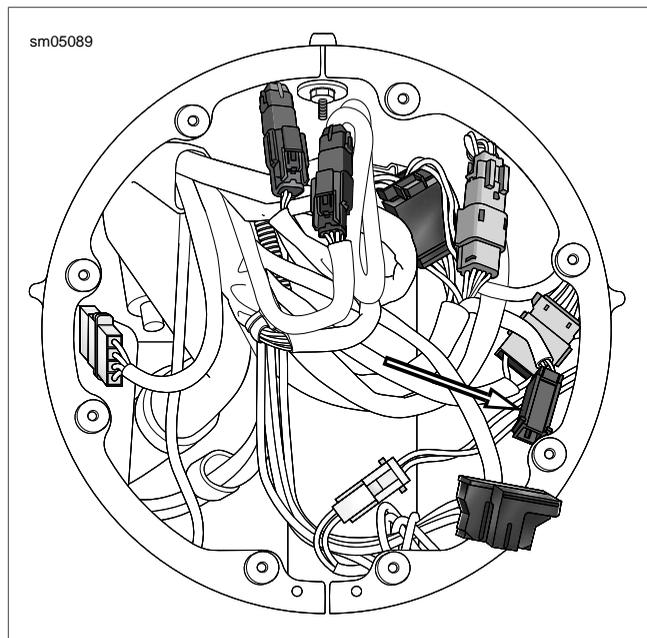
**Figure 8-36. Front Fender Tip Lamp Jumper Harness Connector (FLHR)**
