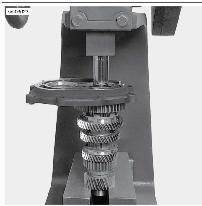
Figure 7-25. Installing Countershaft
