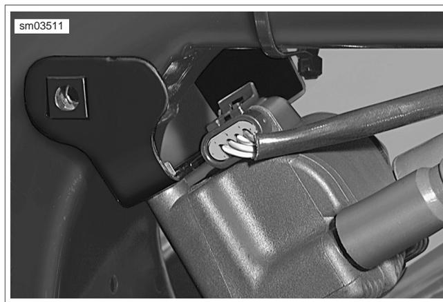
Figure 8-3. Remove Ignition Coil Bracket From Vehicle
