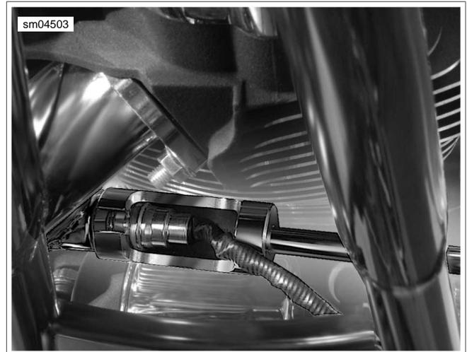
Figure 4-30. Remove/Install Front O2 Sensor
