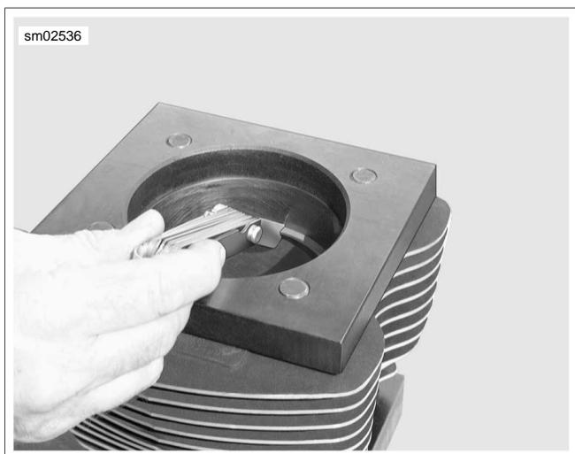
Figure 3-104. Measuring Ring Gap
