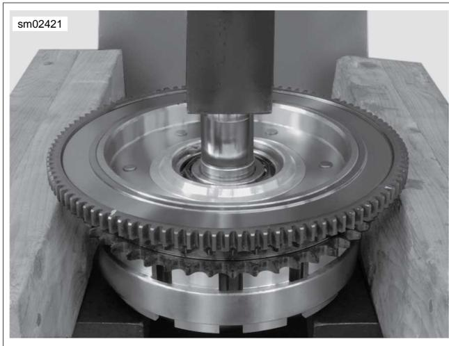
**Figure 6-33. Pressing Clutch Hub From Bearing**
