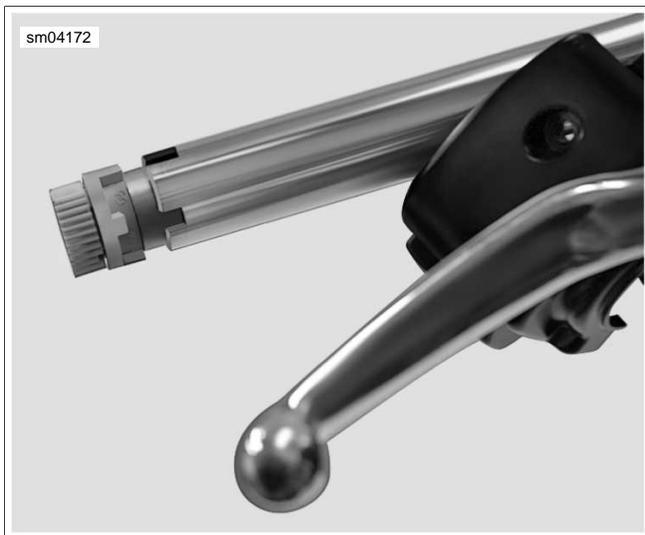
**Figure 4-22. Install Twist Grip Sensor**
