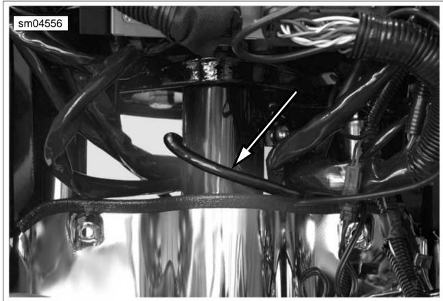
**Figure C-7. Route Brake Line to Front Calipers Above Chrome Skirt**
