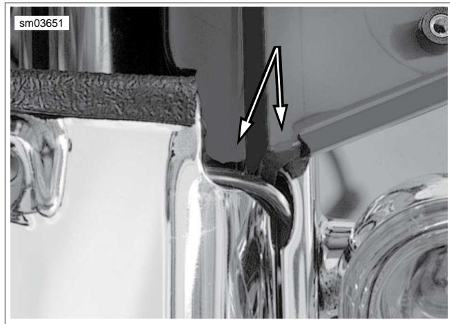
**Figure 8-51. Route Conduit Through Mounting Bracket and Chrome Skirt Reliefs (FLHX)**
