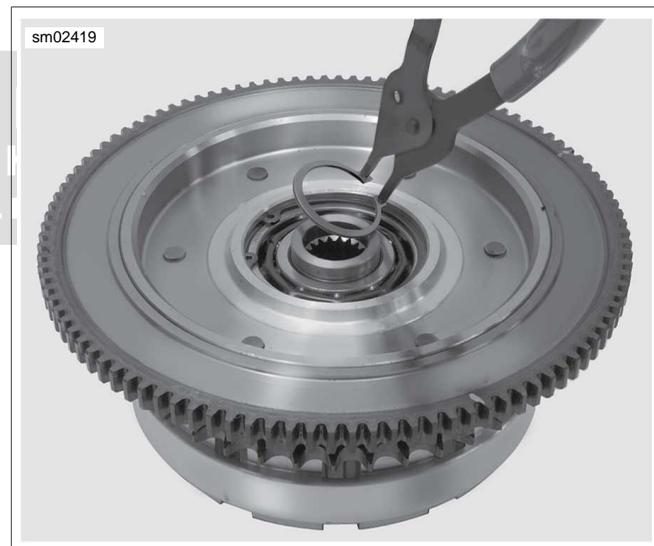
Figure 6-32. Clutch Hub Retaining Ring
