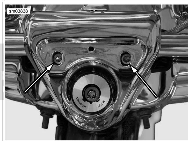
**Figure 2-93. Loosen Upper Handlebar Clamp Screws (FLHR/C)**
