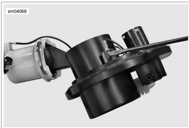
**Figure 4-8. Remove Ground Wire Spade Terminal From Top Plate**
