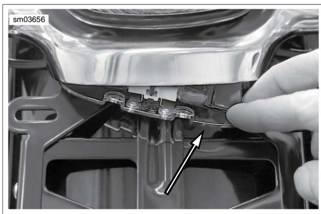
**Figure 8-55. Release Lamp Assembly**
