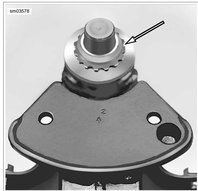
Figure 1-41. Bearing Adjuster Nut
