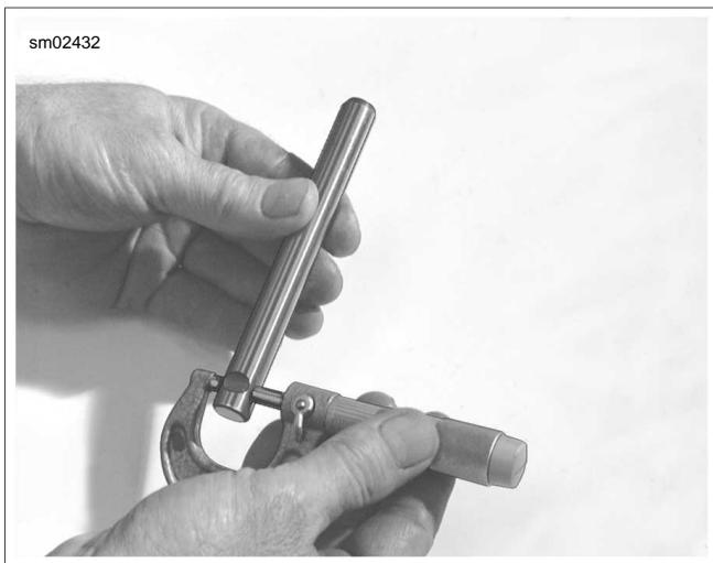
Figure 3-71. Checking Shaft to Support Plate Fit
