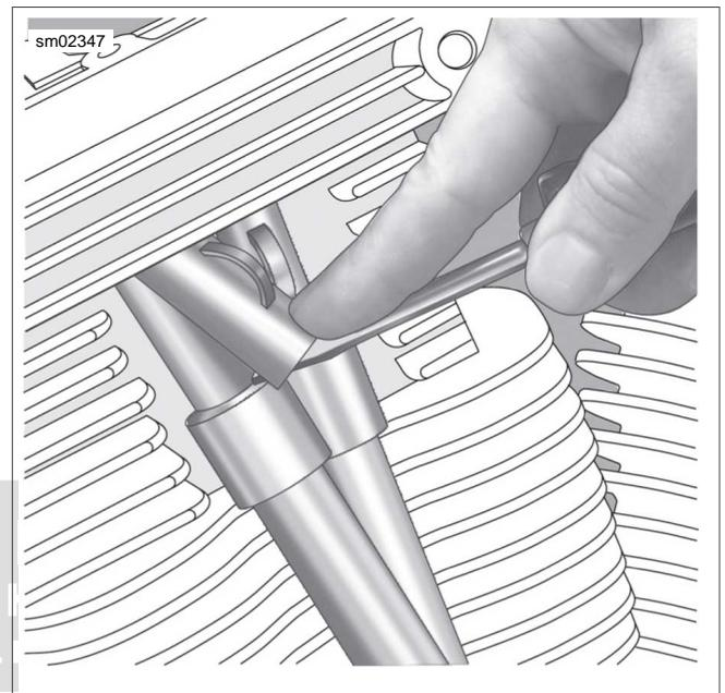
Figure 3-43. Install Spring Cap Retainers
