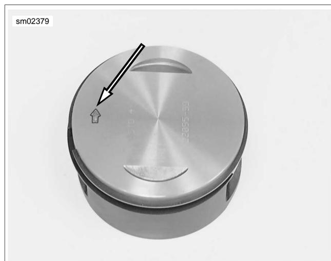
Figure 3-25. Piston Installation Arrow
