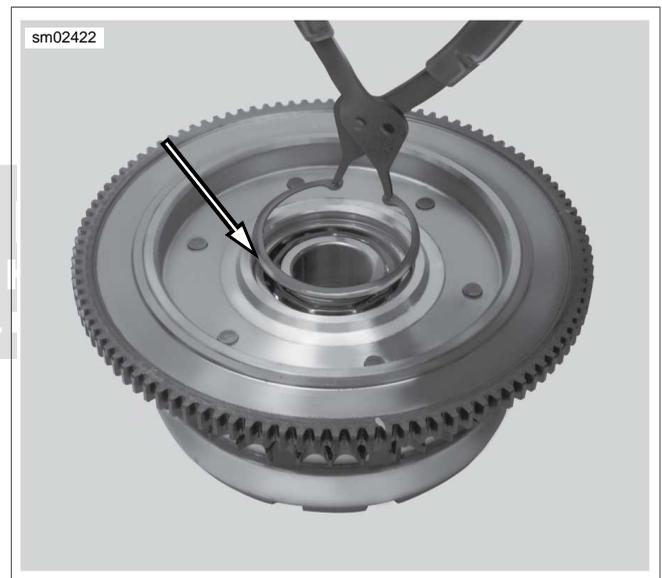
**Figure 6-34. Install Clutch Shell Retaining Ring with Flat Side Against Bearing**
