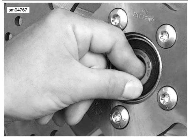
Figure 1-11. Inspect Wheel Bearings
