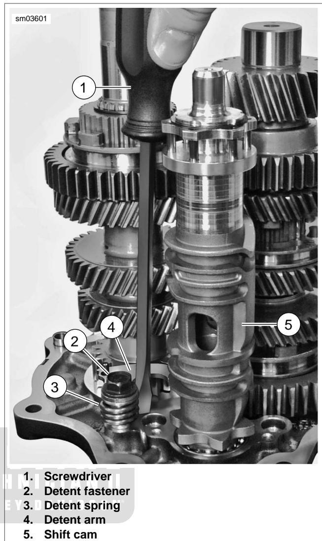
Figure 7-28. Detent Assembly
