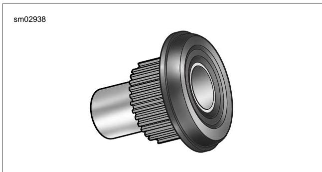
**Figure 2-98. Remove Spacer from Lower Bushing**
