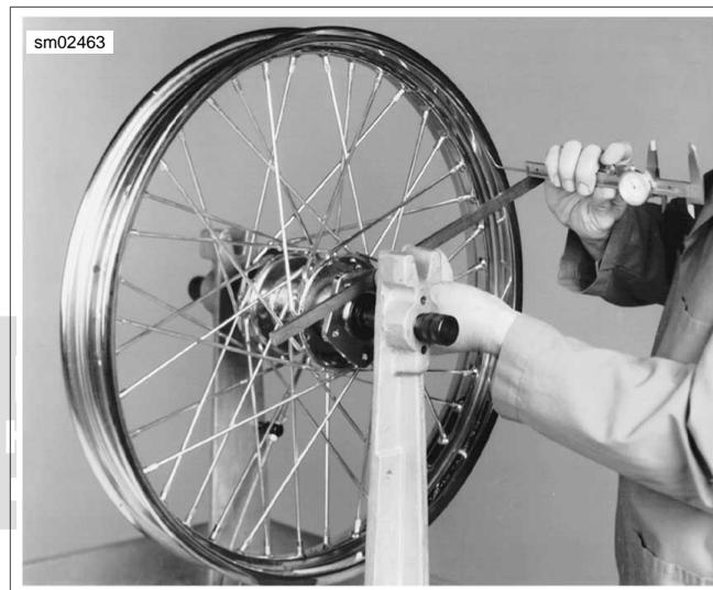
Figure 2-31. Front Wheel Hub Offset Dimension
