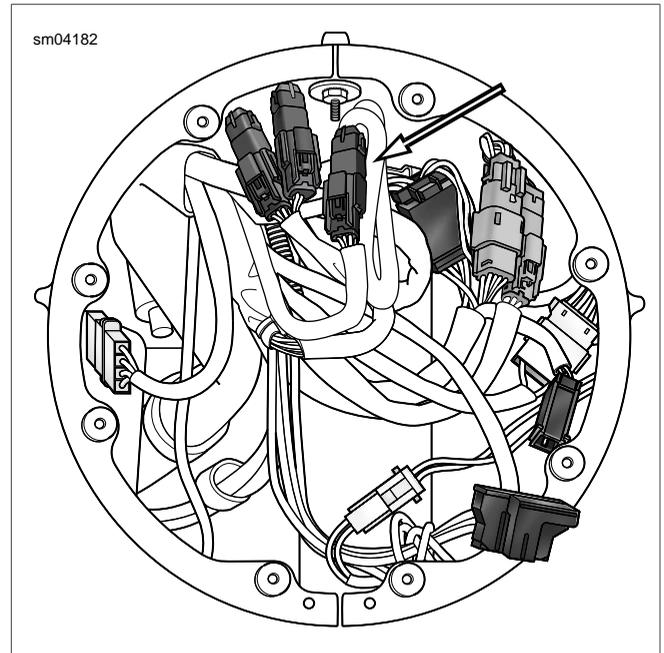
Figure 4-17. Twist Grip Sensor Jumper Harness Connector (FLHR/C)
