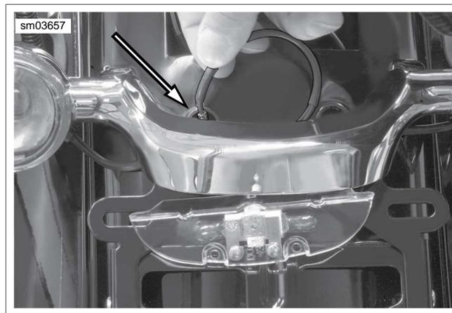
**Figure 8-56. Draw Wires Through Fender Hole**
