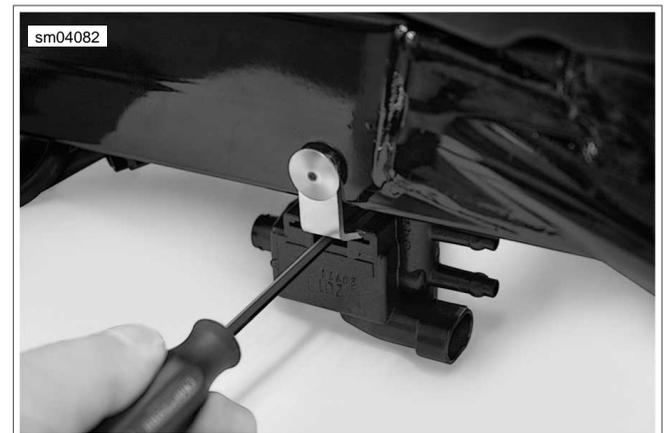
**Figure 4-52. Depress Locking Finger to Release Purge Solenoid**
