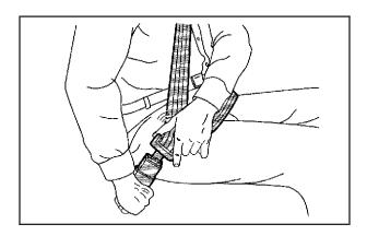
4. Push the latch plate into the buckle until it clicks. If the latch plate will not go fully into the buckle, check if the correct buckle is being used.
