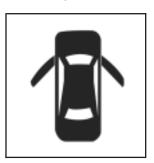
If one of the doors, trunk or liftgate is not closed properly while the ignition is on, the door ajar light on the instrument panel comes on and stays on until the doors are closed.
