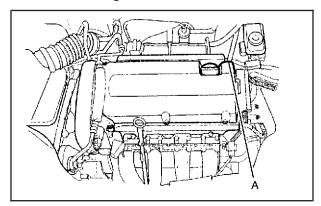
Remove the extension cord from the trunk. Open the hood and connect the electrical cord (A) with the extension cord. 3. Plug the extension cord into a normal, grounded 110-volt AC outlet.
