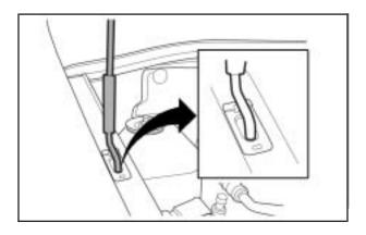
4. Securely place the hood prop into the slot on the inner fender.
