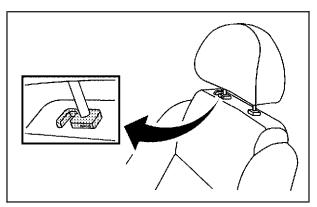
The vehicle has shopping hooks on each front seatback. Lift the headrest to access the hooks.
