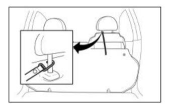
Clip the hook to the front seat head restraint to keep the rear seat secure.
