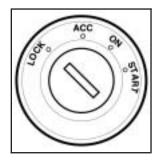
The ignition switch has four different positions.
