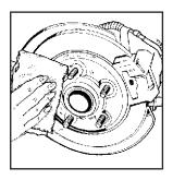
Remove any rust or dirt from the wheel bolts, mounting surfaces and spare wheel.  Place the compact spare tire on the wheel-mounting surface.
