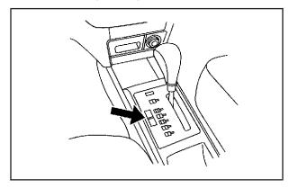
Press the HOLD button on the shift lever console to turn on hold mode. Press the button again to turn off hold mode, and return to normal automatic transmission operation. The HOLD light will light up on the instrument panel cluster. See *Hold Mode Light on page 3-30*.
