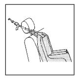
If the position you are using has a headrest or head restraint and you are using a dual tether, route the tether under the headrest or head restraint and in between the headrest or head restraint posts.
