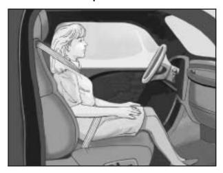
If a person of adult-size is sitting in the right front passenger seat, but the off symbol is lit, it could be because that person is not sitting properly in the seat. If this happens, use the following steps to allow the system to detect that person and enable the right front passenger frontal airbag and seat-mounted side impact airbag (if equipped):
