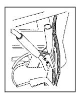
negative (–) terminal of the good battery. Use a remote negative (–) terminal if the vehicle has one. Do not let the other end touch anything until the next step. The other end of the negative (–) cable does not go to the dead battery. It goes to a heavy, unpainted metal engine part or to a remote negative (–) terminal on the vehicle with the dead battery.
