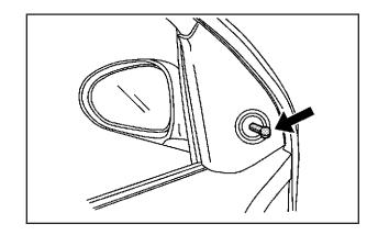
Controls for the outside manual mirrors are located next to each mirror.
