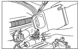
3. Fill the coolant surge tank with the proper mixture to the Maximum mark on the coolant surge tank. Wait about five minutes, then check to see if the level is below the mark. If the level is below the Maximum mark, add additional coolant to bring the level up to the mark.
