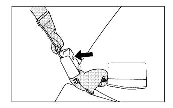
Detach the center safety belt from the mini buckle by inserting the key into the slot in the mini buckle, pressing the release button, and allowing it to retract.
