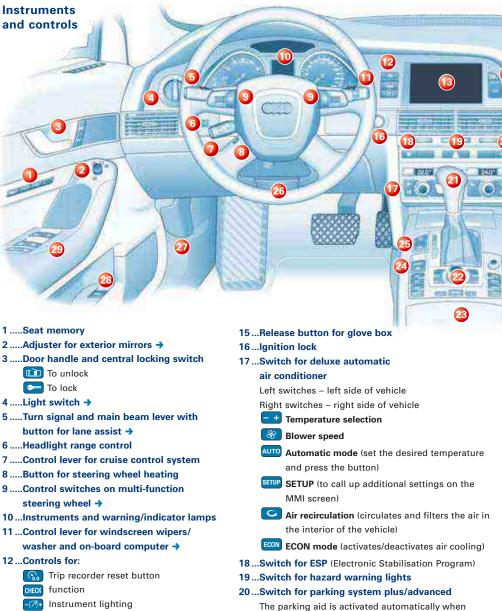
reverse gear is engaged. Press this button to activate the system when moving forwards.
