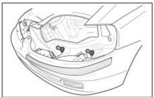
Turn the front turn signal bulb socket counterclockwise.
