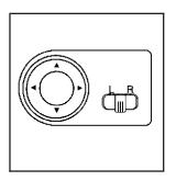
For sedan models, the control for the power mirrors is located on the instrument panel, left of the steering wheel.
