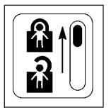
Your vehicle has rear door security locks on each rear door that help prevent passengers from opening the rear doors on your vehicle from the inside.
