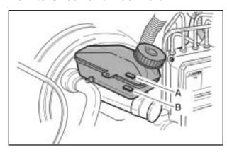
To check the fluid level, look on the side of the reservoir. If the fluid reaches the MAX (A) mark on the reservoir, the fluid level is correct. If the fluid does not reach the MIN (B) mark on the reservoir, then fluid needs to be added. The reservoir is located near the back of the engine compartment on the driver's side of the vehicle. See *Engine Compartment Overview on page 276* for more information on location.
