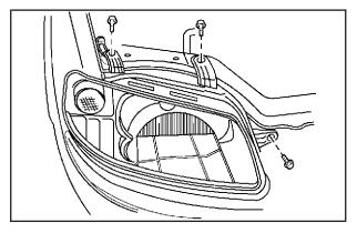
4. Remove the three bolts from the headlamp assembly.
