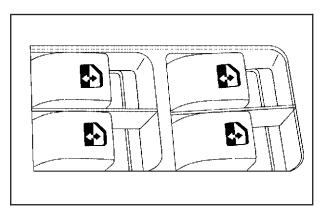
If your vehicle has power windows, the switches are located on the driver's door. In addition, each passenger door has a switch for its own window.
