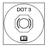
Your vehicle has one reservoir for both the brake and clutch hydraulic systems. It is filled with DOT-3 brake fluid. See *Engine Compartment Overview on page 276* for the location of the reservoir.
