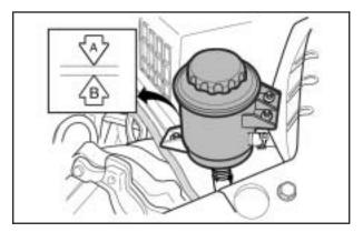
The level should be between the MIN (B) and MAX (A) marks on the reservoir. If the level drops below the MIN (B) mark, add power steering fluid. Do not overfill the reservoir and remember to replace the cap tightly when you are finished and clean up any spilled fluid.
