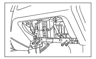
3. For hatchback models remove the four screws on the knee bolster and remove the knee bolster.
