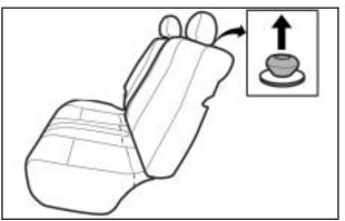
Pull up the release knob, located on the top of the seatback, and fold the seatback forward and down. Notice: Folding a rear seat with the safety belts still fastened may cause damage to the seat or the safety belts. Always unbuckle the safety belts and return them to their normal stowed position before folding a rear seat.
