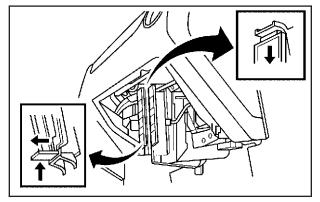
4. Then reverse the steps to install the new air filter and replace the glove box.
