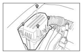
The engine air cleaner/filter is located in the engine compartment on the passenger's side of the vehicle. See *Engine Compartment Overview on page 276* for more information on location.
