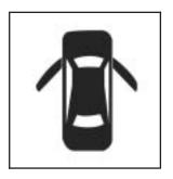
If one of the doors on the sedan is not closed properly while the ignition is on, the door ajar light on the instrument panel comes on and stays on until the doors are closed.
