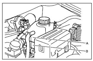
The engine coolant surge tank is located in the rear of the engine compartment on the driver's side of the vehicle. See *Engine Compartment Overview on page 276* for more information on location.
