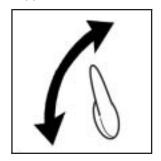
To adjust the front seat lumbar support, use the lever located on the outboard side of the seatback.
