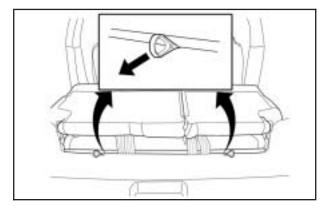
Pull the release handles on the rear side of the seat cushion to unlock the seat cushion. 6. Lift the seat cushion up and flip it forward.
