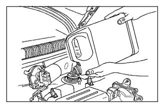
3. Fill the coolant surge tank with the proper mixture to the Maximum mark on the coolant surge tank. Wait about five minutes, then check to see if the level is below the mark. If the level is below the Maximum mark, add additional coolant to bring the level up to the mark. Repeat this procedure until the level remains constant at the Maximum mark for at least five minutes.
