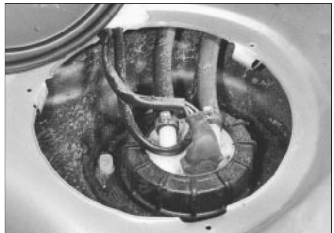
18.2 Fuel tank sender unit and connections
