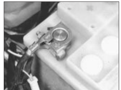
4.2 Battery positive terminal connection
