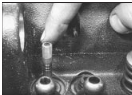
34.3 Locate plastic sleeve on valve stem . . .
