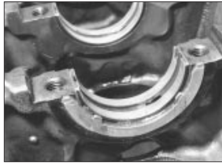
29.3 Thrustwasher location on centre main bearing
