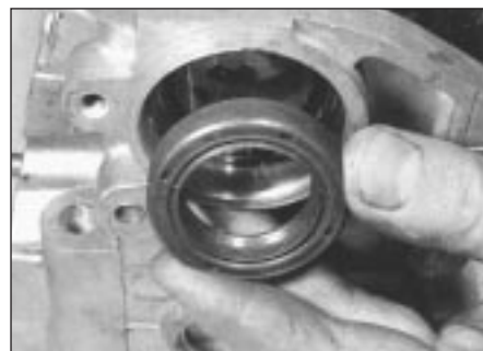
10.15 Removing camshaft oil seal
