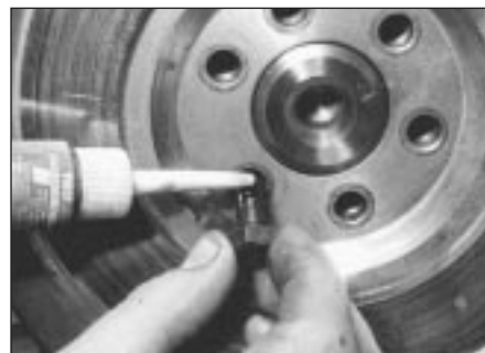
33.3 Applying liquid locking fluid to flywheel bolts
