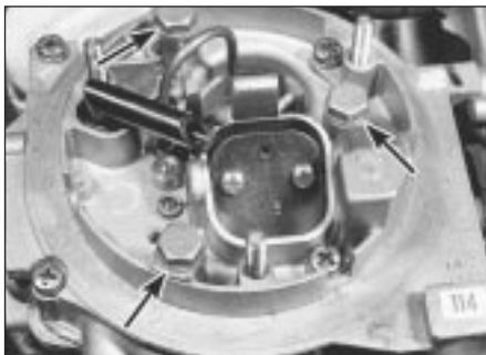
13.8 Carburettor securing bolts (arrowed) - Pierburg/Solex 2E3
