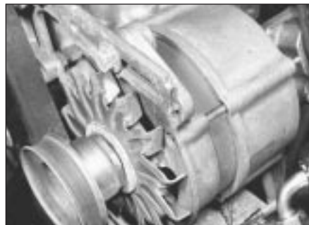
13.4b Alternator drivebelt tensioner link - 1.8 litre
