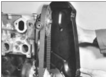
9.4 Removing timing cover
