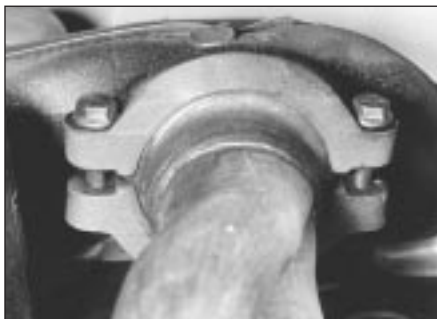
19.10 Exhaust downpipe-to-manifold flange connection - 1.3 litre
