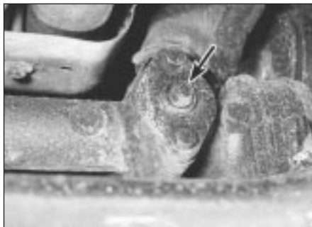
16.1 Manual steering gear adjustment screw (arrowed)
