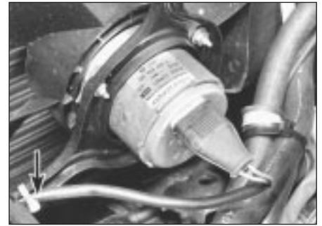
3.15 Secure fan lead with plastic clip (arrowed)
