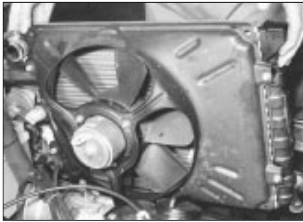
3.8 Lifting out radiator and cooling fan assembly
