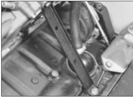
19.5 Inlet manifold support stay - 1.3 litre
