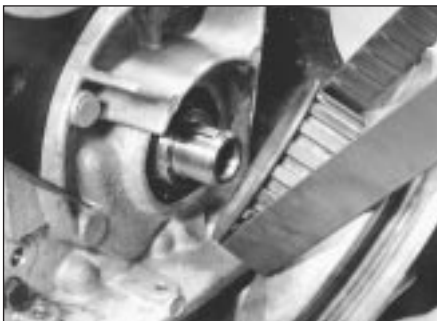
36.9 Fitting crankshaft sprocket and timing belt
