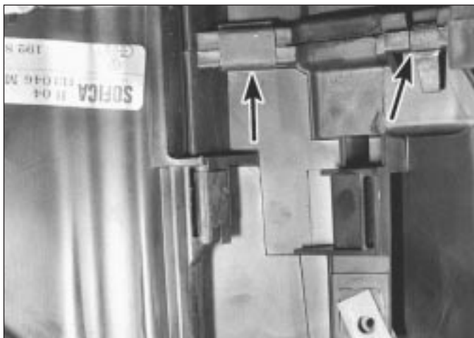
10.10 Upper-to-lower housing retaining clips (arrowed)
