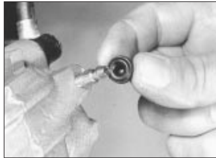
12.23 Fit bleed valve the protector cap
