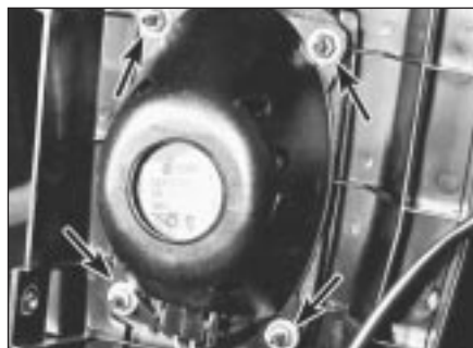
32.5 Luggage compartment loudspeaker retaining nuts (arrowed)
