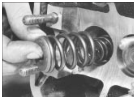
12.12b Locating valve springs and cap . . .
