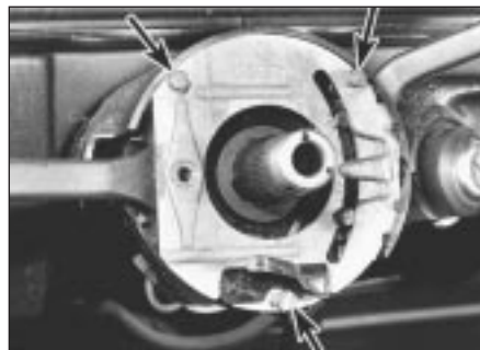
12.4 Combination switch retaining screws (arrowed)
