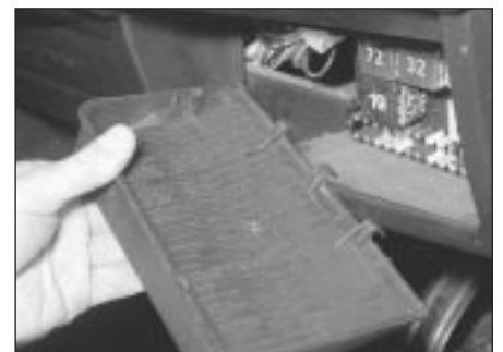
3.1 Removing fuse/relay unit cover
