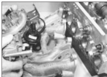
11.2b Fitting inlet manifold complete with carburettor
