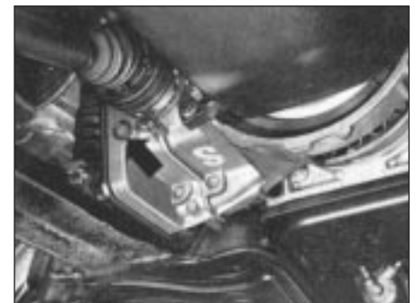
35.10 Final drive unit oil filler/level plug (arrowed)
