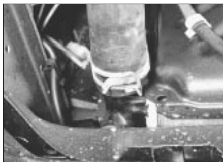
2.4a Radiator bottom hose connection - 1.3 litre
