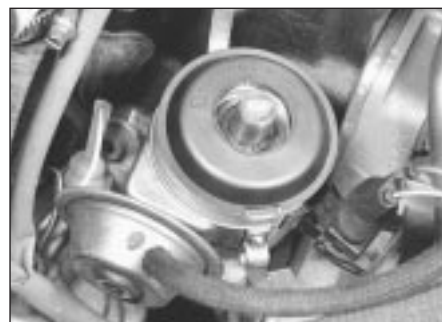
7.3b ... and lift off the dust cap
