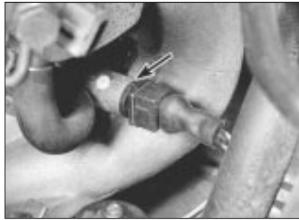
10.3 Auxiliary air valve (arrowed)
