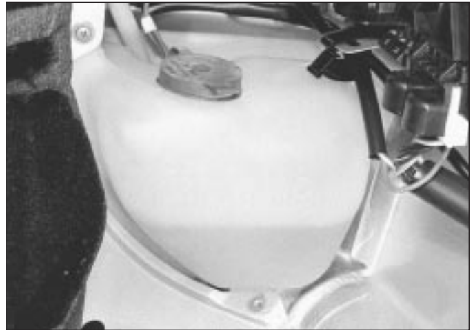
30.2 Rear window washer reservoir unit location
