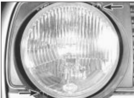
27.3 Turn adjustment screws (arrowed) to adjust headlamp beam alignment
