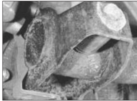
8.6 Rear suspension strut bottom mounting
