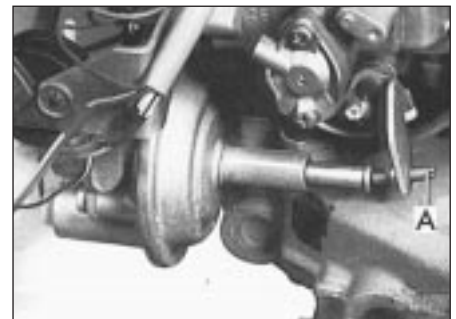
17.39b Fast idle adjustment screw (A)
