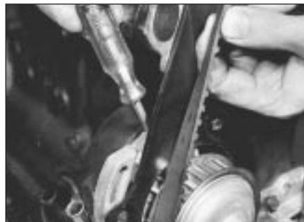
36.13 Tensioning timing belt
