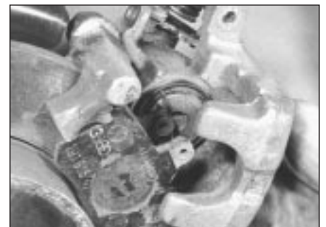
2.17 Rear brake caliper removal
