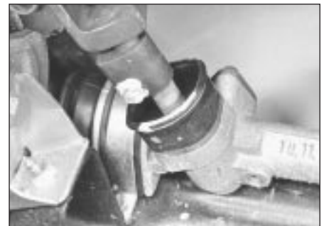
17.6 Steering gear pinion-to-lower column joint
