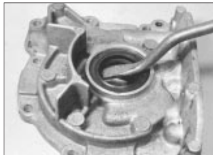
31.1 Prising out oil pump oil seal
