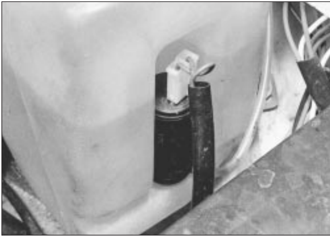
30.1 Windscreen washer pump and wire connector
