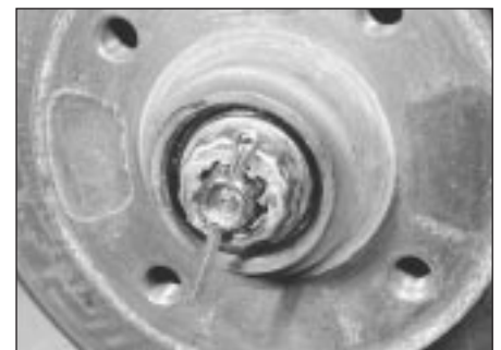
4.14 . . . remove the split pin and locking ring . . .
