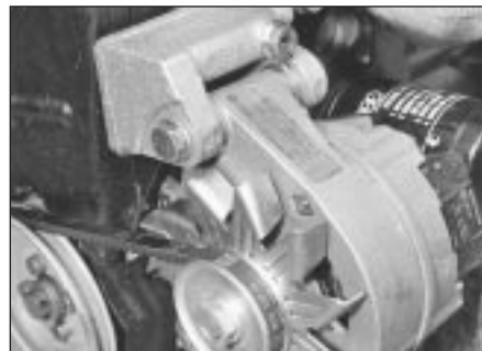
7.3 Alternator pivot bolt and bracket - 1.3 litre
