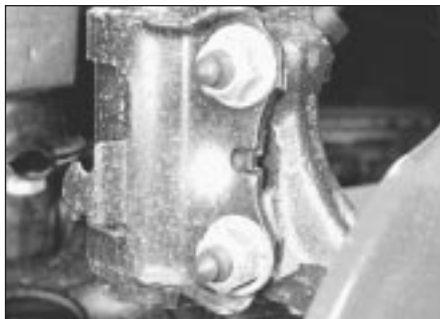
2.7 Strut-to-front wheel bearing housing retaining nuts/bolts
