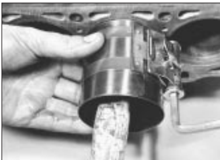
30.4 Using a piston ring compressor
