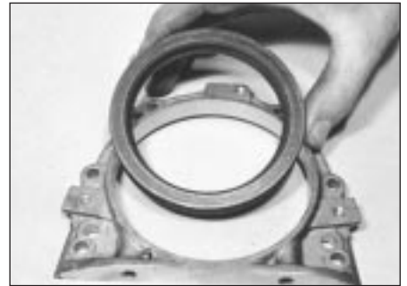
14.14 Remove crankshaft rear oil seal from housing
