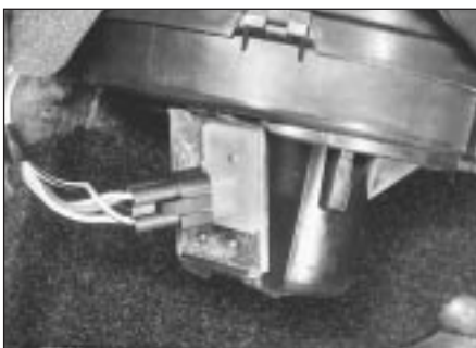
9.3 Blower unit and wiring connection
