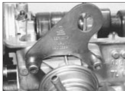
11.7b Location of engine lifting eye
