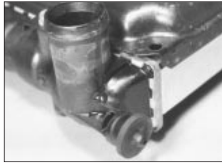
3.13 Radiator lower mounting rubber
