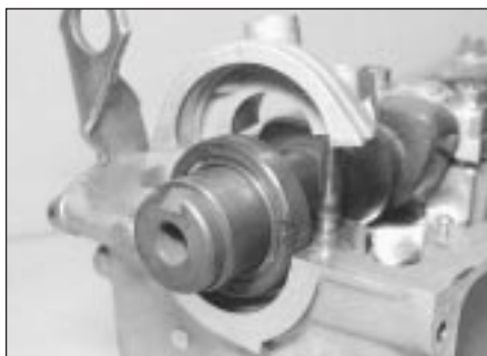
10.3 Camshaft oil seal
