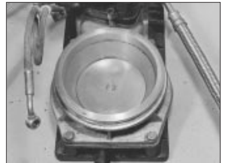
14.2 Top view of airflow sensor plate
