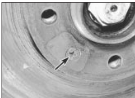
4.5 Front brake disc retaining screw (arrowed)
