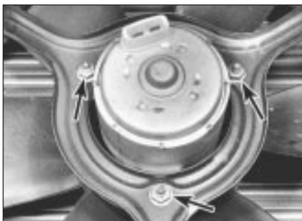
4.4 Cooling fan motor retaining nuts (arrowed)
