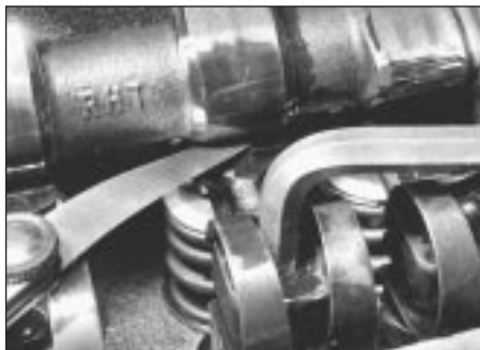
12.4 Adjusting a valve clearance - 1.05 and 1.3 litre
