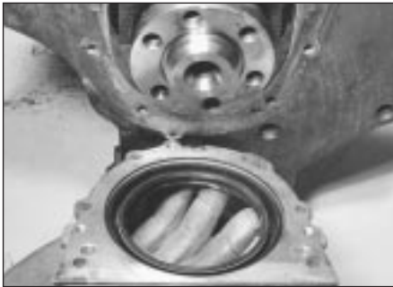
14.13a Withdrawing crankshaft rear oil seal housing . . .
