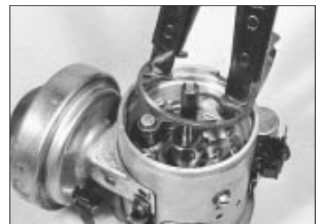
7.10b Removing bearing plate retaining ring
