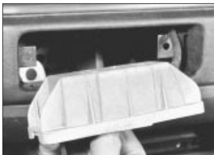
8.6 Front indicator lamp unit removal
