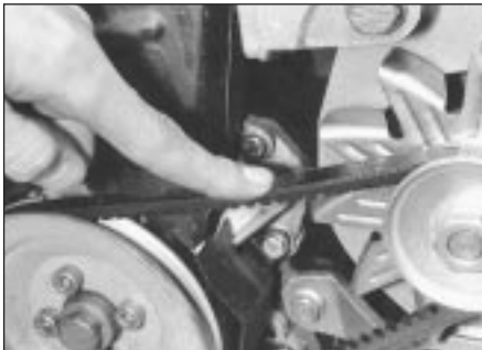
13.2 Checking alternator drivebelt tension
