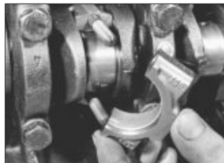
17.7 Withdrawing a big-end cap
