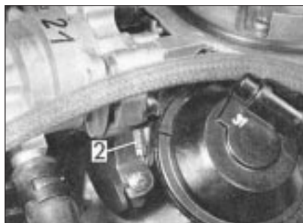
16.10 Fast idle speed adjustment screw (2)
