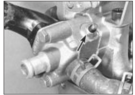
7.12 Temperature sensor (arrowed) - 1.05 and 1.3 litre
