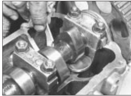
12.12 Removing a tappet bucket shim - 1.6 and 1.8 litre
