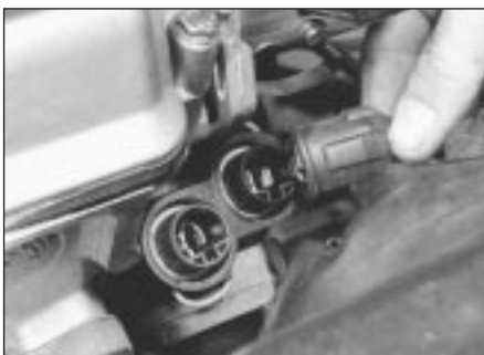
11.23b Coolant temperature switch/sender electrical connection
