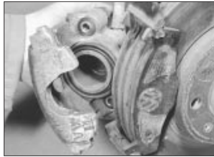
2.3b Removing the caliper
