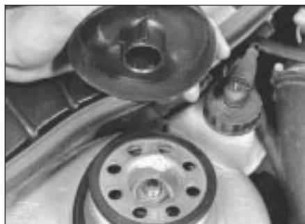
2.3 Removing front suspension strut top cap
