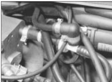
23.5 Vacuum hose-to-cylinder connector
