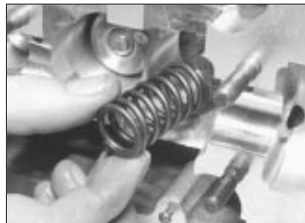
5.11b Removing an inner valve spring
