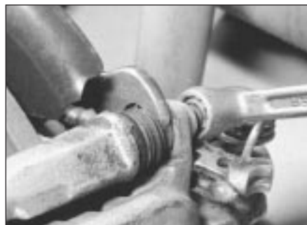
2.16 Rear caliper bolt removal
