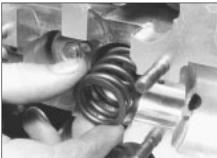
5.11a Removing an outer valve spring
