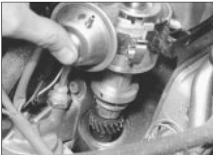
6.6a Distributor removal - 1.8 litre engine
