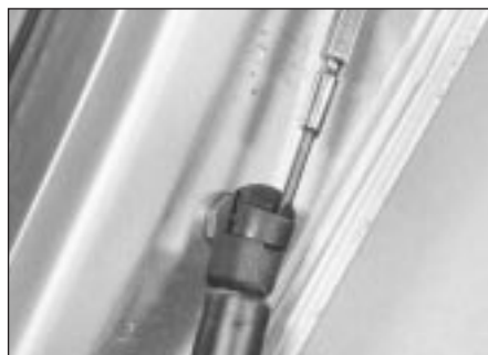
9.2a Releasing tailgate strut balljoint clip
