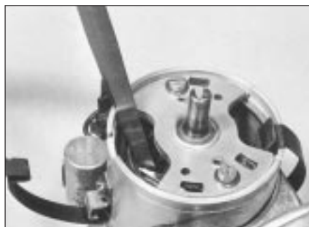
16.10a Checking contact breaker points gap
