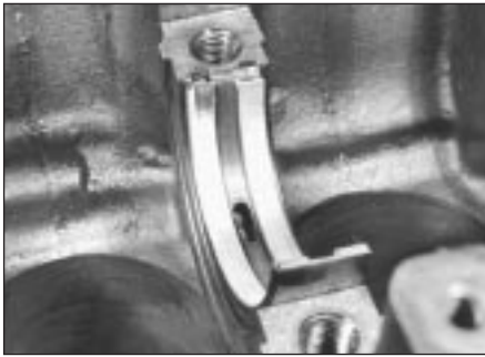
29.2 Fitting centre main bearing shell
