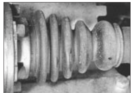
24.2 Inspect condition of each CV joint boot
