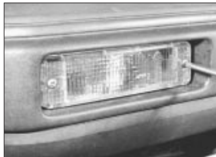
8.4 Front indicator lens removal
