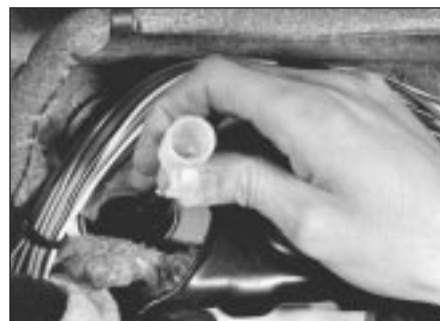
16.4 Disconnect speedometer cable
