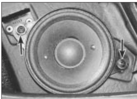
32.3 Facia-mounted loudspeaker retaining screws (arrowed)
