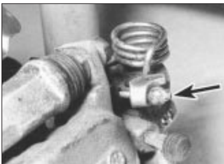
2.15 Release handbrake cable (arrowed) from caliper
