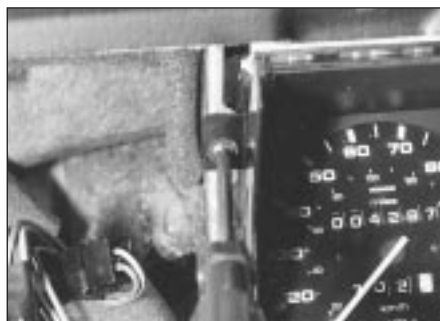
16.3 Instrument panel screw removal
