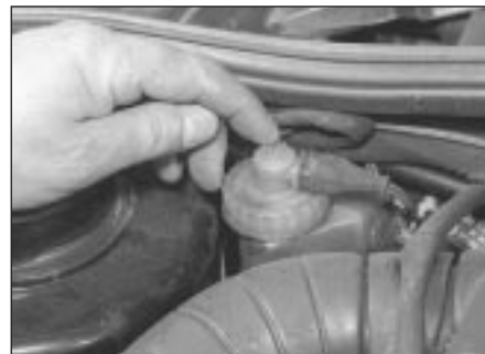
5.4 Check brake fluid level warning device
