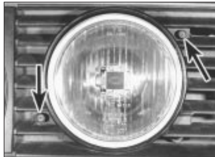
7.4 Foglight beam alignment adjuster screws (arrowed)
