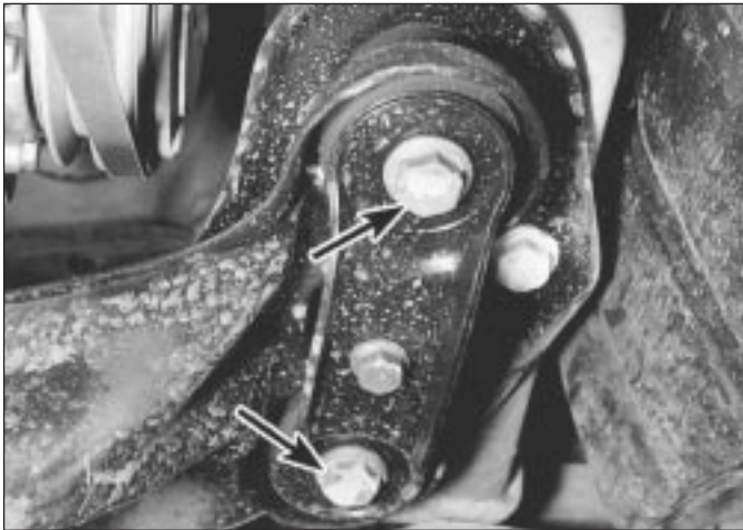
22.4 Front bumper bracket securing points to longitudinal member (arrowed)
