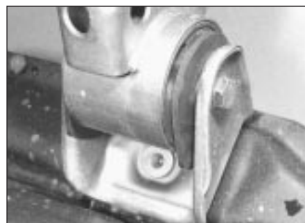
5.25a Engine/gearbox unit front mounting
