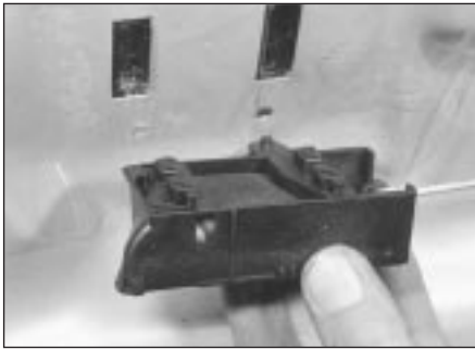
15.3 Removing interior door handle and finger plate
