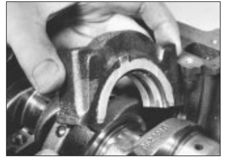
29.4 Fitting centre main bearing cap
