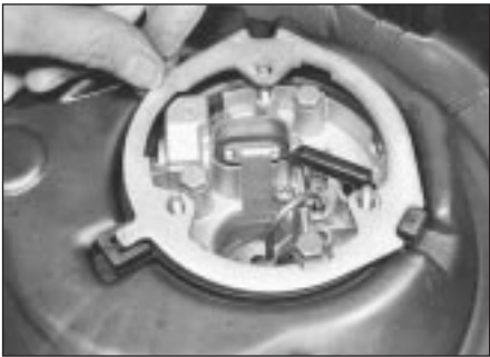
3.2 Removing air cleaner body retaining ring - 1.3 litre
