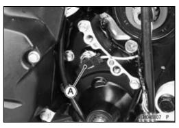
Support the engine using a suitable stand or jack [A].
