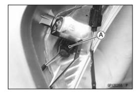
Remove the bulb [A] from the socket [B].
