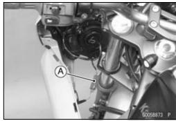
• Remove the quick rivets [A] from the lower fairings.
