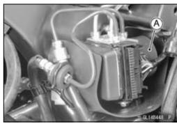
ABS Solenoid Valve Relay Fuse 15 A [A] ABS Motor Relay Fuse 25 A [B]
