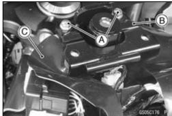
• Remove the bolts [A] and move the bracket [B] aside.
