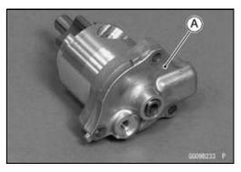
Remove: Inner Rotor [A] for Scavenge Pump Outer Rotor [B] for Scavenge Pump
