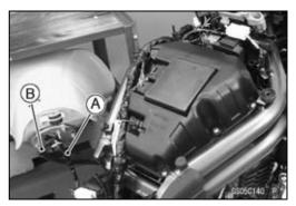
★If any one vacuum is not within the specification, turn in the bypass screws until it seats fully but not tightly.
