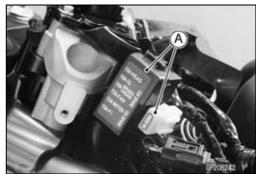
Pull out the fuses [A] straight out of the fuse box with needle nose pliers.
