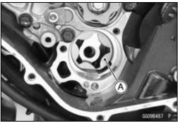
• Remove the oil pump cover [A].
