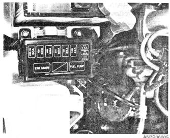
If the 80A "MAIN" fuse is blown, it must be removed as follows:
