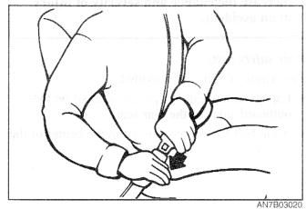
3. Insert the tongue plate into the open end of the buckle until an audible "click" is heard, indicating the belt is locked in the buckle.
