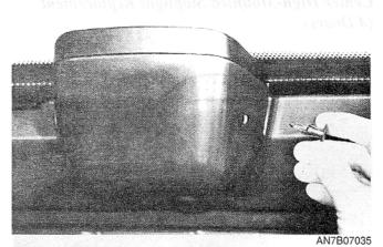
Pull out the retaining clips and remove the cover.
