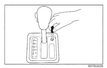
2. Insert the ignition key into the access hole and press down on the key.
