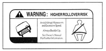
To remind you of the danger of the rollover, the rollover warning label is adhered to the driver's sunvisor. If you close the driver's sunvisor, you can see the rollover warning label which is located on the above the air bag warning label.
