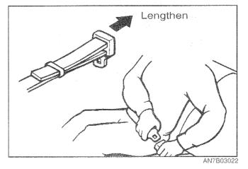
Grasp the free portion of the belt webbing and pull until the belt is snug over the hips and lower abdomen. If it becomes necessary to lengthen or shorten the belt, hold the latch plate tongue at right angles to the webbing and pull.
