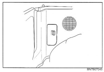
1. Pull out on the finger slots to remove the rear light cover.
