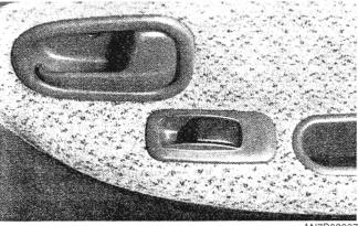
To open a window, press down on the front portion of the power window switch. To close a window, pull up on the front portion of the power window switch.
