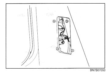
2. Disconnect the electrical connector by pressing on the locking tab while pulling on the connector.
