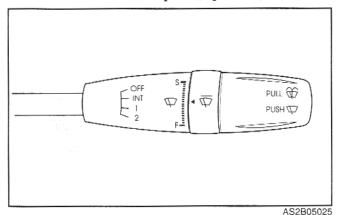
Set the lever to the INT position and choose the desired wiper interval by turning the ring.
