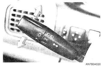
The ignition switch must be on for the turn signals to function. To turn on the turn signals, move the lever up or down. Green arrow indicators on the instrument panel indicate which turn signal is operating. They will self-cancel after a turn is completed. If the indicator continues to flash after a turn, manually return the lever to the OFF (middle) position.
