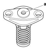
b. While lightly pressing the timing chain tensioner rod by hand, turn the timing chain tensioner rod fully counterclockwise with a hexagon wrench "1".
