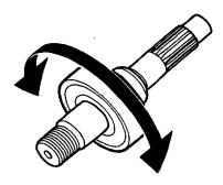
Remove the bearing using the special tool and press.
