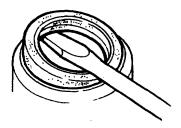
2. Drive the oil seal into the secondary gear shaft, using the special tools as shown.
