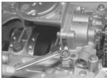
12.40a Unscrew oil pump retaining bolts . . .
