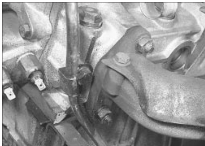
8.6b Dipstick guide tube support bracket
