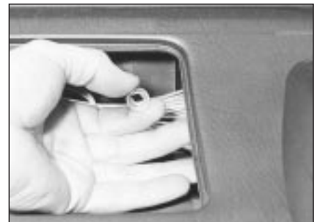
7.16b . . . to remove an instrument panel retaining nut
