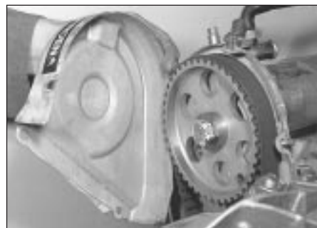
6.3 Camshaft timing sprocket cover removal
