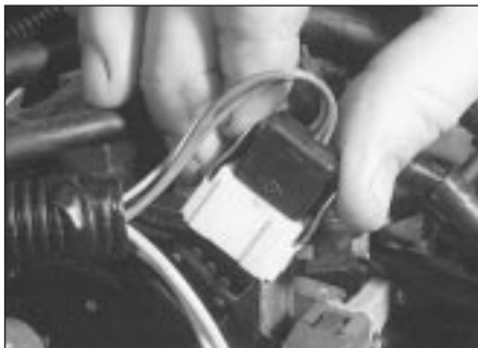
12.2a Disconnect wiring connectors from throttle potentiometer . . .
