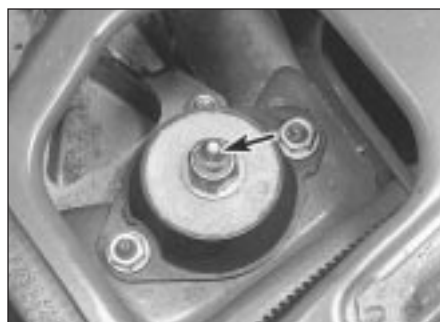
8.30a Left-hand engine mounting through-bolt (arrowed)
