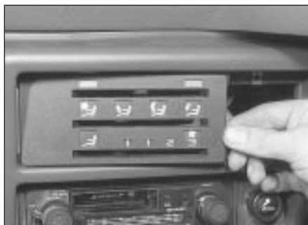
11.8 Heater/ventilation control plate removal
