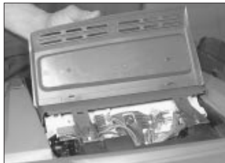
7.2 Instrument panel inspection cover removal
