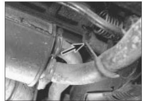
26.3 Exhaust system flexible hanger (arrowed)
