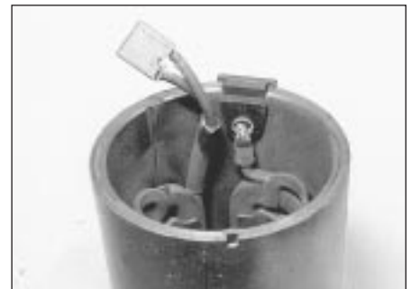
10.7 Brush connections to field coil
