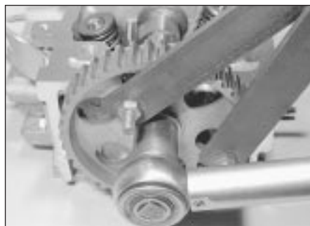
14.1a Using home-made tool to hold camshaft sprocket stationary
