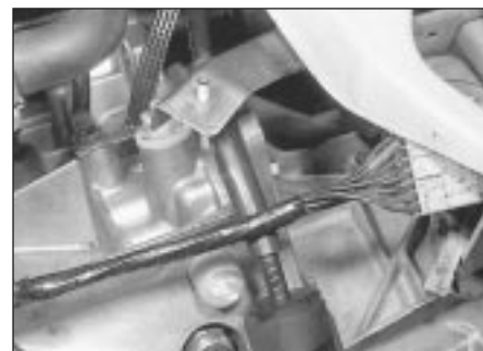
9.9 Air cleaner support bracket
