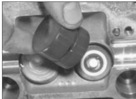
12.4 Removing a hydraulic tappet
