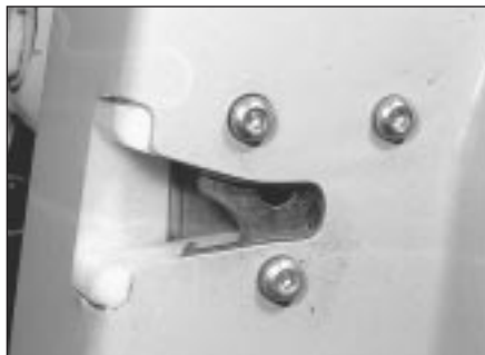
17.2 Door lock retaining screws and nylon grommet
