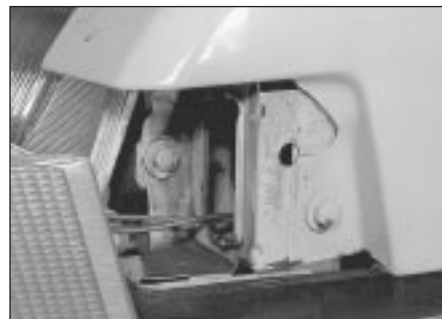
3.13 Withdraw the front indicator unit . . .
