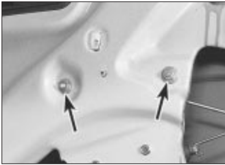
14.2 Door glass runner channel retaining nuts (arrowed)
