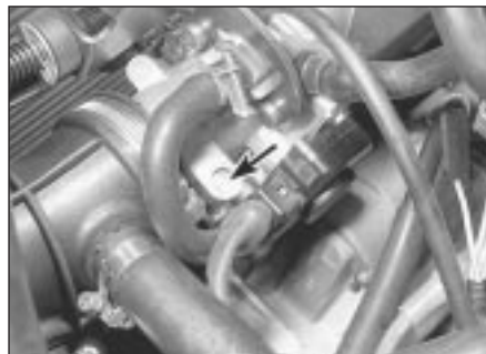
23.9 Idle speed adjustment screw (arrowed) - Bosch LE3 Jetronic
