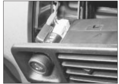
14.8 Withdrawing the grille panel
