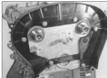
6.34a Timing belt rear cover correctly refitted
