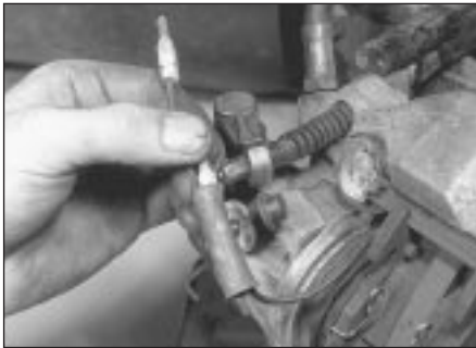
2.4a Disconnect the pad wear warning leads . . .
