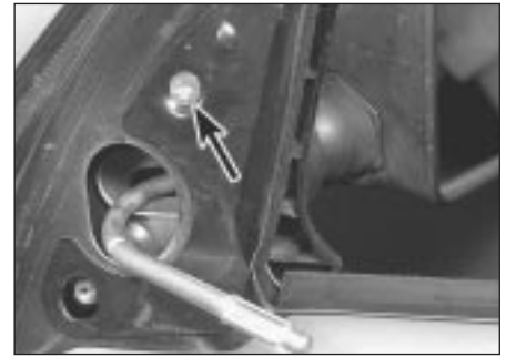
10.3 Countersunk screw retaining the inner plate (arrowed)
