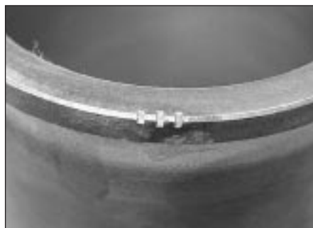
17.4 Piston/liner grading mark
