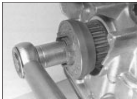
18.28 Tightening crankshaft sprocket bolt
