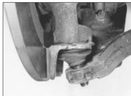
3.10 Separate swivel balljoint from suspension arm
