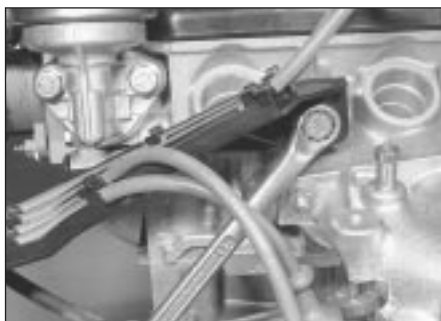
7.6 Unbolting HT lead support
