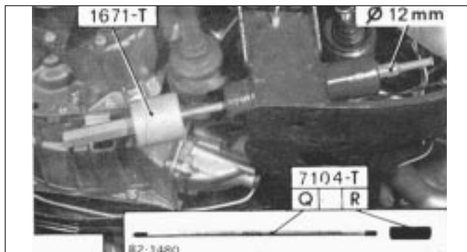
4.4 Citroën special tools in position to remove front bearing track
