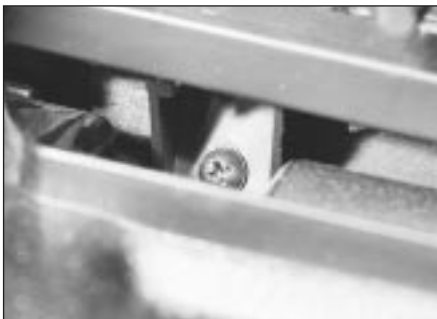
7.15 Instrument panel lower retaining screw
