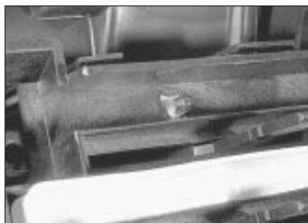
4.14 Heater control panel bulb (arrowed)
