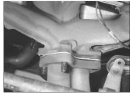
25.3b Exhaust manifold-to-downpipe connection - BX 16
