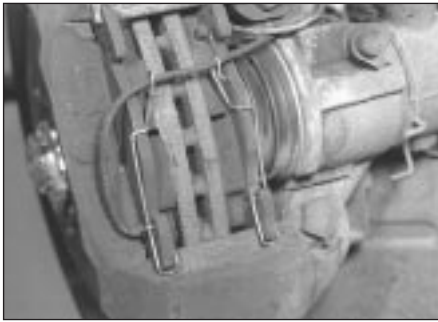
3.0a Ventilated type brake disc
