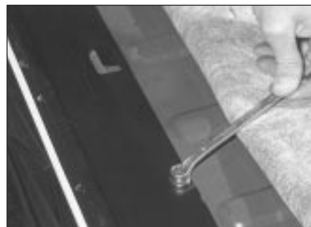
26.4 Unscrewing rear seat back hinge bolt
