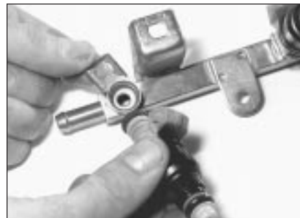
11.1 Removing a fuel injector from the rail
