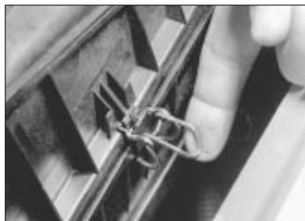
28.18a Release the five retaining clips . . .
