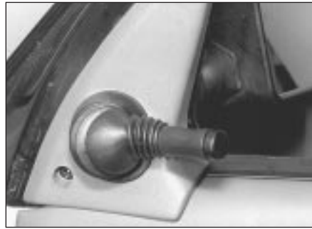
10.1 Door mirror adjuster knob and gaiter
