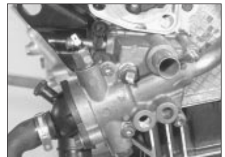
8.1a Thermostat housing in position - BX 19 GTi 16v
