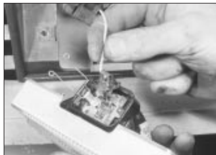
3.11 Extracting the front foglight bulb
