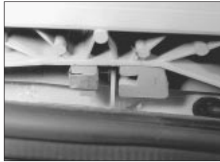
19.7 Tailgate hinge retaining clip
