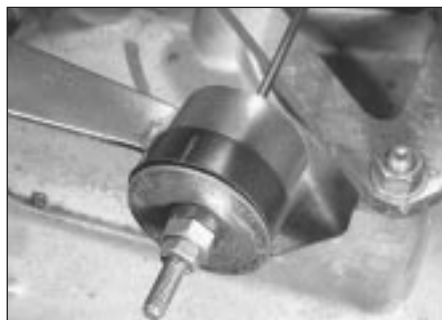
8.24 Clutch cable connection at release lever
