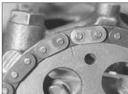
17.34 Timing chain bright links at camshaft sprocket timing mark
