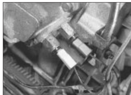
7.2 Coolant temperature switches - BX 16 and BX 19
