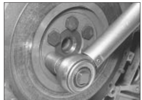
18.14 Tightening flywheel bolts to specified torque
