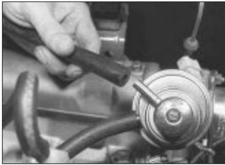
7.1 Fuel supply hose removal from fuel pump
