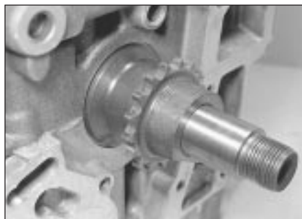
17.32 Locate crankshaft sprocket
