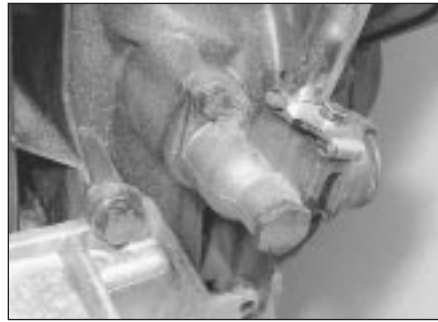
19.49a Securing coolant pipe to inlet housing
