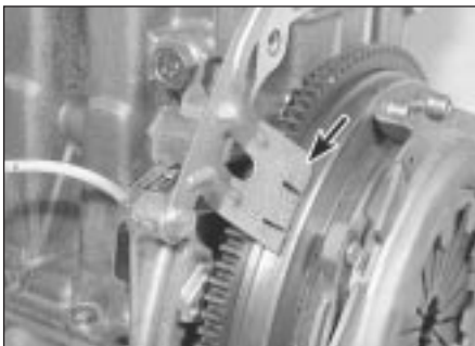
7.20 Timing plate (arrowed)
