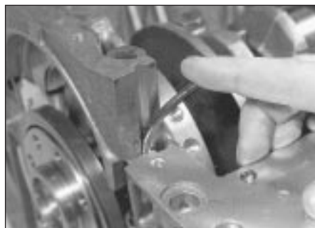
16.6 Flywheel end main bearing cap showing side sealing strip
