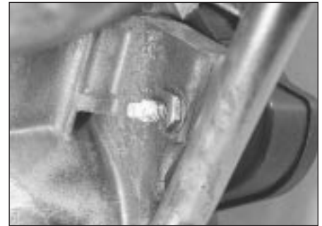
6.8 Tensioner cam spindle (square end) and locknut
