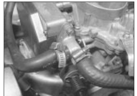
8.5b Coolant hose connections to carburettor auto-choke
