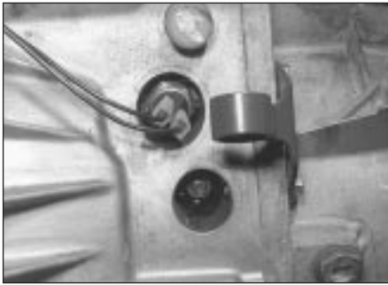
9.16 Reversing light switch and lead connections
