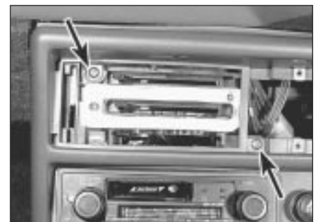
28.4 Remove the panel screws indicated
