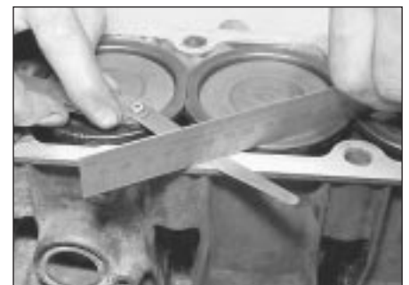
16.6b Measuring cylinder liner projection with a rule and feeler blades
