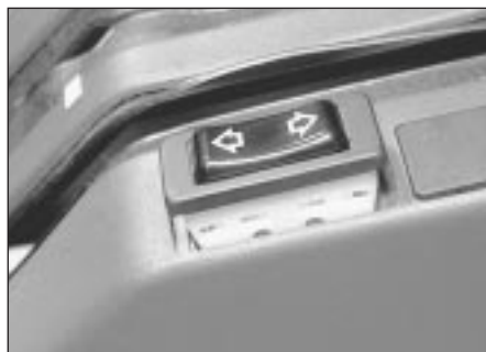
11.2 Electric window operating switch removal
