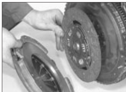
16.21 Fitting clutch components
