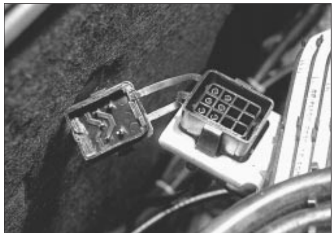
9.1 Diagnostic test socket - BX 16
