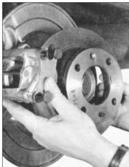
3.9 Rear brake disc removal
