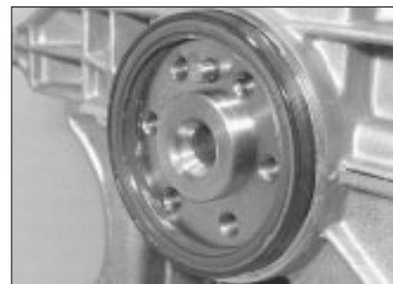
18.23 Crankshaft rear oil seal located over rear of crankshaft
