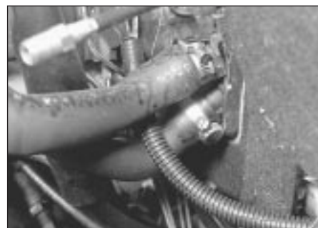
11.21 Heater flow and return hose connections at bulkhead/heater
