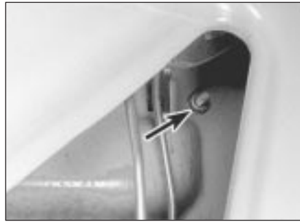
17.8 Door outer handle retaining nut (arrowed)
