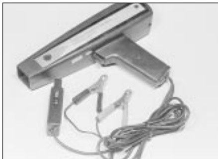
Stroboscopic timing light
