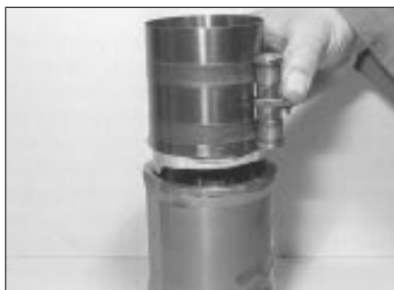
18.14a Fitting a piston ring compressor
