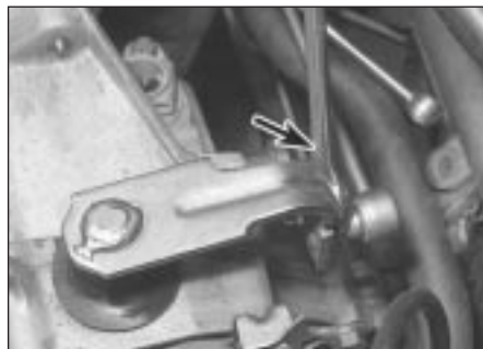
8.15 Using an open-ended spanner (arrowed) to disconnect a gearchange rod balljoint
