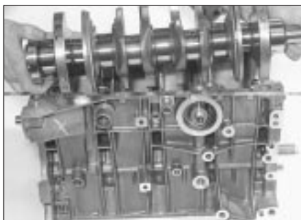
16.4 Lowering crankshaft into crankcase
