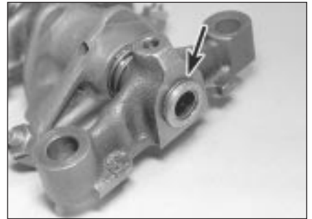
12.34a Rocker shaft retaining circlip (arrowed)
