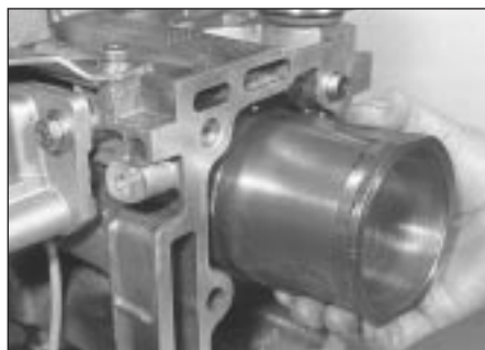
12.45 Removing a liner/piston assembly
