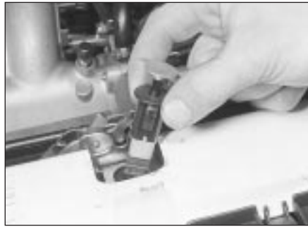
26.4 Removing the bonnet-open warning switch
