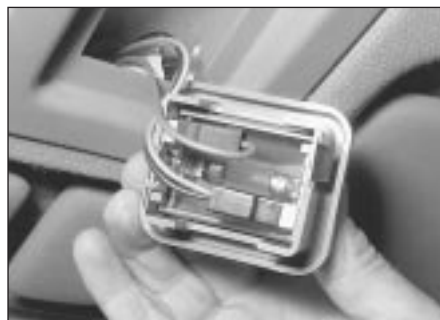
4.6 Interior map lamp bulb - festoon type
