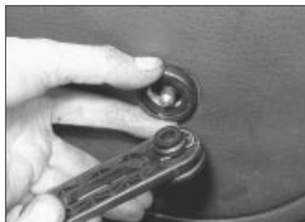
12.1 Removing the window winder handle (manual type)
