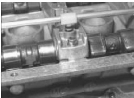
6.33 Camshaft lubrication pipe - note seal on spigot
