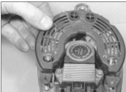
7.3 Removing the rear shield - Paris-Rhone alternator
