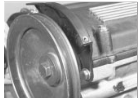
16.36 Camshaft plastic guard and pulley correctly refitted
