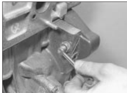
6.12a Turn tensioner cam downwards . . .
