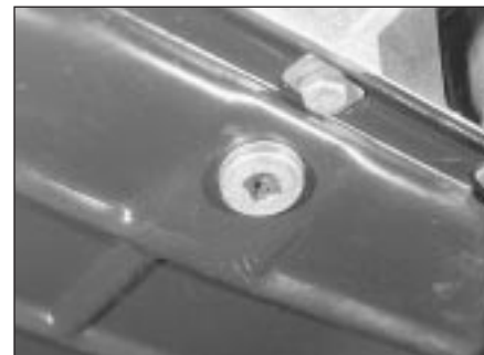
9.3 The engine oil drain plug is located at the lowest point of the sump
