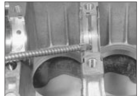
18.3 Oiling main bearing shells
