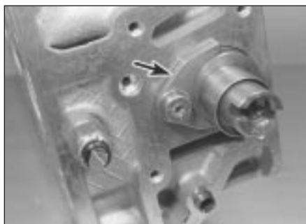
14.2 Camshaft thrust fork (arrowed)
