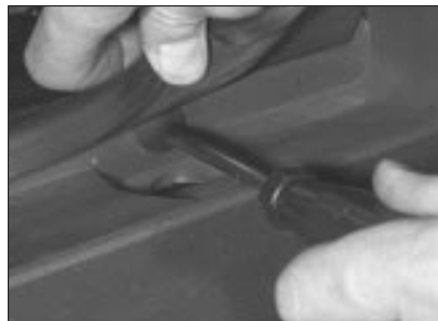
20.11b Unscrewing a rear bumper upper screw
