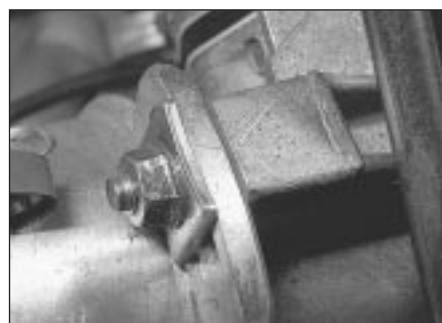
6.6 Distributor timing alignment mark - BX 16
