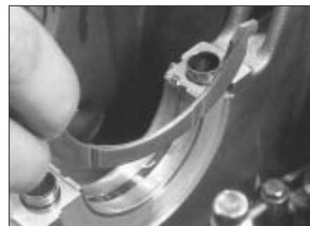
16.3 Fitting a crankshaft thrustwasher
