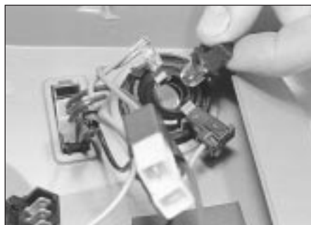
4.4c Removing the map reading light bulb
