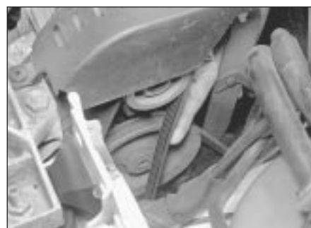
19.2 Checking alternator drivebelt tension
