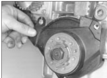
6.5d Removing lower timing cover
