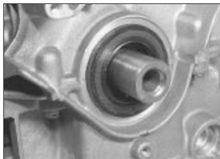
18.27 Crankshaft front oil seal located over front of crankshaft
