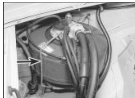
29.3 Spring back the hydraulic reservoir cover retaining clip (arrowed) to release the cover and central block
