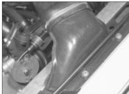
3.4b Air inlet duct attached to crosspanel - GTi
