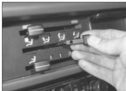
11.6 Heater/ventilation control knob removal
