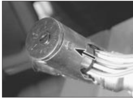
18.4 Remove the bolt (arrowed) . . .
