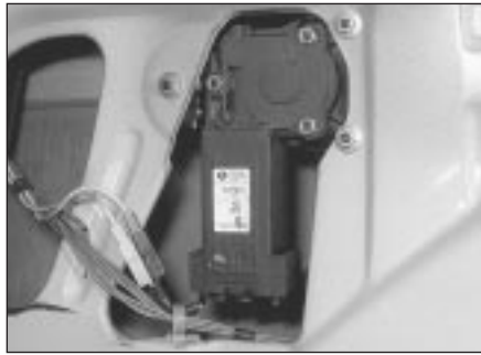
23.3 Electric window regulator unit and wiring connections
