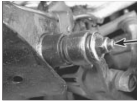
3.13a Remove suspension arm retaining nut at front (arrowed)
