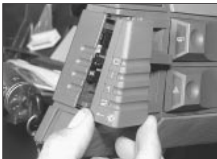
9.3 Removing a central panel
