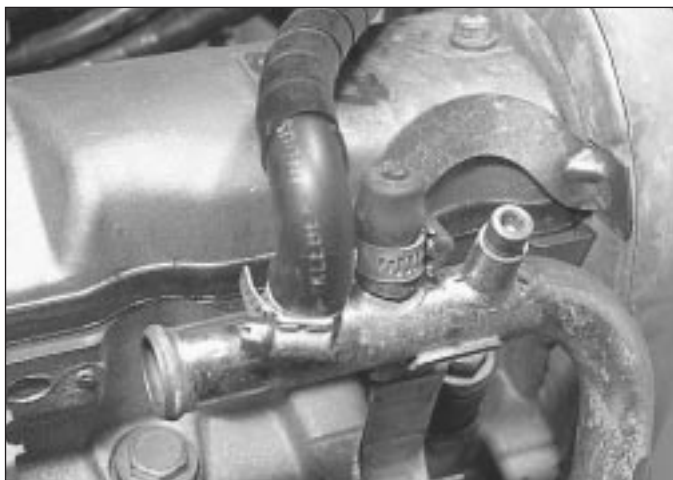
8.6a Heater coolant hose and support clamp
