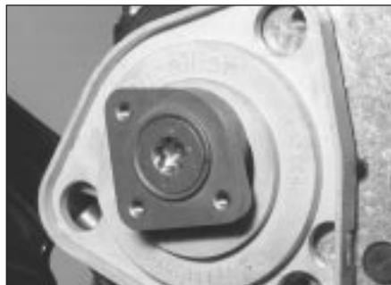
7.4 Rotor drive flange - GTi 16v with Motronic ML4.1
