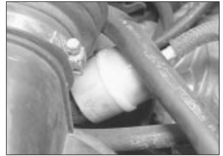
24.1 Note direction of arrow on in-line fuel filter - BX 16 RE
