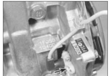
7.19 TDC sensor mounting bolt (arrowed)
