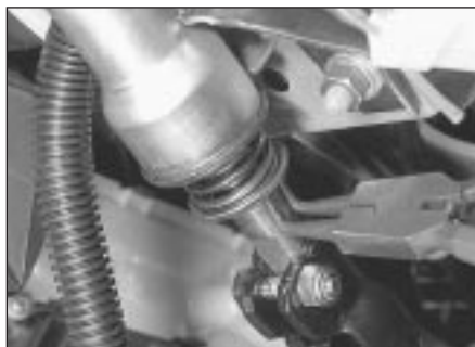
16.10b . . . then locate the circlip in its groove
