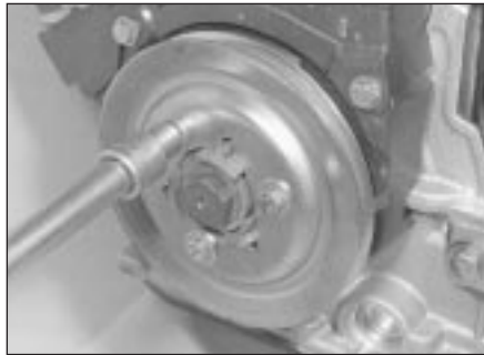
7.12 Unbolting crankshaft pulley
