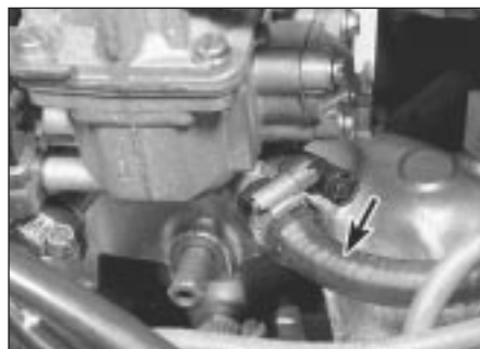
8.26 Heater hose connection at carburettor (arrowed)
