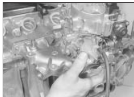
6.14 Timing cover correctly refitted
