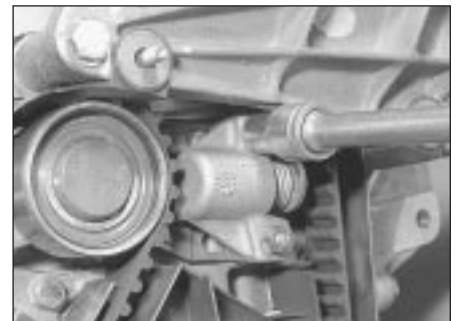
6.12b . . . and tighten drivebelt tensioner front nuts
