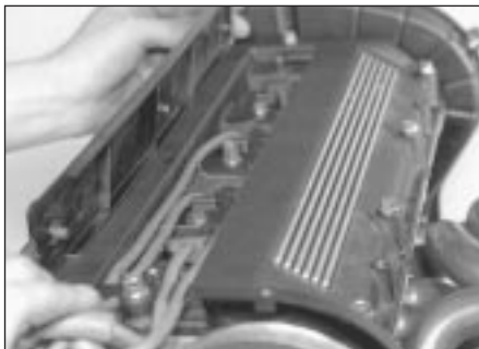
6.2 Removing camshaft centre cover plate
