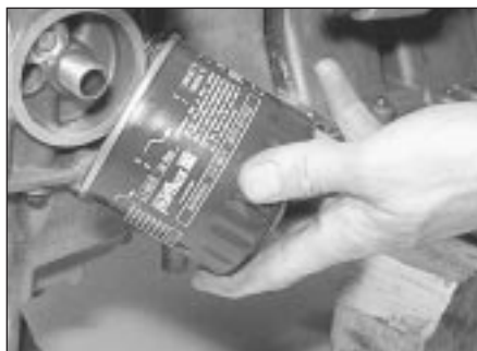
9.7 Removing the engine oil filter
