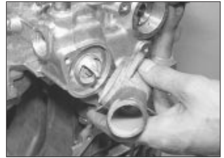
8.3 Thermostat housing cover - BX and BX 14
