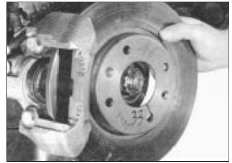
3.2 Front brake disc removal
