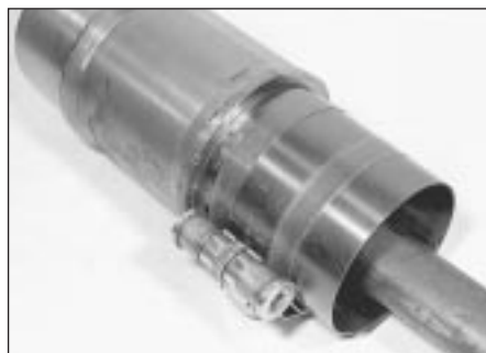
18.14b Using a hammer handle to push a piston into its liner
