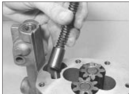
14.11b Oil pump relief valve spring and plunger
