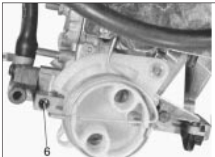
13.5a Solex 32-34 - mixture adjustment screw location (6)
