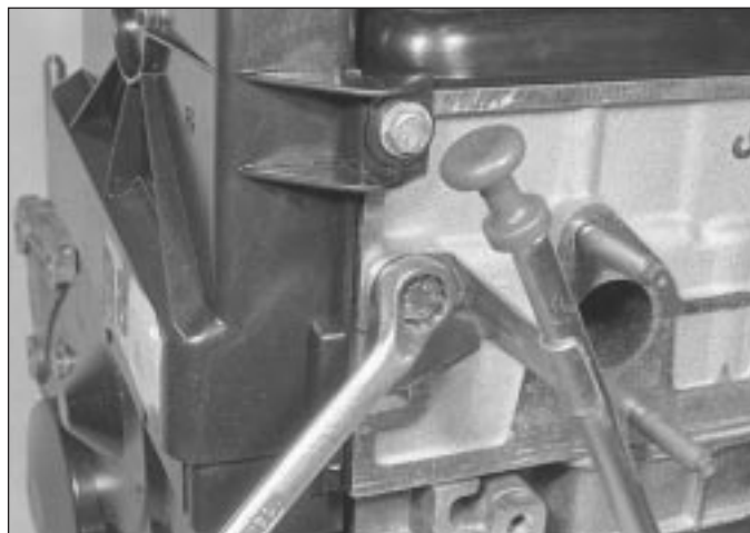
12.18 Unbolting dipstick holder upper mounting
