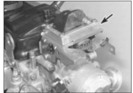
7.13 Ignition coil (arrowed) located above distributor
