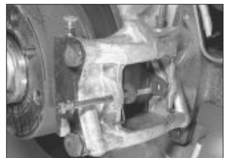
2.25 Locating the through-bolt
