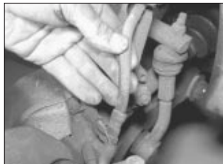
8.4b Examining a brake system hose
