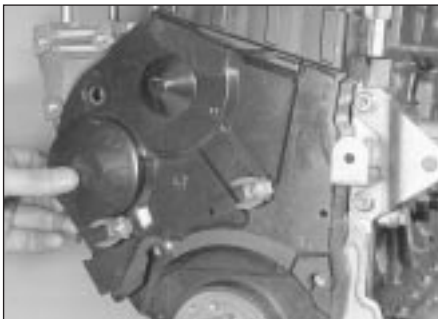
6.5c Removing intermediate timing cover
