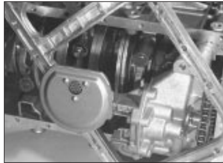
11.32b . . . and remove sump spacer plate
