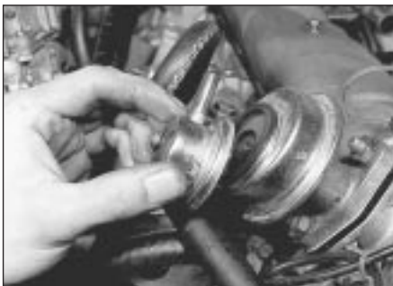
6.1a Fuel pump cover removal - non-removable filter type
