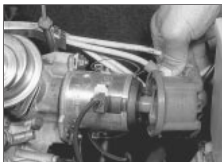
5.3 Removing the distributor cap - BX 16
