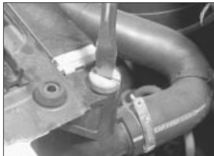
32.2b The radiator bleed screw - all models
