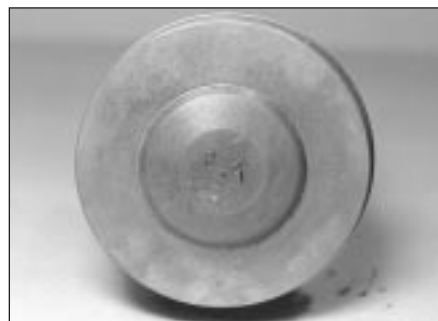
17.6 Piston crown showing directional arrow
