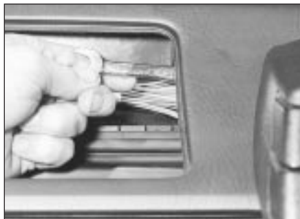
7.16a Working through the facia aperture with a spanner . . .
