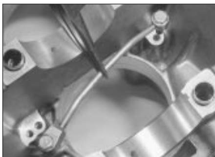
16.1 Fitting a crankcase lubrication pipe
