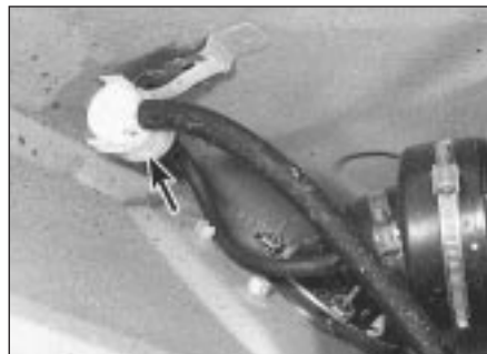
8.3 Vent valve location (arrowed) - GTi
