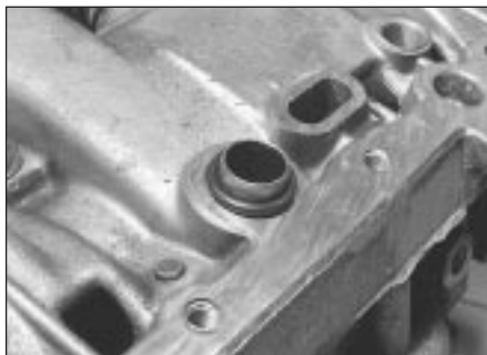
18.6 O-ring seal on transmission casing
