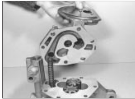
14.10 Separating two halves of oil pump
