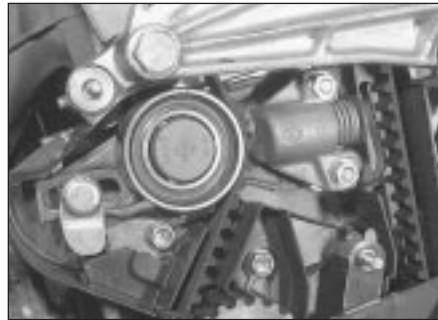
6.7 Central timing cover removed for access to tensioner
