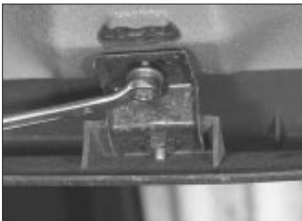
20.11a Unscrewing a rear bumper lower screw
