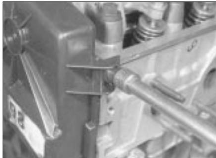
6.5a Unbolting upper timing cover
