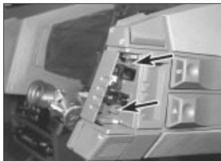
9.4a Remove the two retaining screws (arrowed) . . .
