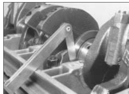
17.17 Checking crankshaft endfloat
