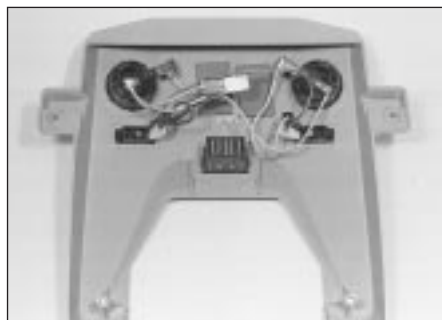
4.4b Map reading light/ sunroof console removed
