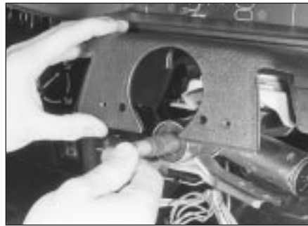
9.13a Removing the steering column upper shroud
