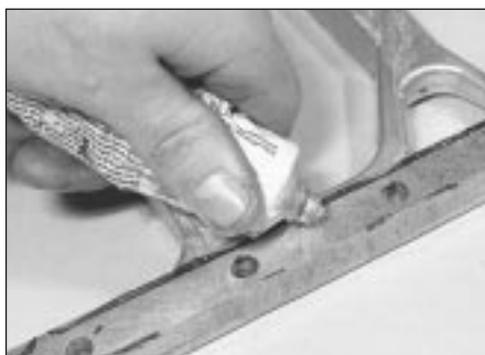
16.18 Applying instant gasket to sump spacer plate
