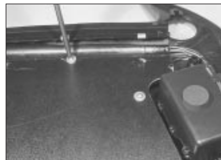
12.10 Extracting a screw from the window regulator mounting panel
