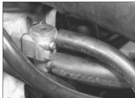
14.9 Solex 32-34 - ventilation hose connections
