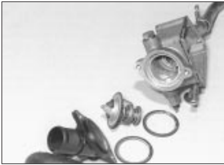
8.1b Thermostat housing dismantled - BX 19 GTi 16v
