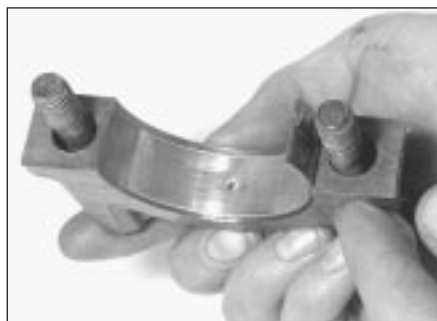
16.5a Main bearing cap with plain shell fitted
