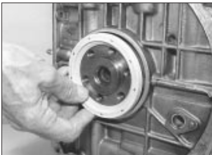
17.27 Fitting new crankshaft oil seal
