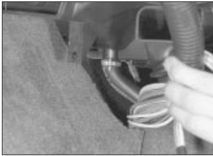
11.27 Heater coolant drain hose
