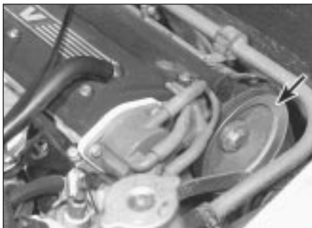
7.3a Hydraulic pump drive pulley (arrowed)
