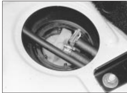
7.2 Fuel tank supply and return hoses - GTi
