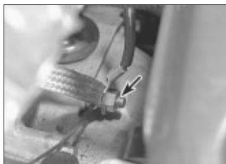
8.27 Earth cables at transmission (arrowed)
