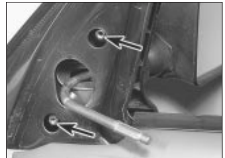
10.4 Door mirror retaining nuts (arrowed)
