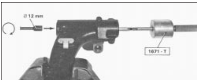
8.12 Rear suspension arm bearing removal tools
