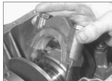
16.5b Fitting a main bearing cap
