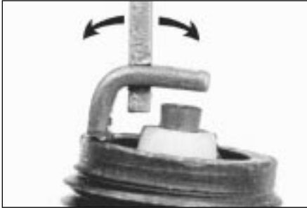
Adjusting spark plug gap
