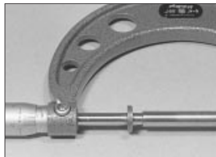
22.11b Measuring shim thickness with a micrometer
