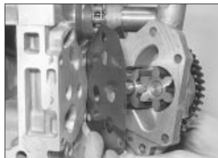
17.39 Fitting oil pump with spacer plate
