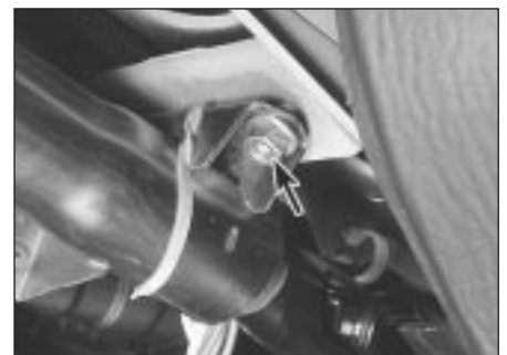
19.4 Steering column upper retaining nut (arrowed)
