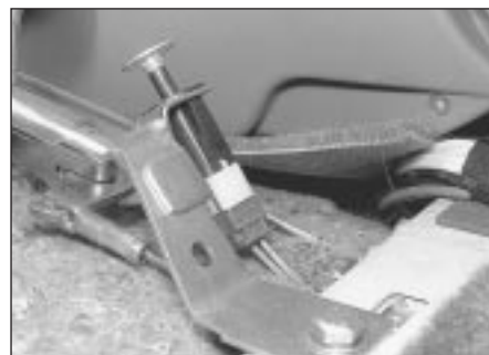
13.5 Handbrake warning light switch
