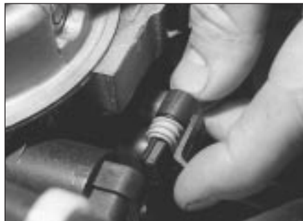
12.2b . . . the idle control stepper motor . . .
