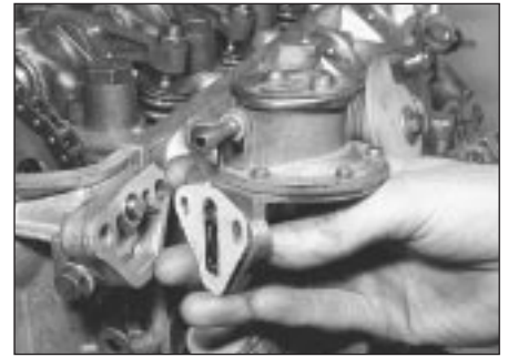
7.3b Fuel pump removal - BX 14
