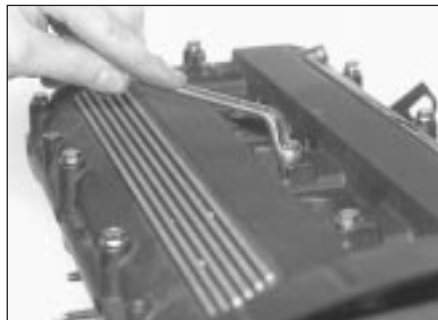
6.8a Extracting a camshaft cover screw
