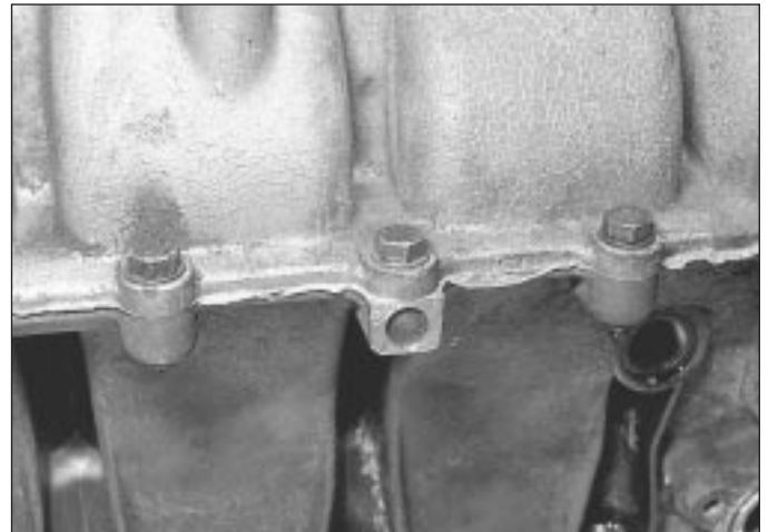
17.26 Crankcase housing flange bolts
