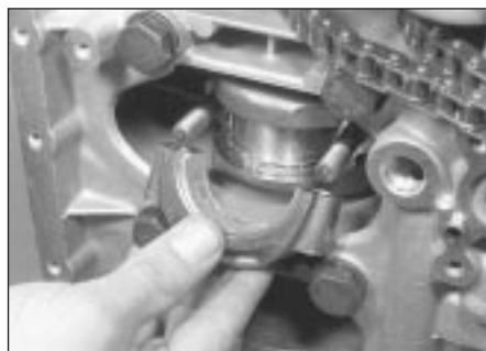
12.44 Removing a big-end bearing cap
