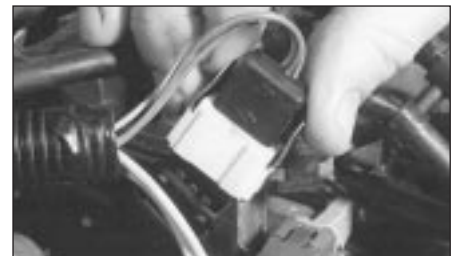
E Check all wiring block connectors are clean and secure.
