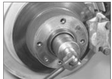
7.1b . . . and loosen the hub nut
