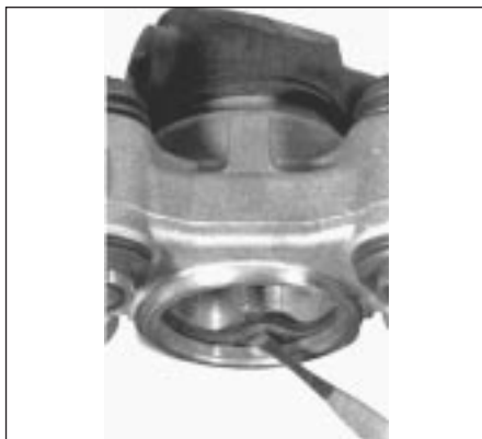
4.15 Prise free the cylinder inner seal
