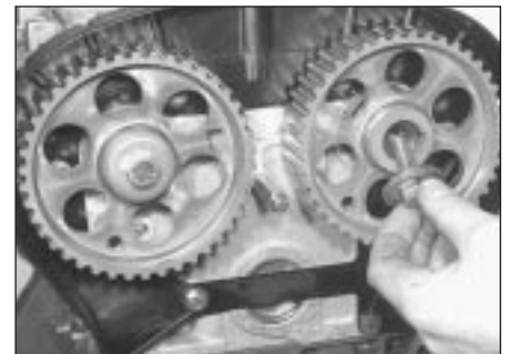
6.34b Fitting a camshaft sprocket bolt
