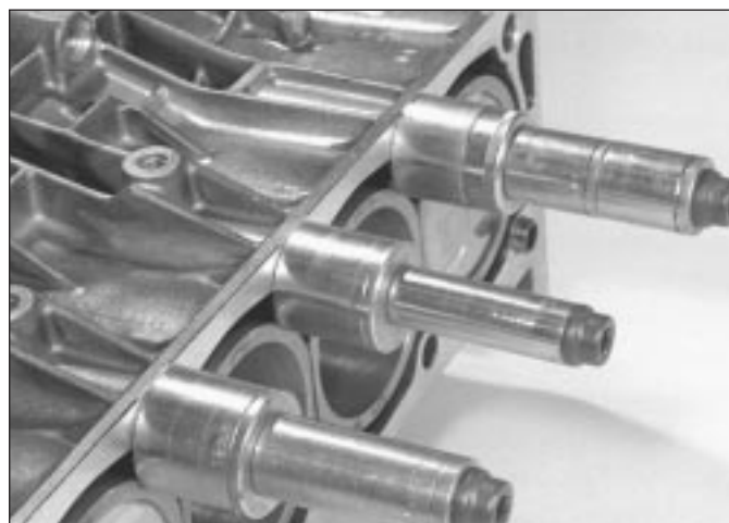
16.12b Typical cylinder liner clamps fitted
