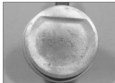
19.16 Arrow mark on piston crowns must point to camshaft sprocket end (letter and number indicate liner and gudgeon pin grade)
