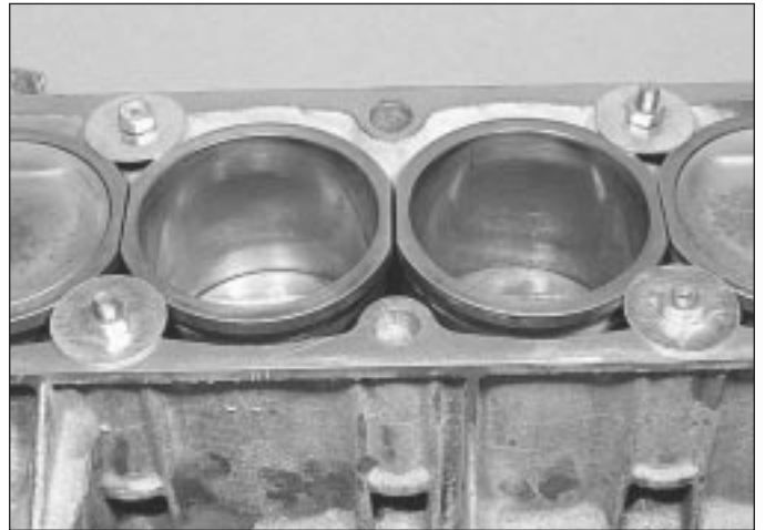
8.20 Cylinder liners clamped with washers and bolts
