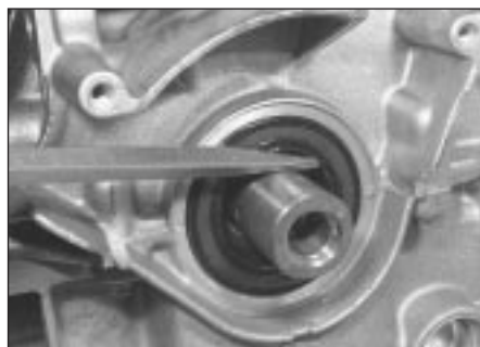
12.35 Prising out crankshaft front oil seal
