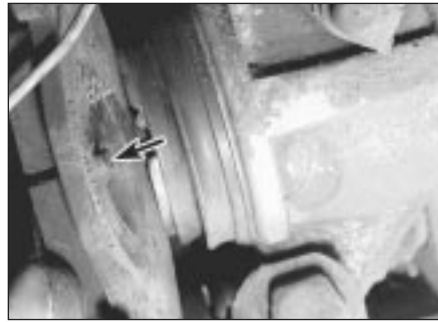
3.0b Locating pip (arrowed) on inboard pad
