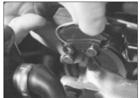
12.4 Disconnecting accelerator inner cable from throttle cam
