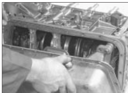
16.19 Refitting sump pan and gasket
