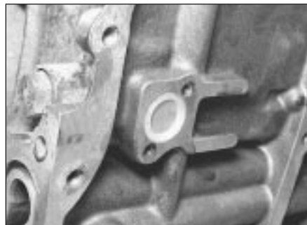
17.29a Locate chain tensioner filter . . .
