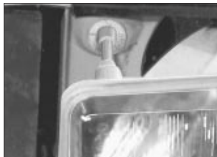
3.6 Headlamp ball and socket mounting
