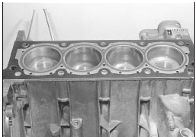
19.28 Head gasket correctly fitted
