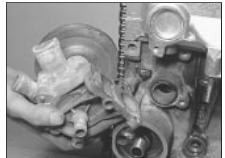
9.5b Fitting coolant pump
