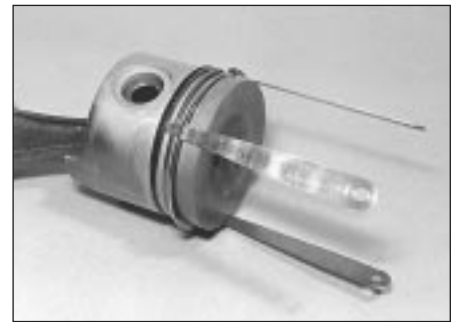
17.1 Method of fitting piston rings
