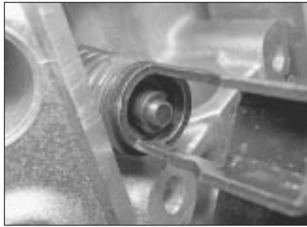
13.2 Compress valve spring ...
