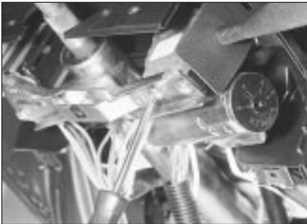
9.14a Removing a steering column switch
