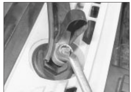
18.3 . . . and unscrew the wiper arm retaining nut
