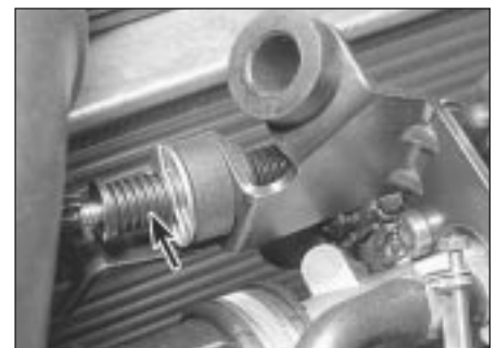
13.1 Accelerator cable adjustment ferrule (arrowed)
