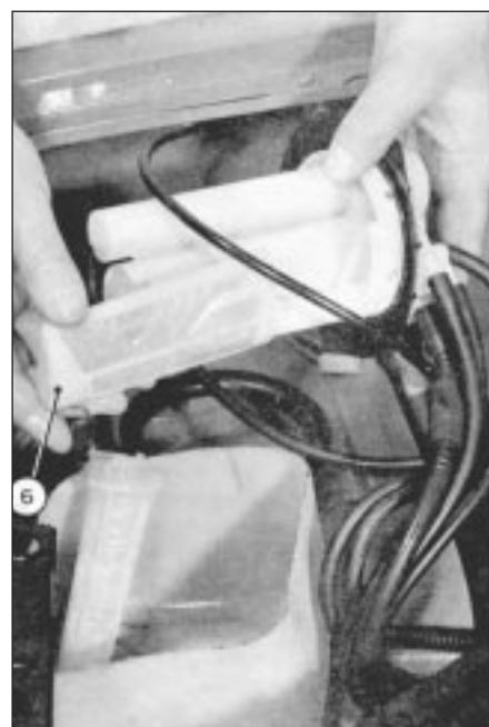
29.4 Remove the hydraulic filter assembly from the central block
