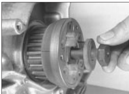
12.34a Removing crankshaft sprocket bolt . . .
