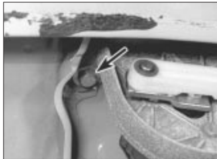
19.6a Wiper motor retaining bolt (arrowed)
