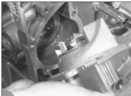
10.6 Withdrawing coolant pump
