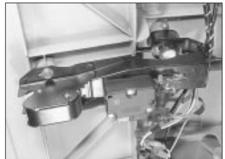
25.10 Tailgate central locking solenoid and lock unit
