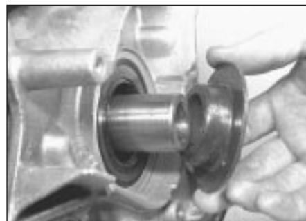
12.34c . . . and timing belt guide plate
