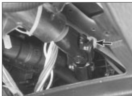
19.3 Steering intermediate shaft universal joint (arrowed)
