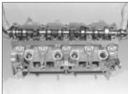
15.9 Fit camshaft into position
