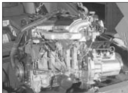
8.33 Lifting engine/transmission unit from vehicle
