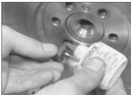
18.25 Applying locking fluid to a flywheel bolt
