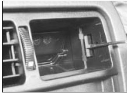
14.7 Centre vent grille retaining clip (grille removed for clarity)
