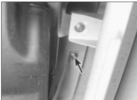
8.2 De-aeration reservoir retaining strap and mounting bolt (arrowed)
