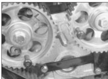
5.12a Camshaft sprocket locking pins in position
