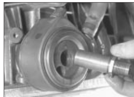
16.32 Fitting oil cooler retaining tube and nut
