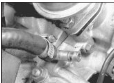
32.2d Bleed screw adjacent to thermostat housing - BX 16 and BX 19
