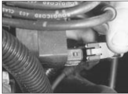
5.8 Disconnect ignition coil wiring connector
