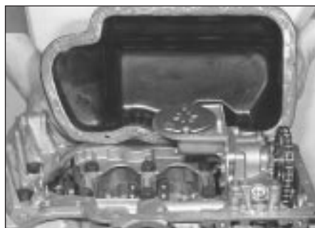
12.39 Removing the sump
