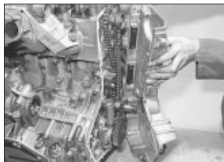
18.8a Refitting timing cover with new gasket
