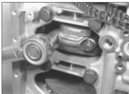
18.17 Tightening a big-end bearing cap nut
