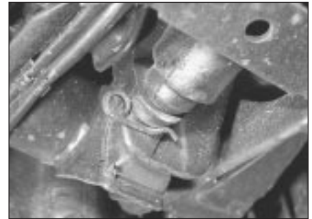
9.7 Rear suspension unit rod clip
