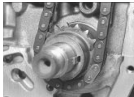
17.33 Timing chain bright link at crankshaft sprocket
