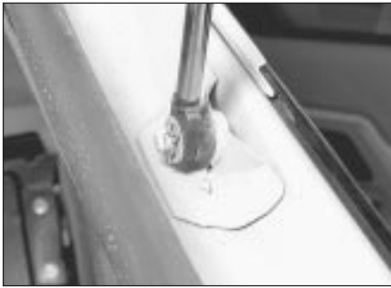
19.6b Tailgate support strut and retaining clip to body
