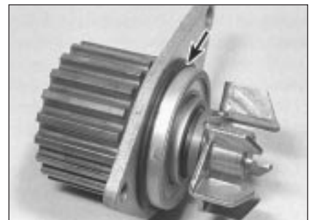
9.19b Coolant pump O-ring (arrowed)
