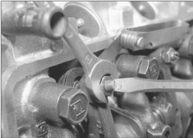
21.6 Adjusting a valve clearance - 150 engine
