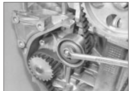
6.8 Loosening timing belt tensioner roller nut
