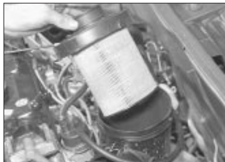
28.5b . . . and withdraw the lid/element assembly - BX 14 with K1G engine
