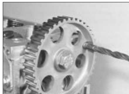
7.37 Camshaft sprocket held at TDC using twist drill
