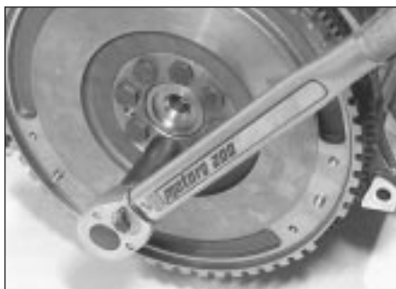
16.20 Tightening a flywheel bolt
