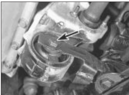
9.30 Torque link and through-bolt (arrowed)
