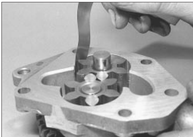
12.41 Checking oil pump lobe tip clearance
