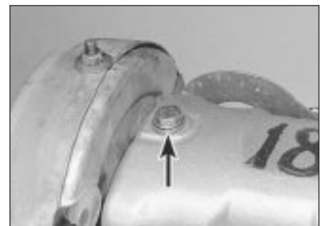
22.9 Copper washer (arrowed) under bolt head
