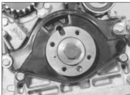
5.18a Timing belt lower cover refitted
