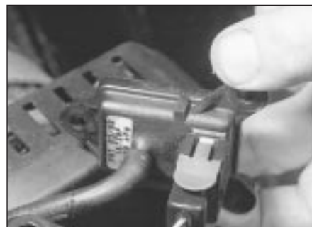
11.18b . . . then free MAP sensor from bracket and disconnect vacuum hose and wiring connector
