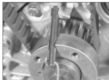
5.12b Crankshaft sprocket locking rod in position
