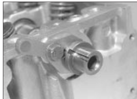
13.1a Remove camshaft retaining plate . . .
