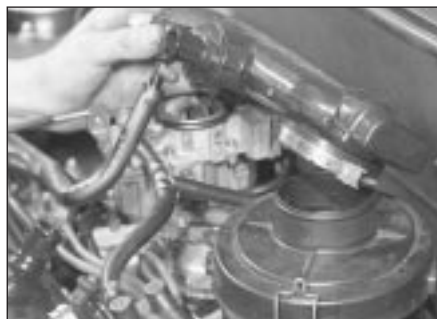
3.3b Removing air intake duct from carburettor and air cleaner
