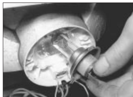
3.2b . . . and remove the headlamp bulb
