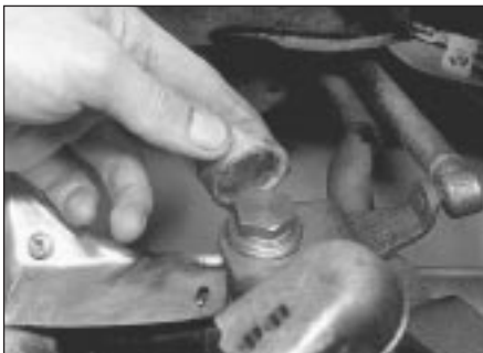
20.7 Gearchange control pivot bolt and cover - BX 16 and BX 19
