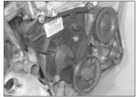
19.49b Refitting HP pump and drivebelt
