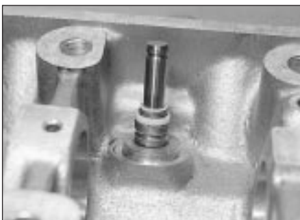
13.15 Valve stem oil seal
