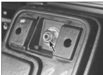
16.15b . . . to expose wheel retaining nut (arrowed)
