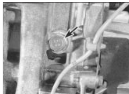
32.4 Cylinder block coolant drain plug - K1G engine
