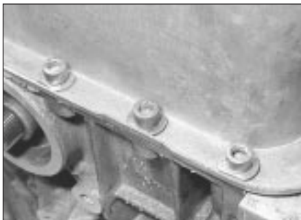
13.19 Location of three Allen head bolts
