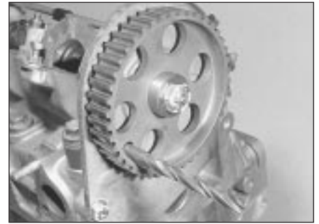
13.12 Lock camshaft sprocket with a 10 mm rod
