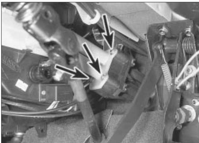
14.3 Heater tap (control) unit retaining screws (arrowed)
