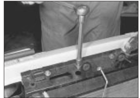
3.4a Undoing radiator retaining bolts
