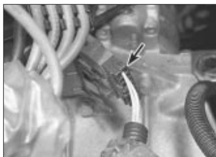
8.28 Temperature switch/oil pressure switch/reversing light switch wiring connector (arrowed)
