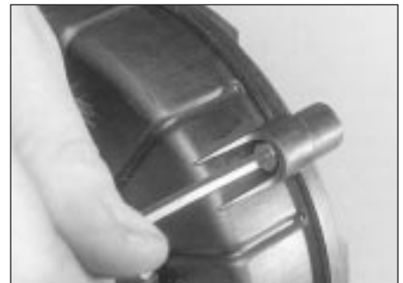
6.8b Extracting a timing belt cover screw
