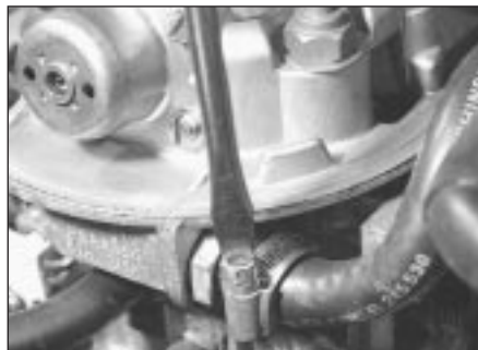
12.3 Slacken throttle body fuel feed hose retaining clip
