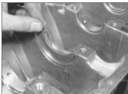
12.51b ... and endfloat thrustwasher
