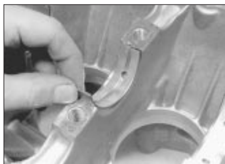
12.51a Removing a main bearing shell ...
