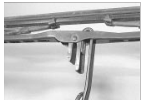
17.2 Wiper blade removal from arm
