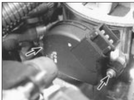
13.2 Throttle potentiometer retaining screws (arrowed)
