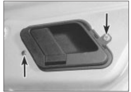
17.10 Door inner handle and retaining bolts (arrowed)
