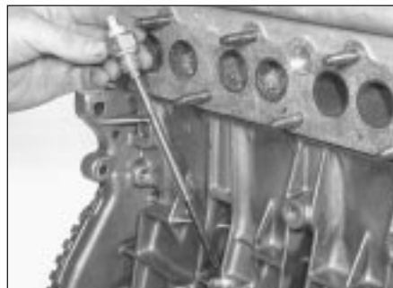
16.35b Refitting oil level sensor
