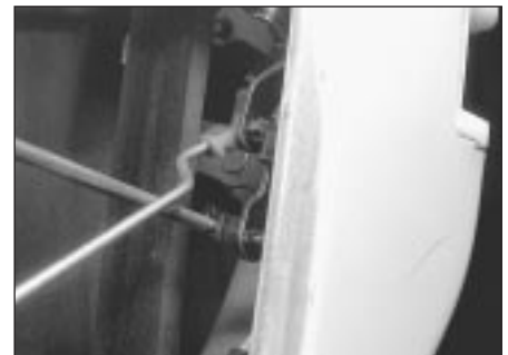
17.3 Door lock control rods and nylon fasteners
