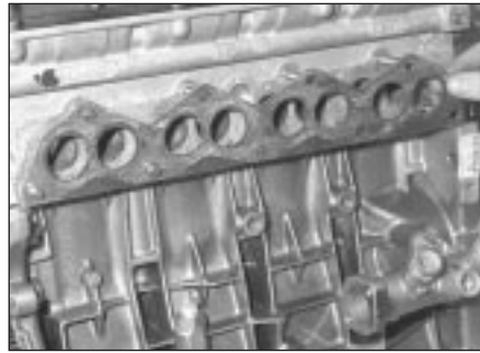
6.38a Exhaust manifold gasket correctly located
