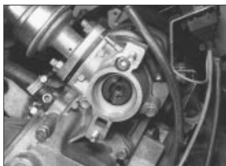
6.9 Distributor drive engagement dog is offset - BX 16
