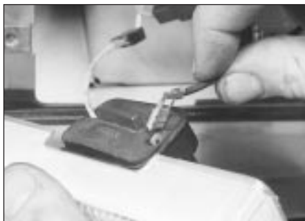
3.10 Disconnecting the foglight wiring
