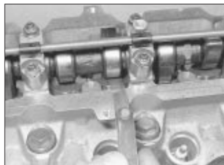
22.5b Measuring a valve clearance - 171 and 159 engines
