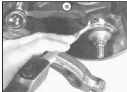
15.8b Lock lower joint by stake punching at points indicated (a)
