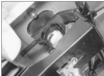
25.9 Lock barrel and retaining clip (central locking)
