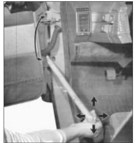
18.7b Adjusting door position by moving a hinge
