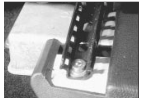
8.1 ECU location - GTi 16v with Motronic ML4.1
