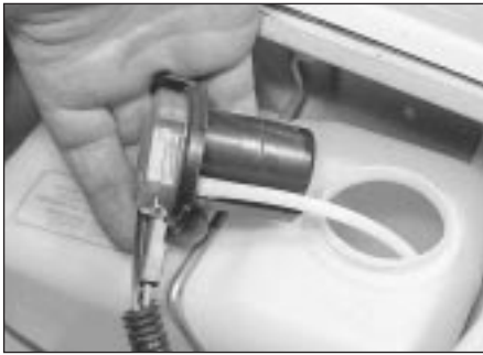
22.2 Washer unit filler cap/pump unit
