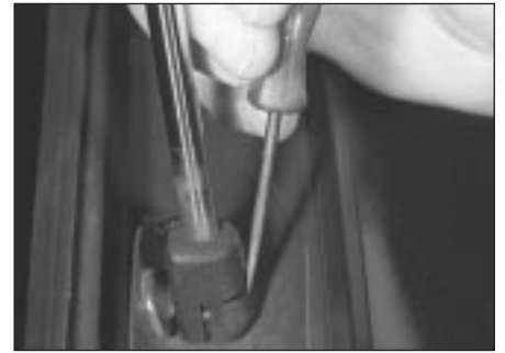
19.11 Prising out tailgate strut balljoint clip
