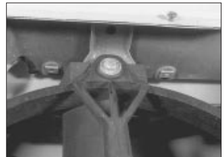
4.4 Cooling fan retaining bolt
