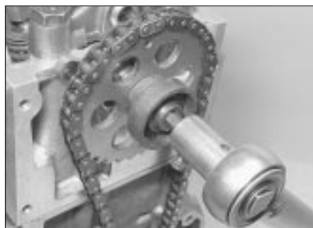
17.35b Tightening sprocket retaining bolt
