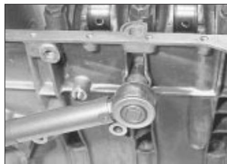
19.12 Tightening No. 3 main bearing side bolt
