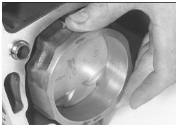
16.12a Fitting a piston/connecting rod/liner assembly
