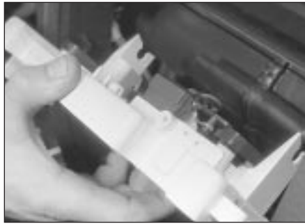
15.6 Withdrawing the heater control unit
