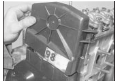
6.5b Removing upper timing cover
