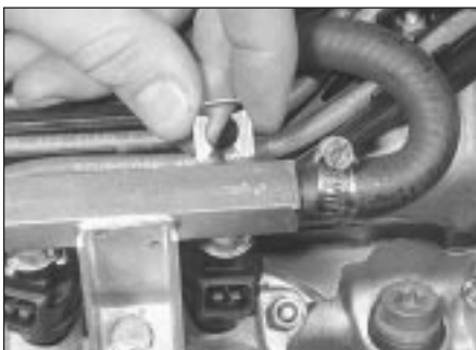
12.3b Fuel rail/injector clip
