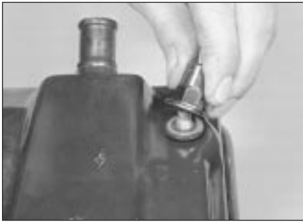
6.3a Removing a rocker cover nut
