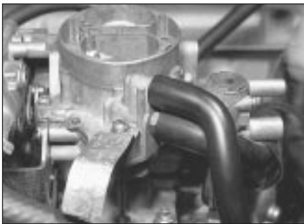
14.4b Solex 32-34 - fuel supply and return hoses
