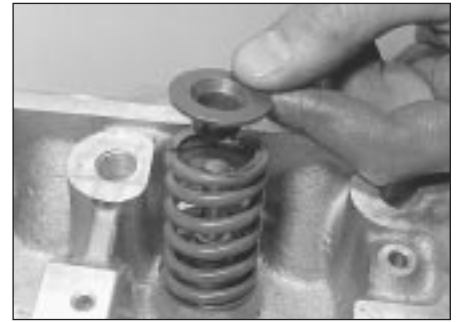
13.3a ... and remove spring cup retainer, spring ...
