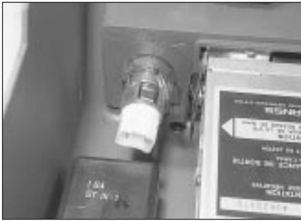
14.4 Cigar lighter with bulb and wiring connector detached
