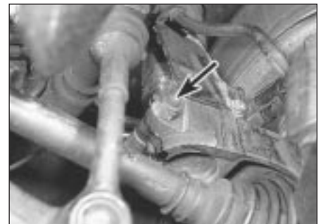
5.8 Swivel hub-to-suspension unit clamp bolt (arrowed)
