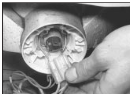
3.2a Disconnect the wiring connector . . .
