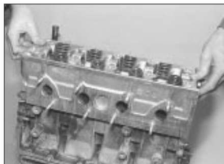
6.34a Lower cylinder head into position . . .
