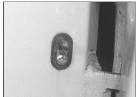
10.2 Door courtesy light switch retaining screw
