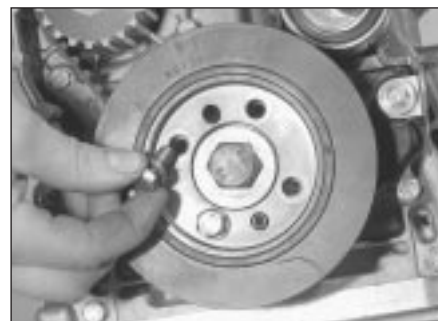
5.18b Fitting a crankshaft damper bolt
