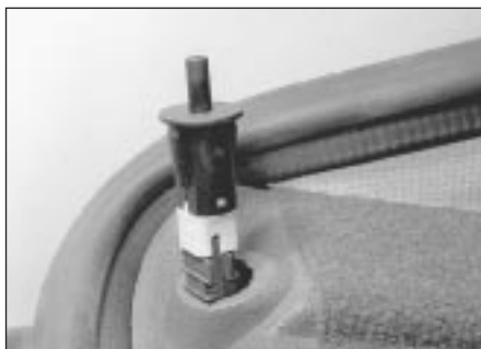
10.5 Boot light switch unit removal
