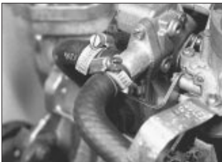
14.8 Solex 32-34 - coolant hose connections
