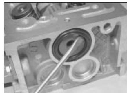
14.3a Prise out camshaft oil seal ...
