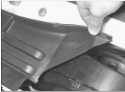
13.13 Removing plastic cover from heater blower motor
