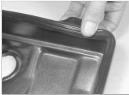
6.3b Removing rocker cover gasket
