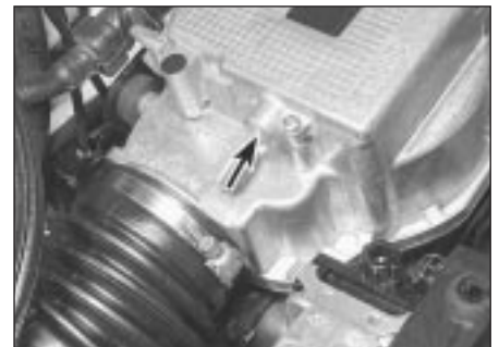
9.3 Mixture adjustment screw (arrowed)
