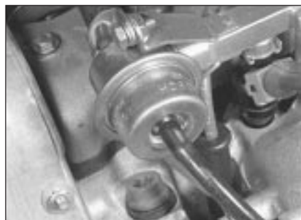
12.4b Pressure regulator attached to fuel rail
