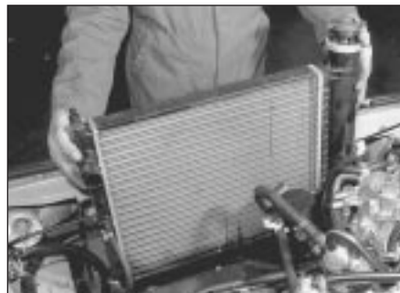
3.5 Lifting radiator out of vehicle
