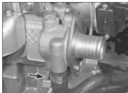
7.8 Water pump hose (arrowed) at thermostat housing
