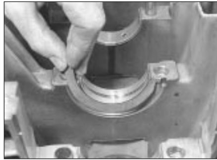
19.3 Fitting thrustwasher upper segments
