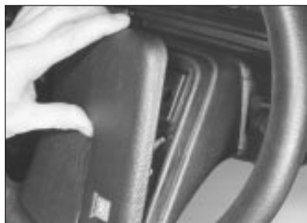
16.15a Remove the centre pad from the steering wheel . . .
