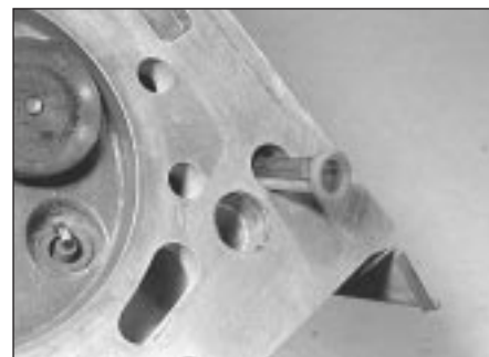
15.12 Insert oil filter gauze in cylinder head oilway
