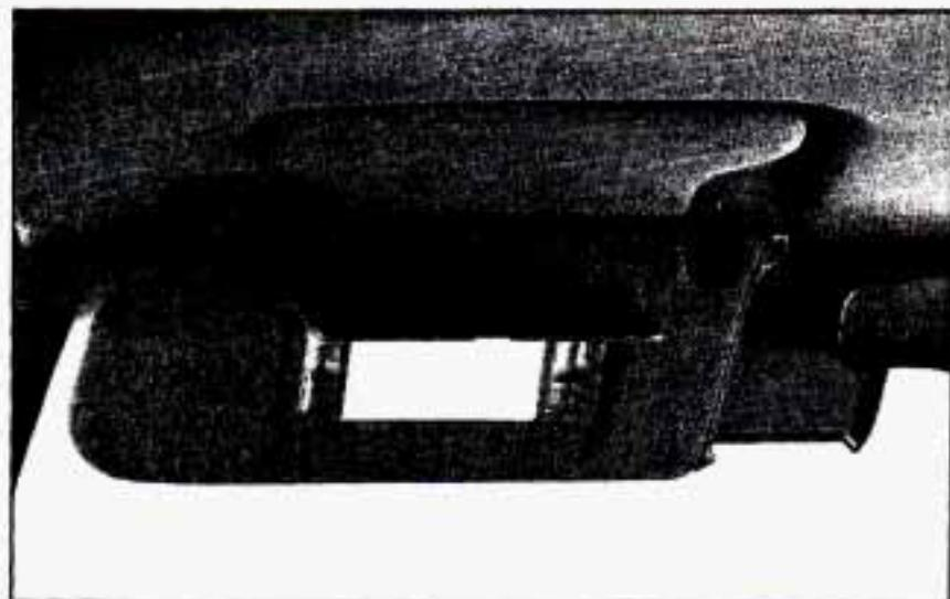
Pull the sun visor down and lift the mirror cover to turn on the lamps.
