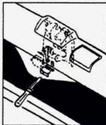
2. Use a thin screwdriver to reach through the access holes in both the trim panel and the hardware cover.
