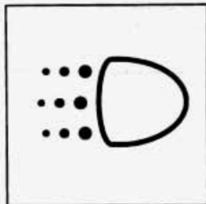
This light is on the instrument panel. It goes on whenever the DRL are on, the ignition is on, the headlamp switch is off and the parking brake is released.
