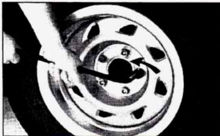
1. Using the wheel wrench, loosen all the wheel nuts. Don't remove them yet.
