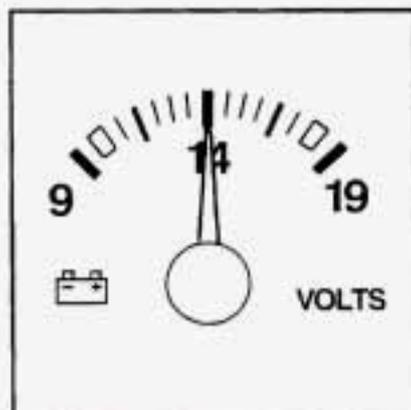
When your engine is not running, but the ignition is on (in the RUN position), this gage shows your battery's state of charge in DC volts.
