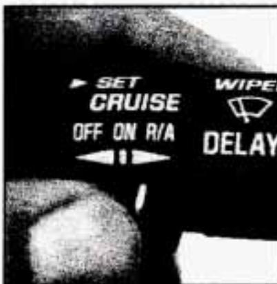
Once you're going about 25 mph (40 km/h) or more, you can move the cruise control switch from ON to R/A for about a half a second.
