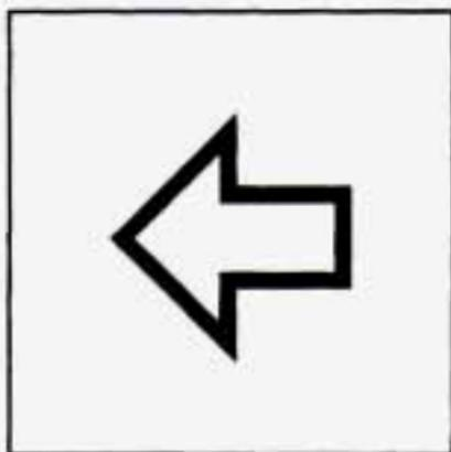
An arrow on the instrument panel will flash in the direction of the turn or lane change.
