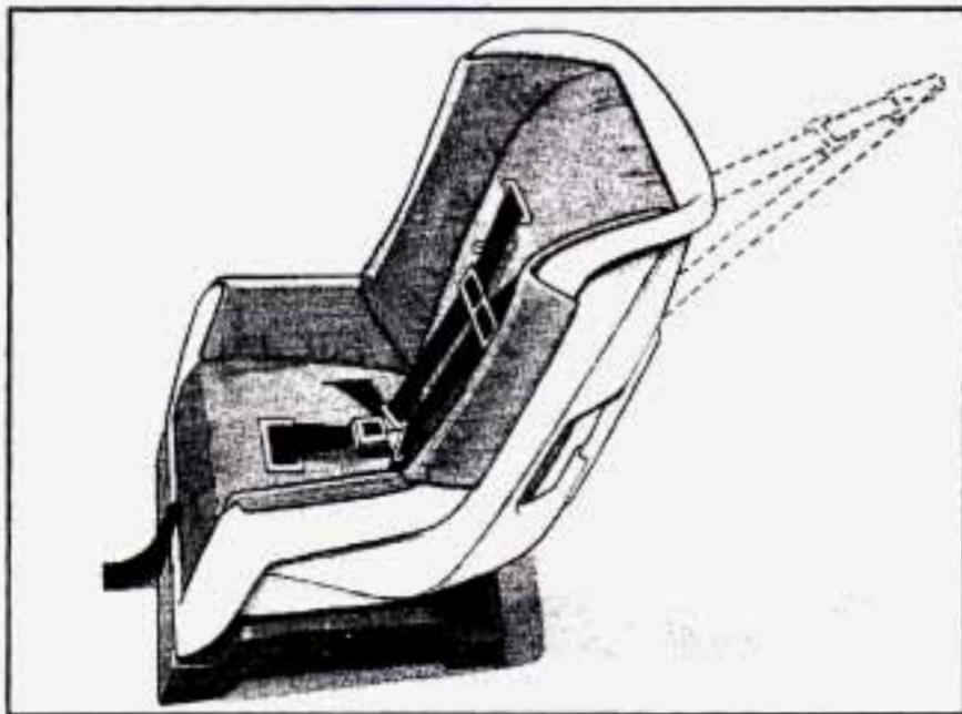
If your child restraint has a top strap, it should be anchored. Anchor brackets for the rear outside seat positions are located on the floor in the cargo area.
