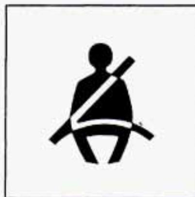
The safety belt light will also come on and stay on for about 20 seconds, then it will flash for about 55 seconds. If the driver's belt is already buckled, neither the tone nor the light will come on.
