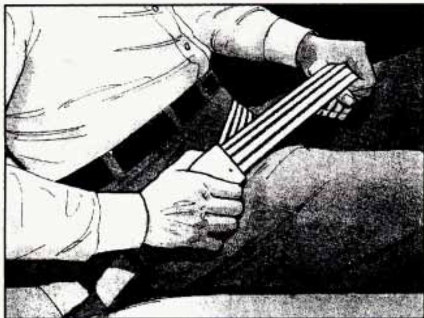
When you sit in the center front seating position, you have a lap safety belt, which has no retractor. To make the belt longer, tilt the latch plate and pull it along the belt.
