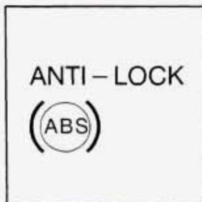
With the anti-lock brake system, this light will come on when you start your engine and may stay on for several seconds. That's normal.
