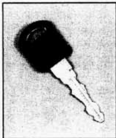
This vehicle has one double-sided key for the ignition, endgate, spare tire lock (two-door vehicles) and door locks. It will fit with either side up.
