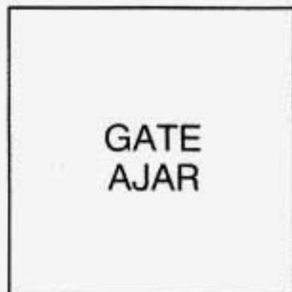
This light will come on briefly when you are starting the engine. If it stays on, your liftgate is ajar. Try closing the liftgate again. Never drive with the liftgate even partially open.
