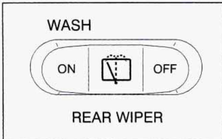
This switch is located on the instrument panel.
