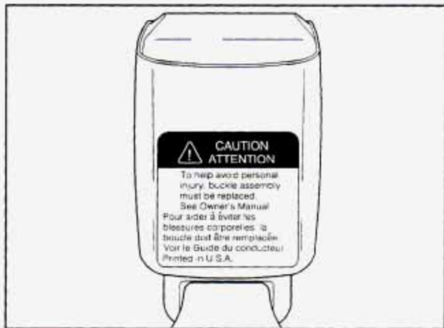
If you ever see a label on the driver's safety belt buckle that says to replace the buckle assembly, be sure to do so. Then the new buckle assembly will be there to help protect you in a collision.
