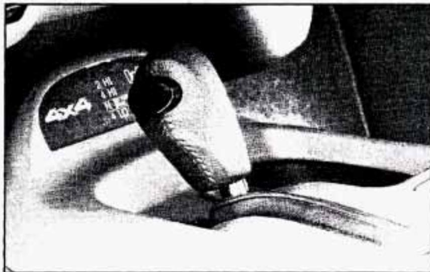
If your four-wheel-drive vehicle has the manual transfer case, the transfer case shift lever is on the floor next to the driver. Use this lever to shift into and out of four-wheel drive.
