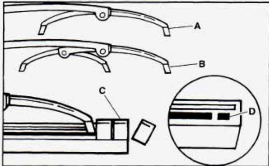
4. To install the new wiper insert, slide the insert (D), notched end last, into the end with two blade claws (A). Slide the insert all the way through the blade claws at the opposite end (B). The plastic caps (C) will be forced off as the insert is fully inserted.
