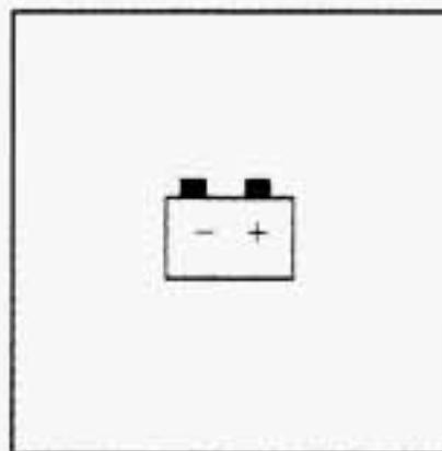
The charging system light will come on briefly when you turn on the ignition, but the engine is not running, as a check to show you it is working.
