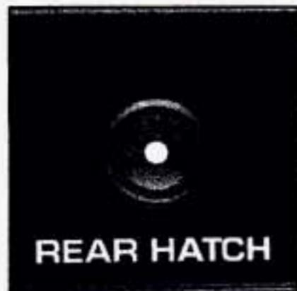
This button on the driver's side of the steering column allows you to release the rear glass from inside the vehicle.
