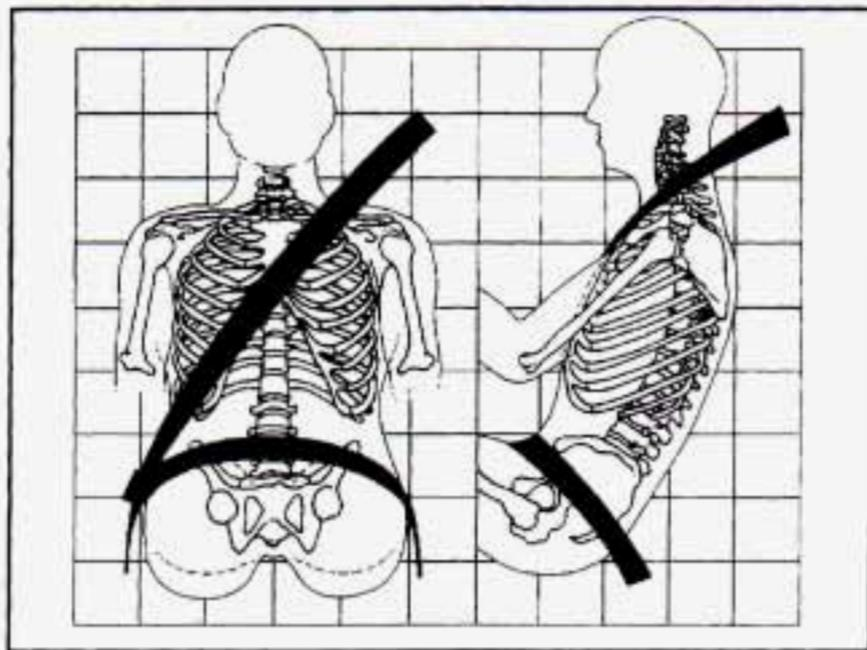
The lap part of the belt should be worn low and snug on the hips, just touching the thighs. In a crash, this applies force to the strong pelvic bones.
