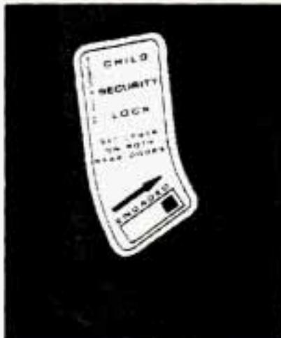
With this feature, you can lock the rear doors so they can't be opened from the inside by passengers.
