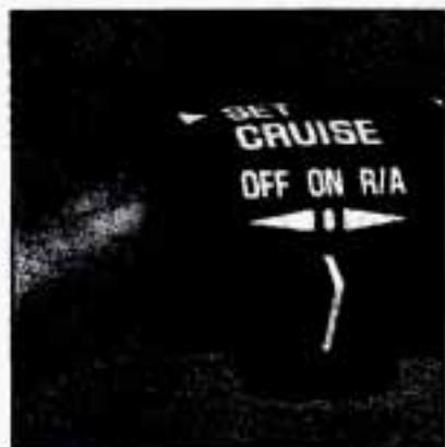
3. Press in the SET button at the end of the lever and release it.
