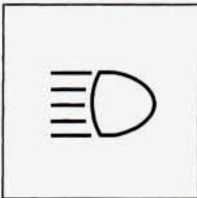
When the high beams are on, this indicator light on the instrument panel will also be on.
