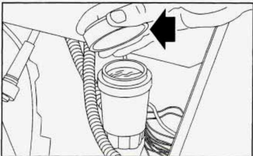
Refer to the Maintenance Schedule, Owner Checks and Services, to determine how often you should check the fluid level in your clutch master cylinder reservoir and for the proper fluid. See "Owner Checks and Services" and "Recommended Fluids and Lubricants" in the Index.
