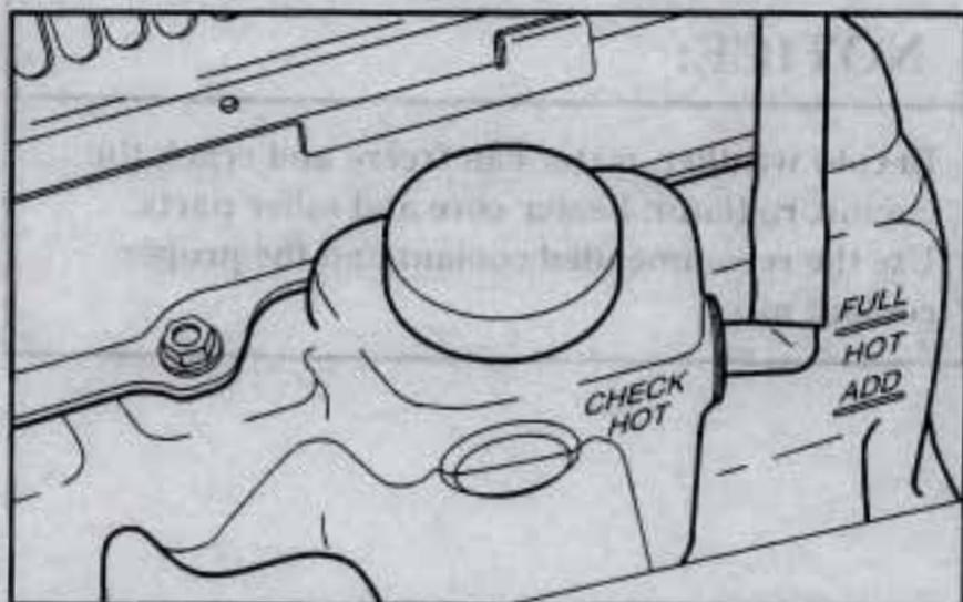
The coolant level should be at the ADD mark.
