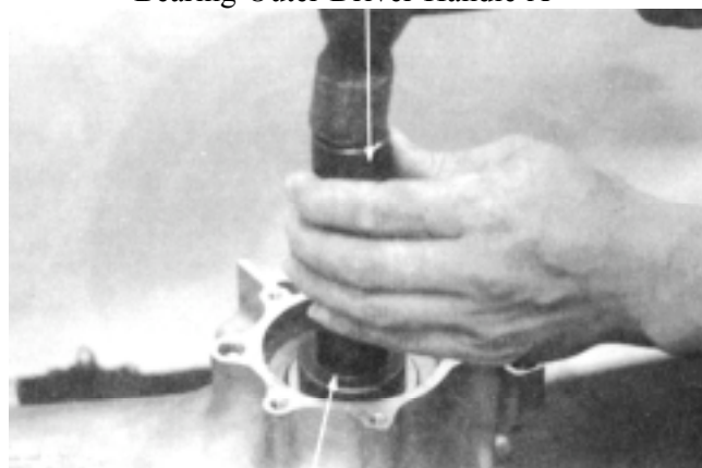
Bearing Outer Driver, 42x47mm Pilot, 20mm
