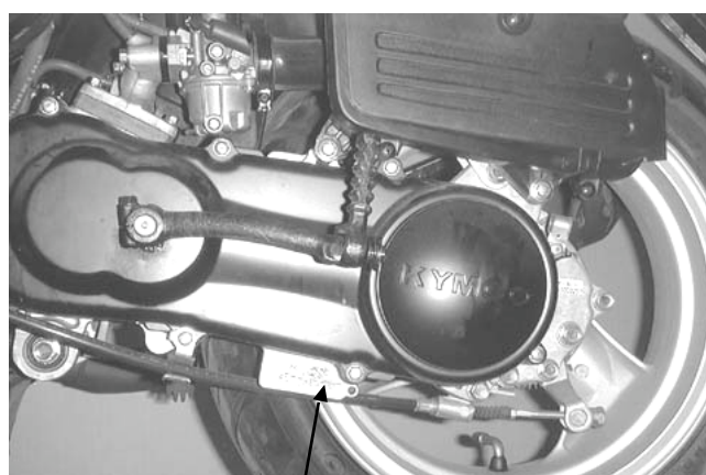
Location of Engine Serial Number
