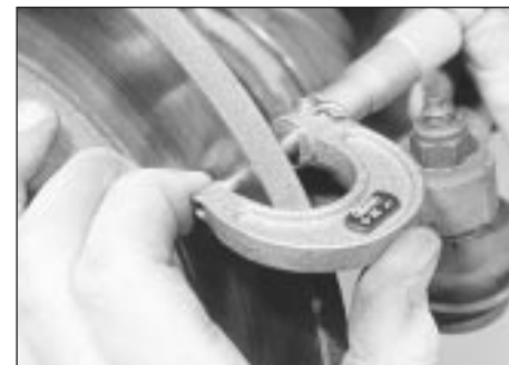
7.3 Using a micrometer to measure disc thickness
