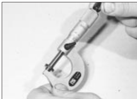
11.16b Using a micrometer to measure shim thickness
