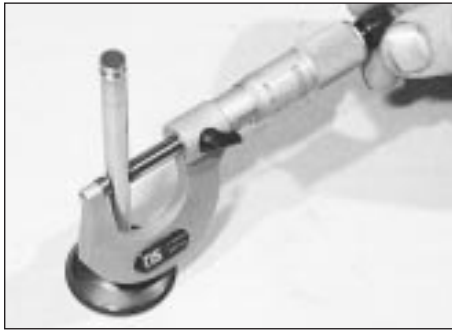
8.11 Measuring a valve stem diameter
