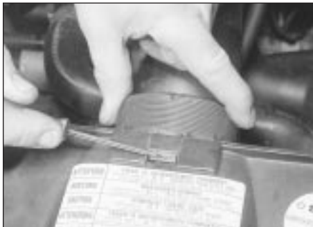
3.5a Depress the securing clip . . .
