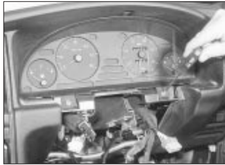
9.21 Unscrew the lower instrument panel securing screws
