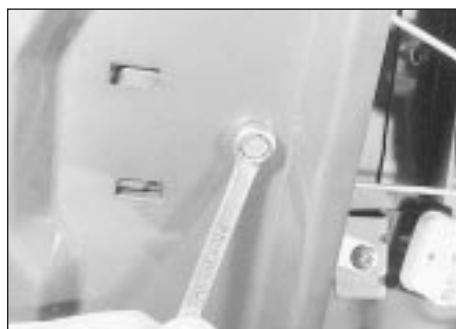
20.8 Unscrewing the tailgate lock motor securing bolt
