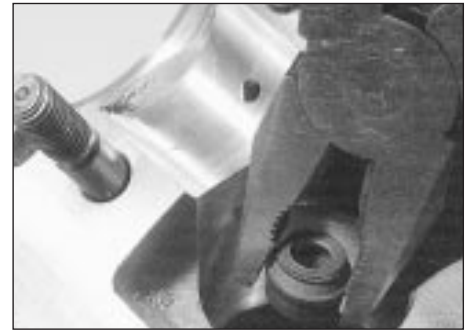
7.4f Remove the valve stem oil seal using a pair of pliers
