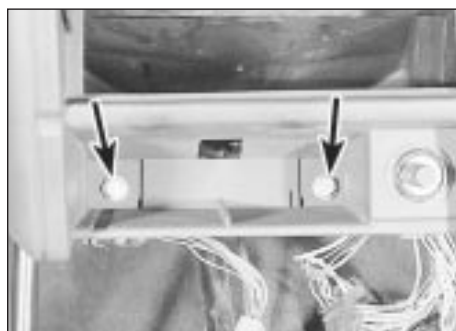
30.9a Remove the two bolts (arrowed) from the ashtray recess . . .
