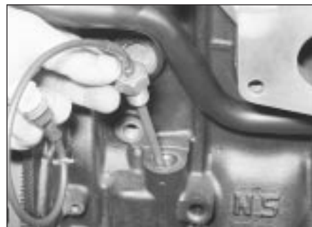
14.2 Removing the oil level sensor from the cylinder block
