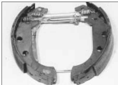
6.19b Rear view of early type Bendix shoe assembly correctly assembled - removed from backplate for clarity
