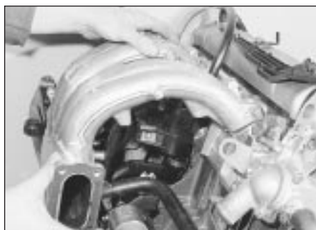
18.12c Fitting the inlet manifold
