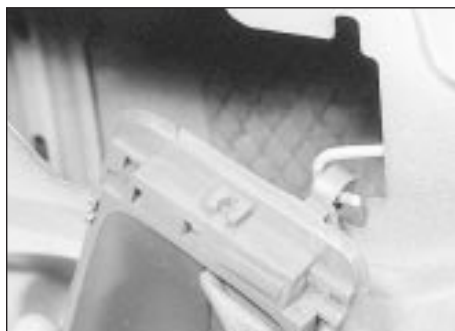
14.3 Unhooking the link rod from the interior door handle
