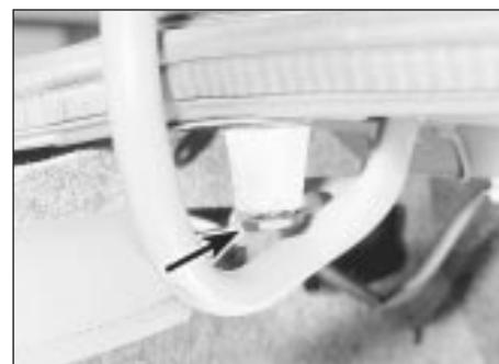
16.6 Rubber stop (arrowed) under boot lid hinge arm
