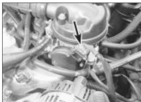
16.14 Throttle potentiometer wiring connector (arrowed)
