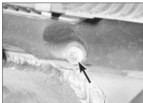
30.20 Fascia securing nut (arrowed) in scuttle
