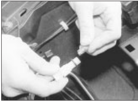
5.11 ... and withdraw the bulb
