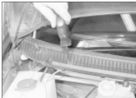
25.9 Unscrew the grille panel securing screws
