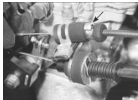
9.10 Choke cable-to-rubber collar retaining clip (arrowed)
