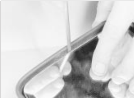
22.9 Releasing a mirror glass locking ring
