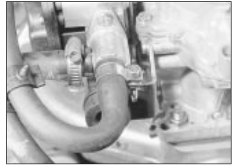
12.6a Automatic choke coolant pipe connection . . .
