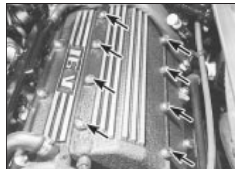
11.2 On 16-valve models undo the eight bolts (arrowed) and remove the access cover to reach the spark plugs
