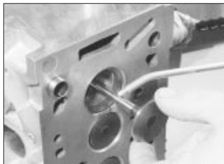
9.1 Lubricate the valve stems prior to refitting
