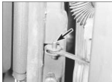
12.3 Drive the roll-pin (arrowed) from the door check strap
