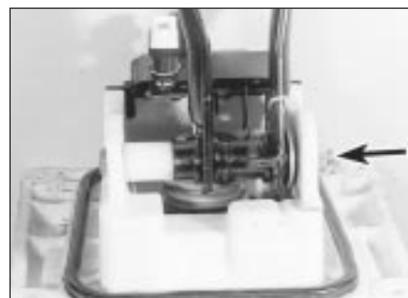
14.4 Pedal pivot bolt and nut (arrowed)
