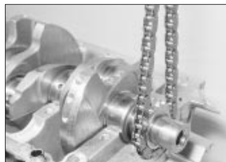
18.42 Refitting the oil pump drive chain and sprocket - TU aluminium block engine
