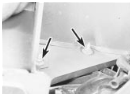
6.3 Front bumper front securing nuts (arrowed)
