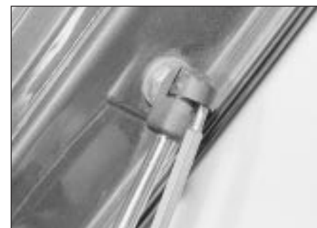
18.16 Prising the spring clip from a tailgate strut balljoint
