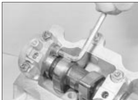
10.38a On early 1580 cc and 1905 cc models, slacken the retaining bolt . . .
