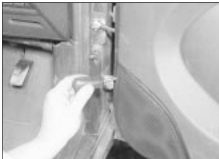
13.3 Removing a loudspeaker cover panel securing screw
