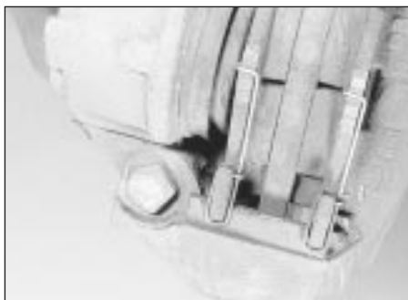
4.12a Correct location of the anti-rattle springs on Bendix brake pads
