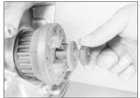
7.11a Remove the crankshaft sprocket retaining bolt ...
