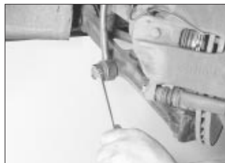
6.2 Remove the bolt securing the anti-roll bar drop link to the lower arm
