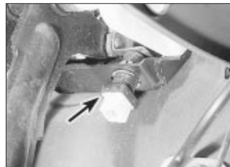
22.1 Stop-light switch (arrowed) on brake pedal bracket
