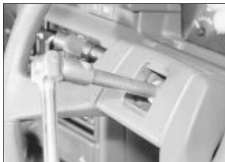
16.4 Unscrewing the steering wheel nut
