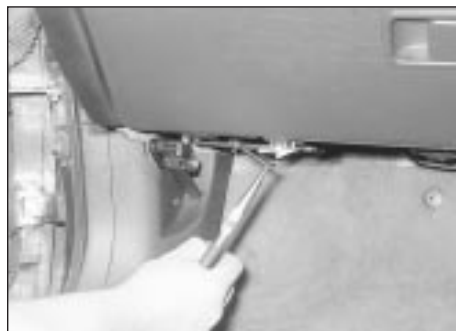
28.13 Remove the hinge pins . . .
