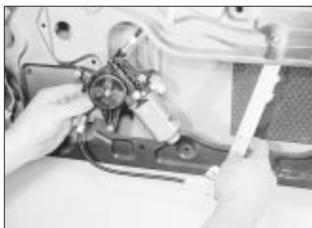
15.16 Removing the front door window regulator assembly
