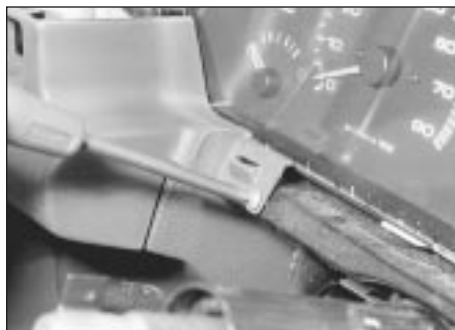
9.5 Removing the upper centre fascia panel securing screw - models up to 1992
