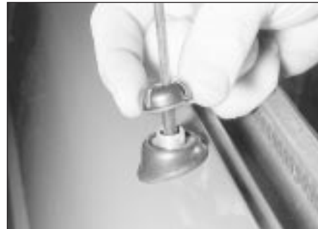
22.15a Unscrew the ring nut . . .
