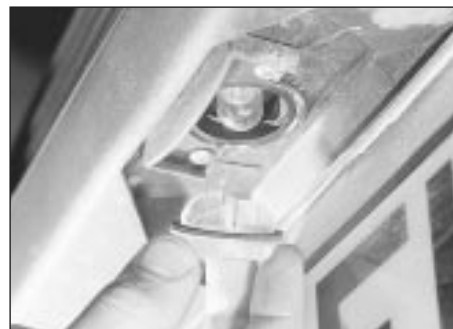
5.39 Prise the lens from the bumper . . .
