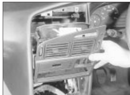
11.15 . . . then withdraw the housing
