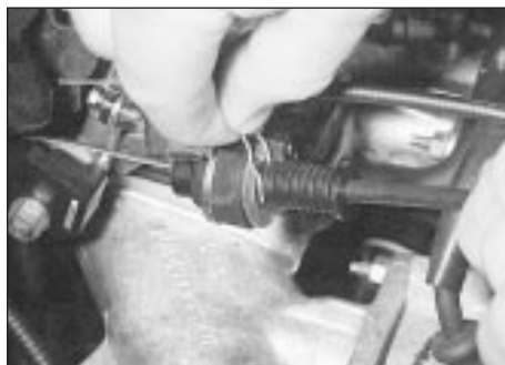
7.9 Adjusting the accelerator cable
