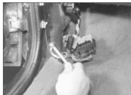
30.52 Unbolt the earth lead from the passenger's footwell
