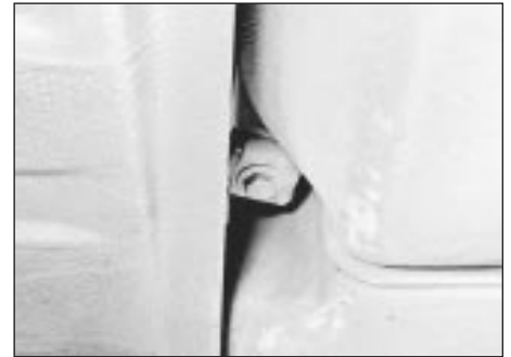
6.9 Fuel tank support strap bolt
