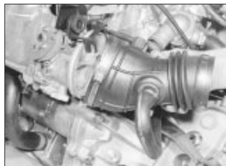
12.6 Detach the plastic duct
