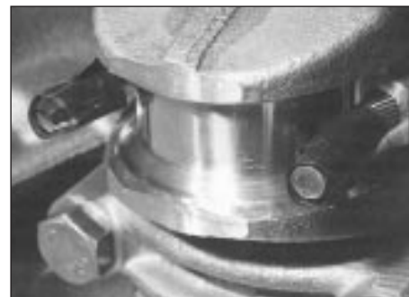
10.6 To protect the crankshaft journals, tape over the connecting rod stud threads prior to removal
