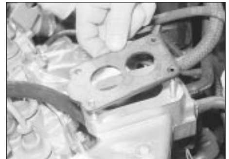
12.11 Removing the insulating spacer
