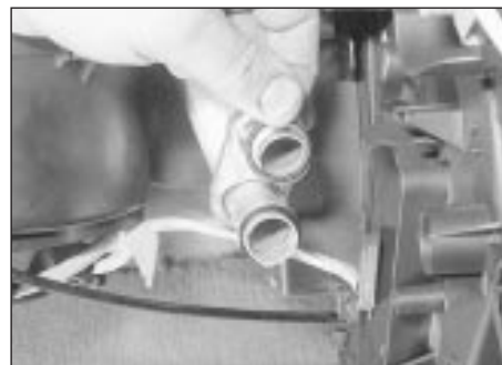
9.36c . . . and recover the O-rings from the pipe connections
