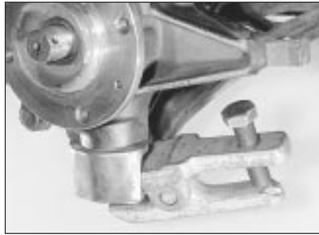
2.11 Release the lower balljoint using a balljoint separator tool
