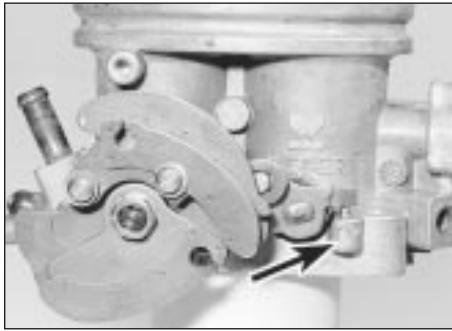
14.6a Secondary throttle adjusting screw (arrowed) . . .
