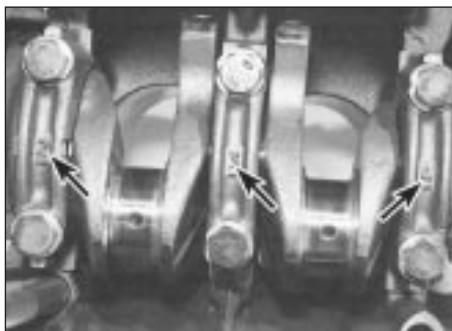
11.17 Main bearing cap identification markings (arrowed)
