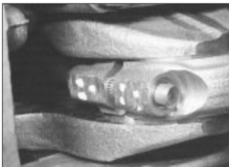
10.3 Connecting rod and big-end bearing cap marked for identification (No 3 cylinder shown)
