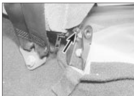
26.18b Split rear seat back inner pivot (arrowed) - Estate model
