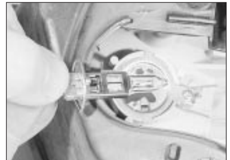
5.23b Removing a headlight-mounted driving light bulb
