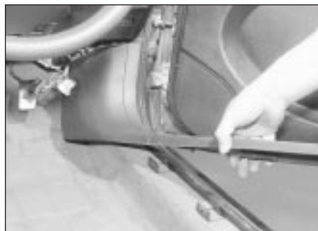
30.42b . . . then remove the footwell side trim panel
