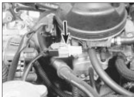
16.3 Injector wiring connector (arrowed)
