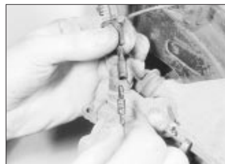
4.2 Disconnecting the pad wear sensor wiring connector
