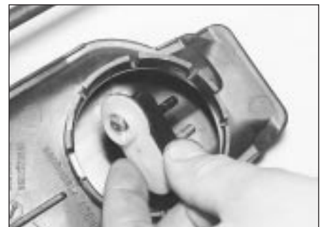
3.14c . . . then withdraw the vacuum switch from inside the duct
