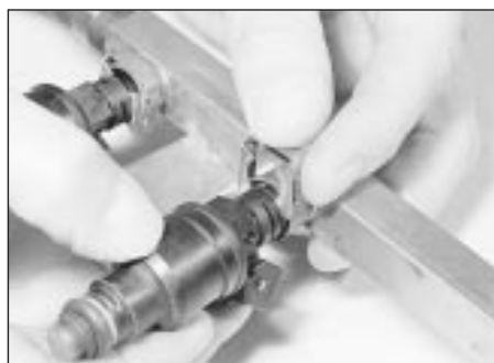
14.29 Removing an injector from the fuel rail
