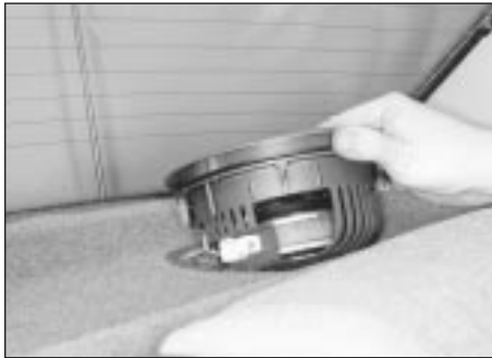
21.13 Removing the rear loudspeaker - Saloon models
