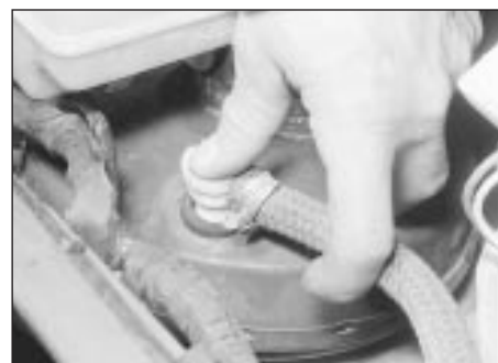
15.7 Pulling the vacuum check valve from the servo
