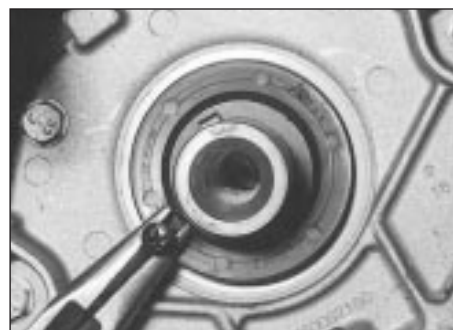
16.2 Using a self-tapping screw and pliers to remove the crankshaft oil seal
