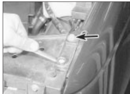
11.14 Unscrew the body front panel upper securing bolts
