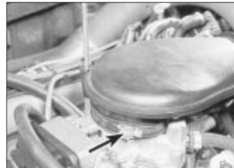
2.5 On the XU engine unscrew the bolt securing the air inlet duct, then loosen the clip
