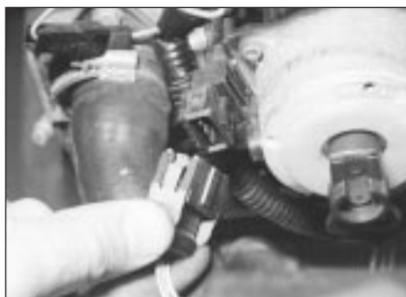
4.3a Disconnect the distributor wiring connector . . .
