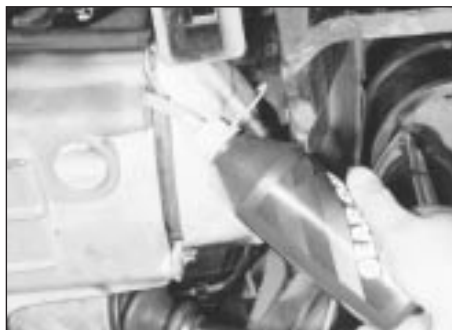
26.4 Topping-up the transmission oil level
