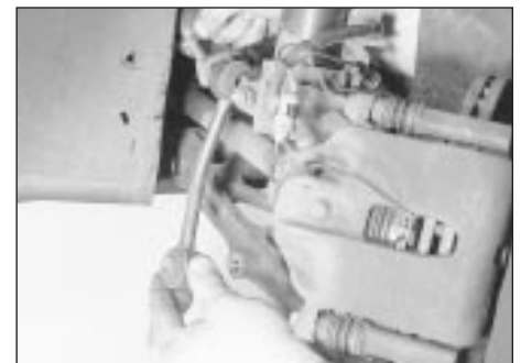
8.3 Removing an anti-roll bar drop link
