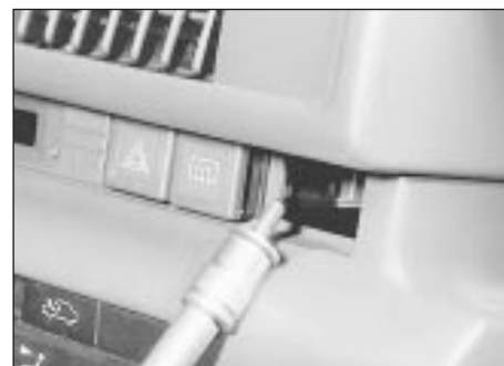
9.3a . . . and remove the visor securing screws
