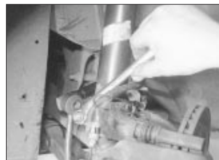
4.5 Unscrewing the hub carrier-to-suspension strut clamp bolt
