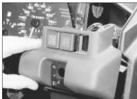
9.6 Withdrawing the driver's side upper fascia panel
