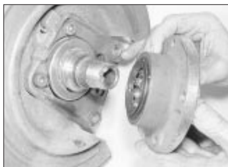
10.11a Fit the hub assembly . . .
