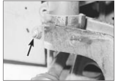
2.12 Hub carrier-to-suspension strut clamp nut (arrowed)
