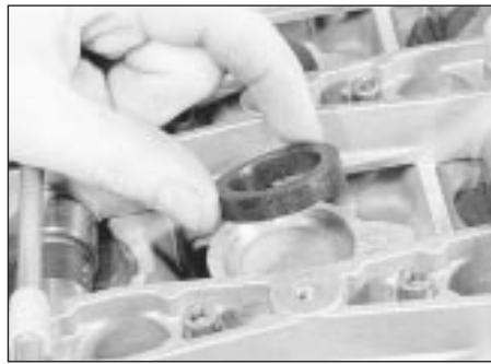
4.32 Fitting a spark plug hole oil seal
