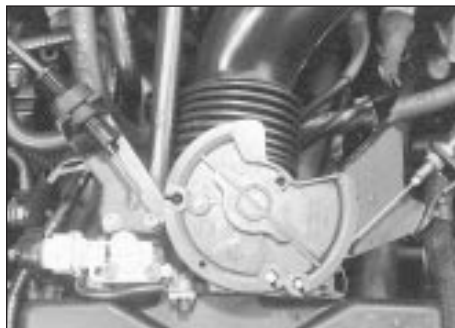
12.19 Accelerator cable and kickdown cable connections on the throttle housing (Magneti Marelli 8P fuel injection system)
