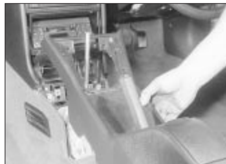
29.32b . . . and withdraw the console ("Lowline" console - models from 1993)
