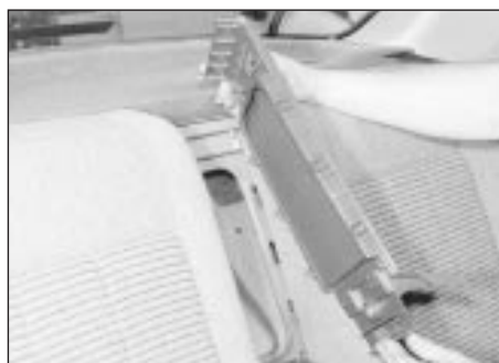
26.12b . . . and withdraw the armrest trim panel - Saloon model
