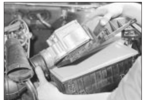
21.8 Lifting off the top cover
