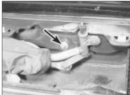
30.70 Fascia securing nut (arrowed) in scuttle
