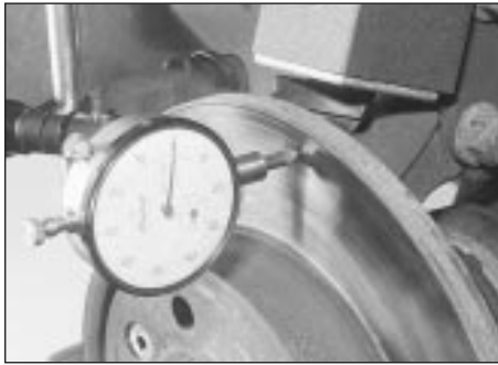
7.4 Checking disc run-out using a dial gauge
