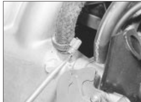
18.3 Disconnecting the brake servo vacuum hose
