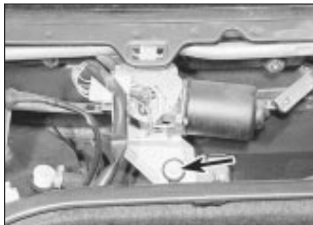
17.8a Windscreen wiper motor securing nut (arrowed)
