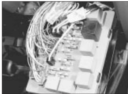
3.3b . . . and lower the fusebox panel - early models
