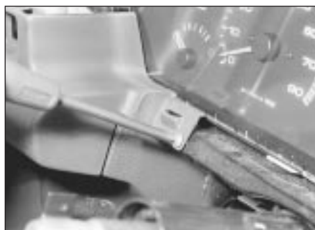
9.7 Remove the upper centre fascia panel securing screw
