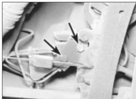
21.4 Rear brake pressure-regulating valve securing bolts (arrowed)
