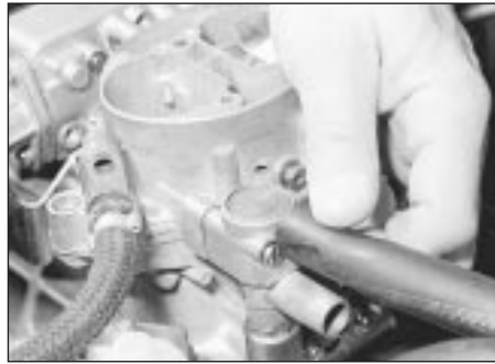
12.5 Disconnecting the float chamber breather pipe
