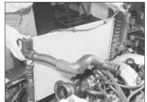
3.11 Lifting out the radiator
