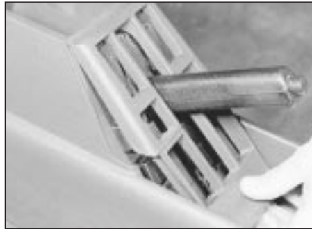
4.20 . . . then prise off the switch trim panel . . .
