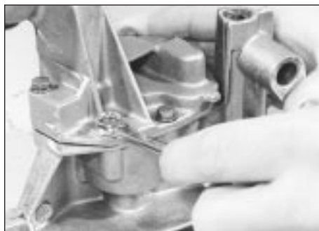
14.5a Remove the oil pump cover retaining bolts . . .
