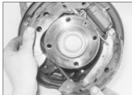
6.19a Fitting the brake shoes - early type Bendix brakes
