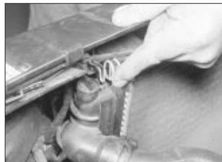
3.10 Releasing a radiator upper securing clip
