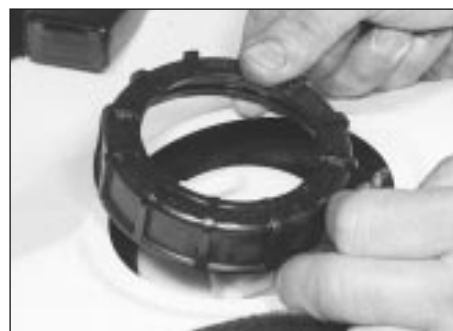
9.11 Unscrew the locking ring . . .
