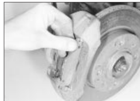
4.6 Withdrawing the outer brake pad - Bendix caliper
