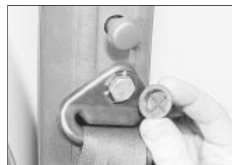
27.3 Removing the trim plate from the front seat belt upper anchor bolt
