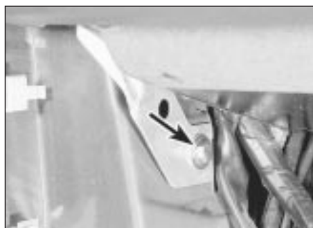
30.21 Lower fascia mounting bracket-to-footwell bolt (arrowed)
