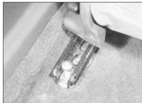
26.3 Front seat rear securing bolt partially removed
