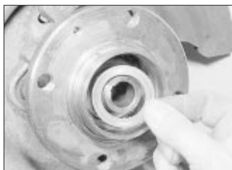
10.12a . . . and the thrustwasher
