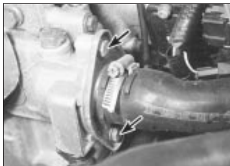
4.4a Thermostat housing cover retaining bolts (arrowed) - 1.4 litre engine
