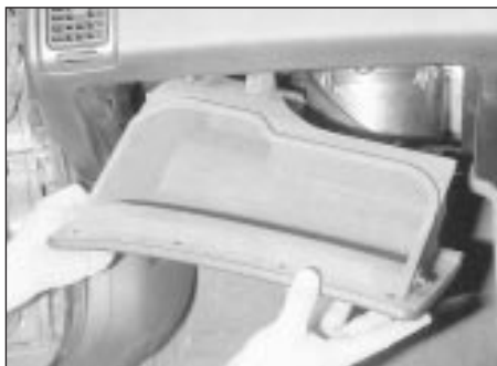
28.14 . . . and withdraw the glovebox - models from 1993
