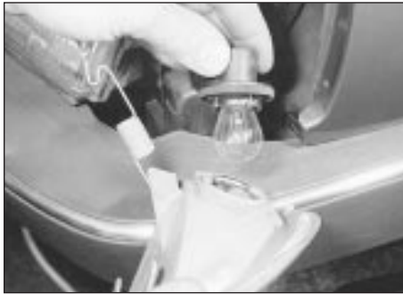
5.15 Withdrawing the bulbholder from the front direction indicator light
