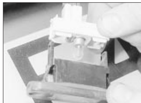
5.43 . . . and unclip the bulbholder from the lens - Estate model
