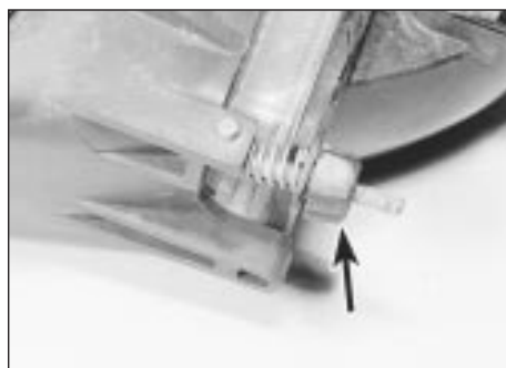
7.17 Unscrew the nut (arrowed) to separate the light from the cowl
