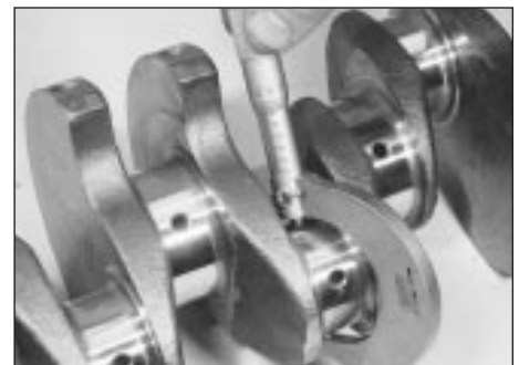
14.10 Measuring a crankshaft big-end journal diameter
