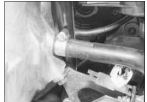
18.6 Supplementary air device air hose connection on inlet manifold
