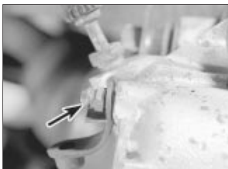
2.12a Bleed nipple (arrowed) on front disc caliper
