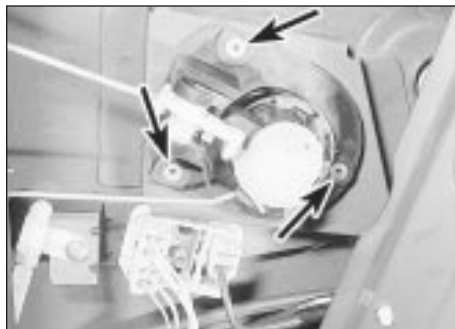
19.4 Tailgate lock cylinder securing rivets (arrowed)
