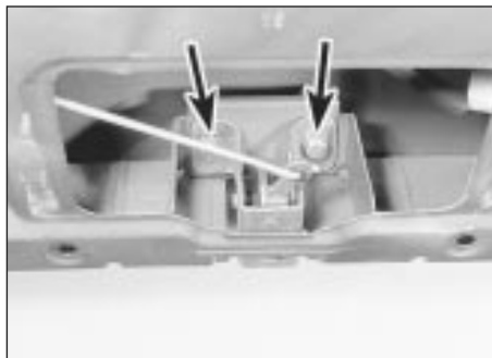
19.9 Tailgate lock securing bolts (arrowed)
