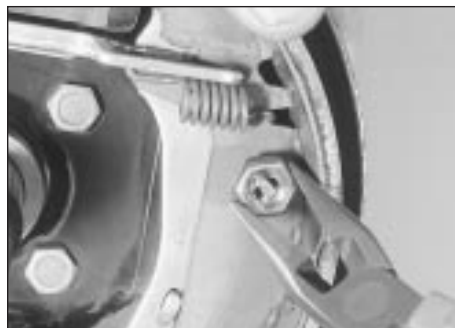
6.7 Removing a later type Bendix shoe retainer spring
