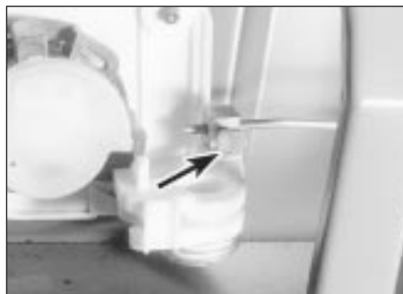
17.4 Unscrew the lock operating rod pinch-bolt (arrowed)
