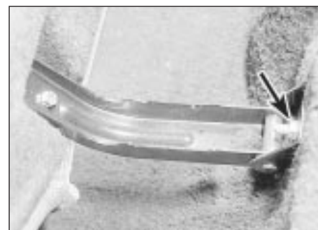
26.15 Rear seat cushion hinge securing nut (arrowed) - Estate model
