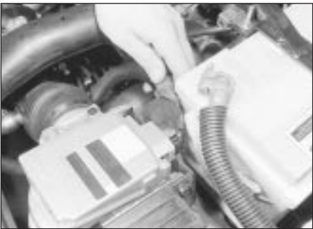
2.1 Disconnecting the airflow meter multi-plug (Bosch L3.1-Jetronic)
