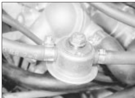
14.40 Fuel pump damper showing fuel hose connections
