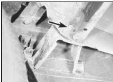
6.4 Front bumper side securing bolt (arrowed)
