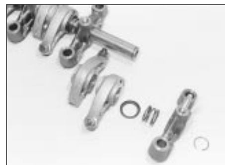
10.4 Remove the circlip, and slide the components off the end of the rocker arm
