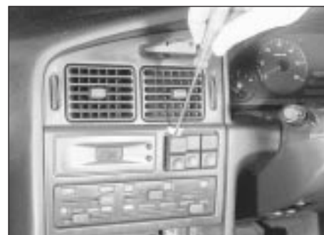
4.14 Prising out a fascia-mounted switch - models from 1993
