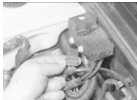
11.7c . . . and disconnect the plug from the terminal block - models from 1993
