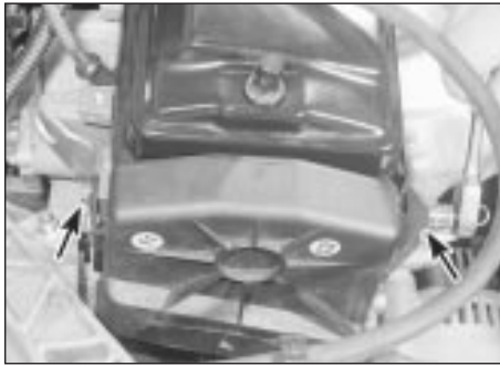
5.1a Undo the two retaining bolts (arrowed) . . .
