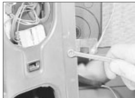
22.18b Unscrew the aerial motor securing bolt . . .
