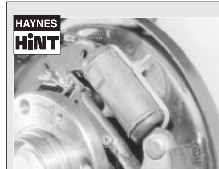
Restrain the wheel cylinder piston with a cable-tie or a strong elastic band
