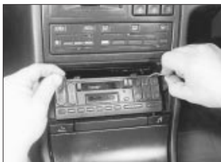
20.14 Insert the removal tools in the holes at the top of the radio/cassette player
