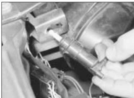
7.4 Removing a cable-operated headlight adjuster
