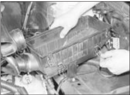
2.4 Removing the air cleaner housing
