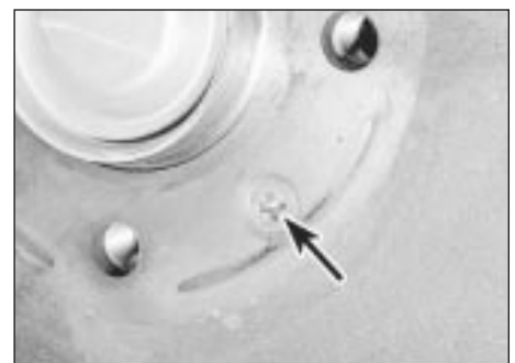
9.2 Rear brake drum retaining screw (arrowed)
