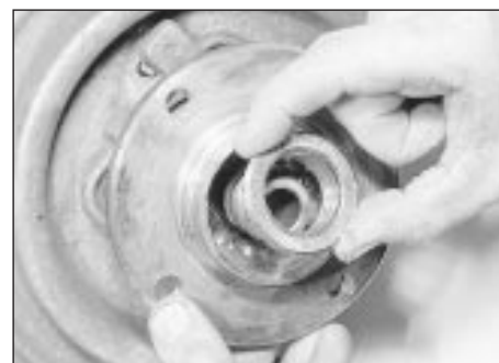
10.11b . . . followed by the outer bearing race . . .
