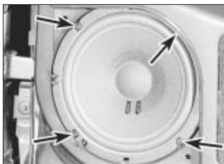
21.3 Door-mounted loudspeaker securing screws (arrowed)
