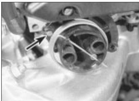
7.1a Accelerator cable connection on the throttle quadrant (arrowed)
