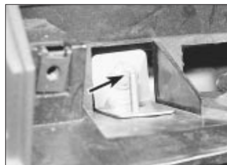
30.23 Upper fascia securing bolt (arrowed)
