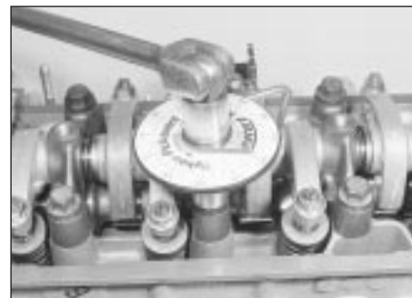
11.38 . . . then through the angle specified for stage 2
