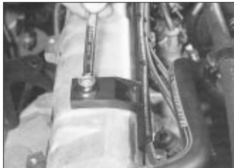
4.5 On 1580 cc and 1905 cc models, undo the retaining bolts/nuts and move the HT lead retaining clips clear of the head cover
