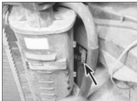
8.2b Headlight beam horizontal fine adjuster (arrowed)
