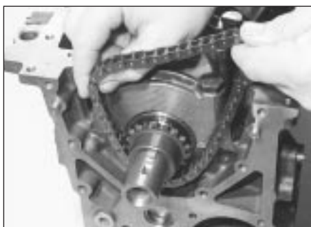
11.16a Remove the oil pump drive chain . . .
