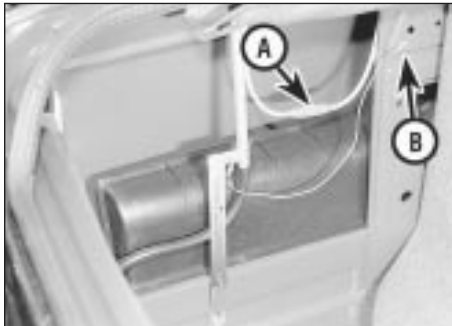
22.13 Aerial lead (A) and earth wire (B) - Saloon (rear wing-mounted manual aerial)
