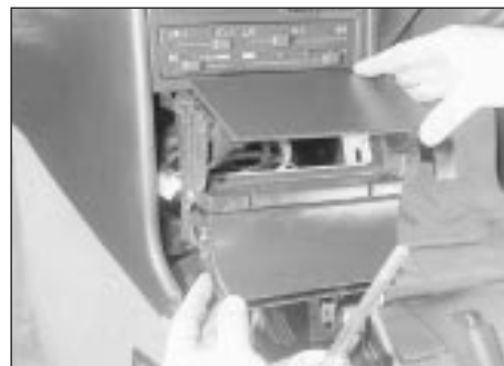
30.36b . . . then withdraw the housing
