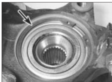
3.3 Front hub bearing retaining circlip (arrowed)
