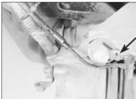
4.5a Extract the spring clip (arrowed) . . .
