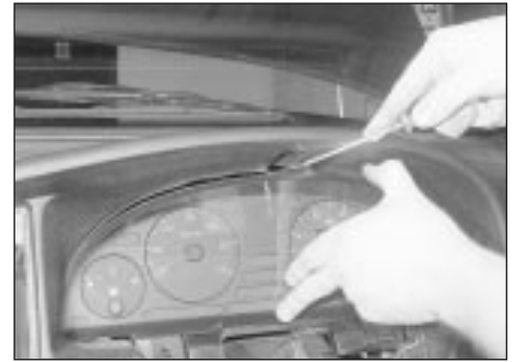
9.22 Lever the upper securing clip down . . .
