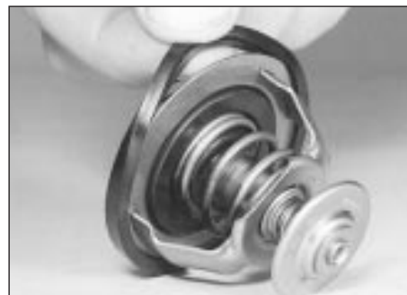
4.5 Removing the sealing ring from the thermostat flange
