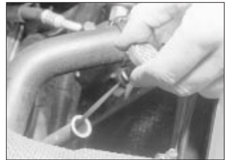
4.2a Withdrawing the automatic transmission dipstick
