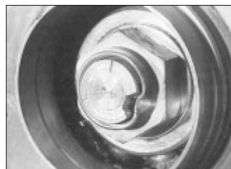
10.12c . . . stake the hub nut firmly into the stub axle groove
