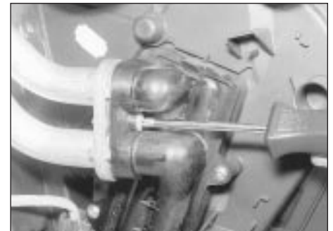
9.35 Remove the screw securing the heater pipes to the matrix connector
