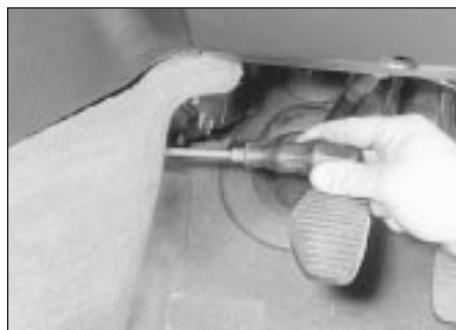
30.45a Remove the securing screws . . .
