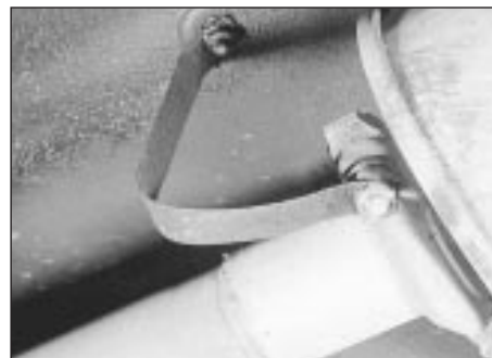
16.1 Exhaust-to-floor panel earth strap fitted to early models
