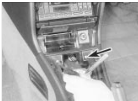
29.32a Remove the front securing screws . . .
