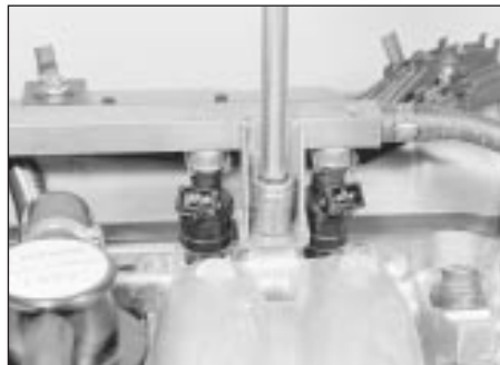
14.28a Removing a fuel rail bolt . . .
