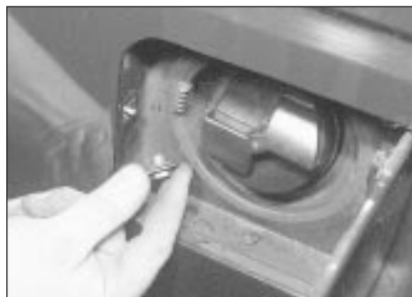
20.24a Remove the bolt securing the fuel filler flap lock motor to the body
