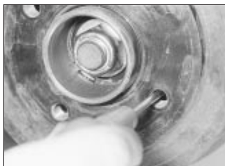
9.3b Releasing the handbrake operating lever
