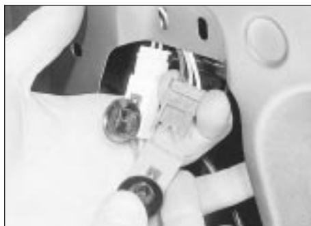
22.3 Disconnecting the door mirror wiring connectors
