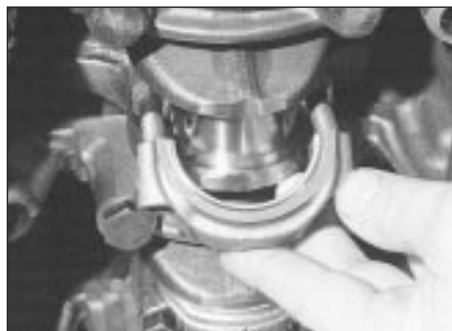
10.5 Removing a big-end bearing cap and shell
