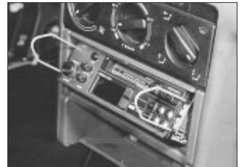
20.3 . . . then insert the removal tools . . .
