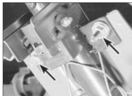
17.12 Steering column upper securing nuts (arrowed) - models up to 1992
