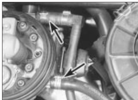
12.4 Fuel feed and return hose connections (arrowed) - later model shown
