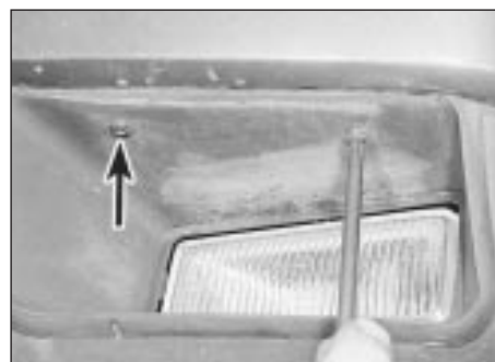
7.16 Remove the front driving light/foglight cowl securing screws
