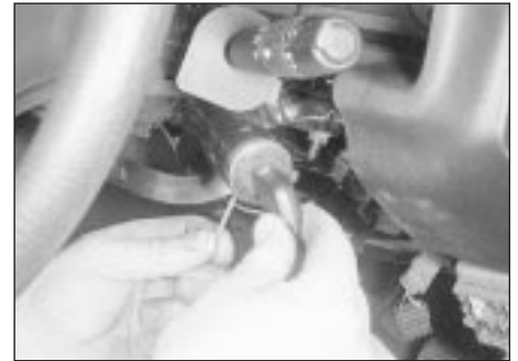
18.6 Depress the lock retaining lug, whilst pulling out the lock using the key
