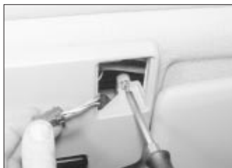
20.31 Removing a roof console securing screw
