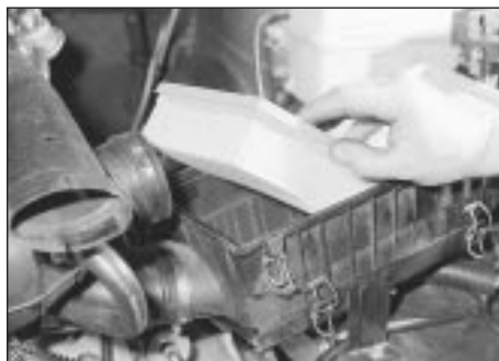
21.9 Removing the air filter element
