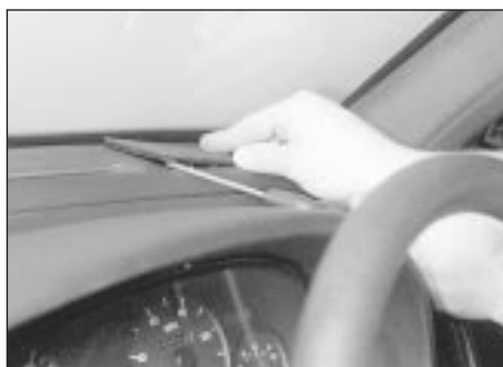
21.9a Prise the loudspeaker from the facia . . .
