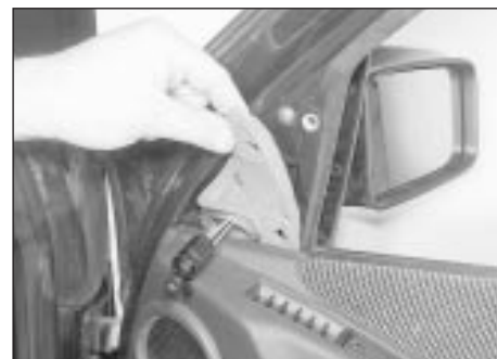
22.5a Prise off the sealing strip . . .
