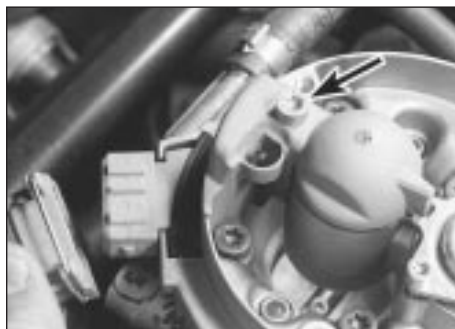
15.16 Disconnecting the injector wiring connector. Injector screw is arrowed
