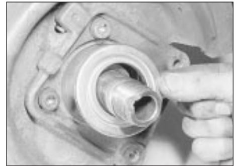
10.6c . . . and the oil seal support cup
