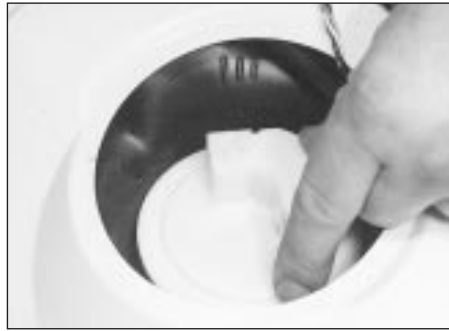
10.1 Removing the fuel gauge sender unit
