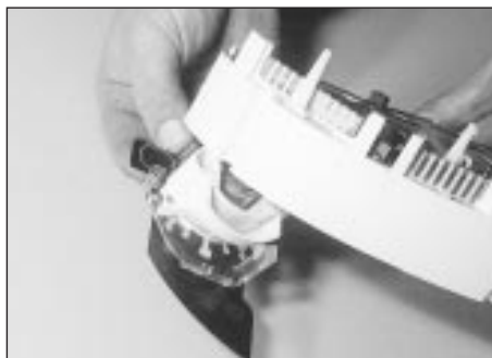
10.11a . . . then withdraw the gauge . . .
