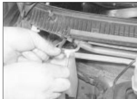
25.8 Disconnect the washer fluid hose
