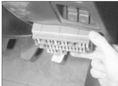
3.11b . . . to release the fusebox - models from 1993
