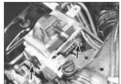
3.5a Undo the two retaining bolts (arrowed) . . .
