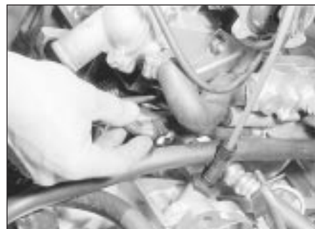
14.45 Disconnecting the supplementary air device plug
