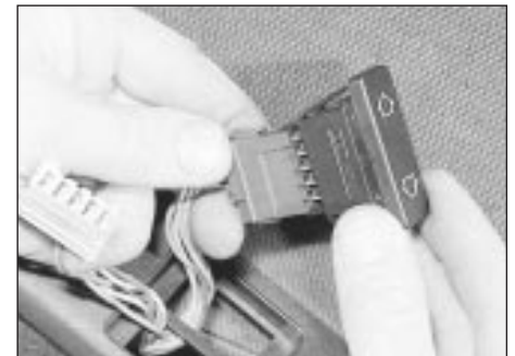
13.7 Removing an electric window switch from the door
