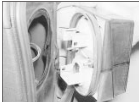
7.34b Withdrawing a rear wing-mounted light cluster - Estate model
