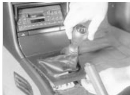
29.31 Removing gear lever gaiter surround ("Lowline" console - models from 1993)
