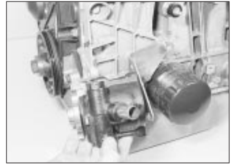
22.9b . . . and remove the pump - XU5 and XU9 engines (engine removed for clarity)
