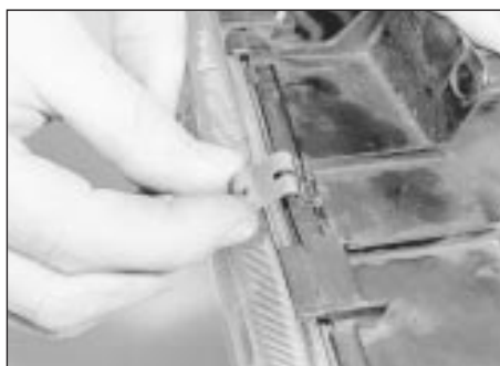
7.9 Removing a headlight lens securing clip
