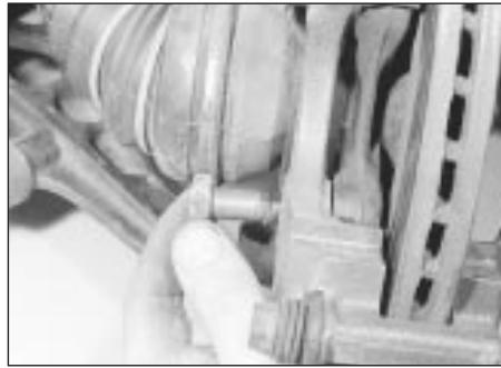
7.7 Removing a Girling caliper mounting bracket bolt
