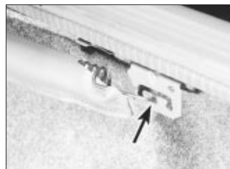
16.2 Note which slots (arrowed) the ends of the boot lid assister springs are positioned in before disconnecting them
