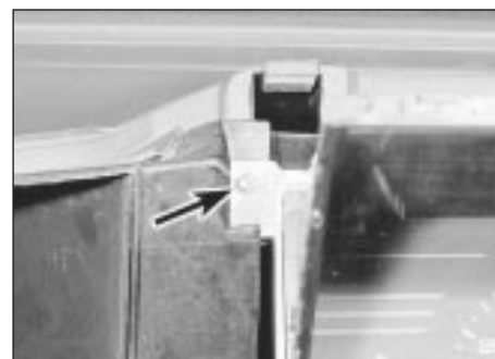
9.8 Instrument panel securing screw (arrowed)
