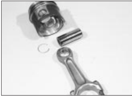
13.15c Piston and connecting rod components
