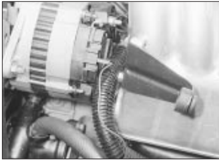
7.2 Connections on the rear of the alternator
