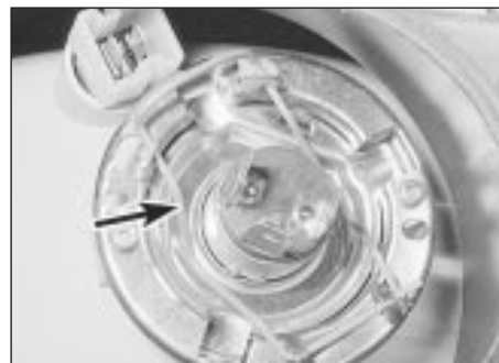
5.4a Release the spring clip (arrowed) . . .
