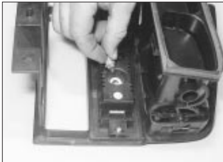
6.23 Removing the clock illumination bulb - models from 1993
