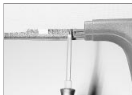
27.2 Removing an upper B-pillar trim panel top securing screw
