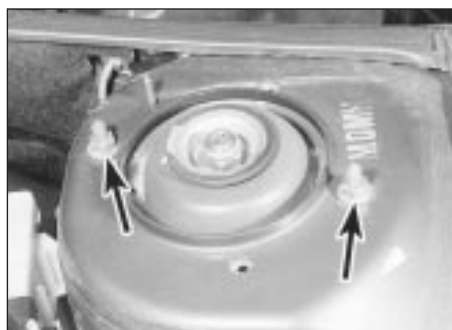
4.2 Suspension strut top mounting nuts (arrowed)
