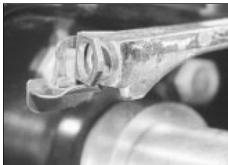
6.13 Correct fitted position of later type Bendix adjuster strut components
