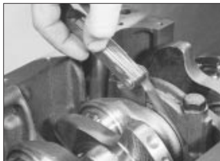
14.3 Checking crankshaft endfloat using feeler gauges
