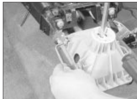
30.67 Unscrew the centre fascia lower securing bolts
