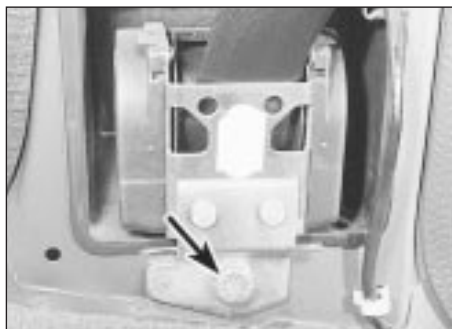
27.7 Front inertia reel securing bolt (arrowed)
