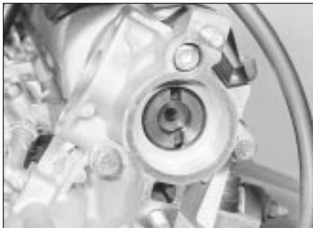
4.10 Off-set drive slots on the camshaft
