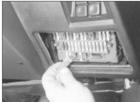
3.7 Removing a fuse using the plastic tool
