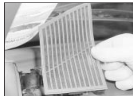
21.6 Remove the loudspeaker cover panel from the top of the facia . . .
