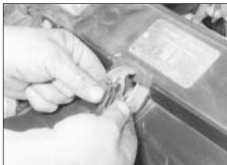
25.4 Push out the bonnet release lever securing pin
