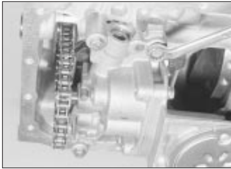
13.2 Oil pump is retained by three bolts
