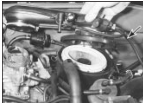
2.2b . . . and remove the duct, disconnecting the air temperature control valve hose (arrowed)
