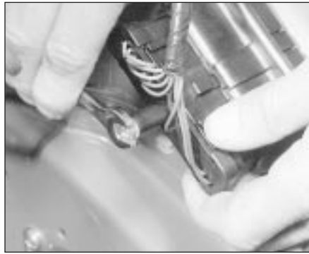
6.18 Unscrewing the ESC module wiring plug securing screw
