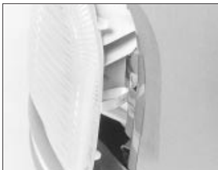
7.10 Release the direction indicator side spring clip
