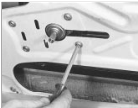
14.40a Removing the regulator retaining screws
