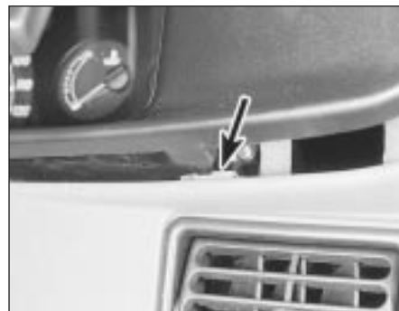
9.8 Bezel lower retaining clip (arrowed) - 1986 models onwards
