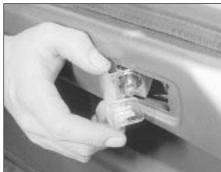
6.11 Removing the load space lamp
