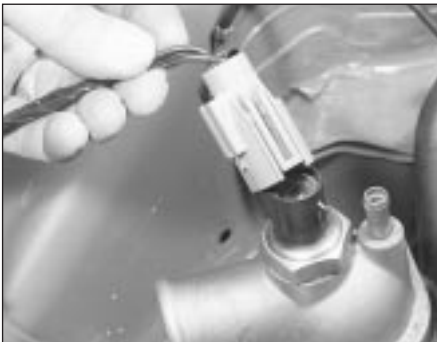
11.49a Disconnecting the cooling fan thermal switch . . .
