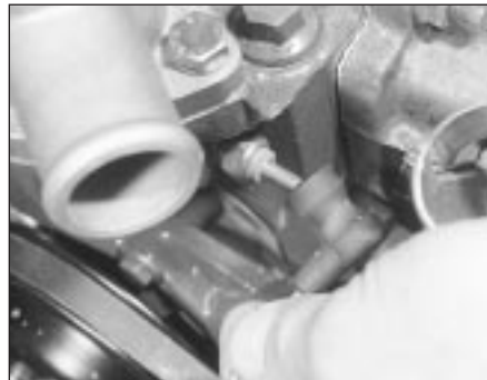
11.49b . . . and coolant temperature sender - HCS engine
