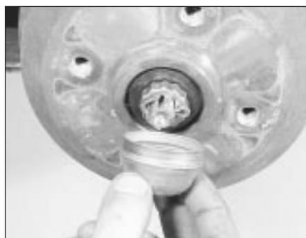
5.3a Remove the rear hub dust cap . . .
