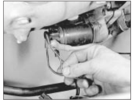
8.2 Disconnecting the wiring from the starter motor solenoid
