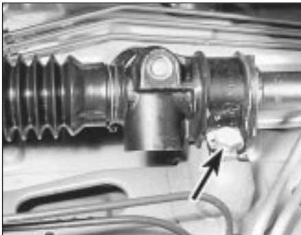
26.6a Steering gear-to-bulkhead mounting retaining bolt and locktab (arrowed)
