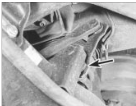
13.3 Anti-roll bar-to-lower arm shackle attachment (arrowed)
