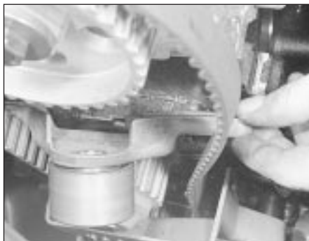
5.19 Removing the timing belt tensioner - CVH engine
