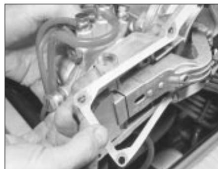
34.12 Locating the sensor unit gasket
