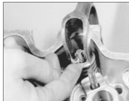
13.38 Compress the spring and fit the collets
