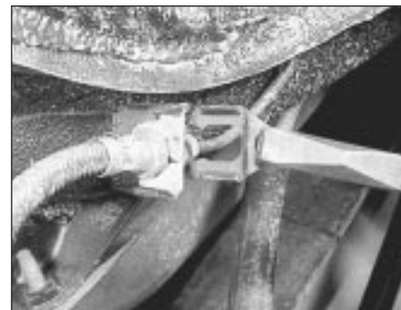
15.1 Removing a flexible hose spring anchor clip
