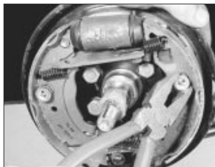
5.6 Removing the brake shoe hold-down washer and spring
