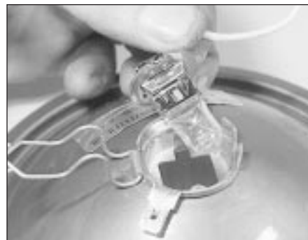
5.18 Removing the auxiliary lamp bulbholder
