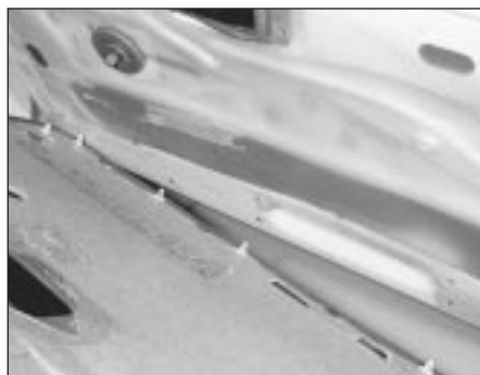
11.6 Removing the door trim panel
