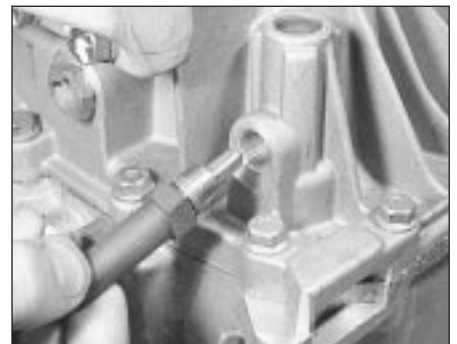
16.5 Fitting the selector shaft cap nut, spring and interlock pin
