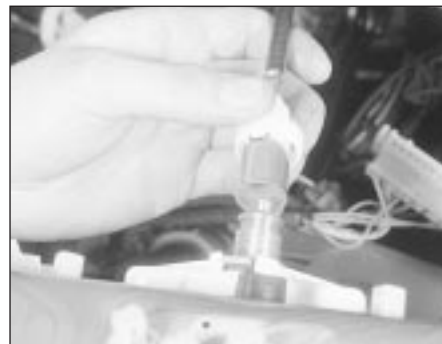
9.10 Disconnecting the speedometer cable
