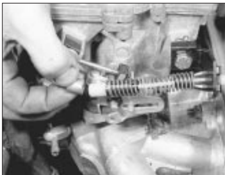
11.9 Disconnecting the throttle cable end (1.3 litre carburettor engine)
