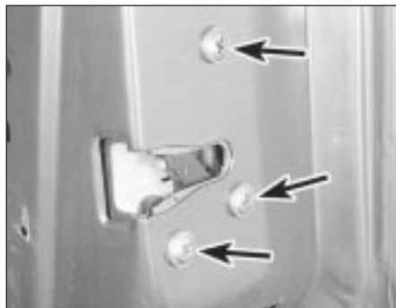
13.14 Door lock retaining screws (arrowed)
