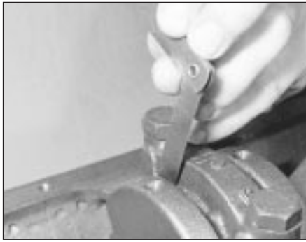
15.9 Using feeler blades to check crankshaft endfloat
