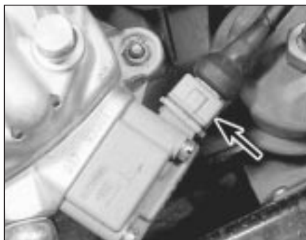
10.29 Pressure actuator wiring multi-plug (arrowed) - KE-Jetronic system
