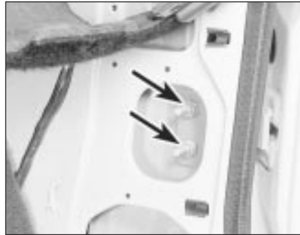
12.7a Front door lower hinge nuts (arrowed)
