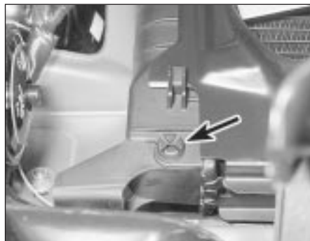
33.3 Radiator drain plug location (arrowed)
