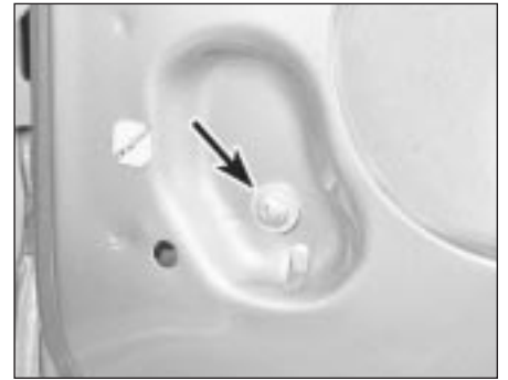
14.5 Glass run extension retaining screw (arrowed)
