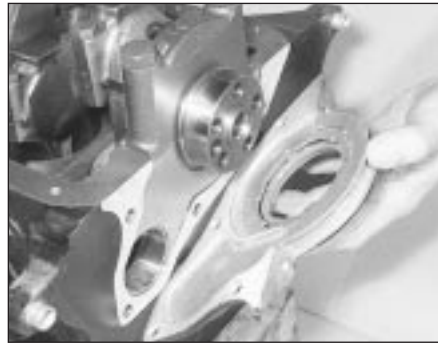
15.17 Fitting the crankshaft rear oil seal retainer
