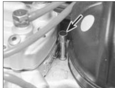
10.21 K-Jetronic system mixture adjustment screw location (arrowed)
