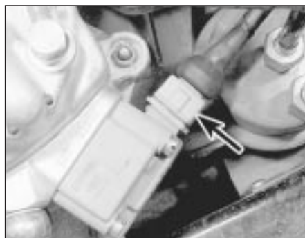
15.5 Pressure actuator wiring multi-plug (arrowed)
