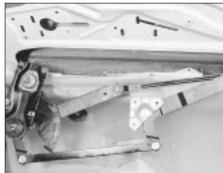
14.41 Withdrawing the window regulator
