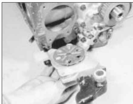
15.18 Fitting the water pump
