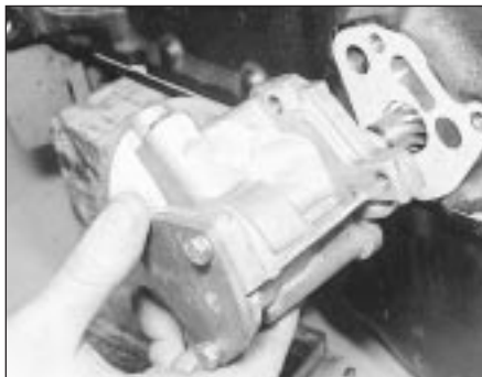
10.3 Removing the oil pump
