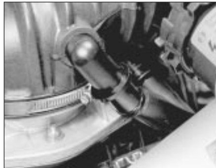
34.7 Detach the shut-off valve hose - K-Jetronic system
