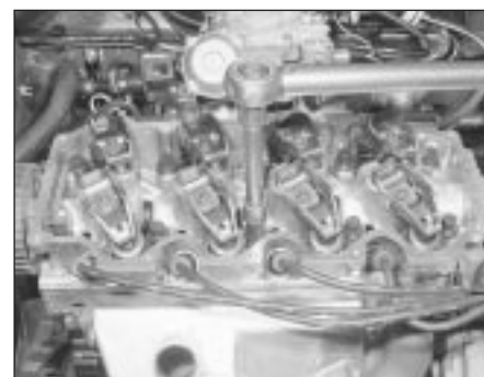
7.23b Tightening the cylinder head bolts
