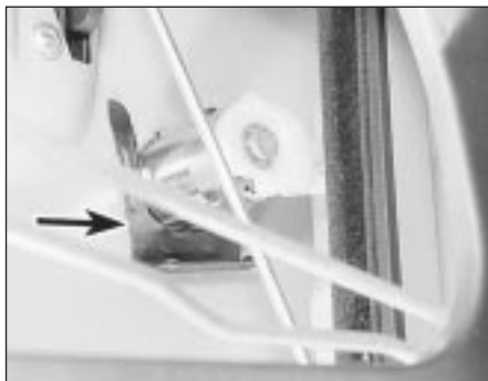
13.13 Door lock cylinder retaining clip (arrowed)
