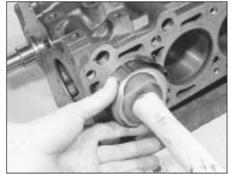
9.13b Installing a piston/connecting rod assembly
