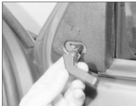
19.5b Removing the remote control handle
