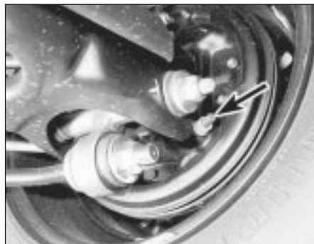
8.5 Handbrake adjustment plunger location (arrowed) on backplate
