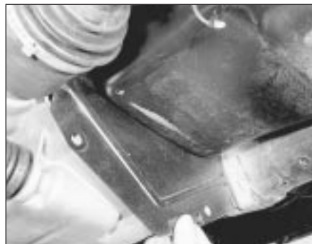
8.5 Remove the clutch housing cover plate
