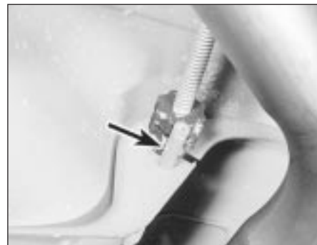
8.14 Handbrake cable adjuster nylon locking pin (arrowed)
