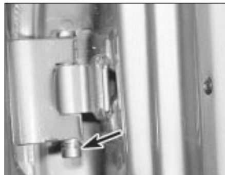
12.10a Front door upper hinge pin (arrowed) on 1986 models onwards
