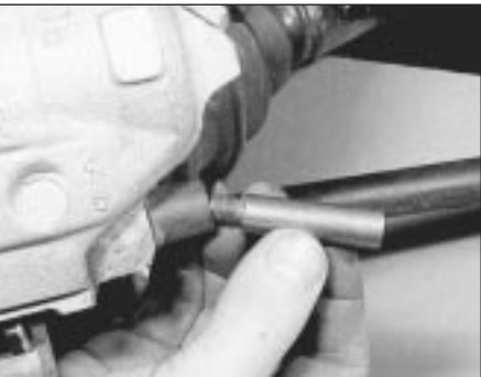
2.4b ... and withdraw the bolt from the anchor bracket
