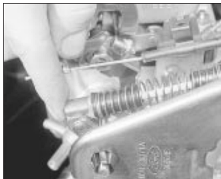
7.12 Release the cable end fitting spring retaining clip
