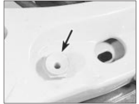
7.8 Bonnet bump stop (arrowed)
