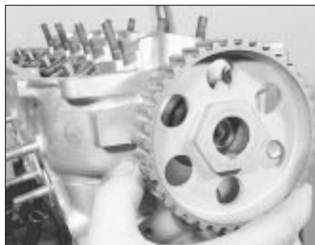
6.12 Removing the camshaft sprocket
