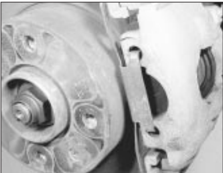
2.3 Disc pad retaining clip
