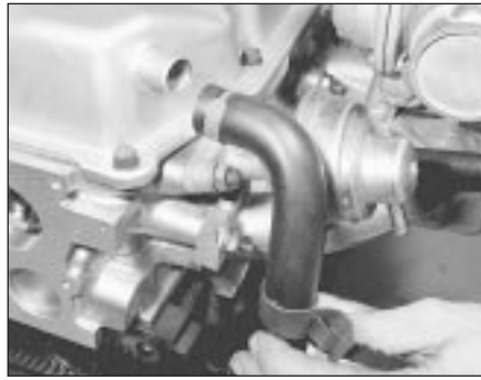
15.27a Connecting the crankcase rear ventilation hose ...
