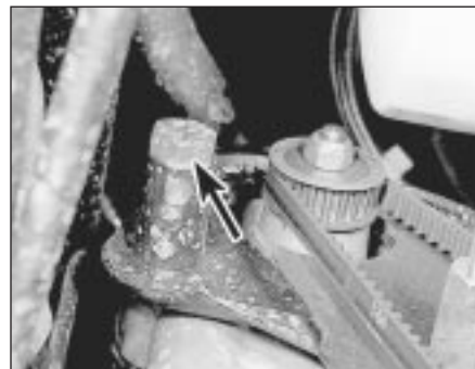
20.5 Modulator adjuster bolt (arrowed)
