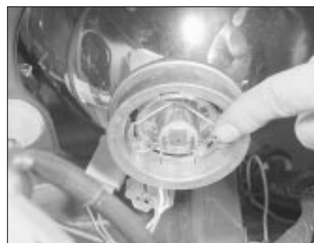
5.2 Releasing headlamp bulb spring clip arms
