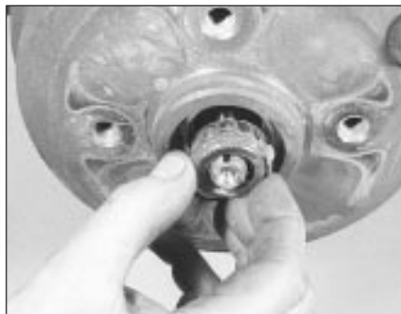
9.6 Rear hub outboard bearing removal
