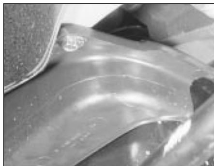
11.25a Remove the right-hand splash shield . . .
