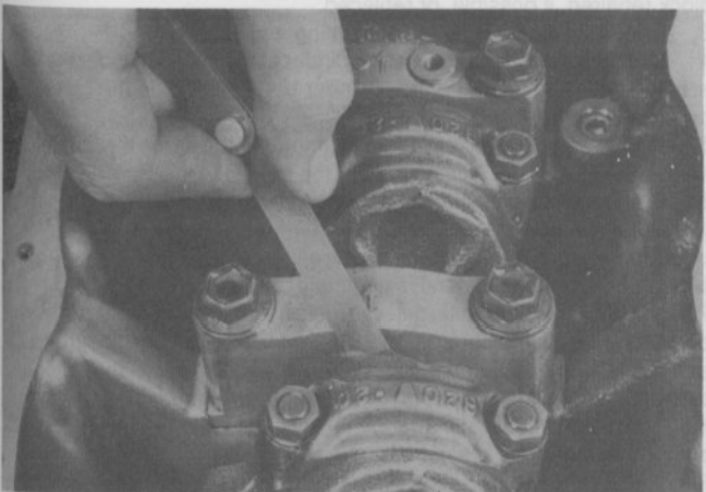
13.3 Checking crankshaft endplay with a feeler gauge
