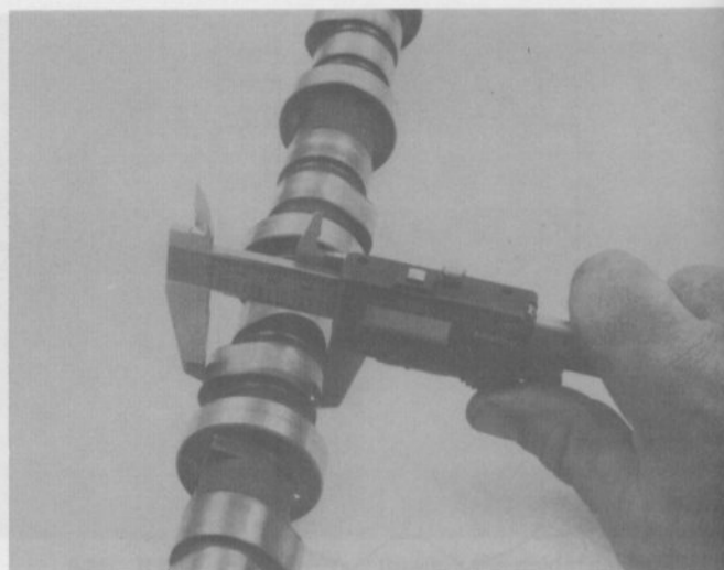
9.25 Measure the height of each lobe – if any lobe height is less than the specified minimum, replace the camshaft
