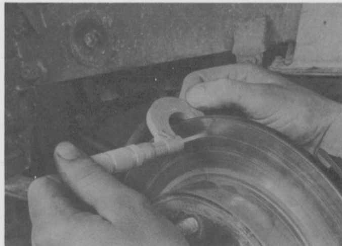
5.5 Use a micrometer to measure disc thickness
