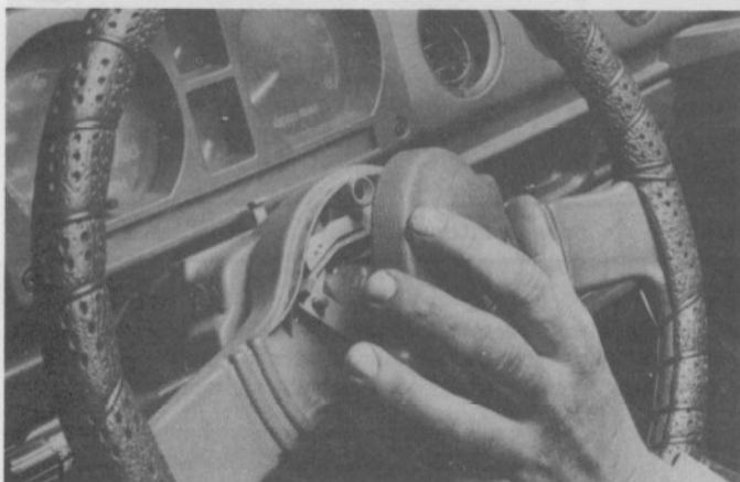
15.2 To remove the horn pad, pull it straight off the wheel
