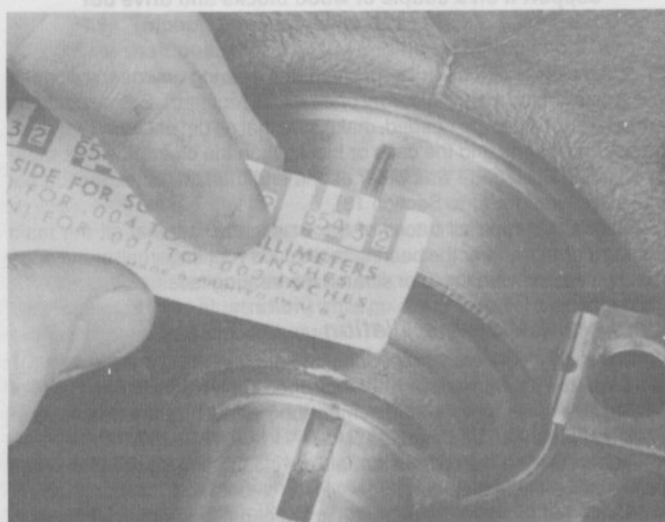
22.15 Compare the width of the crushed Plastigage to the scale on the envelope to determine the main bearing oil clearance (always take the measurement at the widest point of the Plastigage); be sure to use the correct scale – standard and metric scales are included
