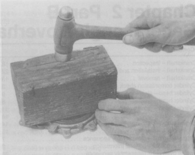
16.6 Drive the new seal into the retainer with a block of wood or a section of pipe, if you have one large enough – make sure that you don't cock the seal in the retainer bore
