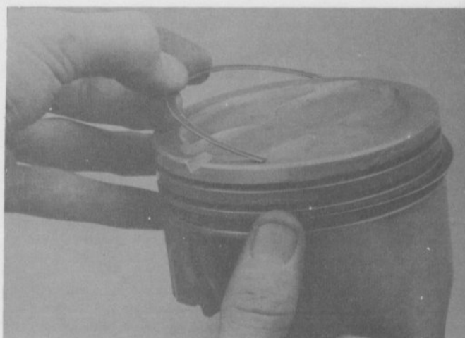
21.9b DO NOT use a piston ring installation tool when installing the oil ring side rails
