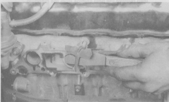
5.10 Remove all traces of old gasket material – scrape gently to avoid gouging the aluminum
