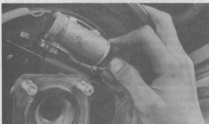
18.15 Carefully peel back the rubber boots on both sides of the wheel cylinder – if there's any brake fluid behind the boots, the wheel cylinders must be rebuilt or replaced
