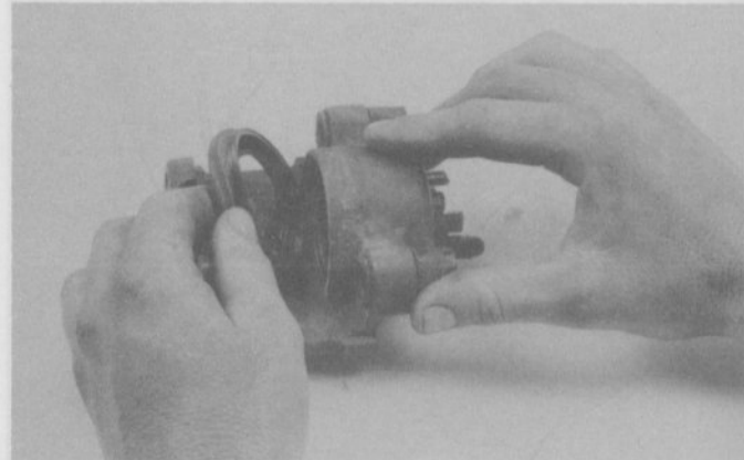
4.9 Remove the dust boot from the caliper
