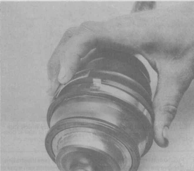
16.17a To install the new clamps, bend the tang down and ...
