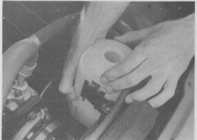
6.2 The coolant reservoir slips off/onto the bracket
