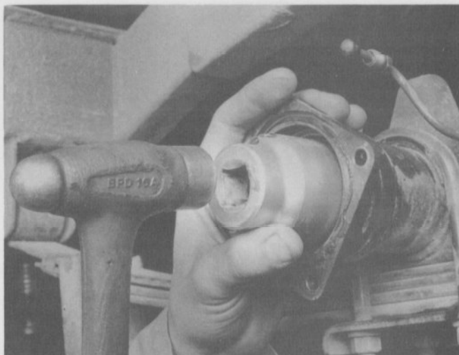
20.4 To install the axle seal, use a large socket, piece of pipe or seal installation tool
