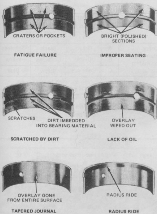
19.1 Typical bearing failures
