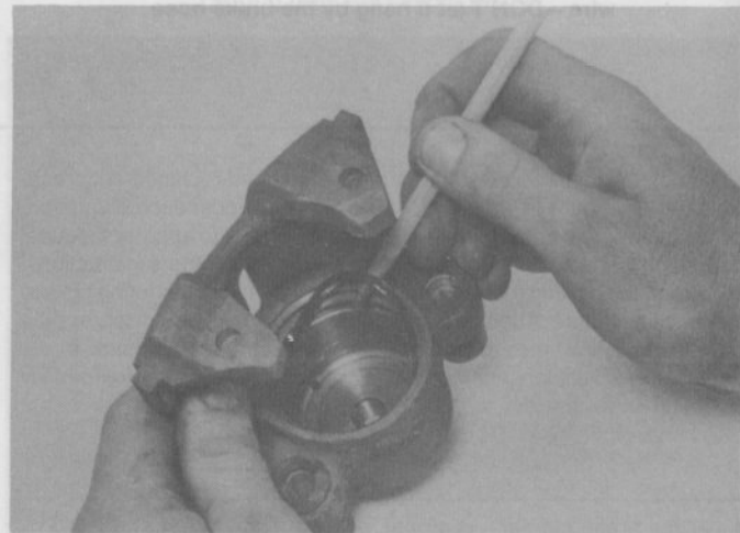
4.10 The piston seal should be removed with a plastic or wooden tool to avoid damage to the bore and seal groove – a pencil will do the job
