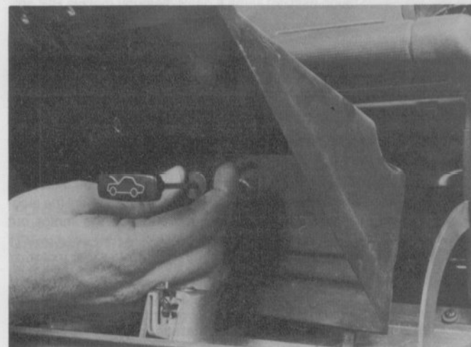
13.6 Remove the glove box with the hood latch cable
