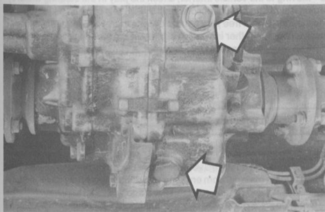
20.1a On Samurai models, locate the two transfer case plugs – the upper one is used for checking and refilling and the lower one is used for draining
