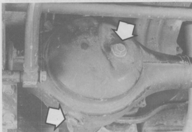
21.2a Front differential check/fill plug and drain plug locations
