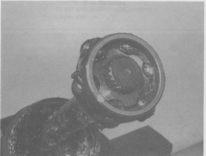
16.7 Apply match marks to the bearing to identify which side faces out during reassembly
