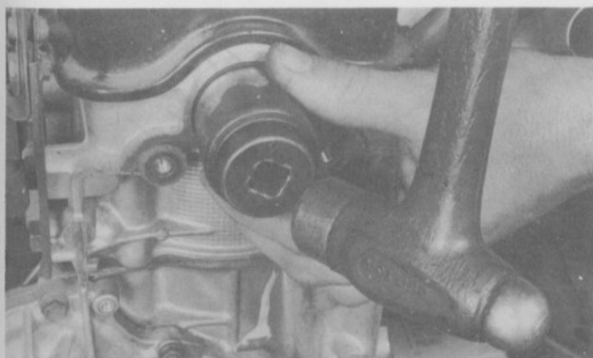
10.4 Gently tap the new oil seal into place with a socket and a small hammer
