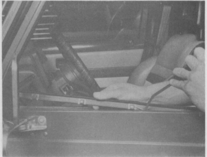
17.2 Locate the molding clips and pry them up to remove the molding pieces
