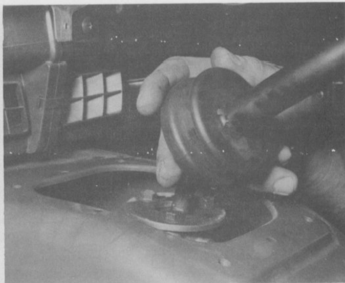
3.4 Pull the small inner boot up off the lever retainer
