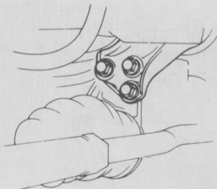
15.16 Remove the three right hand mounting bolts when removing the front axle housing
