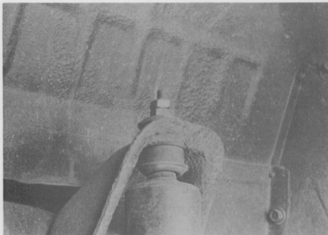
3.2 When removing the front shock absorber, remove the locknut first then the stem nut – it may be necessary to hold the stem with an open end wrench or locking pliers to prevent it from turning
