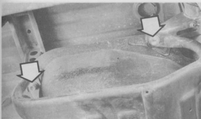
6.8 The fuel tank and skid plate are secured to the underside of the vehicle with four bolts (one at each corner)
