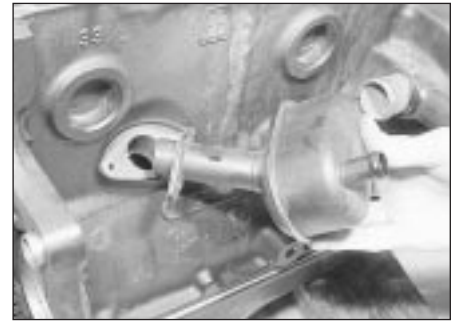
22.8 Crankcase ventilation system oil separator - 1.3 litre engine
