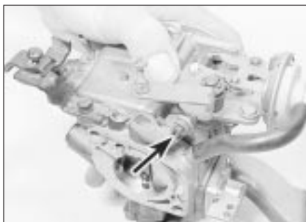
12.4 Fast idle adjusting screw (arrowed)
