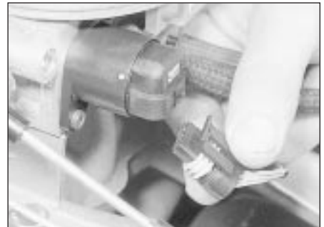
11.11a Detach the wiring connector . . .
