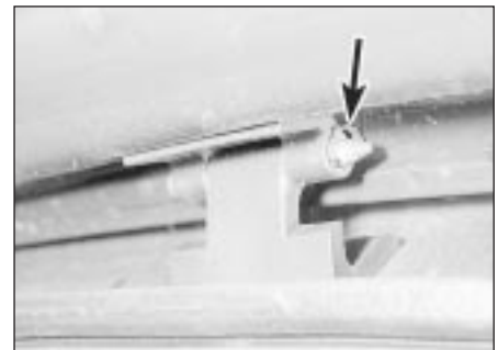
20.4 Tailgate hinge showing circlip (arrowed)
