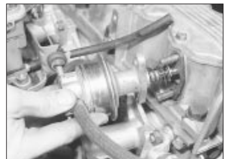
5.5 Removing the fuel pump (1.3 litre engine shown)
