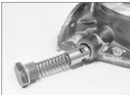
14.5 Oil pressure regulator valve components
