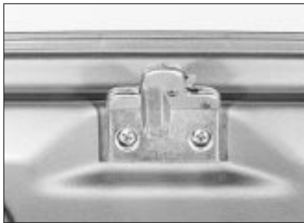
26.2 Boot lid lock securing screws
