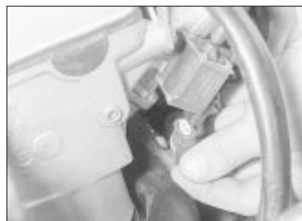
12.100 Disconnecting the vent valve multi-plug
