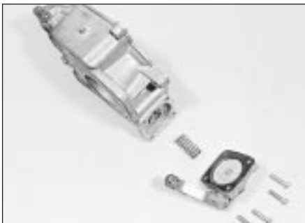
19.9 Accelerator pump components
