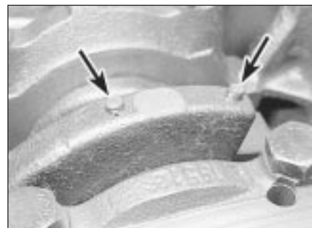
20.7 TDC sensor contact pins (arrowed) in crankshaft web
