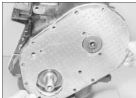
18.4b Removing the engine front plate
