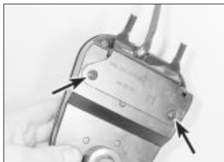
21.13a Undo the retaining screws and remove the mounting bracket . . .
