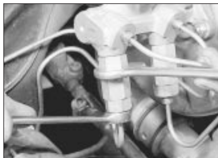
13.3 Slackening the brake pipe union from the pressure regulating valve
