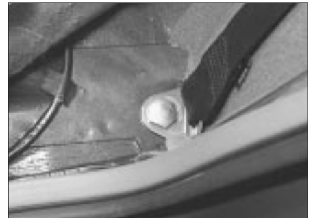
37.7c Rear seat belt floorpan mounting
