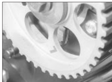
10.4 Exhaust camshaft sprocket is marked 'L'
