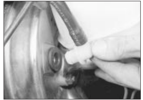
15.3 Brake servo vacuum connection at servo
