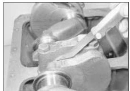
20.18 Checking the crankshaft endfloat
