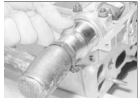
9.4b Seating a camshaft oil seal
