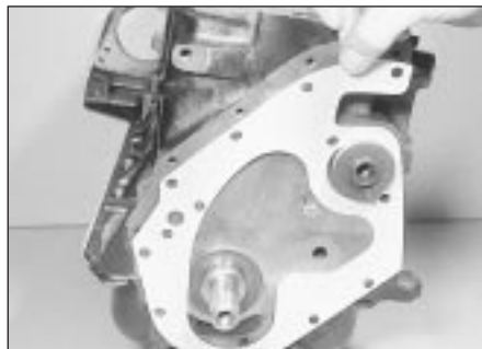
18.10 Fitting a new front plate gasket
