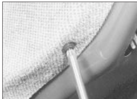
12.7 Trim securing screw on the door shut face - rear door shown
