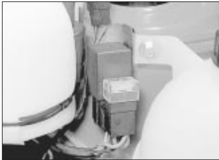
3.7a Headlamp washer relay and fuse
