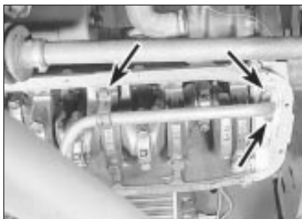
13.4 Oil pick-up pipe retaining bolts (arrowed)
