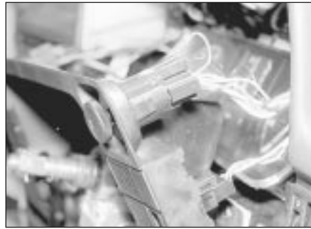
8.5 Withdrawing the instrument panel surround
