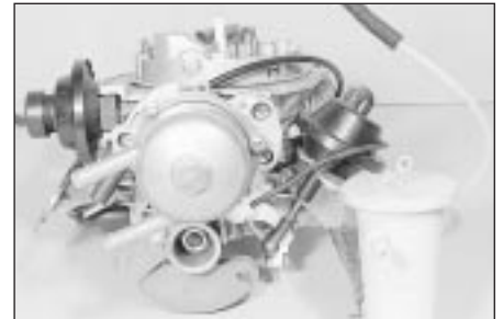
22.2b 2E3 carburettor - choke cover side view
