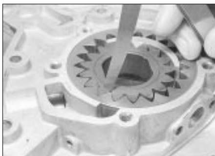
14.2 Checking oil pump gear teeth backlash
