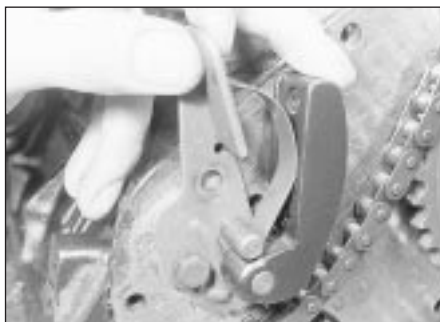
14.19a Fit the tensioner lower bolt . . .
