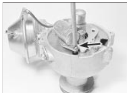
7.5 Undoing the condenser retaining screw
