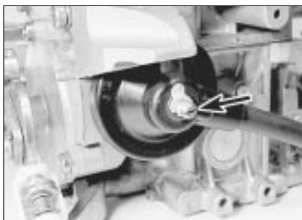
14.8a Choke valve gap adjustment screw (arrowed)
