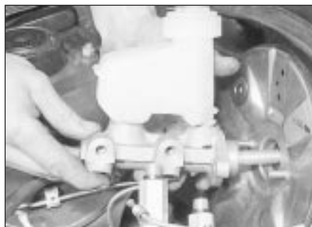
13.5 Removing the master cylinder
