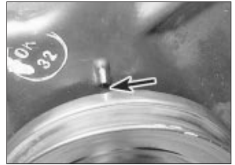
7.7 Ignition timing marks (arrowed) in alignment
