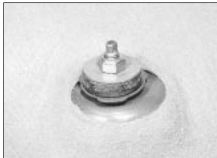
12.2 Rear shock absorber upper mounting - Hatchback
