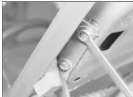
6.3 Removing a bonnet hinge bolt
