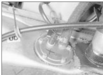
6.3 Fuel gauge sender unit secured by bolts
