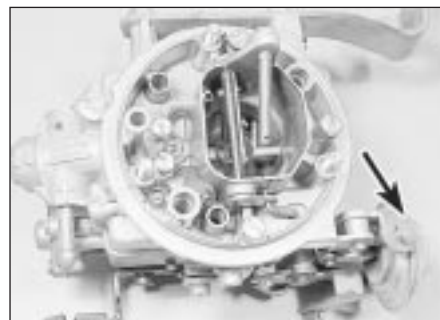
12.11b Choke valve gap adjusting screw (arrowed)
