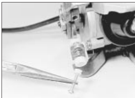
14.4 Removing the tamperproof cap from the fast idle adjustment screw
