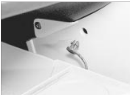
36.1 Glovebox check strap disconnected
