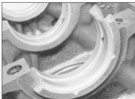
20.12 Centre main bearing shell, showing thrust flanges
