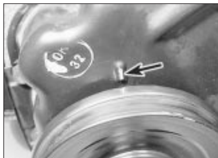
6.3 Ignition timing marks (arrowed) in alignment
