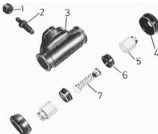
12.6 Exploded view of a rear wheel cylinder
