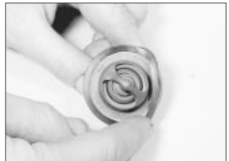
4.14 Fitting a new seal to the thermostat
