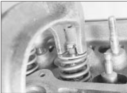
9.20 Compress the spring and fit the collets
