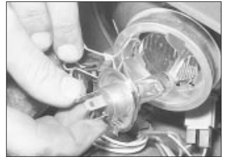
11.3 Removing a headlamp bulb
