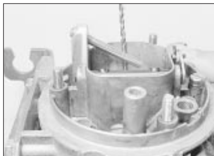
12.11a Using a drill bit to check the choke valve gap
