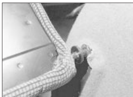
33.3b Seat pivot lifts out of hinge
