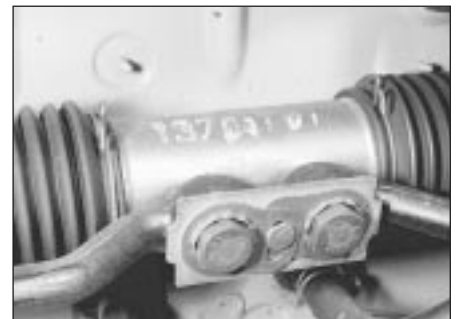
27.4 Tie-rod connection to steering rack
