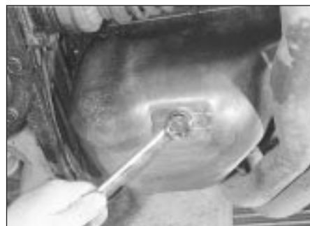
6.4 Removing the sump drain plug
