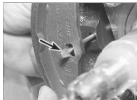
20.3b . . . and the rear steady pin
