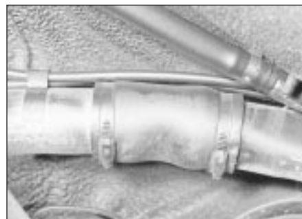
7.11 Fuel tank filler pipe-to-neck junction
