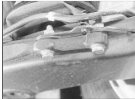
13.7 Auxiliary anti-roll bar mounting - 2.0 litre 16-valve models
