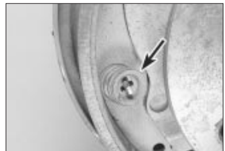
6.5b Brake shoe steady pin and washer (arrowed)
