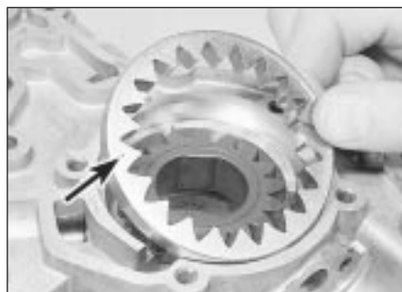
14.4 Gear outer face identification mark (arrowed)
