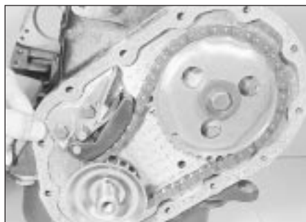
14.20 Fitting a new timing cover gasket
