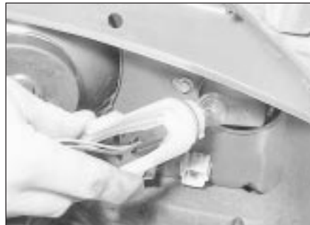
11.9 Removing a direction indicator bulb and holder
