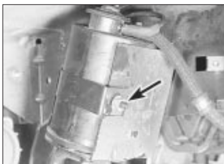
12.98a Canister clamp nut (arrowed)
