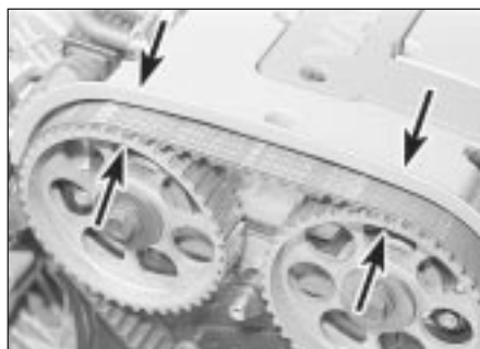
7.8b . . . and sprocket marks align with backplate notches (arrowed)
