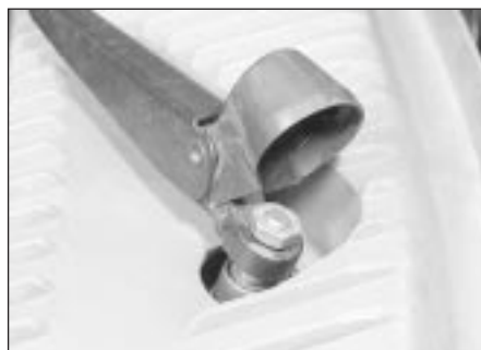
19.3 Wiper arm retaining nut
