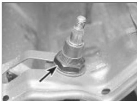
20.4 Wiper spindle clamp nut (arrowed)
