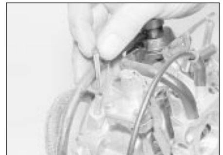
22.4 Fuel inlet fuel strainer
