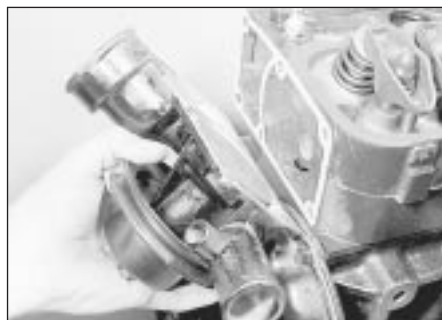
5.4 Removing the water pump - 1.2 litre model
