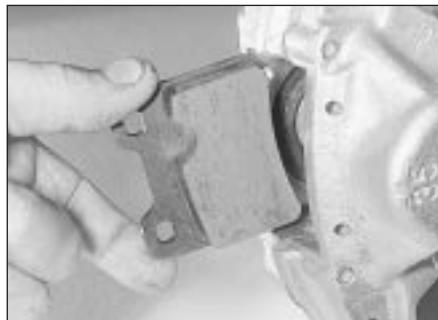
5.9a Fitting a rear pad
