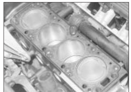
11.22 New head gasket in position
