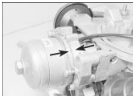
15.12 Choke cover alignment marks (arrowed)
