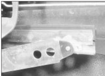
18.6 Scissors lifting mechanism slider
