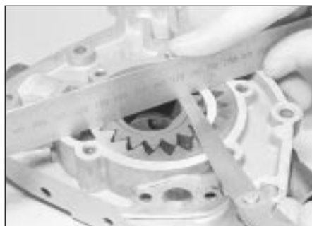
14.3 Checking oil pump gear endfloat
