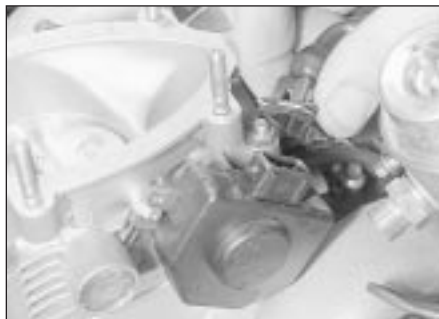
12.82 Disconnecting the throttle valve switch multi-plug
