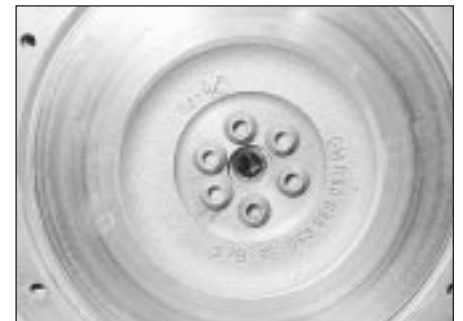
16.4 Flywheel retaining bolts are socket-headed
