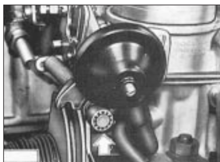
13.2 Fast idle adjustment screw (arrowed)
