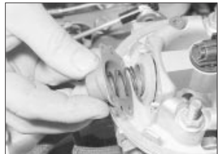
11.17b . . . and remove the pressure regulator cover, spring and diaphragm
