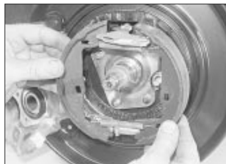
20.4 Removing the handbrake shoe assembly
