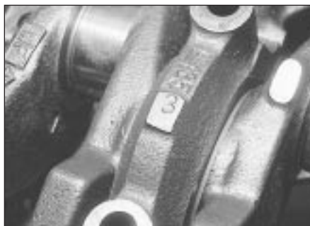
20.3 Identification number on No 3 main bearing cap
