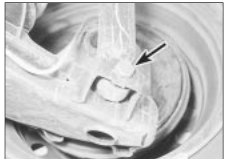
12.5 Rear shock absorber lower mounting bolt (arrowed) - Hatchback
