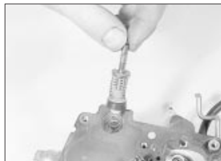
23.10 Accelerator pump plunger and spring
