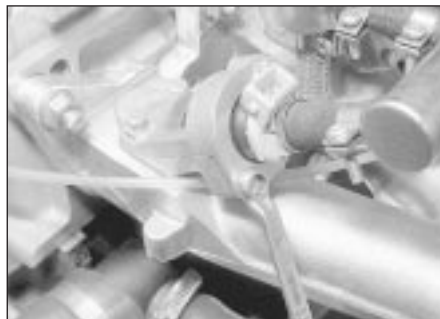
12.8 Undoing a fuel injector retaining bolt
