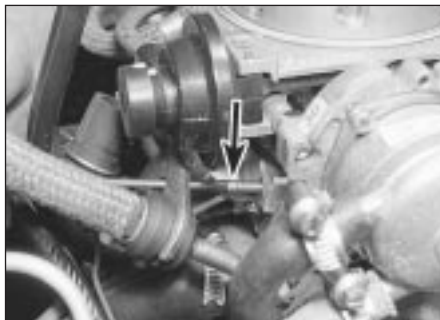
11.4b Idle speed adjustment screw (arrowed) - 2E3 carburettor
