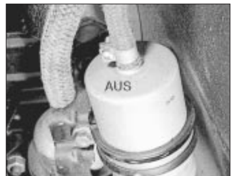
25.4 Fuel filter directional marking
