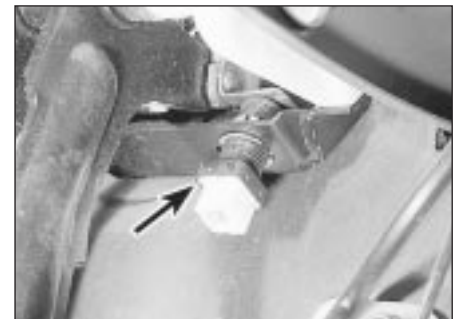
22.1 Stop-light switch (arrowed) on brake pedal bracket
