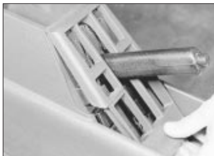
4.20 ... then prise off the switch trim panel ...
