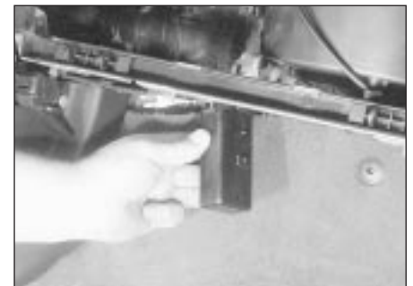
20.2 Removing the central locking electronic control unit - models from 1993
