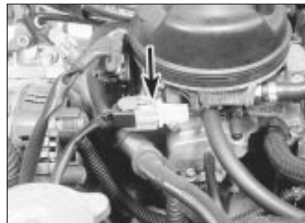
16.3 Injector wiring connector (arrowed)
