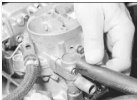
12.5 Disconnecting the float chamber breather pipe
