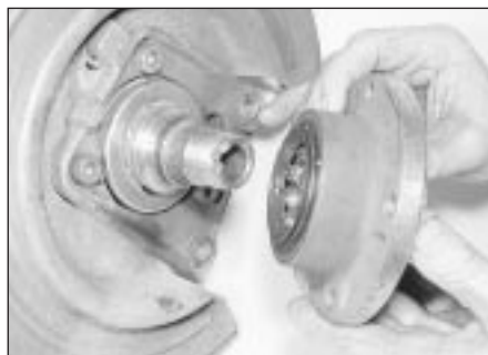
10.11a Fit the hub assembly ...
