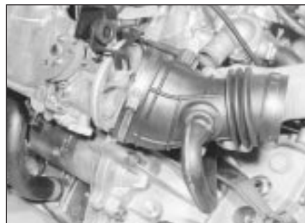
12.6 Detach the plastic duct
