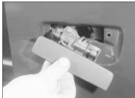
14.8 Withdrawing the exterior door handle
