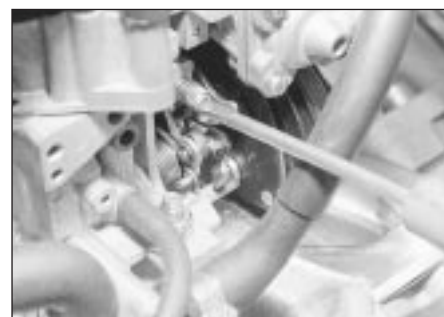
10.4b Idle speed adjustment screw
