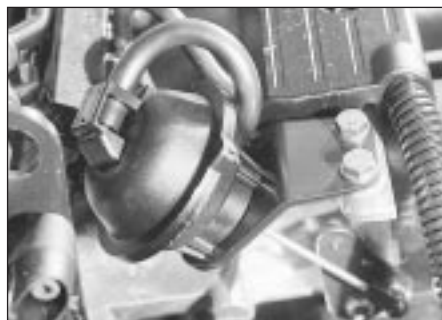
19.16 ACAV vacuum diaphragm unit
