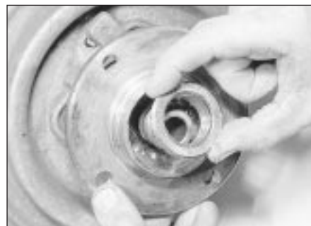
10.11b ... followed by the outer bearing race ...
