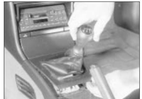
29.31 Removing gear lever gaiter surround ("Lowline" console - models from 1993)
