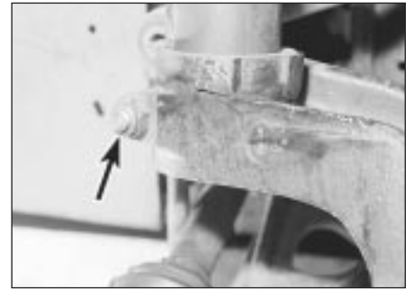
2.12 Hub carrier-to-suspension strut clamp nut (arrowed)
