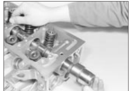
10.9b . . . and slide out the camshaft
