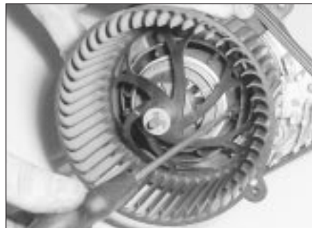
9.65b . . . and release the clips . . .
