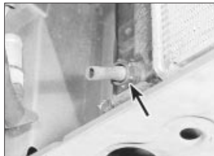
20.3 Radiator drain outlet (arrowed)
