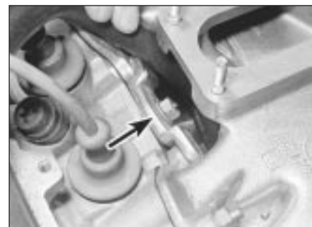
14.6 Inlet manifold centre clamp on the XU engine
