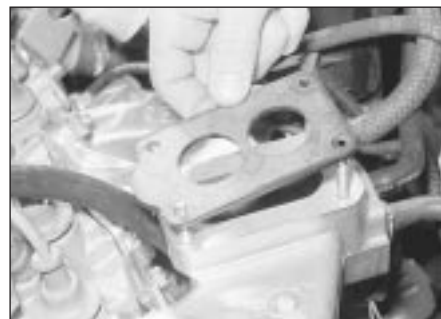
12.11 Removing the insulating spacer
