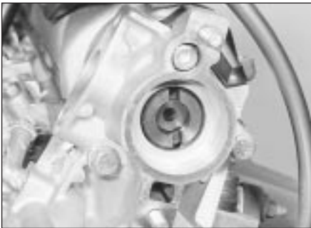
4.10 Off-set drive slots on the camshaft
