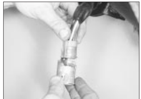
18.8c ... and slide out the ignition switch
