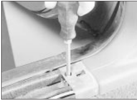
27.6 Removing a lower B-pillar trim panel bottom securing screw
