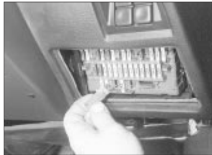
3.7 Removing a fuse using the plastic tool
