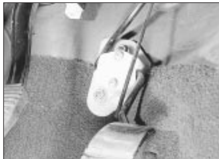
8.2 Accelerator pedal pivot bush
