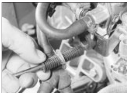
7.1b Outer cable end fitting
