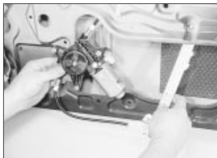
15.16 Removing the front door window regulator assembly
