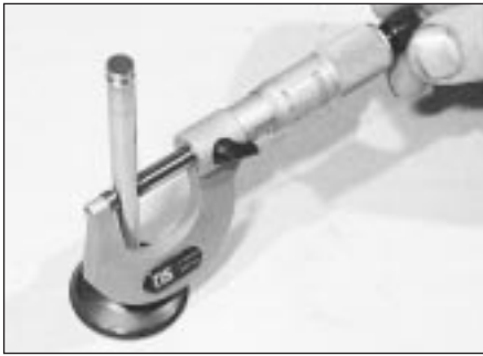
8.11 Measuring a valve stem diameter
