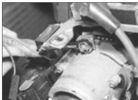
4.4b Unscrew the retaining nuts . . .
