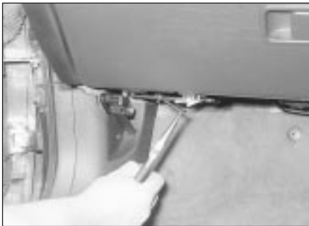
28.13 Remove the hinge pins . . .
