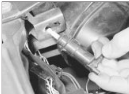
7.4 Removing a cable-operated headlight adjuster
