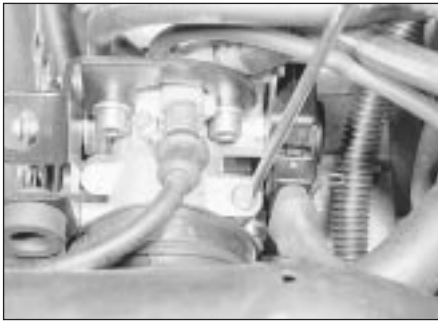
11.4 Adjusting the idle speed screw on the Bosch L3.1 system
