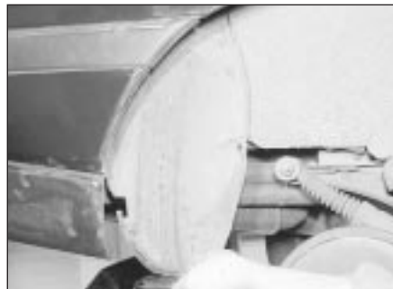
7.2 Removing a rear wheel arch liner
