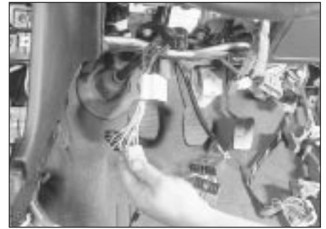
30.60 Unplug the main wiring harness connectors
