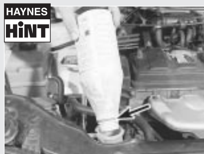
20.22 Peugeot cooling system "header tank" in position
