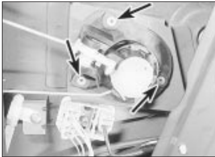
19.4 Tailgate lock cylinder securing rivets (arrowed)
