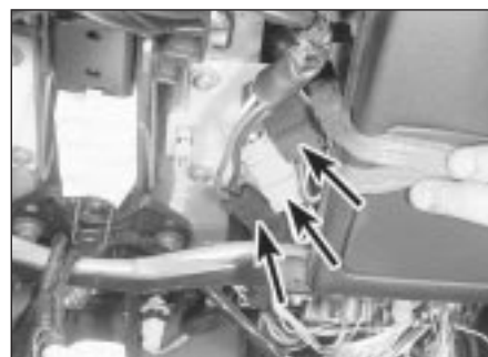
17.8 Ignition switch wiring connectors (arrowed) - models from 1993
