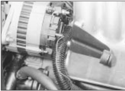
7.2 Connections on the rear of the alternator
