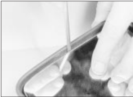
22.9 Releasing a mirror glass locking ring
