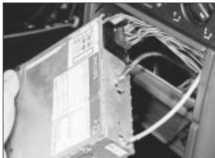
20.4 . . . and withdraw the unit
