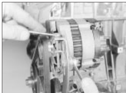
5.8 Loosening the alternator adjustment bolts (early models)
