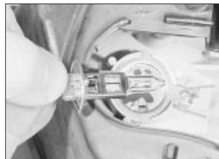
5.23b Removing a headlight-mounted driving light bulb
