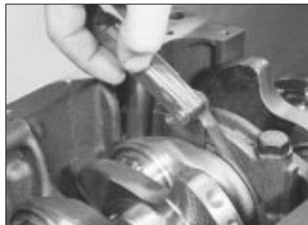
14.3 Checking crankshaft endfloat using feeler gauges
