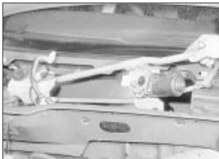
17.8c Withdrawing the windscreen wiper motor and linkage assembly
