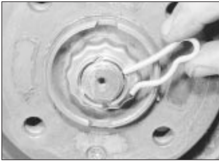
2.3 Withdraw the R-clip from the driveshaft nut locking cap
