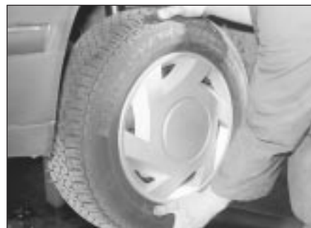
16.4 Check for wear in the hub bearings by grasping the wheel and trying to rock it
