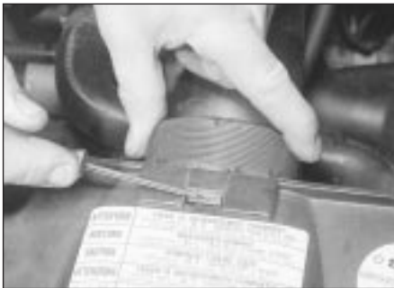
3.5a Depress the securing clip . . .
