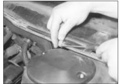
30.64a Remove the securing clip . . .
