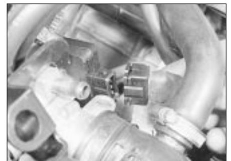
12.5 Disconnecting the multi-plug
