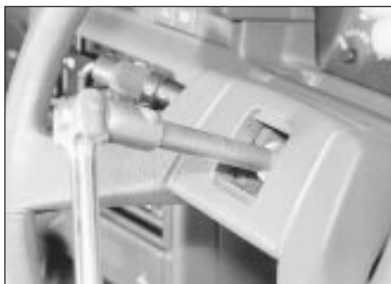
16.4 Unscrewing the steering wheel nut
