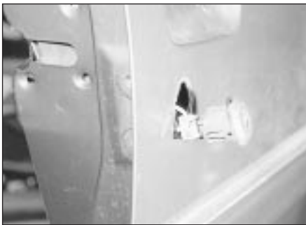
14.13b ... then withdraw the lock cylinder
