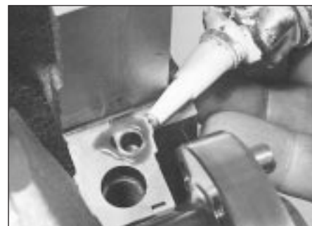
18.71 Applying sealant to the cylinder block No 1 main bearing cap mating face
