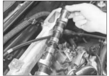
10.33 . . . then lift the camshaft away from the cylinder head
