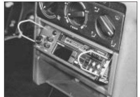
20.3 . . . then insert the removal tools . . .
