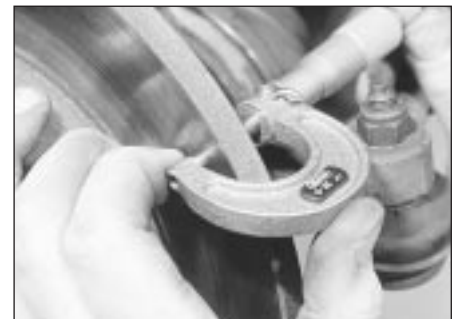
7.3 Using a micrometer to measure disc thickness
