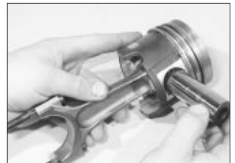
13.15b . . . and withdraw the gudgeon pin
