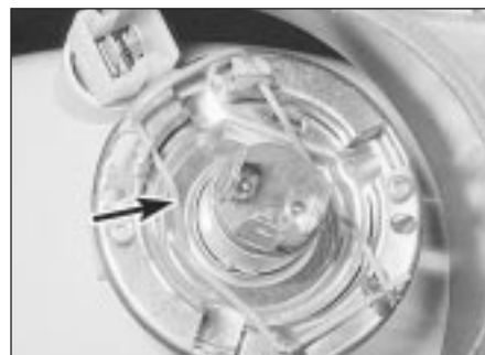
5.4a Release the spring clip (arrowed) . . .
