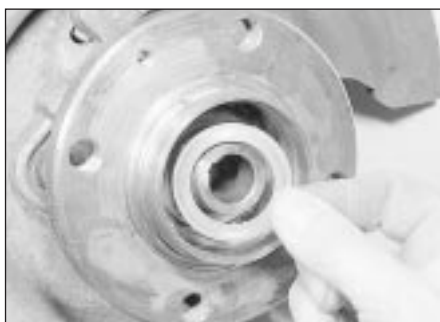
10.12a ... and the thrustwasher
