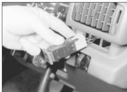
4.11 Removing a driver's side fascia-mounted switch - models up to 1992
