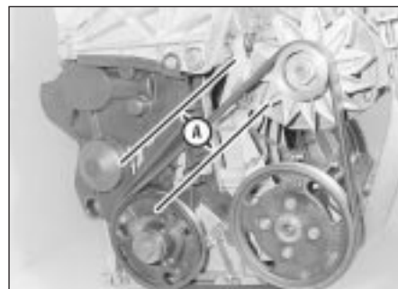
5.11 Alternator drivebelt deflection (A)
