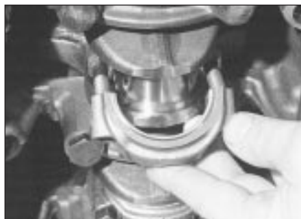
10.5 Removing a big-end bearing cap and shell
