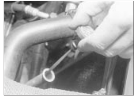
4.2a Withdrawing the automatic transmission dipstick
