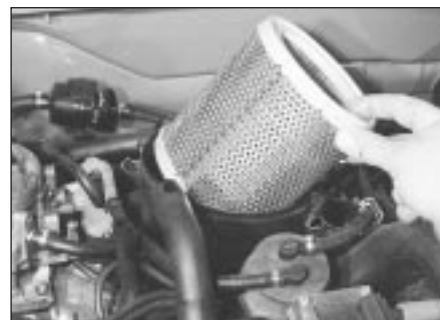
21.3 Removing the air cleaner element on TU models
