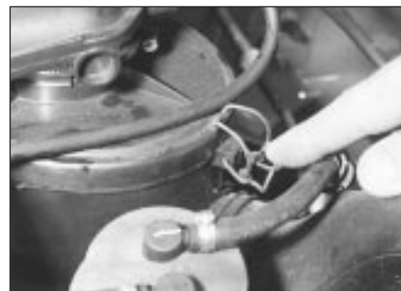
21.2a . . . then release the air cleaner lid retaining clips, and the duct clip . . .
