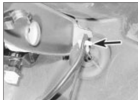
7.4 Accelerator cable connection to accelerator pedal (arrowed)
