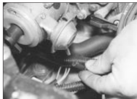
4.3b . . . and the vacuum diaphragm hose
