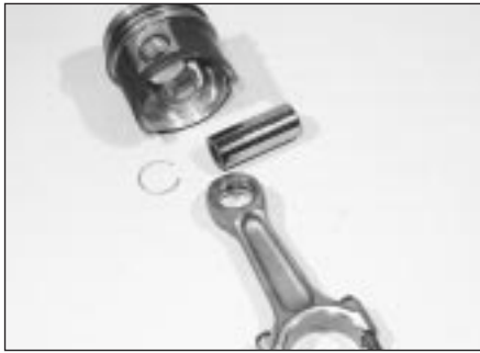
13.15c Piston and connecting rod components
