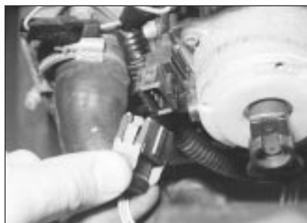
4.3a Disconnect the distributor wiring connector . . .
