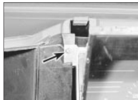
9.8 Instrument panel securing screw (arrowed)
