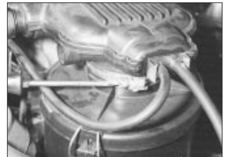
2.2a . . . slacken the retaining clips . . .
