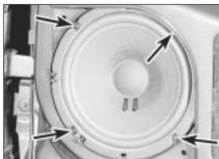
21.3 Door-mounted loudspeaker securing screws (arrowed)
