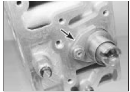
10.8 Undo the retaining bolt, and remove the camshaft thrust fork (arrowed) . . .
