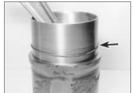
12.18b . . . and recover the bottom O-ring seal (arrowed)
