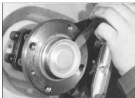
10.4a Tap the cap from the centre of the hub . . .
