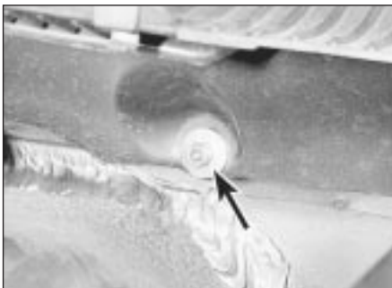
30.20 Facia securing nut (arrowed) in scuttle
