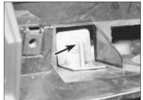
30.23 Upper facia securing bolt (arrowed)
