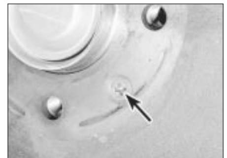
9.2 Rear brake drum retaining screw (arrowed)
