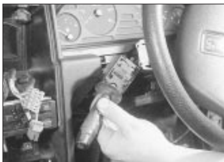
4.6b . . . and withdraw the steering column combination switch - models from 1993
