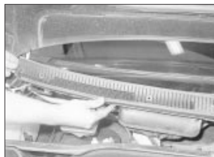
25.11 Removing the scuttle grille panel
