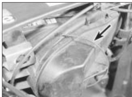
5.2 Headlight rear cover securing clip (arrowed)
