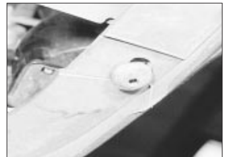
6.1 Front bumper lower securing screw
