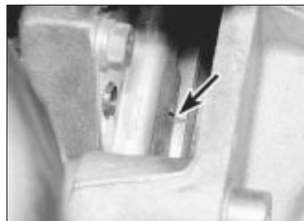
6.2b Timing marks on the flywheel and timing plate
