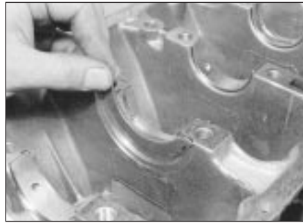
18.40 Refitting a crankshaft thrustwasher - TU series aluminium block engine
