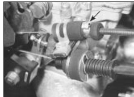
9.10 Choke cable-to-rubber collar retaining clip (arrowed)
