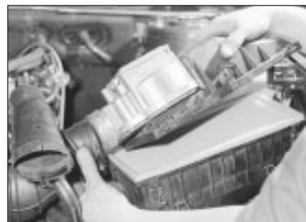
21.8 Lifting off the top cover
