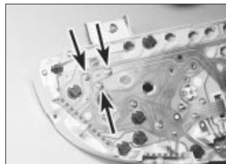
10.9 Fuel gauge securing nuts (arrowed)
