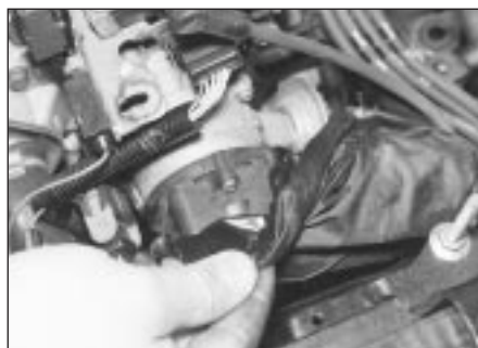
4.2a Peel back the waterproof cover . . .
