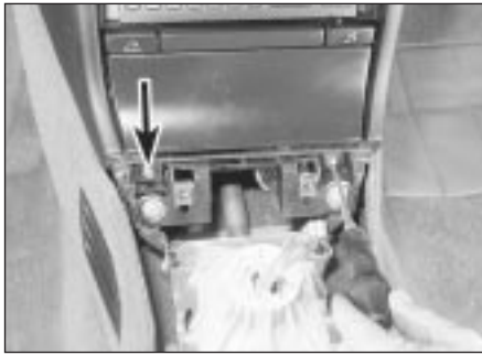
30.34 Unscrew the two screws below the ashtray housing
