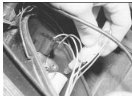
5.10 Pull out the sidelight bulbholder . . .
