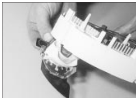
10.11a . . . then withdraw the gauge . . .
