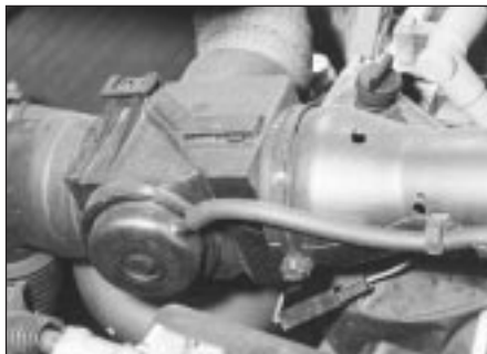
3.17 Air temperature control valve assembly (TU engine)
