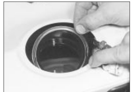
9.12b . . . and recover the rubber sealing ring
