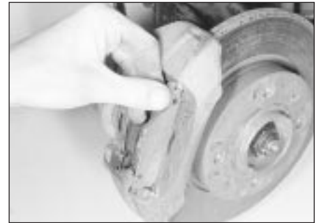
4.6 Withdrawing the outer brake pad - Bendix caliper
