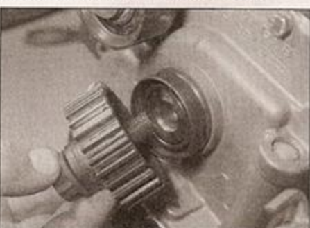
9.9b ... then fit the crankshaft sprocket and bolt, and use the sprocket to press the new seal into place
