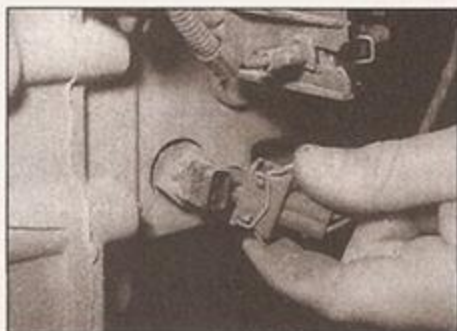
5.2 Disconnecting the reversing light switch
