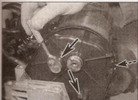
8.3a Remove two bolts on the end of the engine, and one at the front (arrowed) ...
