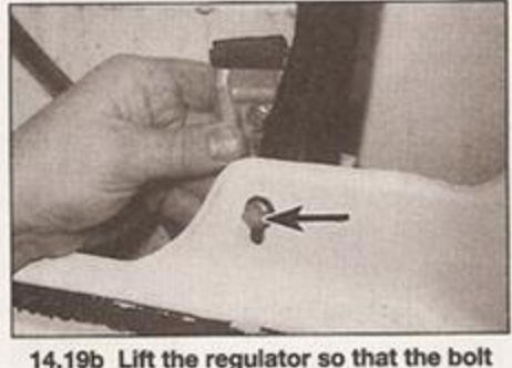
14.19b Lift the regulator so that the bolt heads (arrowed) can pass through the holes in the door frame
