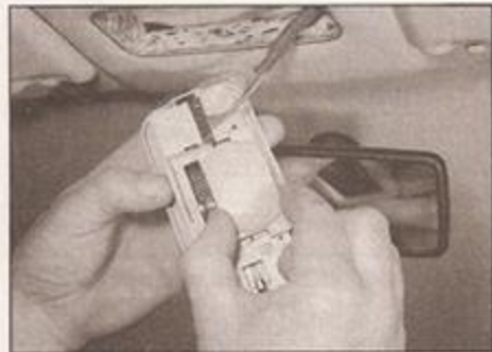
8.3 To renew the bulb, slide up the cover ...
