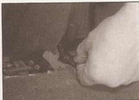
15.7a Release the handbrake warning light switch from the base of the lever . . .
