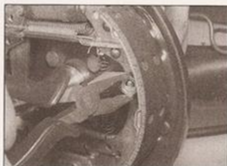
5.7a Using pliers, remove the spring cup . . .
