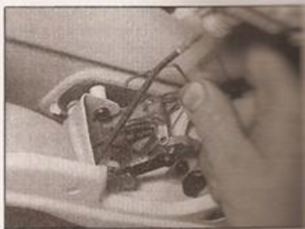
16.6a Prise out the wire clip
