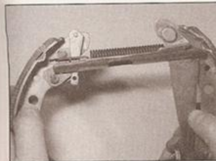
5.17a Locate the leading shoe in the pushrod ...
