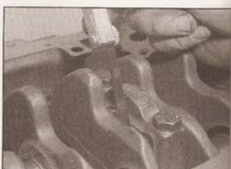
6.5 Measuring crankshaft endfloat using feeler blades
