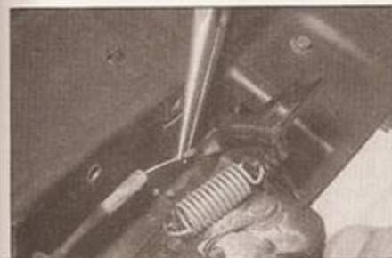
9.1a Unhook the bonnet release inner cable ...
