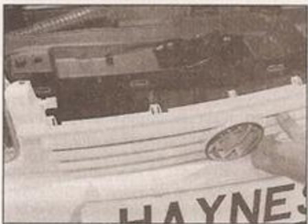
29.2d ... and remove the grille from the front of the car
