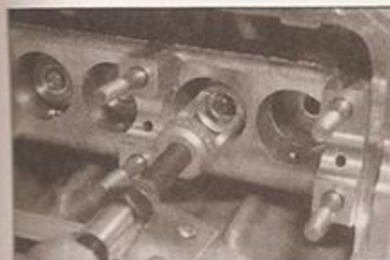
4.13a Valve spring compressor jaws located on the upper spring seat ...
