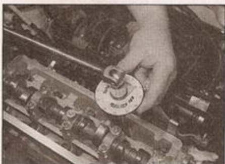
10.39 Use an angle gauge to ensure accuracy when angle-tightening the cylinder head bolts
