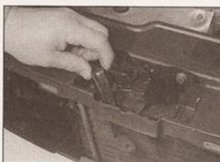
10.2b ... then unhook the arm from the lock carrier, and remove it
