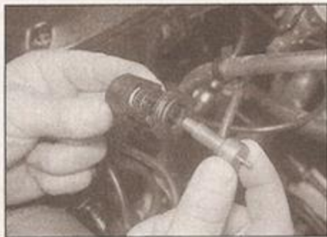
4.6b The thermostat can be separated from its spring housing
