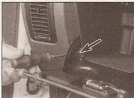
26.10a Remove the screw behind each hinge ...
