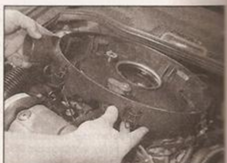
2.8 Withdraw the air cleaner housing from the engine compartment
