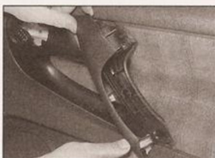
12.7b ... and remove it from the door
