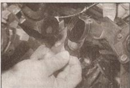
10.10 Pull out the horseshoe clip from the base of the thermostat housing - seen here with the housing removed, for clarity
