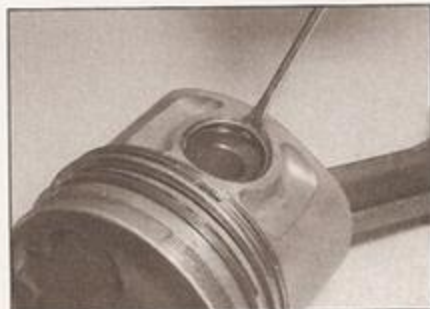
5.12a Insert a small screwdriver into the slot and prise off the gudgeon pin circlips
