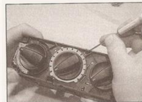
9.8a Using a small screwdriver, release the cover retaining lugs . . .
