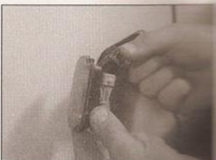
7.23 To remove the light unit, disconnect the wiring plug
