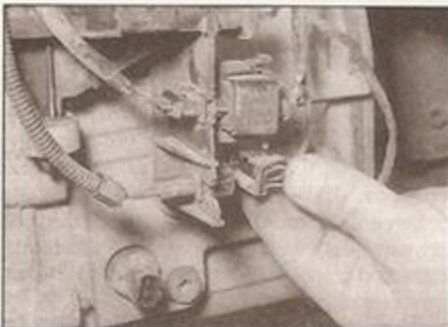
3.9 Disconnect any wiring harness multi-plugs at the front of the gearbox
