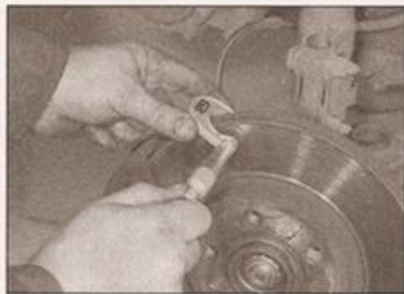
6.3 Measuring brake disc thickness with a micrometer
