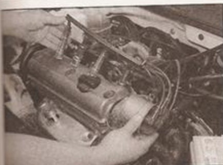
2.15 Removing the HT leads and distributor cap as an assembly, for cleaning
