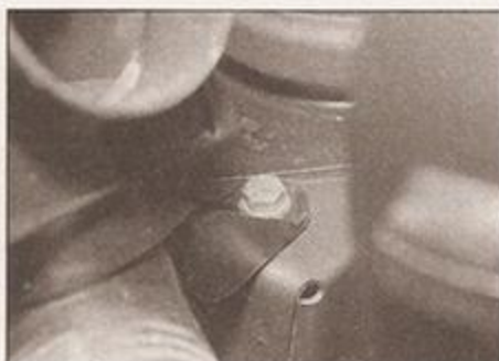
2.9b Air temperature control valve housing mounting bolt on inner wing
