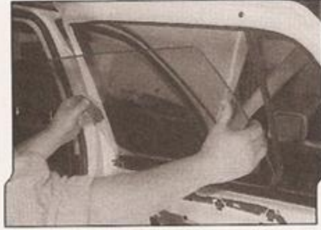
14.15 Lifting out the rear door window glass
