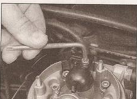
5.11 Removing the injector securing screw
