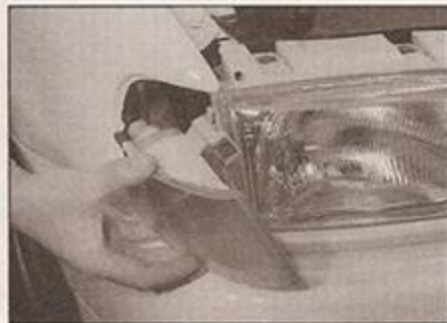
7.16a ... pull out the light unit ...
