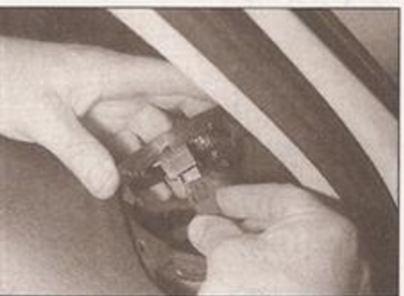
19.3b . . . and disconnect the wiring plug
