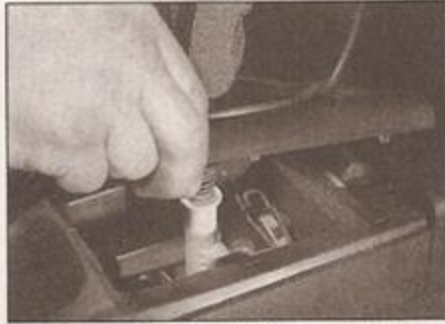
27.1b ... then unclip the console top cover, and lift it over the gear lever
