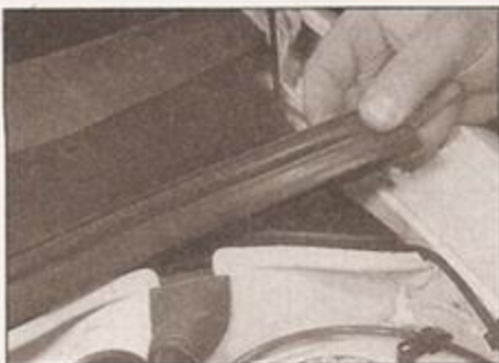
22.2 Pull off the rubber weatherstrip from the top of the bulkhead
