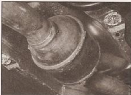
6.1 Oxidation catalyst fitted to diesel engine models
