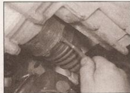
2.7b Using a suitable key or socket, slacken the splined bolts...
