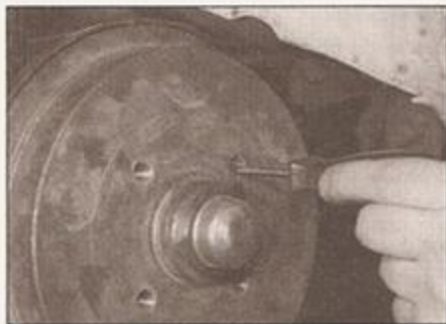
7.7a Release the brake shoes by inserting a screwdriver through the drum hole ...
