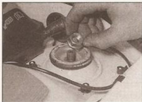
2.3b . . . loosen and remove the strut upper mounting nut
