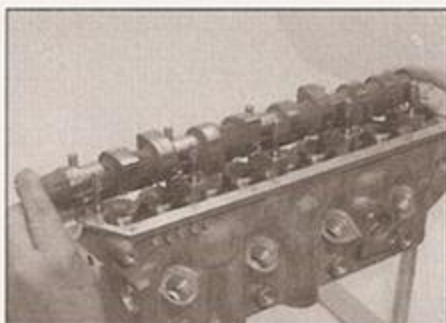
4.65b . . . then lower the camshaft into position on the cylinder head
