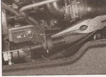
3.6 Using a suitable pair of pliers, pull out the metal clip used to set the cable adjustment
