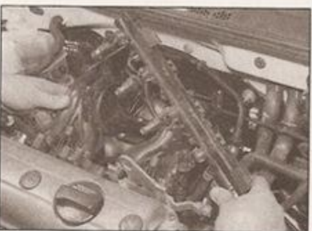
10.7b . . . and withdraw the manifold (and fuel rail) from the cylinder head
