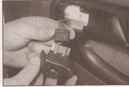
12.6b ... and disconnect the mirror switch wiring connector
