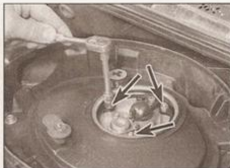
2.2a Remove the air cleaner housing securing nuts around the top of the throttle body (arrowed) . . .
