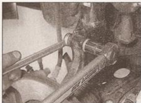
2.7 Tighten the strut-to-swivel hub nuts/bolts to the specified torque
