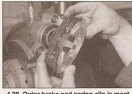
4.28 Outer brake pad spring clip is most easily engaged in the caliper by pressing in downwards
