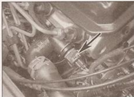
6.15a Coolant temperature sender wiring plug (arrowed)
