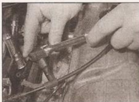
21.7a Unscrew the spark plugs using a suitable socket . . .
