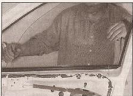
14.6b ... then lift the window glass upwards and out of the door frame
