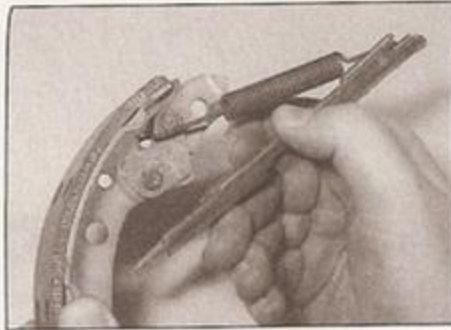
5.15b ... then engage the pushrod with the opposite end of the spring ...
