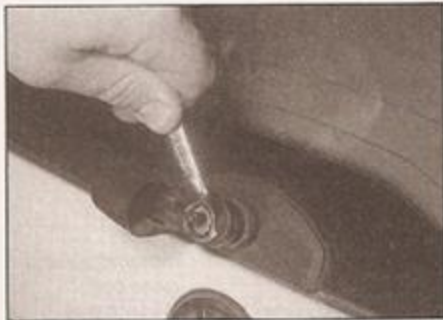
15.3b . . . then remove the wiper arm nut . . .
