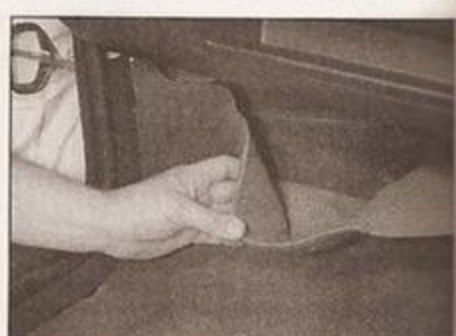
9.39a Fold back the carpet from the passenger footwell ...
