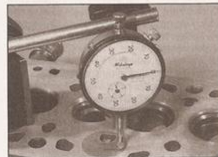
4.57 Measuring swirl chamber projection using a DTI gauge
