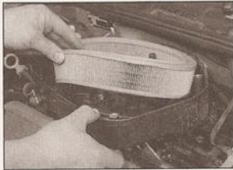
2.3 Removing the air cleaner element (not essential, if just the housing is to be removed)
