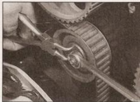
4.31a Tensioning the timing belt using a pair of circlip pliers in the belt tensioner
