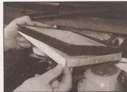
24.7a Separating the pollen filter from the frame
