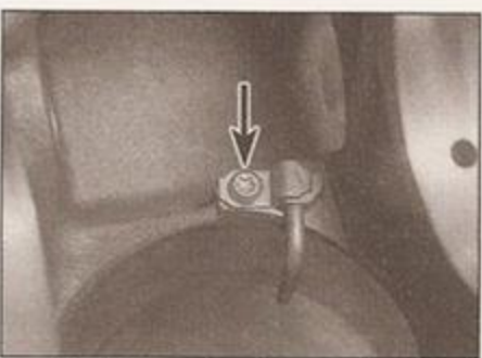
5.5a Remove the piston cooling jet retaining screw (arrowed) . . .
