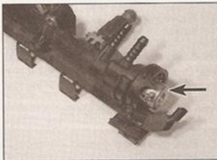
5.23a The fuel pressure regulator is mounted in the end of the fuel rail (arrowed)
