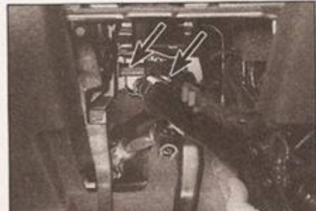
14.13a Unhook the column tube from the mounting (arrowed) ...
