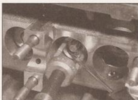
4.62b Use grease to hold the two halves of the split collet in the groove
