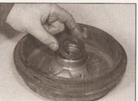
8.6 Grease the lips of the oil seal, and press it into the rear of the hub
