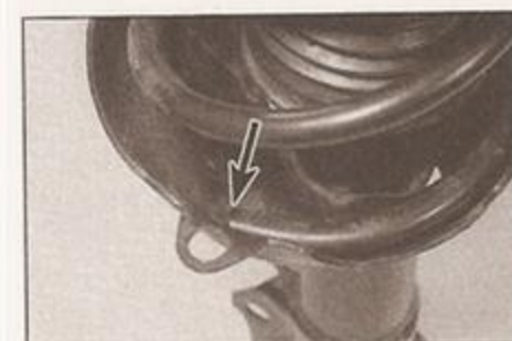
3.9d ... ensuring that the spring end (arrowed) engages with the recess in the lower spring seat
