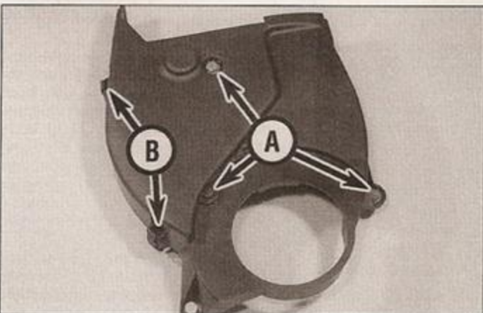
4.12 Timing belt lower cover removed, showing locations of retaining bolts (A) and clips (B)
