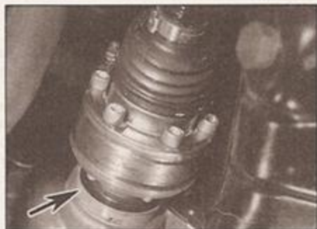
13.2 Driveshaft inner CV joint, showing driveshaft seal (arrowed)
