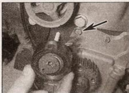
5.7 Slide tensioner onto its mounting stud, fitting the U-shaped baseplate over the bolt (arrowed)
