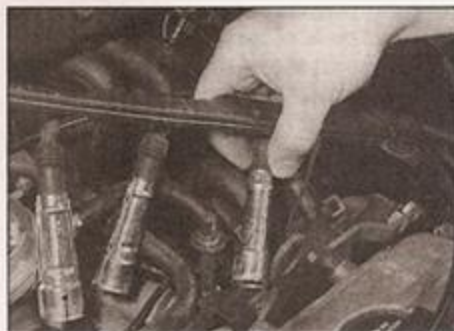
21.5 Pull the HT lead end fittings off the plugs
