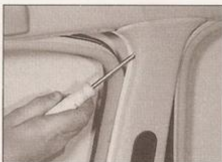
25.12b Prise off the B-pillar upper trim panel ...
