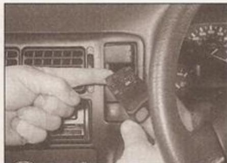
6.3 ... and disconnect the wiring plug
