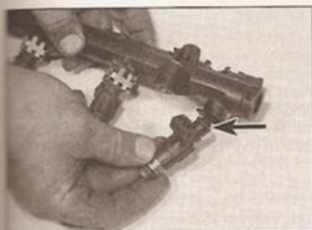
5.15c Ease out the injector, and recover the upper O-ring seal (arrowed)
