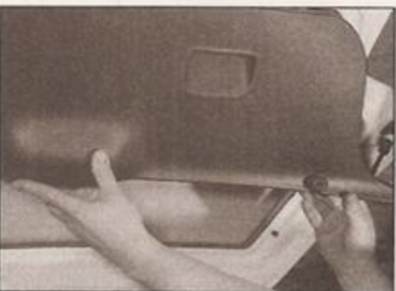
15.2b . . . then release the securing clips and remove the tailgate trim panel
