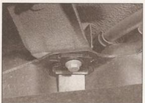
5.9 Fuel tank strap securing bolt
