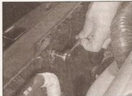
3.8a Loosen and remove the radiator retaining bolts . . .
