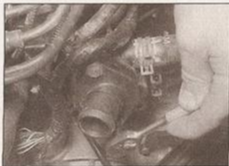
4.5a Loosen and remove the thermostat cover bolts . . .
