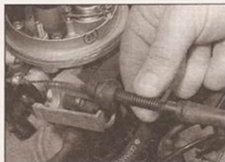
4.3 Removing the accelerator cable from the mounting bracket
