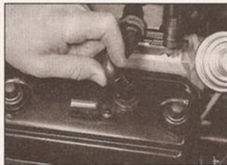
13.2 Pull the breather hose out of the camshaft cover
