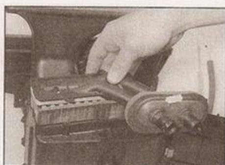
9.36b ... and withdraw the heater matrix from the air distribution housing
