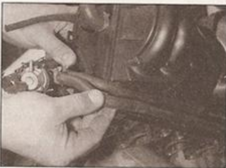
10.8 Unclip the fuel hoses from the base of the manifold, and remove the manifold from the engine compartment
