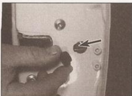
13.30 Door lock adjustment screw (arrowed)
