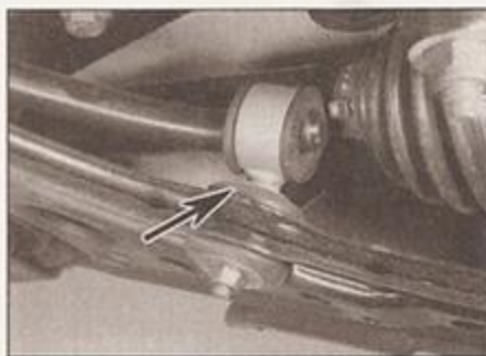
17.6 Anti-roll bar mounting bushes (arrowed) - only on 1.6 litre models
