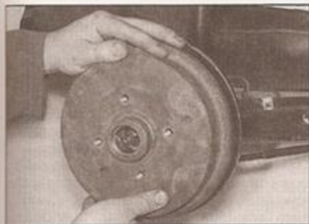
7.5 ... and remove the brake drum
