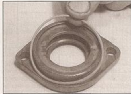
7.3d . . . then recover the O-ring seal
