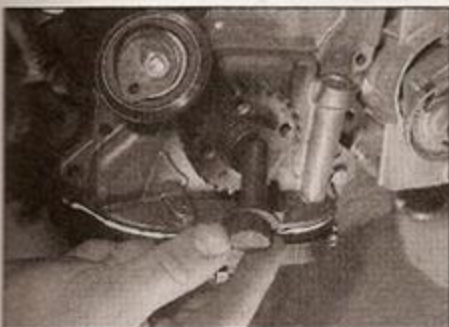
5.25a Remove the crankshaft sprocket bolt (this is a bi-hex type) ...
