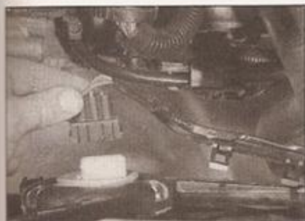
5.5 Disconnect the cooling fan motor wiring connector
