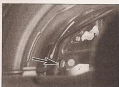
16.2 Rear brake backplate inspection hole (arrowed) for assessing brake lining wear
