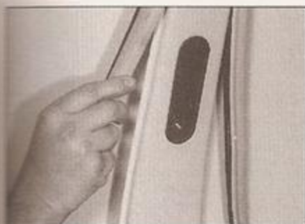
25.12a Pulling off the weatherstrip from the door aperture
