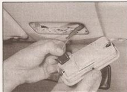
8.2b ... and disconnect the wiring plug, if required
