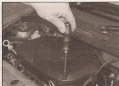
26.2a Unscrew the cover retaining screws . . .
