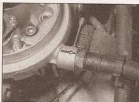
5.3b ... and fuel return connection
