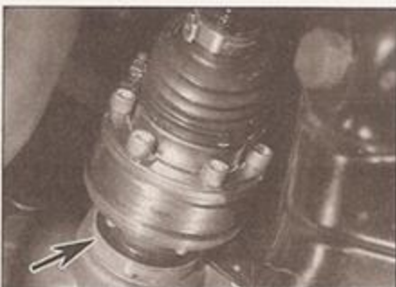
14.2 Driveshaft inner CV joint, showing driveshaft seal (arrowed)
