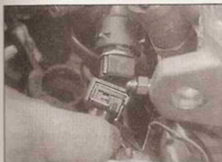
11.13 Disconnect the wiring plug from the coolant temperature sensor
