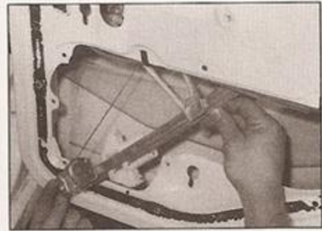
14.23 Removing the rear door window regulator
