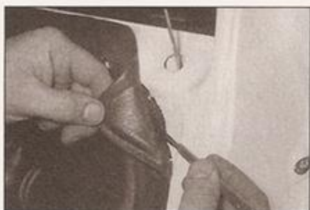
14.4a Using a small knife to slice through the adhesive securing the foam panel to the door
