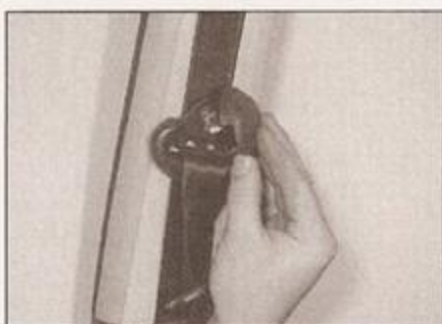
25.1 Unclip the cover from the seat belt upper mounting ...
