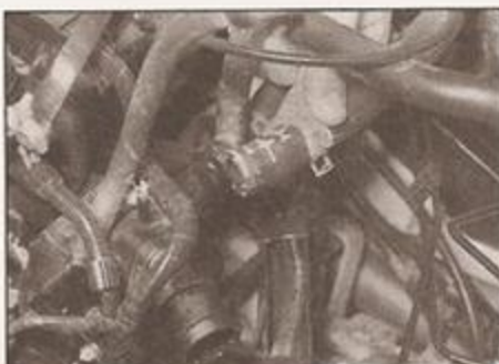
2.8 Disconnecting a heater hose from the thermostat housing (petrol engine model)
