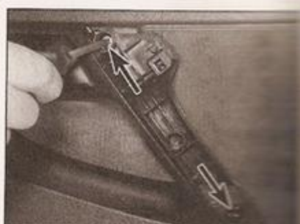
12.8 Door handle surround securing screws (arrowed)
