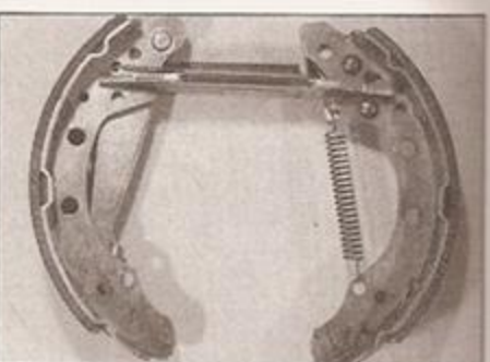
5.10 Prior to dismantling, note the correct fitted location of the shoe components
