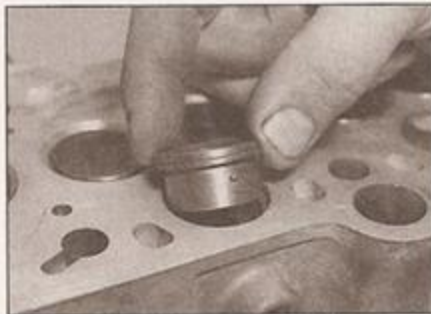
4.56a Fitting a swirl chamber (diesel engine code AEF)
