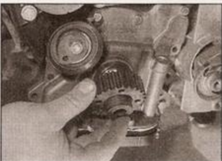
5.25b ... then slide the sprocket off the crankshaft
