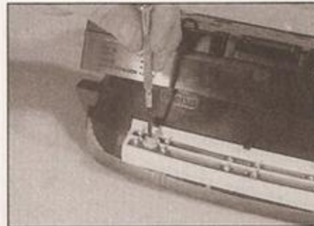
8.11a Turn the bulbholder using a small screwdriver ...
