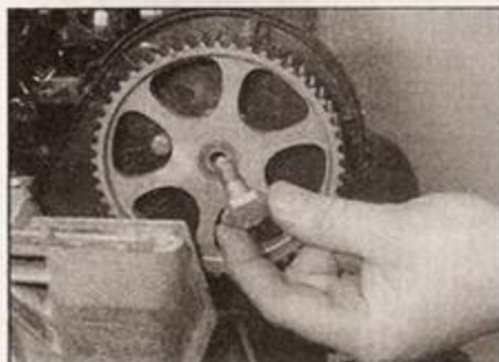
5.14 Remove the camshaft sprocket bolt ...
