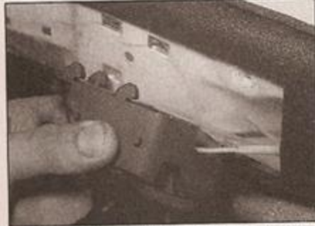
13.3b ... then slide the handle out of the door ...
