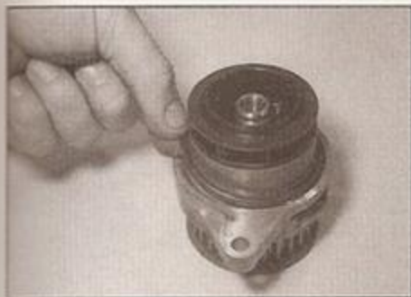
7.13 Fit a new O-ring to the coolant pump
