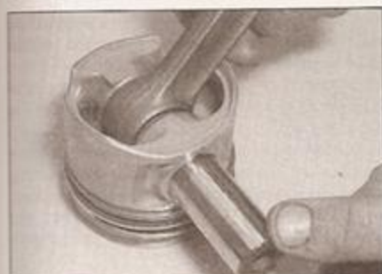
5.12b Push out the gudgeon pin and separate the piston and connecting rod
