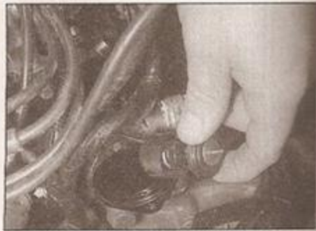
4.6a Withdraw the thermostat from the housing
