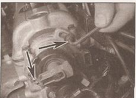
4.8a Loosen the clamp bolts (arrowed) using an Allen key ...
