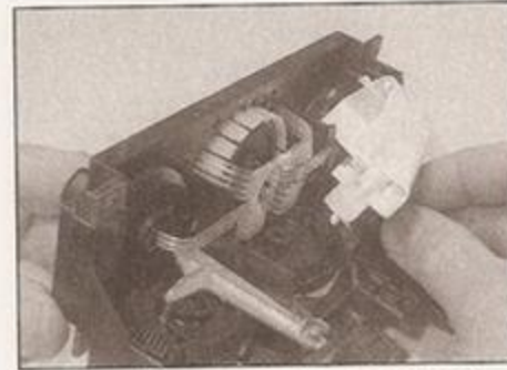
9.8b . . . then remove the cover from the rear of the heater control panel
