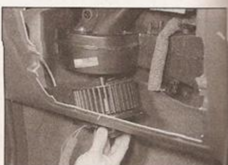
9.41 Twist the blower motor to release it, and lower it out of the housing
