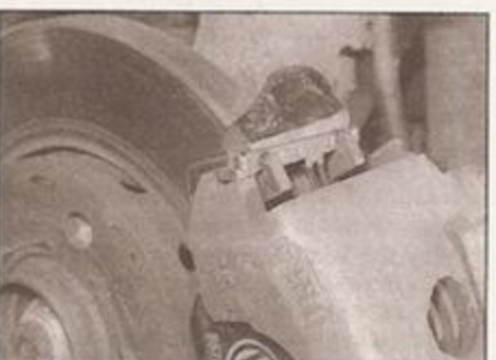
4.12b ... ensuring that the caliper lugs engage properly with the anti-rattle springs
