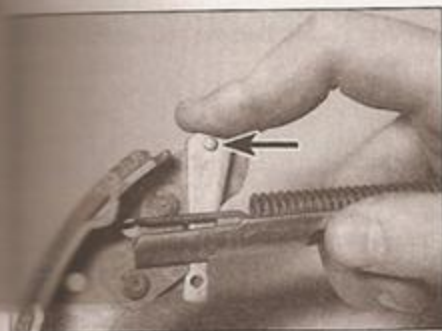
5.16 Slot the wedge key into position. Ensure raised dot (arrowed) is facing away from the shoe
