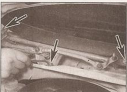
13.9a Wiper frame-to-body bolts (arrowed)
