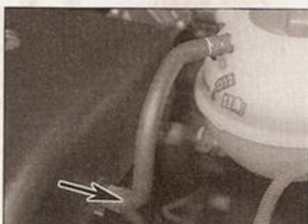
16.3b ... unclip the expansion tank hose from the cover (arrowed)
