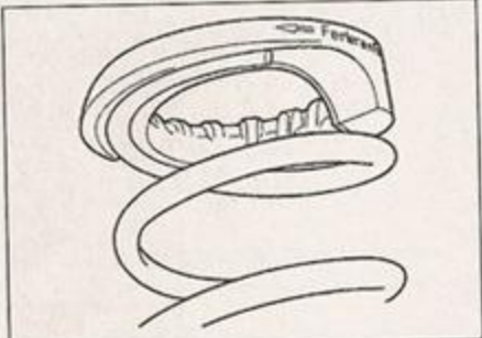
11.10 The spring seat must be installed so that the arrow aligns with the end of the spring
