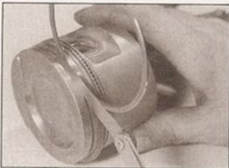
5.21 Measuring the piston ring-to-groove clearance using a feeler blade
