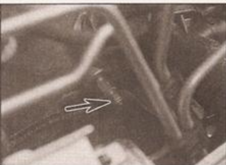
3.4 Glow plug and supply cable retaining nut (arrowed)
