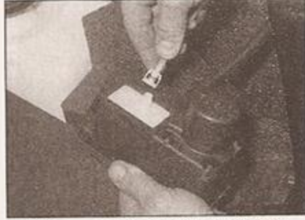
17.5c ... and the vacuum connection
