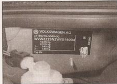
VIN plate on engine compartment bulkhead
