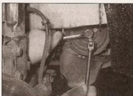
4.10a Loosen the crankshaft pulley bolts, counterholding on the centre bolt . . .
