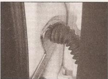
28.11a Using a C-spanner, turn the harness locking ring ...
