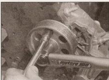
5.31 Brace the intermediate shaft sprocket, then remove the retaining bolt
