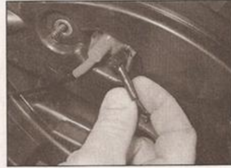
2.6b The air temperature vacuum switch hose fittings are colour-coded
