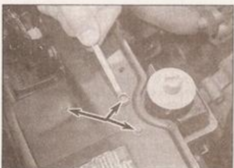
2.5g Remove the power steering reservoir mounting bolts (arrowed) ...
