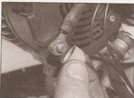
5.4a Remove the protective cap . . .
