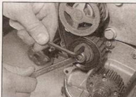
4.22b When the belt tension is correctly set, tighten the tensioner locknut
