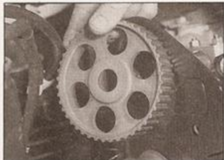
5.13 Removing the camshaft sprocket
