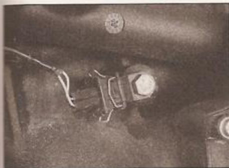
6.4 Knock sensor and wiring plug - seen with engine removed, for clarity
