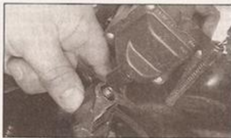
C Check that the HT lead to the ignition coil is securely connected (petrol engine models).
