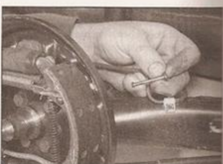
5.7c . . . and withdraw the retainer pin from the rear of the backplate
