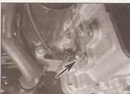
14.3 Reversing light switch (arrowed) - seen from below
