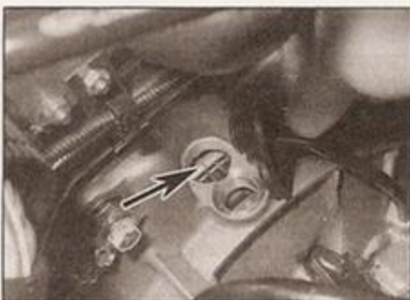
2.2b ... to see the TDC 0 marking (arrowed) on the flywheel
