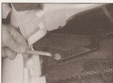
13.3b ... then unscrew the nut and remove the wiper arm
