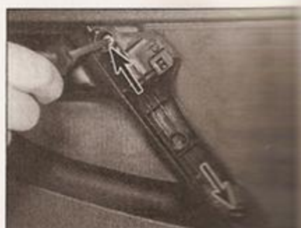
12.8 Door handle surround security screws (arrowed)
