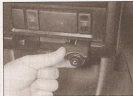
12.4 Pull the cigar lighter downwards and out of the fascia
