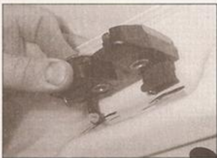
16.3b Removing the tailgate lock
