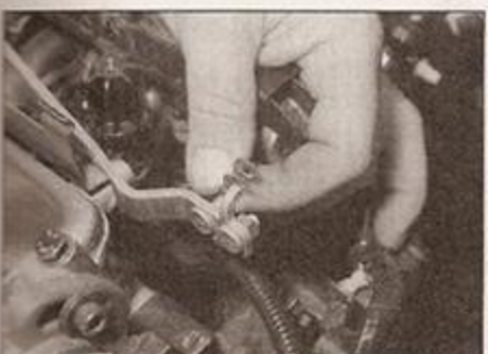
10.8c . . . additional earth wires . . .
