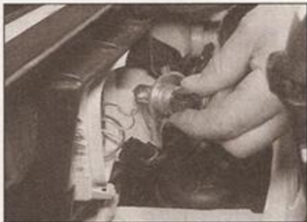
7.5 ... and pull out the bulb
