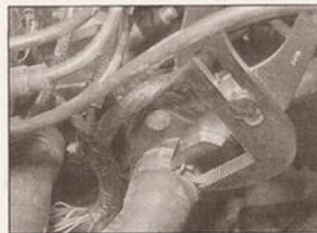
4.4a Using a suitable pair of pliers, compress and release the hose clip . . .
