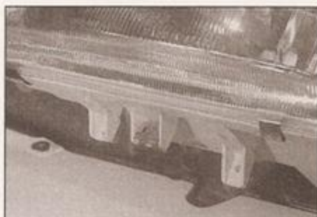
9.2c ... then lift up the headlight to free the lower lugs
