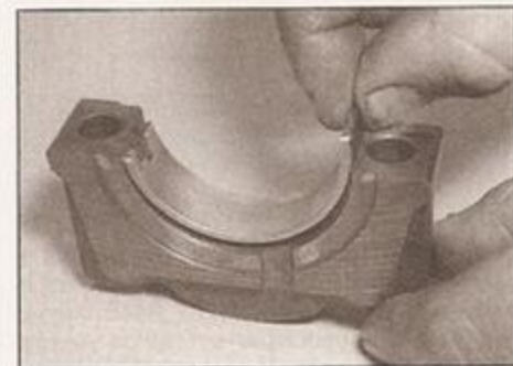
11.8 Fit the new lower half main bearing shells to the main bearing caps
