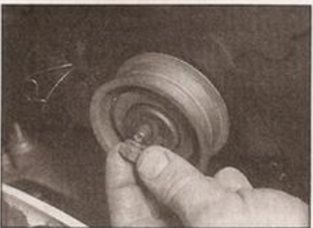
5.3a Remove the tensioner nut and recover the washer
