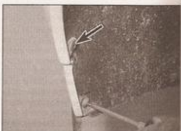
6.4b ... and lower screw (arrowed) - wheel arch liner screw also being removed
