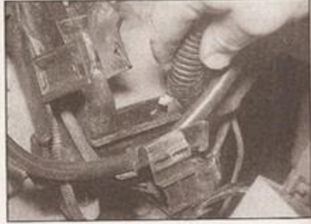
2.24 Disconnecting the wiring harness from the engine
