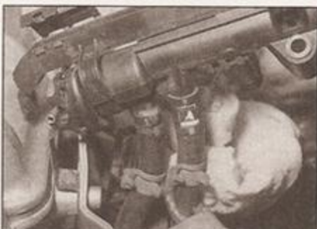
5.13 Fuel supply and return connections at the fuel rail - note direction-of-flow arrows and colour-coding
