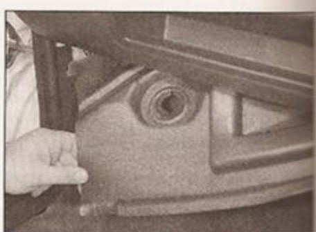
9.39b ... and withdraw the foam cover below the blower motor
