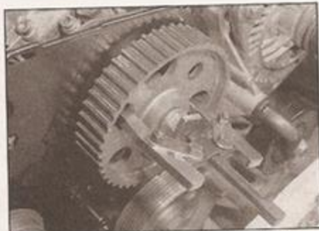
6.8 Attach a two-legged puller to the injection pump sprocket
