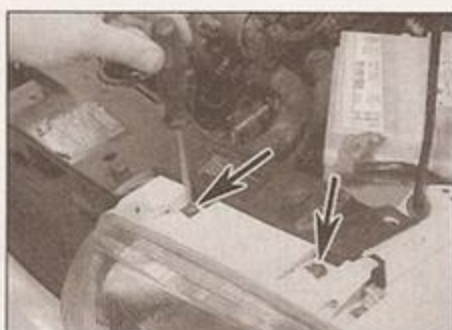
9.2a Remove the two screws at the top (arrowed) ...
