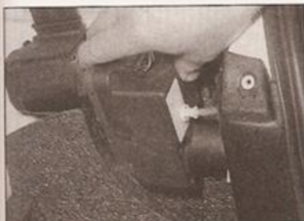
17.5a Pull out the bi-pressure pump ...
