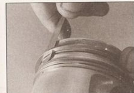
5.13 Piston rings can be removed using an old feeler blade
