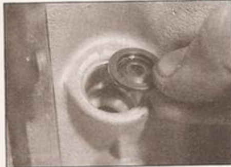
10.7b Recover the heat shield washer
