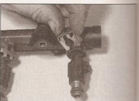
5.15b ... and remove it from the fuel rail
