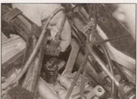
10.8d . . . road speed sensor wiring plug . . .
