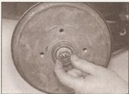
7.3 Remove the split pin and locking cap ...
