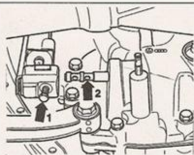
3.27 Selector finger securing bolt (1) fits into forward recess in inner finger (2) when assembled - rod-type gear linkage
