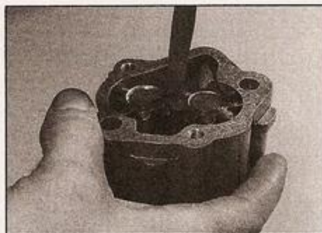
16.7 Checking the oil pump backlash
