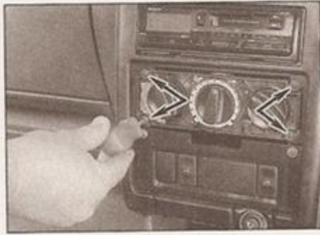
9.2b . . . for access to the four retaining screws beneath (arrowed)
