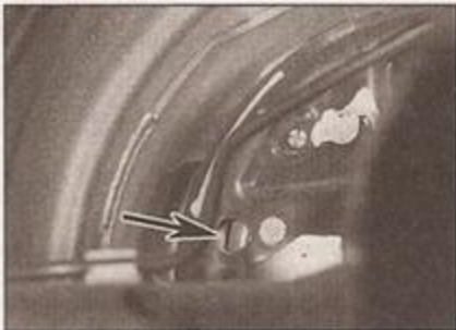
15.2 Rear brake backplate inspection hole (arrowed) for assessing brake lining wear
