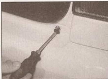
7.3 Removing one of the upper retaining screws
