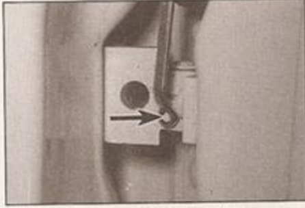
11.4 Loosen the hinge grub screw (arrowed)
