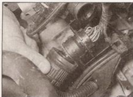
10.8a Disconnecting the main engine wiring harness plug connector . . .
