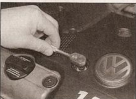
16.3a Unscrew and remove the nuts and washers ...
