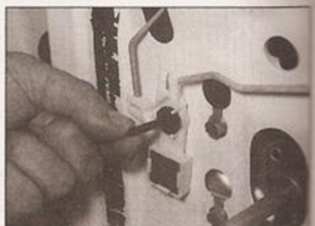
13.18b ... which fits in the centre of the link rod pivot
