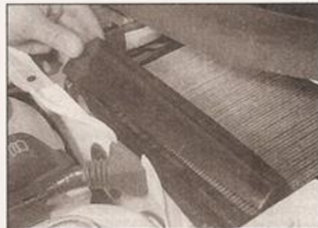
22.5 Removing the pollen filter air deflector plate
