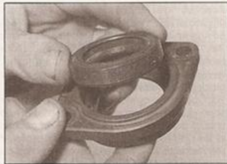
7.3c Press out the oil seal . . .
