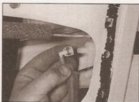
13.15a Pull the vacuum pipe off the central locking unit ...
