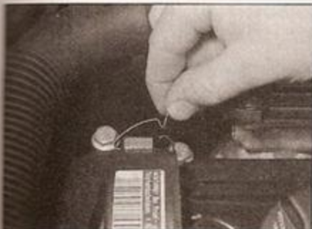
4.14a Prise open the spring clips ...
