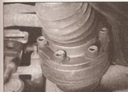
2.7a Inner CV joint splined bolts and retaining plates
