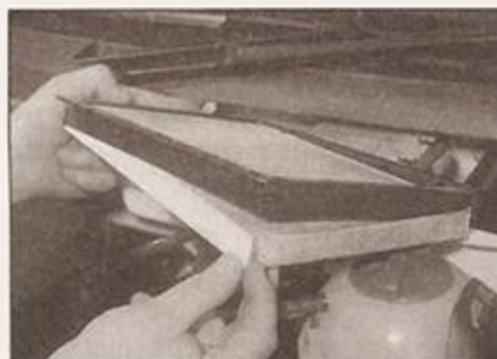
22.7a Separating the pollen filter from the frame
