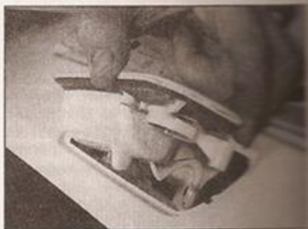
16.7b ... and withdraw the handle from the tailgate
