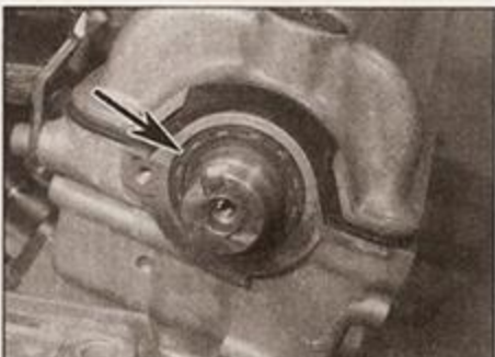
8.3c Camshaft oil seal (arrowed)
