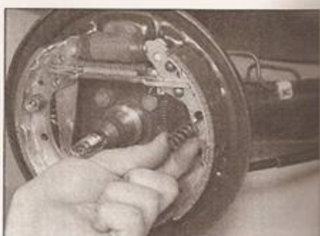
5.7b . . . then lift off the spring . . .
