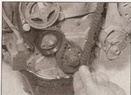
4.20 Engaging the timing belt with the crankshaft sprocket
