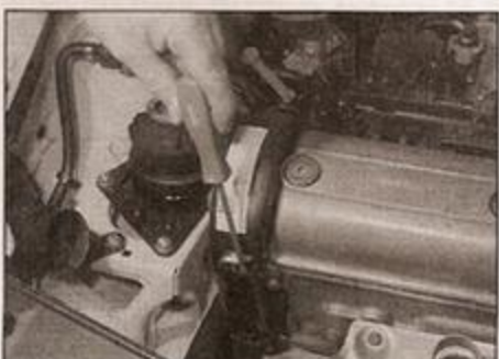
4.11a Release the timing belt upper cover retaining clips . . .
