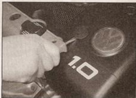
16.2a Prise out the blanking plugs ...
