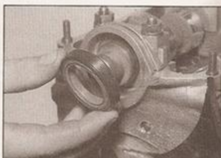
4.73 Fitting a new camshaft oil seal
