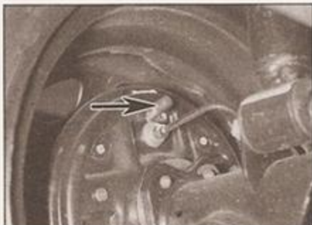
2.14 Dust cap (arrowed) over bleed screw on rear brake wheel cylinder
