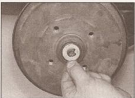
7.4a ... then unscrew the retaining nut and remove the toothed washer
