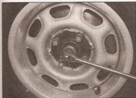
2.1 Remove the trim/hub cap and slacken the driveshaft retaining nut
