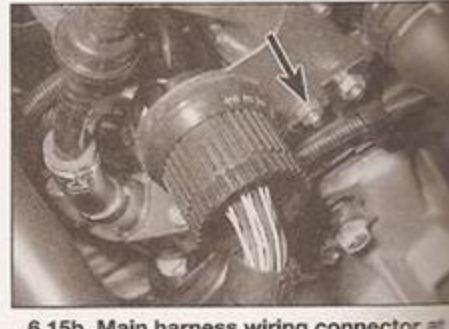
6.15b Main harness wiring connector at left-hand end of cylinder head, and earth connection (arrowed)
