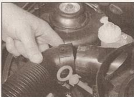
2.4 Slacken the cross-head screw and detach the inlet duct from the housing
