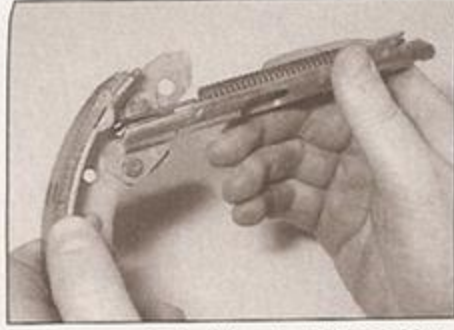
5.15c ... and pivot the strut into position on the shoe
