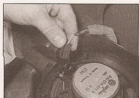
14.3c Disconnect the wiring from the rear of the speaker
