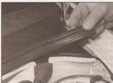
24.2 Pull off the rubber weatherstrip from the top of the bulkhead
