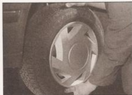
18.4 Check for wear in the hub bearings by grasping the wheel and trying to rock it
