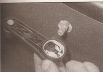
12.4b ... and remove the handle from the splines
