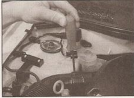
2.4 Slackening the air ducting retaining screw
