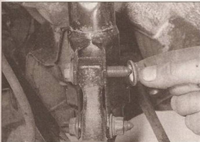
2.4a Loosen and remove the strut-to-swivel hub nuts . . .
