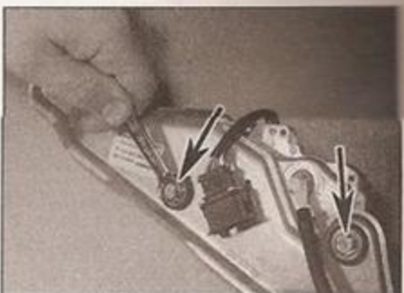
15.6c Wiper motor mounting bolts (arrowed)
