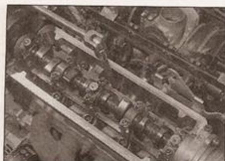
10.20b Loosen the bolts by half a turn at a time, using a suitable splined adapter
