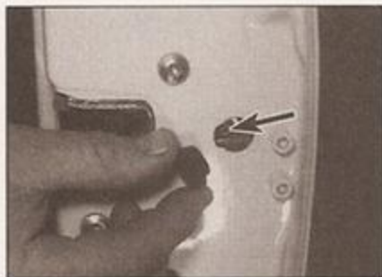
13.30 Door lock adjustment screw (arrowed)
