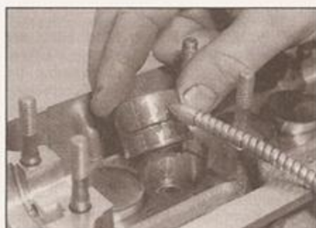
4.64 Fit the tappets into their bores in the cylinder head
