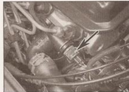
6.10b Coolant temperature sensor (arrowed) - diesel engine models
