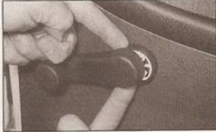
12.4a Slide out the spacer behind the regulator handle (the direction will not necessarily be as shown) ...
