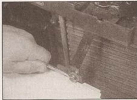
3.6a Remove the bonnet lock support arm securing bolt . . .
