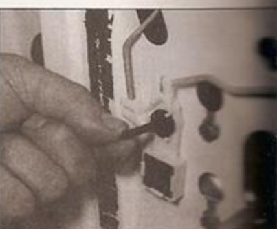
13.18b ... which fits in the central locking link rod pivot
