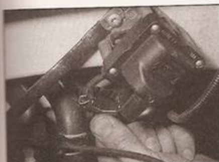
3.4 Disconnect the LT wiring plug from the ignition coil
