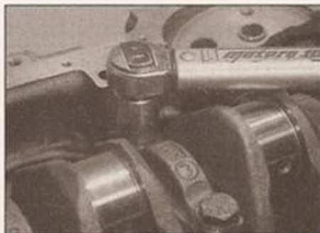
11.19 Tighten the bearing cap bolts to the specified torque
