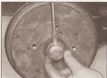
7.2 Lever out the cap from the centre of the brake drum
