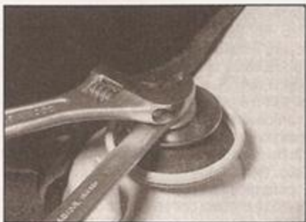
10.6 Hold the piston rod stationary using a suitable spanner, and unscrew the upper mounting nut
