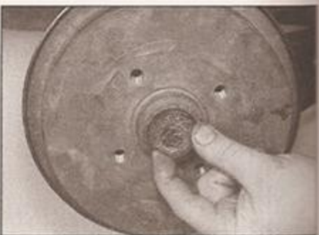
7.4b Withdraw the outer bearing ...
