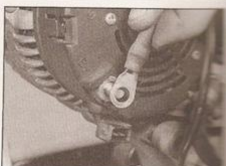
5.4b . . . remove the nut and washers, then disconnect the power cable
