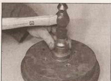
8.4 Drive the new races in squarely, using a socket on the outer edge
