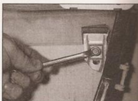
14.6a Loosen the window clamp bolts ...
