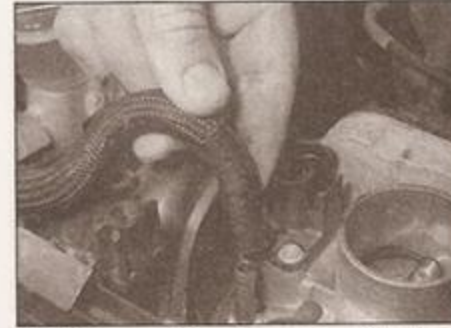
5.5 Disconnect the charcoal canister hose from the stub on the throttle body
