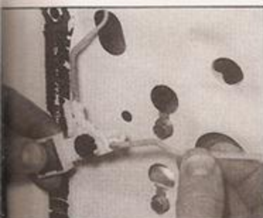
13.18c Unclip the link rods
