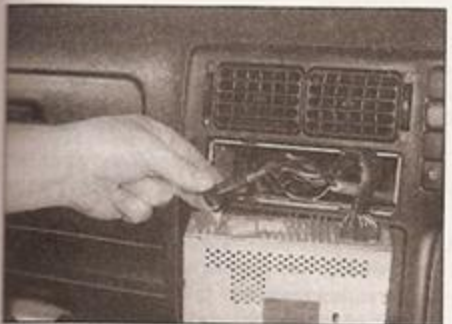
17.4b Disconnect the aerial lead ...
