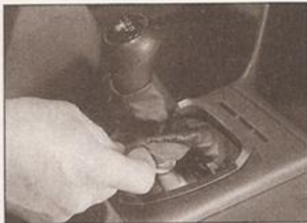
27.1a Unclip the gear lever gaiter ...
