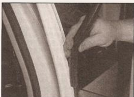
14.10a Pull off the rubber guides in front ...
