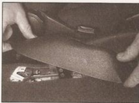
14.4a Pull up the handbrake lever trim . . .
