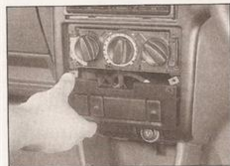
9.3b . . . and withdraw the panel from the fascia
