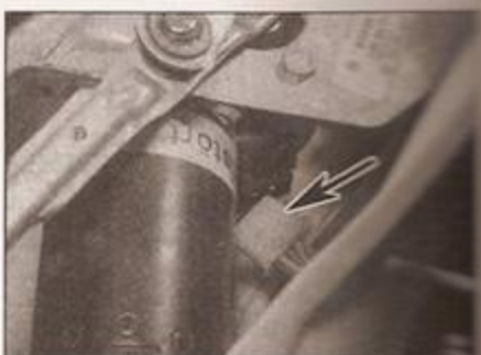
13.8 Wiper motor wiring plug (arrowed)
