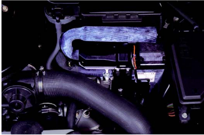
Figure 65: Fuel burning heater
