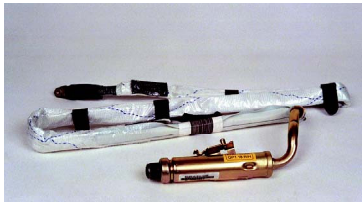
Figure 132 Inflatable tubular structure
