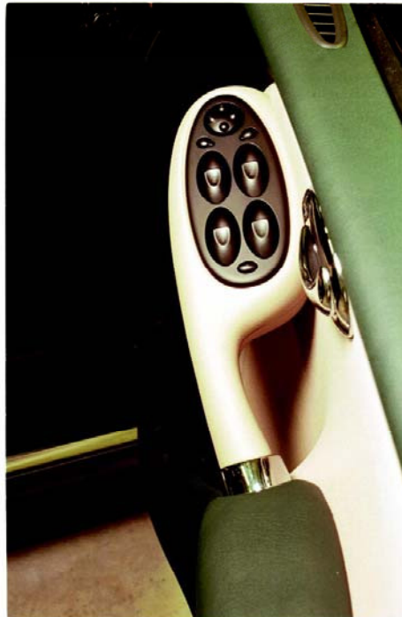
Figure 15: Driver's door switchpack
