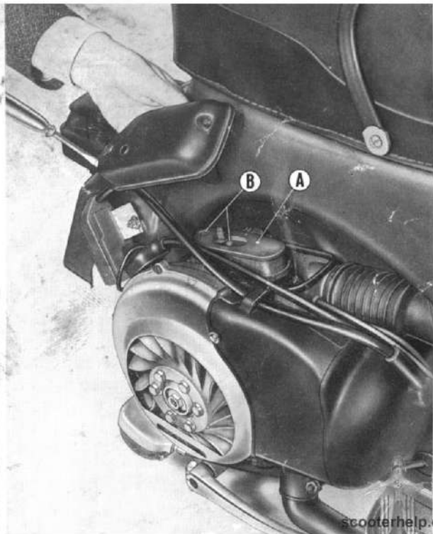
Fig. 14 - Dismantling the air cleaner
