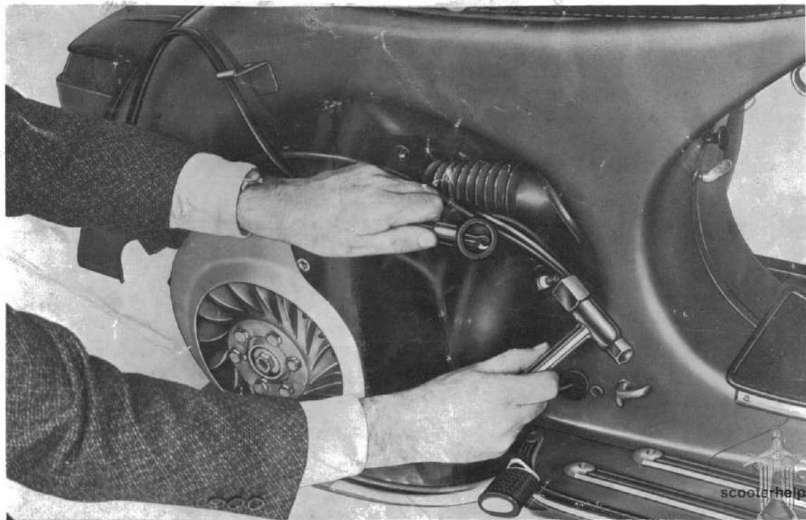
Fig. 15 - Dismantling spark plug
