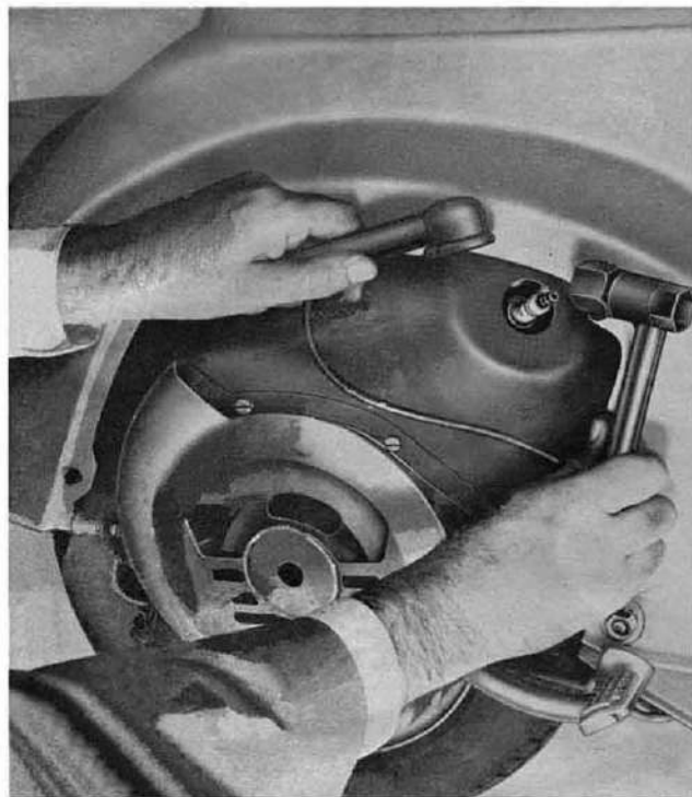
Fig. 10 - Dismantling spark - plug
