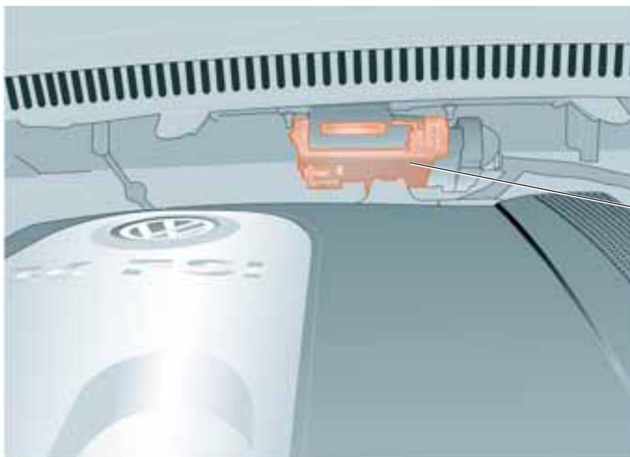
Engine control unit with ambient air pressure sender J220
