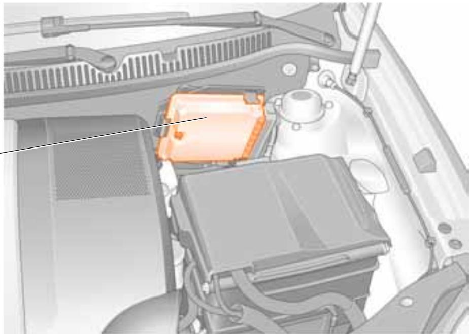
Engine control unit with ambient air pressure sender J220
