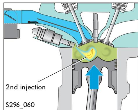
The warmer exhaust gas heats up the catalyst, which allows it to reach its optimal operating temperature.
