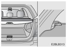
To use the rear shade of the tonneau cover, pull the handle backward and insert the edges into the slots.
