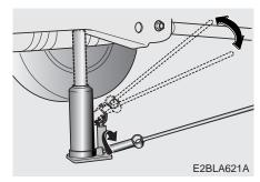
Securely tighten the valve of the jack. Move the jack handle up and down until the top of the jack contacts the proper point and takes on a slight load.
