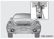
Go to the front of the vehicle, raise the hood slightly, pull the secondary latch inside of the hood center and lift the hood.
