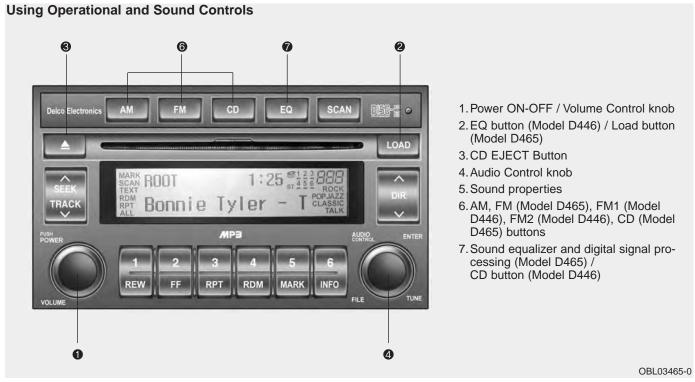
Model shown is Model D465. The buttons on your audio system may differ. For details, see specific descriptions in the following sections.
