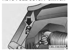
The auto fuel cutoff switch is located on the passenger's side of the engine compartment. In the event of a collision or sudden impact, the auto fuel cutoff device cuts off the fuel supply. If this device is activated, it must be reset by pressing in on the top of the switch before the engine can be restarted.
