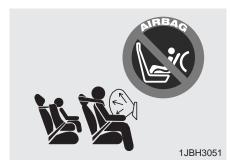
Installing a child restraint on a front passenger seat is extremely dangerous and should never be done.
