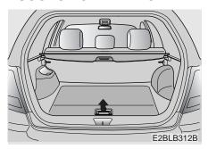
The luggage center box is located under the floor in cargo area. You can place a first aid kit, a reflector triangle, tools, etc. in the box for easy access.
