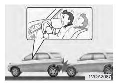
Air bags may not inflate in rear collisions, because occupants are moved backward by the force of the impact. In this case, the air bags do not provide protection.
