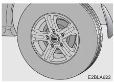
10. Mount the spare tire into position and install the wheel lug nuts with the beveled edge inward.
