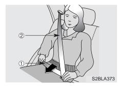
4. Position the lap portion (①) of the belt across your lap as LOW ON THE HIPS as possible to reduce the risk of sliding under it during an accident. Adjust the belt to a SNUG FIT by pulling up on the shoulder portion (②) of the safety belt. The belt retractor is designed to take up excess webbing automatically and to maintain tension on the belt. For your safety, do not put any excess slack into the safety belt at any location.
