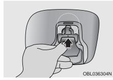
3. Insert the tongue plate into the hole on the belt assembly cover.
