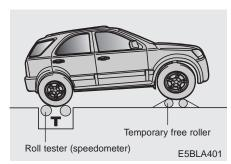
For speedometer test or inspection/ maintenance (I/M) program of full-time 4WD vehicle, use a four wheel chassis dynamometer.
