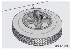
5. Remove the retainer from the center of the spare tire.
