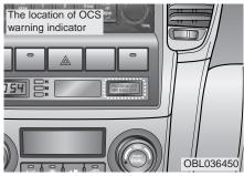
If there is no passenger in the front passenger seat or if the passenger in the front passenger seat is very light, (such as a child), the front **PASSENGER AIR BAG OFF** indicator may illuminate.
