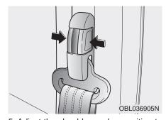
5. Adjust the shoulder anchor position to your size. To raise the anchor position, push the anchor up. To lower the anchor position, press the button and slide the anchor down. After adjustment, make sure the anchor is locked in position.
