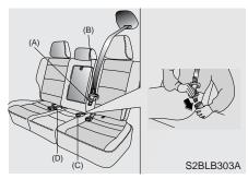
Insert the tongue plate (A) into the open end of the buckle (C) until an audible "click" is heard, indicating the latch is locked. Make sure the belt is not twisted.
