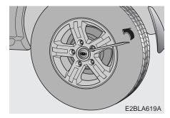
6. Loosen the wheel lug nuts counterclockwise one turn each, but do not remove any nut until the tire has been raised off the ground.
