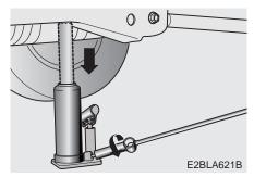
11. Gradually loosen the valve of the jack with the groove on the jack handle to lower the vehicle.
