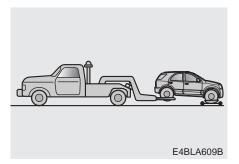
On 4WD vehicles, your vehicle must be towed with a wheel lift and dollies or flatbed equipment with all the wheels off the ground.
