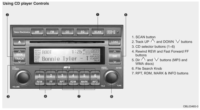
The functions of the buttons and controls described below are only applicable when you select the CD mode by pressing the CD selector button (for both Model D446 and Model D465).
