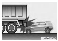
Just before impact, drivers often brake heavily. Such heavy braking lowers the front portion of the vehicle causing it to "ride" under a vehicle with a higher ground clearance. Air bags may not inflate in this "under-ride" situation because deceleration forces that are detected by sensors may be significantly altered by such "under-ride" collisions.
