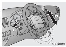
To change the steering wheel angle, pull up the lock release lever (1), adjust the steering wheel to the desired angle (2), then release the lock-release lever to lock the steering wheel in place. Be sure to adjust the steering wheel to the desired position before driving.
