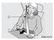
4. Position the lap portion (①) of the belt across your lap as LOW ON THE HIPS as possible to reduce the risk of sliding under it during an accident. Adjust the belt to a SNUG FIT by pulling up on the shoulder portion (②) of the safety belt. The belt retractor is designed to take up excess webbing automatically and to maintain tension on the belt. For your safety do not put any excess slack into the safety belt.
