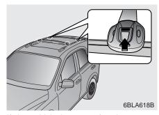
If the vehicle has a roof rack, you can load things on top of your vehicle. The two cross bars on the roof rack can be repositioned forward or rearward for conveniently loading cargo or luggage. With an assistant on the opposite side of the vehicle, press and hold the slider lock buttons on each side, then move the cross bar to the desired position. Release the buttons and lock the cross bar by moving the crossbar slightly forward or rearward.
