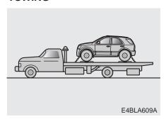
If emergency towing is necessary, we recommend having it done by an authorized Kia dealer or a commercial tow-truck service. Proper lifting and towing procedures are necessary to prevent damage to the vehicle. The use of wheel dollies or flatbed is recommended.
