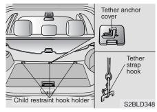
Securing a child restraint seat with "Tether Anchor" system
