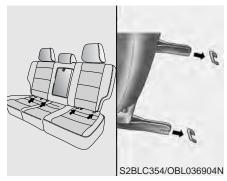
LATCH anchors have been provided in your vehicle. The LATCH anchors are located in the left and right outboard rear seating positions. Their locations are shown in the illustration. There is no LATCH anchor provided for the center rear seating position.
