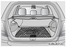
To keep items from shifting in the cargo area, you can use the four rings located in the cargo area to attach the luggage net.
