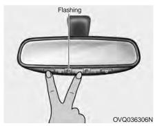
When programming the buttons for the first time, press and hold the left and center buttons (♠,♠) simultaneously until the indicator light begins to flash after approximately 20 seconds. (This procedure erases the factory-set default codes. Do Not perform this step to program additional hand-held transmitters.)
