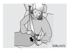
3. Insert the tongue plate (①) into the open end of the buckle (②) until an audible "click" is heard, indicating the belt is locked in the buckle.
