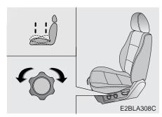
Adjusting the height of seat cushion (for driver's seat)
