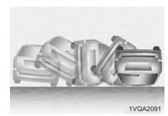
Air bags may not inflate in rollover accidents. Air bag deployment would not provide proper protection to the occupants.
