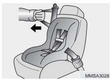
3. Pull the shoulder portion of the safety belt all the way out. When the shoulder portion of the safety belt is fully extended, it will shift the retractor to the "Auto Lock" (child restraint) mode.
