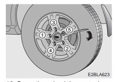
12. Once the wheel lug nuts have been tightened, lower the vehicle fully to the ground and continue to tighten the lug nuts until they are fully secured. Tighten the wheel lug nuts firmly in a "star" pattern.
