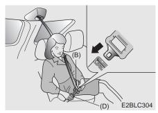
3. Pull the tongue plate (B) and insert the tongue plate (B) into the open end of the buckle (D) until an audible "click" is heard, indicating the latch is locked. Make sure the belt is not twisted.
