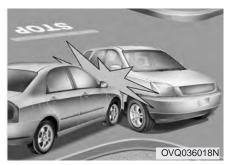
Front air bags may not inflate in side impact collision, because occupants move to the direction of the collision, and thus front air bag deployment does not provide proper protection.
