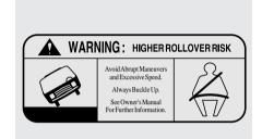
To remind you of the danger of the rollover, the rollover warning label is adhered to the driver's sunvisor. If you close the driver's sunvisor, you can see the rollover warning label which is located at the side of the air bag warning label.
