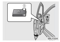
To lock a door without the key, push the inside door lock switch (①) to the "LOCK" position and close the door (②).
