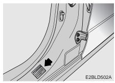
All specifications (sizes and pressures) can be found on a label attached to the front driver's door sill.
