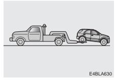
On 2WD vehicles, it is acceptable to tow the vehicle with the front wheels on the ground (without dollies) and the rear wheels off the ground.
