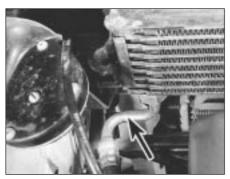
6B.24A Oil cooler pipe connection (arrowed)
