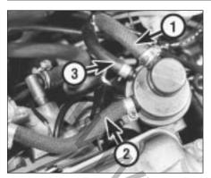
5C.9 Fuel hose identification at pump; inlet hose (1), hose to carburettor (2), return hose (3)
