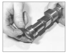
5B.26A Camshaft oil seal
