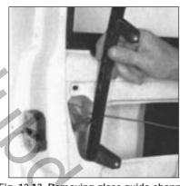
Fig. 12.13 Removing glass guide channel (Sec 12)
