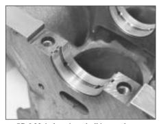
5D.2 Main bearing shell in crankcase
