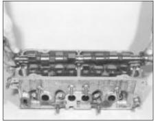
5B.24 Removing the camshaft
