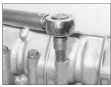
27.18 Tightening a camshaft carrier bolt
