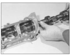
7B.93 Withdrawing the camshaft from its housing
