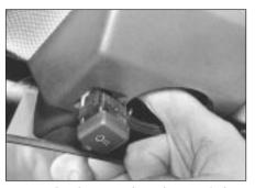
15.81 Roof-mounted spotlamp switch removal
