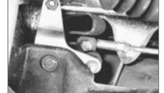
12B.31 Gear control and selector link rod joints
