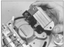
5.3B Removing alternator brush holder
