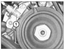
Fig. 13.77 Crankshaft pulley timing mark aligned with timing pointer - Microplex ignition system (Sec 10)
