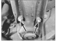
16.4 Anti-roll bar fixing nuts (arrowed)
