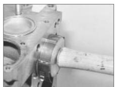
5B.97 Fitting a piston/connecting rod
