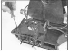
Fig. 2.9 Control lever platform screw (Sec 13)
