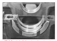
5D.3 Crankshaft thrust washer at centre bearing
