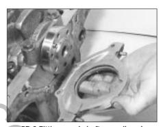
5D.9 Fitting crankshaft rear oil seal retainer
