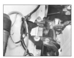
44.8C Right-hand engine mounting brackets
