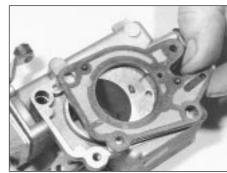
9B.26E Throttle valve block gasket on the Weber 32 TLF carburettor
