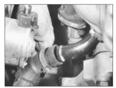
5C.7A Radiator hose connection to coolant distribution tube
