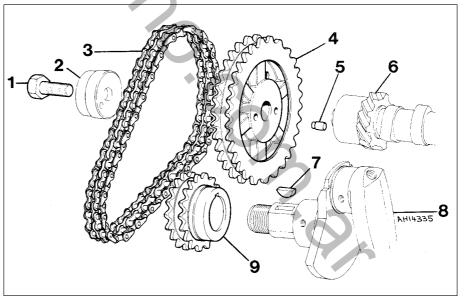
Fig. 1.6 Timing chain and sprockets (Sec 6)
