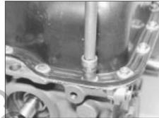
42.14 Tightening sump pan bolt
