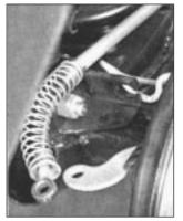
Fig. 11.11 Handbrake cable and lever at brake backplate (Sec 11)
