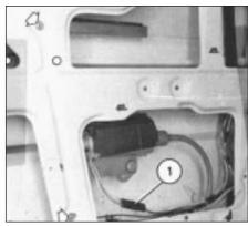
Fig. 9.11 Power-operated window motor (Sec 31)
