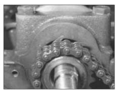
6.13C Self-tensioning links on inside of chain
