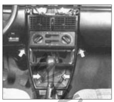
Fig. 13.32 Heater unit facia to main facia retaining screw locations (arrowed) (Sec 8D)
