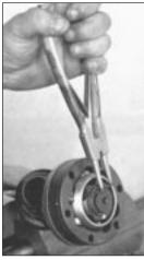
Fig. 13.99 Extracting the CV joint circlip -Turbo ie models (Sec 13)
