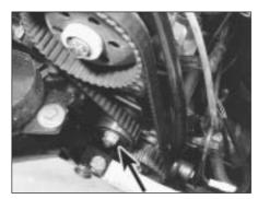
6B.20 Belt tensioner pulley locknut (arrowed)
