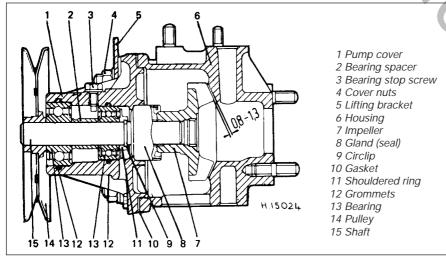
Fig. 2.5 Sectional views of 1116 cc and 1301 cc engine coolant pump (Sec 9)
