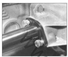
9.4 Coolant distribution tube at rear of pump
