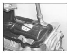
42.26 Tightening a camshaft carrier cover nut
