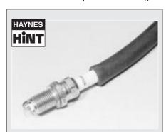
It's often difficult to insert spark plugs into their holes without cross-threading them. To avoid this possibility, fit a short piece of rubber hose over the end of the spark plug. The flexible hose acts as a universal joint, to help align the plug with the plug hole. Should the plug begin to cross-thread, the hose will slip on the spark plug, preventing thread damage.
