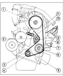
Fig. 1.29 Timing belt arrangement (Sec 28)
