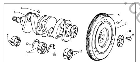
Fig. 1.24 Crankshaft and flywheel (Sec 16)
