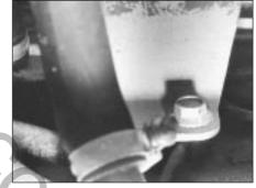
9F.21 Exhaust manifold support bracket
