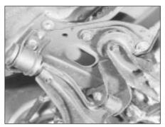
6.3 Track control arm inboard fixing
