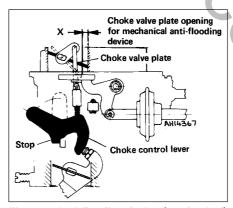
Fig. 3.26 Anti-flooding device (mechanical) adjustment diagram (Weber 30/32 DMTR 90/250) (Sec 14)
