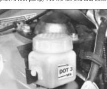
11.7A Clutch hydraulic fluid reservoir showing MIN and MAX markings
