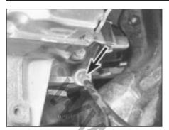
23.3 Speedometer cable connector at transmission
