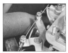
9B.37C Choke cable connection on the Weber 30/32 DMTE carburettor
