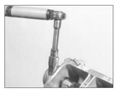
7B.85 Tightening a camshaft housing securing bolt
