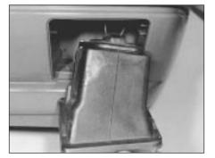
15.37B . . . and withdraw the front fog lamp unit . . .
