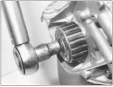
5D.16B Tightening the crankshaft sprocket bolt
