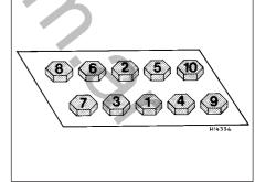
Fig. 1.30 Cylinder head bolt tightening sequence (Sec 29)
