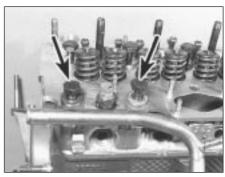
7.24B Cylinder head bolts holding coolant pipe
