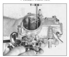
Fig. 3.15 Choke valve gap opening (Weber 32 ICEV 50/250) (Sec 9)
