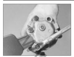
7B.171 Undo the oil pump cover bolts
