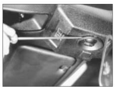
15.82 Roof-mounted clock retaining screw removal
