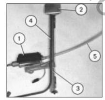
Fig. 9.12 Power operated window components (Sec 31)
