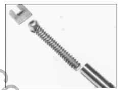
5B.72B Oil pump relief valve components
