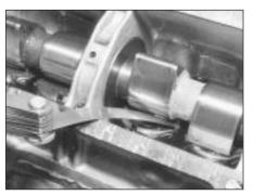
25.4 Checking a valve clearance
