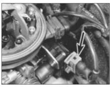
7C.10 Engine idle speed actuator/SPi unit lead connection (arrowed)
