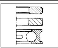
Fig. 13.5 Piston ring arrangement on the 999 cc engine (Sec 5B)
