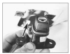
17.13 Tailgate handle link rod (arrowed)
