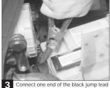
Connect one end of the black jump lead to the negative (-) terminal of the booster battery
