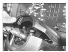
5.2 Removing steering column shrouds
