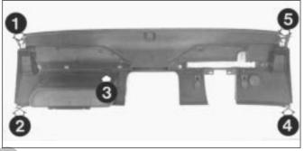
Fig. 12.20 Rear view of facia panel showing fixing screw locations (Sec 22) 1 and 5 Clips 2, 3 and 4 Screws
