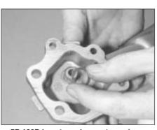
7B.180B Locate spring seat over boss within pump cover . . .
