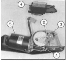
Fig. 9.6 Windscreen wiper motor components (Sec 25)
