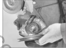
7B.35 Crankshaft pulley removal
