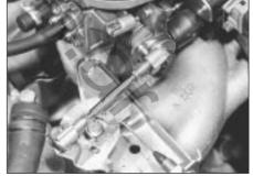
9D.22 Accelerator control rod and cable connections
