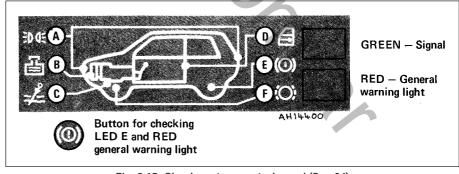
Fig. 9.15 Check system control panel (Sec 34)
