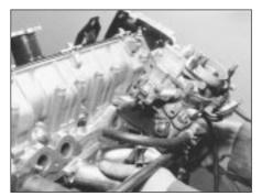
19.4C Fitting intake manifold complete with carburettor
