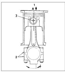
Fig. 13.6 Piston/connecting rod correctly assembled - 999 and 1108 cc engine (Sec 5B)
