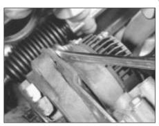
8C.53 Tightening the alternator adjuster nut
