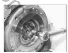
5D.14 Tightening a flywheel bolt
