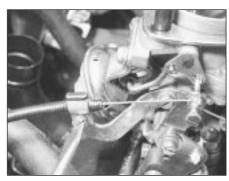
18.2 Choke cable at carburettor
