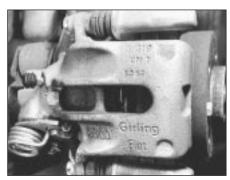
14B.23 Rear brake pad inspection aperture
