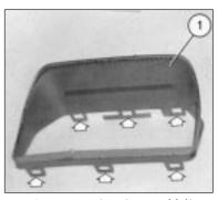
Fig. 9.4 Instrument hood cover (1) (Sec 21)
