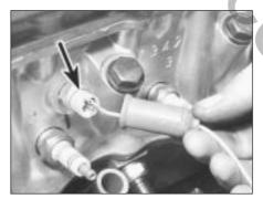
44.26B Coolant temperature switch
