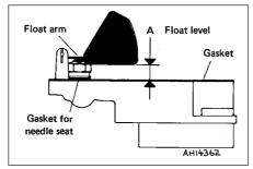
Fig. 3.16 Float setting diagram (Solex C32 DISA 11) (Sec 10)
