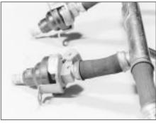
9C.81A Fuel injectors attached to fuel rail
