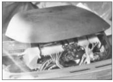
21.2 Removing instrument panel hood cover
