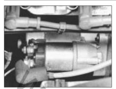
12B.24A Starter motor electrical connection . . .
