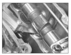
5B.1A Checking a valve clearance
