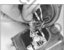
15.39 . . . detach the wires, extract the bulb
