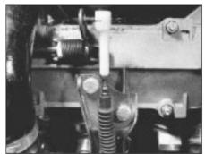
9C.99A Throttle cable and end fitting (primary section)
