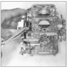
Fig. 3.23 Bending throttle lever stop (Weber 30/32 DMTR 90/250) (Sec 14)
