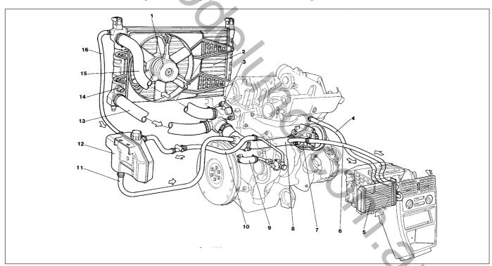
Fig. 13.30 Cooling system circuit - 1372 cc Turbo ie engine (Sec 8C)
