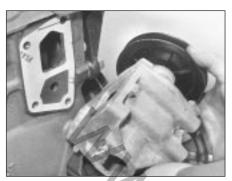
9.21 Fitting coolant pump (1116 cc engine)
