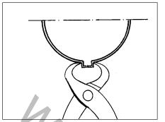
Fig. 13.97 Crimping the driveshaft boot securing band (Sec 13)
