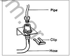
Fig. 8.11 Typical hydraulic hose connection (Sec 11)
