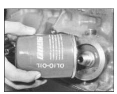
2.8 Screwing on the oil filter (903 cc)
