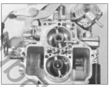
9B.34E Weber 30/32 DMTE carburettor from above (with cover removed)
