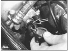
9F.5 Maximum air pressure switch (arrowed)
