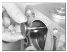
17.17B Inserting a valve into its guide
