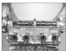
5B.51 Fitting the cylinder head
