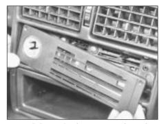
12.6B Removing heater control panel escutcheon
