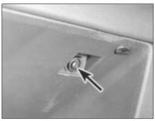
22.5A Facia fixing screw inside glovebox
