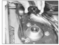
16.7 Suspension strut upper mounting nuts, showing bracket and cable clip on the 1372 cc ie model
