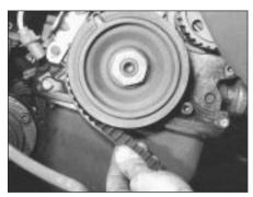
6B.19B Removing the timing belt
