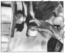
5C.24B Gearchange rod with ball socket connection
