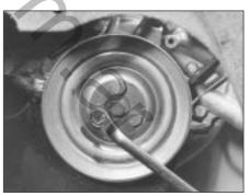
5B.7 Unscrewing the crankshaft pulley bolts
