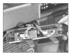
15.63 . . . and withdraw the auxiliary control panel
