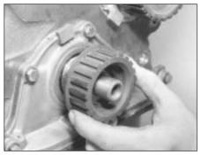
42.20 Fitting crankshaft timing belt sprocket
