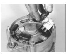
15.16B Removing the alternator brush holder
