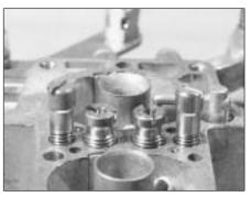
9B.41 Jets on the Weber 30/32 DMTE carburettor (top cover removed)
