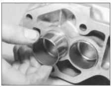
39.10 Cam followers fitted to camshaft carrier
