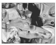
5C.26 Left-hand rear (lower) transmission mounting disconnected
