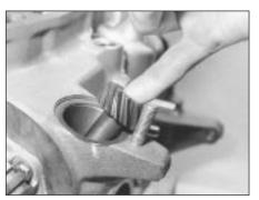
42.15 Fitting oil pump driveshaft
