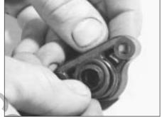
9C.95C Fuel injector insulator seal
