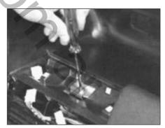
Fig. 13.31 Removing the heater unit-tofacia upper retaining screw (Sec 8D)
