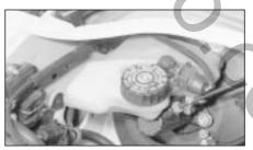
☐ The fluid reservoir must be secure and the fluid level must be between the upper (A) and lower (B) markings.
