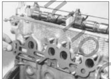
5D.25A Inlet manifold gasket
