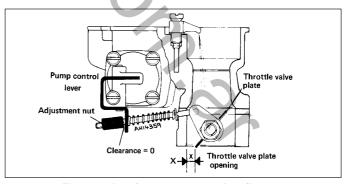
Fig. 3.11 Accelerator pump setting diagram (Weber 32 ICEV 50/250) (Sec 9)
