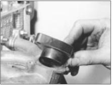
9B.19 Carburettor insulator block
