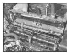
5B.20B Removing the camshaft cover
