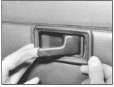
11.3A Removing remote control handle escutcheon
