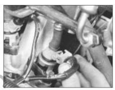
9C.81C Injector wiring plug refitting
