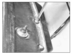
25.4 Removing windscreen wiper motor mounting screws
