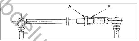
Fig. 13.95 Gear selector adjustable rod (C514 type transmissions)
