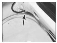
17.15 Tailgate release cable (arrowed)
