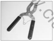
Piston ring removal/installation tool
