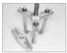
Three-legged hub and bearing puller
