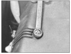
9A.6 Air cleaner casing nut on the 999 cc
