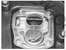
9A.9A Circular type air cleaner fixing nuts
