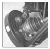
Fig. 1.18 Hub carrier detached from strut clamp (Sec 13)
