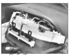
15.59A . . . withdraw the instrument panel . . .
