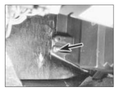
12.10 Heater lower mounting bolt
