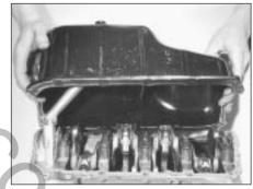
5C.60A Removing the sump pan
