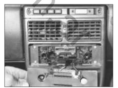
15.69B . . . and withdraw the heater control panel
