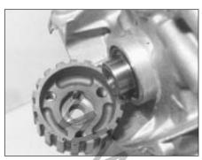
5D.16A Crankshaft sprocket showing integral key
