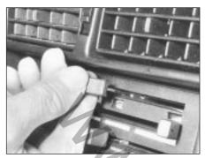
12.5 Pulling off heater control lever knob
