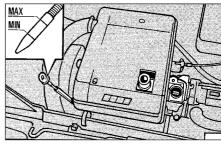
Fig. 13.15 Engine oil level dipstick location and level markings on the 1372 cc ie and Turbo ie engines (Sec 7A)
