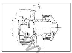
Fig. 13.28 Sectional view of the coolant pump on the 999 and 1108 cc engines (Sec 8A)
