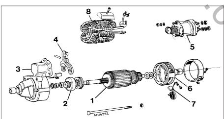
Fig. 9.2 Exploded view of typical starter motor (Sec 9)
