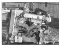
5C.34 Lifting out the engine and transmission
