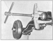
Fig. 11.10 Method of renewing trailing arm bush (Sec 10)
