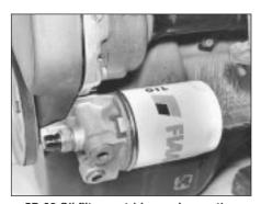
5D.29 Oil filter cartridge and mounting base
