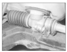
6.4 Steering rack housing at pinion end
