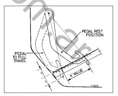
Fig. 13.87 Clutch pedal adjustment diagram - cable clutch (Sec 11)
