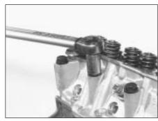
7B.121A Tighten main cylinder head bolts to specified torque . . .
