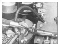
Fig. 13.60 Disconnecting the injector fuel supply pipe and fuel pressure regulator pipe on the 1372 cc Turbo ie engine (Sec 9E)
