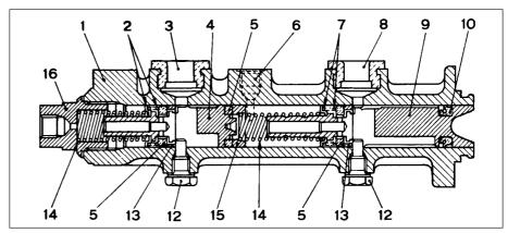
Fig. 8.5 Sectional view of master cylinder (Sec 9)
