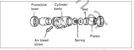
Fig. 8.4 Exploded view of a rear wheel cylinder (Sec 7)
