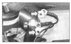
Fig. 13.59 Disconnecting the earth leads (arrowed) on the 1372 cc Turbo ie engine (Sec 9E)
