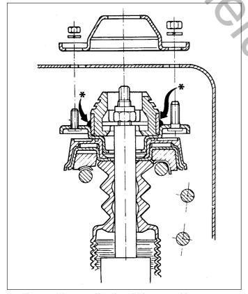
Fig. 11.4 Waterproof bead applied to strut with top cover removed (Sec 3)
