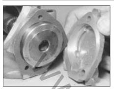
27.13A Removing camshaft end cover
