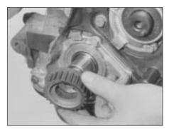
7B.47 Refitting the crankshaft sprocket
