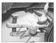
2.2 Disconnecting a tie-rod end balljoint
