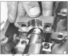
5B.23D Camshaft bearing cap showing short and long positioning dowels for correct fitting
