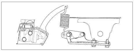
Fig. 8.8 Pressure regulating valve (Sec 10)
