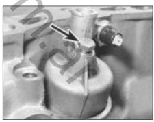
42.16B Crankcase breather and retaining bolt
