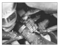
8C.21B Cooling fan switch wiring connector
