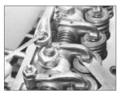
5.7 Adjusting a valve clearance
