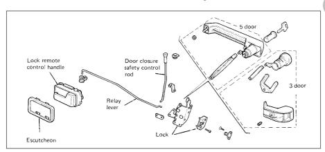
Fig. 12.15 Door lock components (Sec 12)
