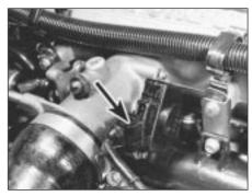
9C.90 Throttle position switch (wiring plug arrowed)
