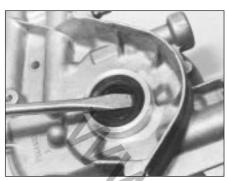
5B.77A Removing the oil pump seal
