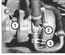
9F.18B Turbocharger connections
