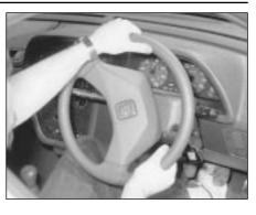
movement of the steering wheel, indicating wear in the column support bearings or couplings.
