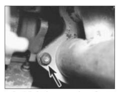
9F.16A Turbocharger-to-exhaust flange nut (arrowed)
