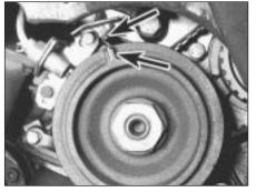
10.39 Crankshaft pulley timing marks (arrowed)
