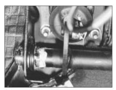
14B.46 Left-hand end of brake pedal cross-shaft
