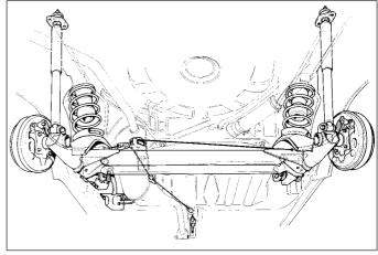
Fig. 11.1 Front suspension arrangement (Sec 1)
