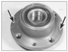
4.11 Rear hub showing cut-outs on rear face for shoe self-adjuster bosses
