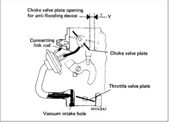
Fig. 3.13 Anti-flooding device (Weber 32 ICEV 50/250) (Sec 9)
