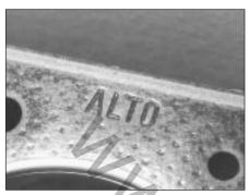
29.21A Cylinder head gasket top face marking
