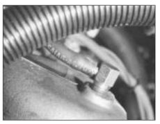
9C.70B Fuel pressure regulator vacuum hose connection at the inlet manifold
