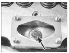
7.24A Cylinder head bolt in intake manifold
