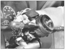
15.47B . . . and remove the column switch
