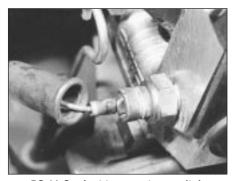
5C.16 Coolant temperature switch
