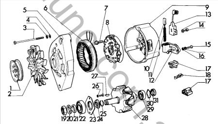
Fig. 9.1 Exploded view of typical alternator (Sec 5)
