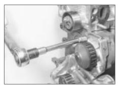
8A.17B Tightening the coolant pump bolts
