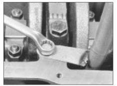
42.12 Tightening oil drain pipe bolt
