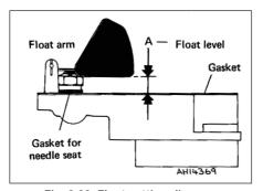
Fig. 3.28 Float setting diagram (Solex C30-32 CIC/1) (Sec 14)
