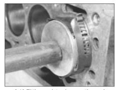
9.19 Fitting a piston/connecting rod
