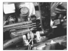
9C.88B Supplementary air valve (arrowed)
