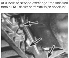
12B.33 Lower cover plate and retaining bolts (arrowed)
