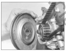
5D.22 Crankshaft pulley installation
