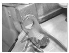
44.2 Lifting lug at bellhousing bolt
