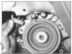
6B.19A Removing the TDC sensor
