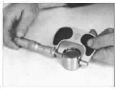
Fig. 13.8 Checking a cam follower for ovality - 999 and 1108 cc engine (Sec 5C)
