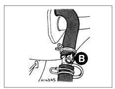
Fig. 2.2 Plug (B) in heater hose (Sec 2)
