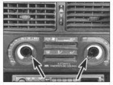
15.69A . . . undo the retaining screws (arrowed)
