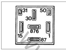
Fig. 13.43 System control relay connector plug terminals 1301 cc Turbo ie engine (Sec 9C)
