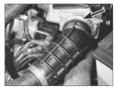
9C.56 Air intake duct at airflow meter (securing clip arrowed)
