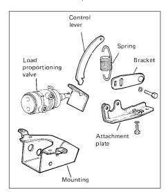
Fig. 8.9 Components of the pressure regulating valve (Sec 10)
