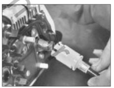
23.2 Speedometer cable connector at head
