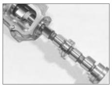
27.13B Withdrawing camshaft from carrier
