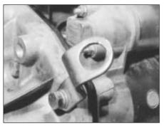
5D.38 Lifting eye on flywheel housing flange
