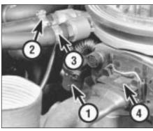
9D.8 Atmospheric air intake for air temperature sensor (1). Also shown are the supply and return fuel line connections (2 and 3) and the throttle position sensor (4)
