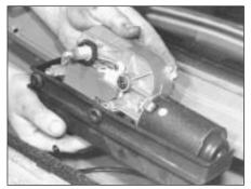
15.98B . . . separate the wiper motor from its cover . . .
