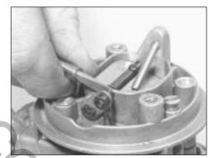
9B.23B Disconnecting the choke linkage on the Weber 32 TLF carburettor
