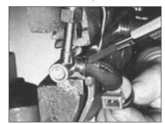
Fig. 13.61 Cutting free the hose from an injector on the 1372 cc Turbo ie engine (Sec 9E)
