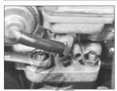
9B.37F Unscrewing a carburettor fixing nut
