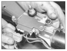
15.98C . . . and detach the wiring connector
