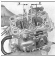
Fig. 3.24 Throttle valve plate openings (Weber 30/32 DMTR 90/250) (Sec 14)
