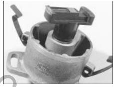
10.41A Distributor body showing elongated slots in the mounting lugs
