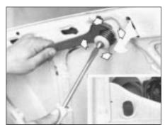
Fig. 12.2 Adjusting bonnet lock striker (Sec 8)
