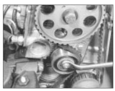
5B.9 Releasing the timing belt tensioner nut
