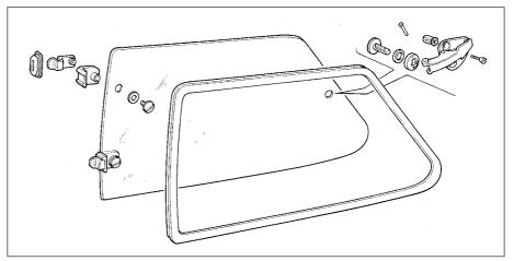
Fig. 12.18 Components of opening side window (Sec 18)
