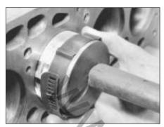
32.14 Fitting piston into cylinder bore
