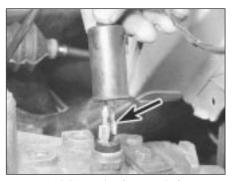
44.22A Reversing lamp switch on transmission
