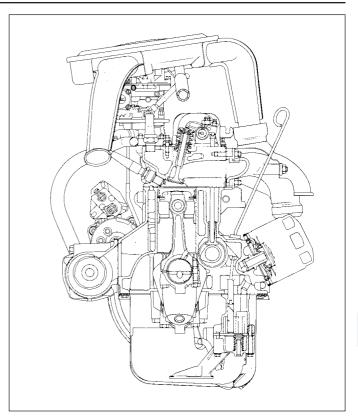
Fig. 1.2 Cross-section of 903 cc engine (Sec 1)
