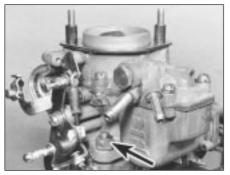
8.6 Carburettor mounting flange nut
