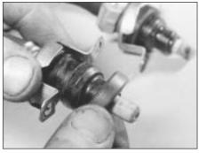
9C.95A Fuel injector large seal
