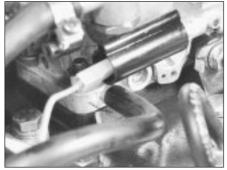
9B.37D Electrical lead to automatic antiflood device on the Weber 30/32 DMTE carburettor
