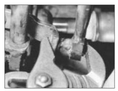
5D.45 Connecting ball socket type gearchange rod
