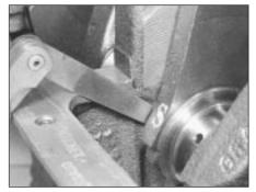
20.10 Checking crankshaft end float
