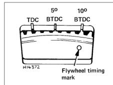
Fig. 4.5 Flywheel housing timing marks (Sec 4)
