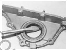
42.7A Removing oil seal from carrier
