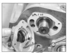
42.10A Auxiliary shaft end plate and
