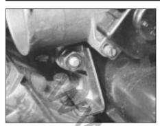
9C.78 Throttle valve housing support bracket
