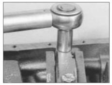
20.9 Tightening main bearing cap bolts
