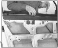
Fig. 12.7 Removing door weatherseal (Sec 12)
