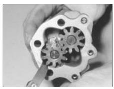
7B.176 Check gear-to-body clearance
