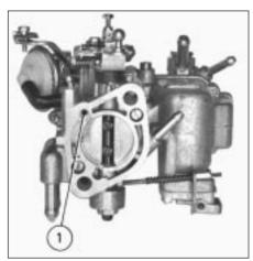
Fig. 3.14 Anti-flooding device vacuum intake (Weber 342 ICEV 50/250) (Sec 9)
