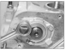
42.10B Tightening auxiliary shaft end plate bolt
