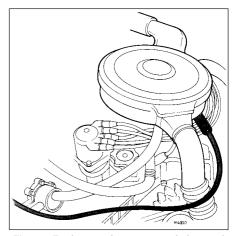
Fig. 3.9 Fuel return hose correctly located (Sec 8)
