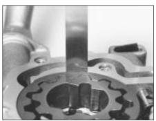
5B.74A Checking the oil pump gear-tohousing clearance
