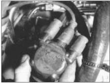
10.38 Removing the distributor cap
