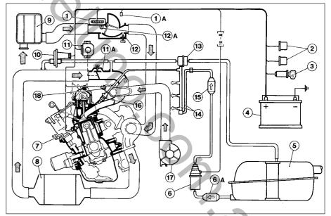
Fig. 13.48 Bosch L3.1 Jetronic fuel injection system - 1372 cc Turbo ie engine (Sec 9E)
