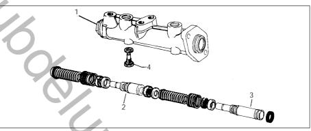
Fig. 8.6 Exploded view of master cylinder (Sec 9)
