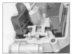
9B.26A Floats and pivot pin arrangement on the Weber 32 TLF carburettor
