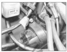
9D.15 Secondary fuel filter element
