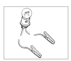
A simple test lamp is useful for checking electrical faults
