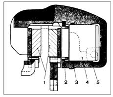
Fig. 8.3 Sectional view of caliper (Sec 5)
