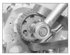
42.11 Tightening camshaft sprocket bolt. Note sprocket locking device
