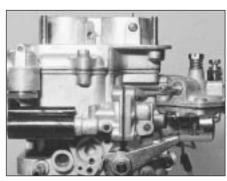
9B.34A Weber 30/32 DMTE carburettor from anti-flood device link side
