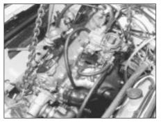
44.8A Raising engine/transmission into engine compartment
