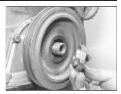
42.21 Crankshaft pulley and nut
