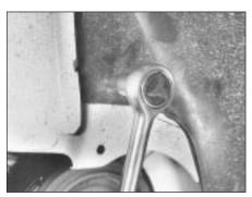
10.4A Unscrewing wing shield screw
