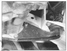
44.9A Engine/transmission lower mounting
