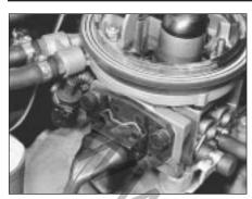
7C.20 Fuel injector wiring connection
