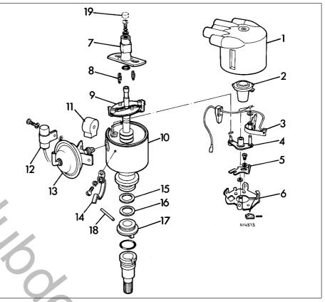
Fig. 4.6 Exploded view of typical Ducellier distributor (Sec 7)
