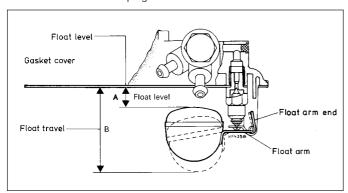
Fig. 3.10 Float setting diagram (Weber 32 ICEV 50/250) (Sec 9)
