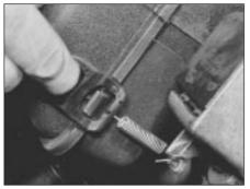
9D.17A Release the air cleaner end cover retaining clips . . .
