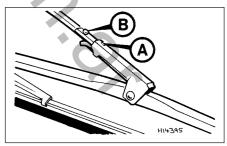
Fig. 9.7 Tailgate wiper blade fixing (Sec 26)
