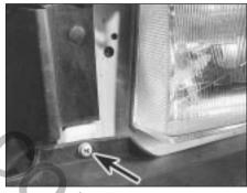
17.24 Front bumper upper mounting screw (arrowed)
