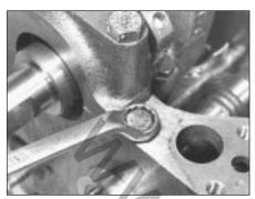
20.17 Camshaft front bearing lockscrew
