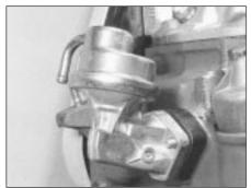
3.6A Fuel pump on mounting studs
