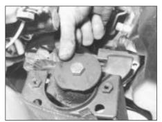
5C.31A Right-hand engine mounting disconnected
