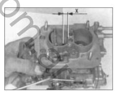
Fig. 3.32 Choke valve plate setting (Solex C30-32 CIC/1) (Sec 15) X = 4.75 to 5.25 mm (0.187 to 0.207 in)
