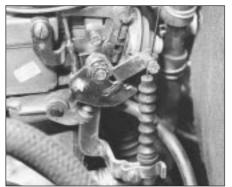
5C.12 Choke cable connection at carburettor
