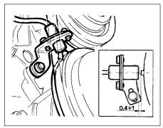
Fig. 4.11 TDC sensor gap (Sec 10)
