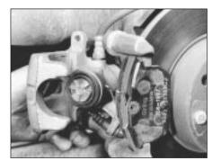
14B.26 Withdrawing the rear brake caliper
