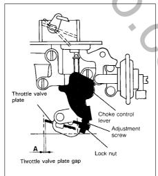
Fig. 13.37 Fast idle adjustment - Weber 32 TLF carburettor (Sec 9B)
