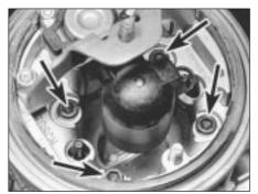
9D.44 Injector unit retaining screws (arrowed)
