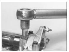
5B.23B Unscrewing the camshaft bearing/banjo union bolt
