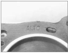
5B.50B Cylinder head gasket top surface marking
