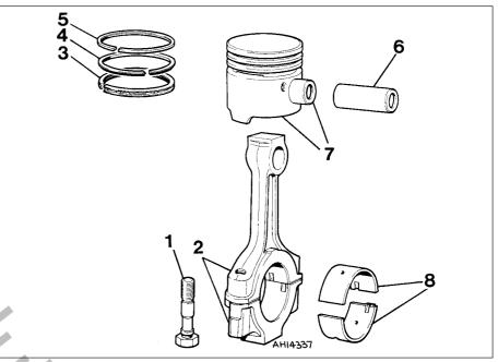
Fig. 1.8 Piston/connecting rod components (Sec 9)
