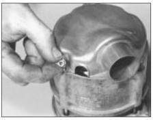
15.12B Alternator rear cover and fixing nut
