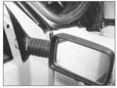
24.4 Withdrawing exterior mirror and trim plate
