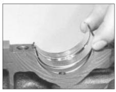
20.1 Fitting a main bearing shell
