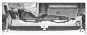
Fig. 12.5 Front bumper lower screws (Sec 9)
