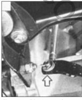
Fig. 13.24 Disconnect the gear selector rod at the connection indicated on the 1372 cc ie and Turbo ie engines (Sec 7C)
