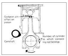
Fig. 1.26 Piston/connecting rod relationship (Sec 18)
