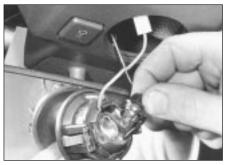
15.80B Roof-mounted spotlamp bulb removal
