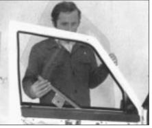
Fig. 12.8 Removing door glass (Sec 12)
