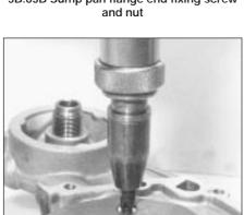
5B.73 Removing the oil pump rear cover plate screws
