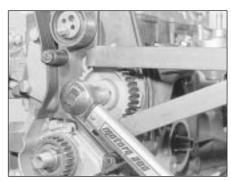
7B.46 Tightening the auxiliary shaft sprocket bolt
