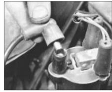
5C.15 Ignition coil HT lead connection
