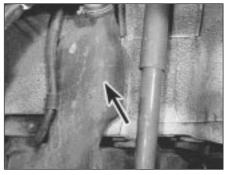
9C.101 Fuel tank anti-blow-back compartment (arrowed)
