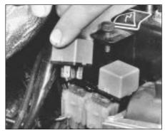
9D.27 Fuel pump relay removal
