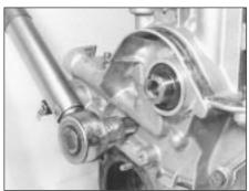
5D.12B Tightening an oil pump bolt
