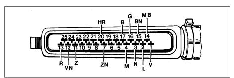
Fig. 13.80 Microplex ignition system ECU multipin connector (Sec 10)
