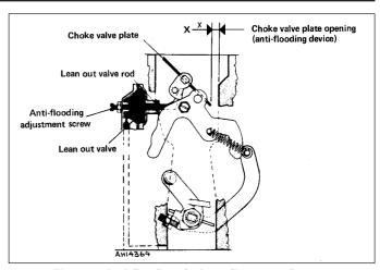
Fig. 3.19 Anti-flooding device adjustment diagram (Solex C32 DISA 11) (Sec 10)
