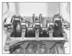
5D.4 Fitting the crankshaft
