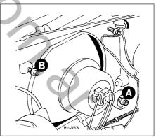
Fig. 9.3 Headlamp beam adjustment screws (Sec 17)
