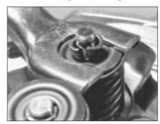
39.2 Valve spring compressor and split collets
