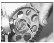
5B.22C Camshaft sprocket showing integral key (arrowed)
