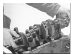
7D.10 Lower the crankshaft into position
