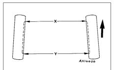
Fig. 10.8 Front wheel alignment diagram (Sec 8)
