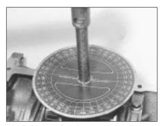
5D.7B Angle-tightening a main bearing cap bolt
