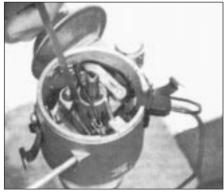
Fig. 4.4 Adjusting Marelli type contact breaker points gap (Sec 2)
