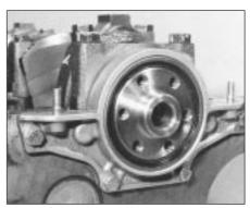
20.11B Crankshaft oil seal and carrier fitted
