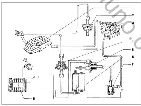
Fig. 13.46 Fuel evaporation control system (Sec 9D)
