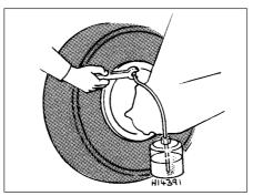
Fig. 8.12 Bleeding a rear wheel cylinder (Sec 12)
