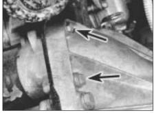
12B.24B . . . and retaining bolts (arrowed) on the 1372 cc ie engine
