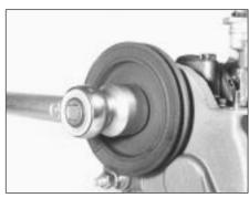
20.23 Tightening crankshaft pulley nut
