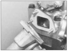
4.4 Fitting thermostat housing (1116 cc engine)
