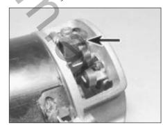
9.4 Starter motor brush partly withdrawn
