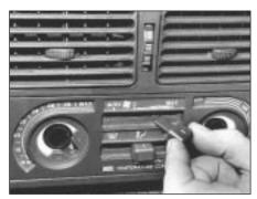
15.68 Remove the control knobs . . .
