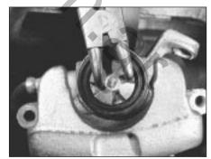
14B.28 Rotating a rear caliper piston
