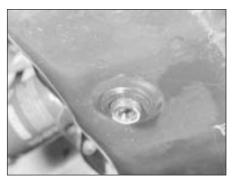
2.6 Engine sump drain plug
