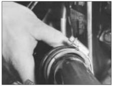
9C.55A Disconnecting the duct from the air cleaner
