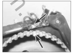
28.4 Camshaft sprocket alignment marks
