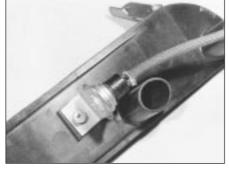
9C.79 Fan thermostatic switch on underside of injector cooling air duct (duct removed for clarity)
