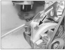
4.2B Alternator adjuster bolt
