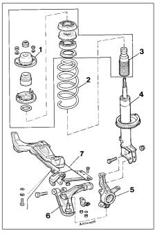
Fig. 11.3 Front strut components (Sec 3)
