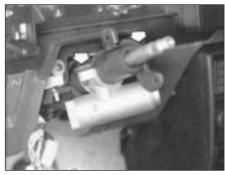
Fig. 10.9 Steering column lock shear bolts (arrowed) (Sec 9)
