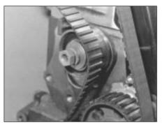
28.8 Slipping timing belt onto tensioner pulley
