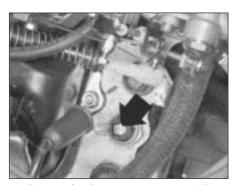
Fig. 1.9 Coolant temperature switch (Sec 13)
