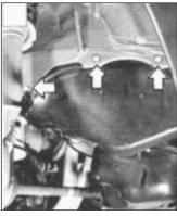
Fig. 13.22 The underwing shield retaining clips (arrowed) on the 1372 cc ie and Turbo ie engines (Sec 7C)
