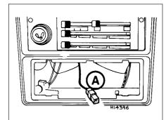
Fig. 9.8 Radio housing and power lead (A) (Sec 30)
