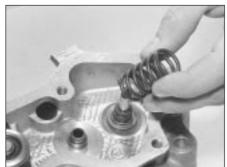
7B.130G  $\dots$  the inner spring  $\dots$
