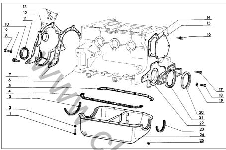
Fig. 1.23 Timing cover, sump pan and oil seals (Sec 16)
