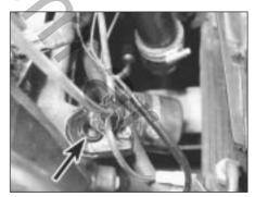
6B.22 Distributor drive hole cover plate (arrowed)
