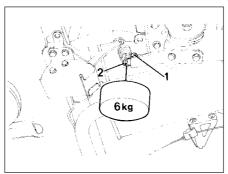
Fig. 8.10 Weight attachment point for pressure regulating valve adjustment (Sec 10)
