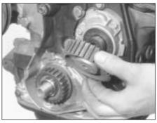
7B.45 Withdrawing the auxiliary shaft sprocket
