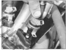
9C.80B Fuel injector removal
