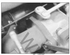
9F.16B Unscrewing turbocharger-toexhaust manifold nut
