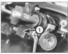
11.4 Unscrewing steering column switch clamp nut
