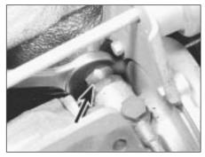
9F.18A Releasing turbocharger coolant inlet union (arrowed)
