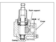
Fig. 10.5 Sectional view of rack damper (Sec 7)
