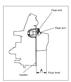
Fig. 13.36 Float level measurement -Weber 32 TLF carburettor (Sec 9B)
