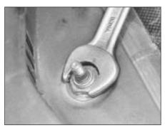
15.95 Unscrewing the wiper pivot nut
