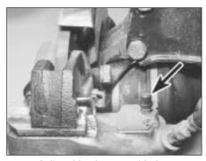
12.8 Caliper bleed screw with dust cap fitted
