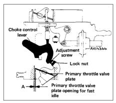
Fig. 3.25 Fast idle adjustment diagram (Weber 30/32 DMTR 90/250) (Sec 14)
