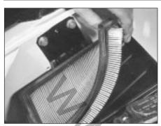
9C.27B Removing the air cleaner element
