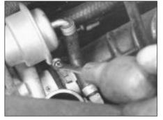
9F.17 Releasing turbocharger air hose clip
