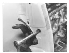
28.10 Tightening timing belt cover nut
