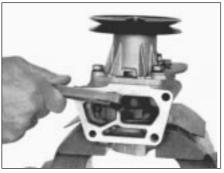
Fig. 2.6 Checking impeller clearance (Sec 9)
