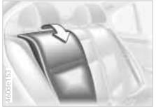
The rear backrest section will move forward slightly when it is unlocked. Reach into the gap and pull the backrest down.
