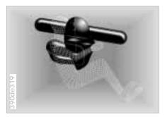
Deceleration sensors continuously monitor the acceleration forces acting upon the vehicle. If, as the result of a frontal collision, a deceleration is reached at which the protection of the safety belts alone is no longer adequate, the gas generators of the driver and passenger-front airbags are ignited. However, the passenger-side airbag is only triggered if an additional sensor has recognized that the passenger seat is occupied.
