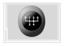
The shift lever's neutral plane (dot in the illustration) is located between 3rd and 4th gears.
