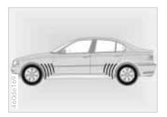
Near every wheel is an antenna in the body that receives the signal from the wheel. A central electronics system evaluates the quadruple signals and forwards any changes.
