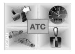
On vehicles with an automatic transmission, the ATC (Adaptive Transmission Control) uses a number of factors to calculate the gear which provides the maximum efficiency. In this process, it considers your individual driving style as well as current driving conditions.
