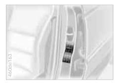
The inflation pressures are indicated on a sticker attached to the door pillar behind the driver's door (visible with door open).
