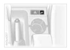
Use this button to operate the central locking system when the front doors are closed. The doors and luggage compartment lid are unlocked or locked only. The antitheft alarm system is not activated.
