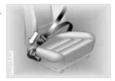
The safety belt tensioner responds to severe collisions by tightening the belts to ensure that occupants remain firmly positioned in their seats. A gas-pressure system retracts the buckle assembly to tension the shoulder and lap belts within fractions of a second. This reduces the tendency to slide under the lap belt.
