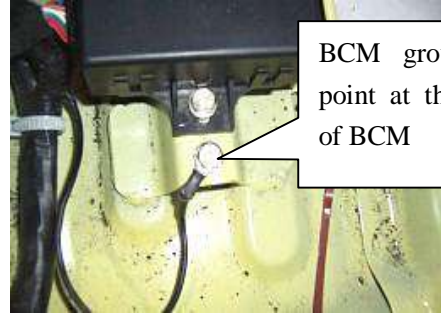
Grounding point of interior harness under the left A post.
