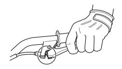
The pivoting points of the front and rear brake levers must be lubricated at the intervals specified in the periodic maintenance and lubrication chart.
