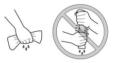
Apply oil of the recommended type to the entire surface of the sponge material, and then squeeze the excess oil out.
