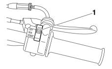
1. Engine stop switch "OFF/RUN/START"
