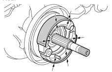
If the lining thickness of a brake shoe is less than 1.5 mm (0.06 in), have a Yamaha dealer replace the brake shoes as a set.
