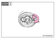
Release the bulb retaining spring.
