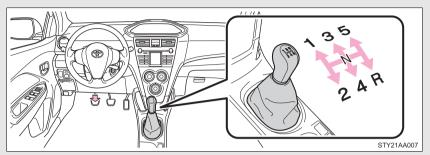
Fully depress the clutch pedal before operating the shift lever, and then release it slowly.
