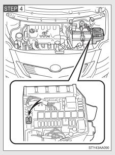
Remove the fuse with the pullout tool.
