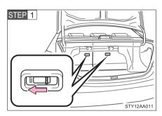
Vehicles with split rear seats: Move the security lock levers to lock the rear seatbacks.
