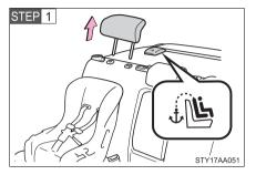
Remove the head restraint.
