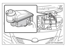
The brake fluid level should be between the MAX and MIN lines. on the reservoir.
