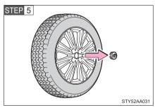
Vehicles with an aluminum wheels, remove the center wheel ornament by pushing from the reverse side.
