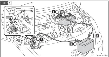
Connecting the jumper cables
