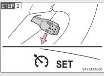
Accelerate or decelerate to the desired speed and push the lever down to set the cruise control speed.
