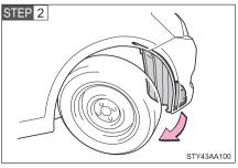
Partly remove the fender liner.
