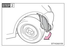
Partly remove the fender liner.
