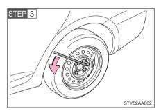
Slightly loosen the wheel nuts (one turn).
