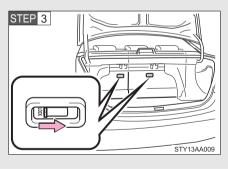
Check that the security lock levers in the trunk are in unlock position.
