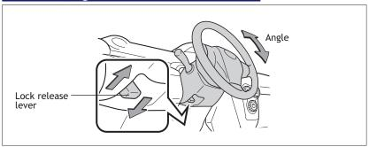
Hold wheel, push lever down, set angle and return lever.
