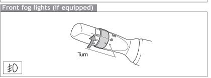
Front fog lights turn on only when the headlights are on low beam.
