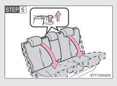
Fold the seatbacks down while pulling the seatback lock release knobs.
