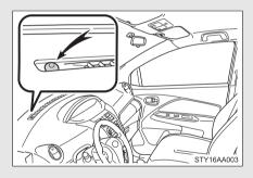
Close the doors, trunk and hood, and lock all doors using the key (vehicles without wireless remote control) or wireless remote control door lock function (vehicles with wireless remote control). The system will be set automatically after 30 seconds.
