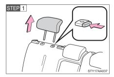
Remove the head restraint.
