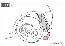
Partly remove the fender liner.
