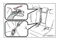
Tilt the rear seatback up until it locks, making sure that you hold the seat belt to prevent it from getting caught between the seatback and the inner side of the vehicle.
