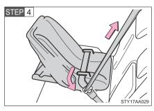
While pushing the child seat down into the rear seat, allow the shoulder belt to retract until the child seat is securely in place.
