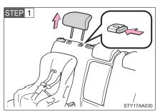
Remove the head restraint. Place the child seat on the seat facing the front of the vehicle.
