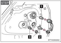
Partly remove the cover and turn the bulb bases counterclockwise.
