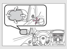
Adjust the mirror up, down, in or out using the lever.
