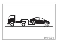
Vehicles with an automatic transmission: Use a towing dolly under the front wheels.
