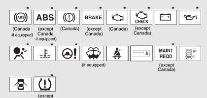
\*: These lights turn on when the engine switch is turned to the ON position to indicate that a system check is being performed. They will turn off after the engine is started, or after a few seconds. There may be a malfunction in a system if a light does not come on, or if the lights do not turn off. Have the vehicle inspected by your Toyota dealer.
