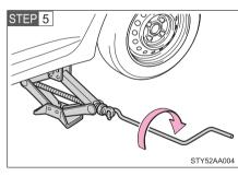
Raise the vehicle until the tire is slightly raised off the ground.
