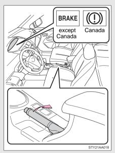
Fully set the parking brake while depressing the brake pedal.
