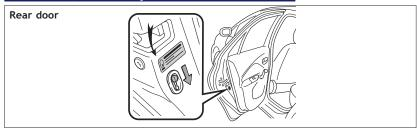
Moving the lever to "LOCK" will allow the door to be opened only from the outside.
