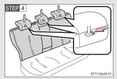
Lower each head restraints while pushing the lock release button.
