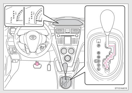
While the engine switch is on, depress the brake pedal and move the shift lever.
