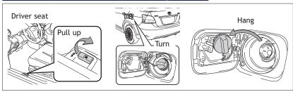
**NOTE:** Tighten until one click is heard. If the cap is not tightened enough, Check Engine "  $\Box$  " indicator may illuminate.
