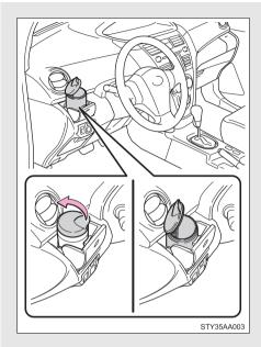
The ashtray can be installed in a cup holder. ( $\rightarrow$ P. 196)
