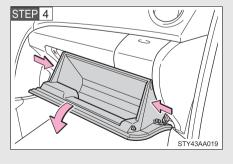
Push in each side of the glove box to disconnect the claws.
