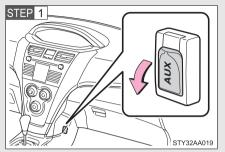
Connect the portable audio device.
